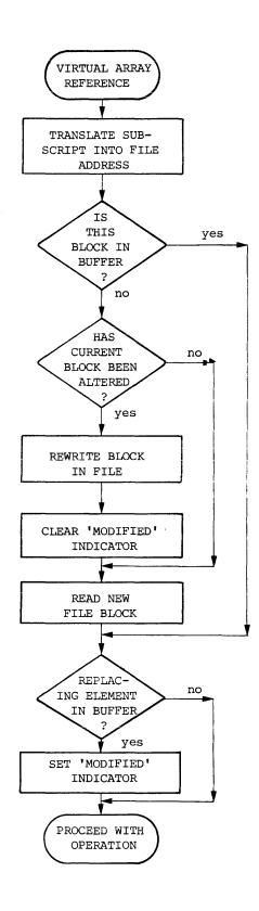
Figure C-1 Virtual Array Accessing Algorithm
