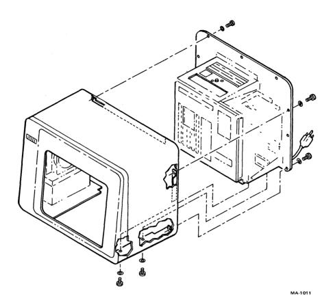
Figure 2-12 RT805 Disassembly for Option Modules Installation
