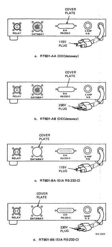
Figure 1-16 RT801 Connector Panel Configurations
