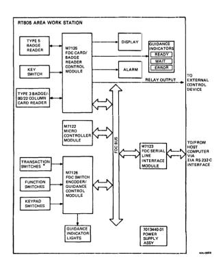
Figure 1-21 RT805-BA/BB (EIA RS-232-C) - Block Diagram
