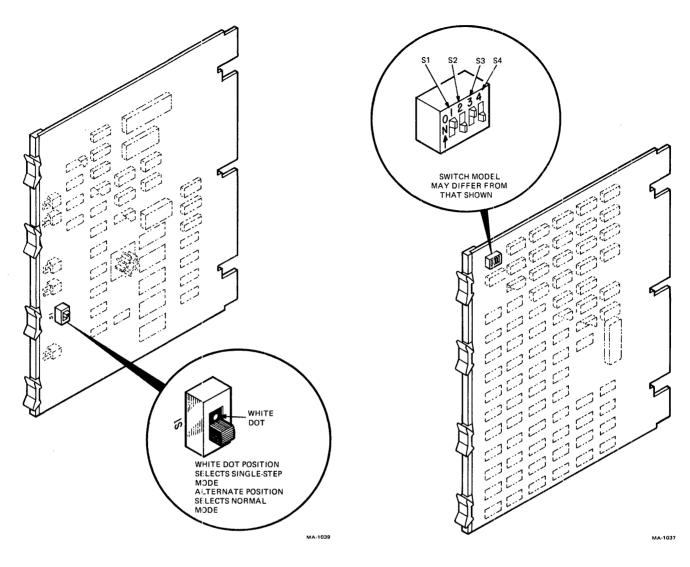
Figure 4-1 M7122 Normal/Single-Step Switch
