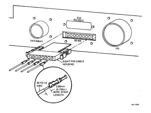
Figure 2-15 20 mA Cable Assembly Details
