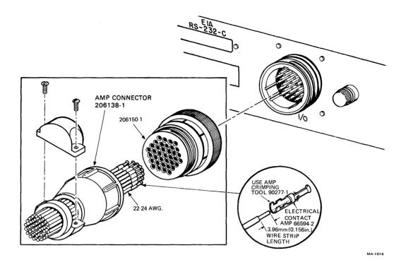
Figure 2-20 User-Fabricated I/O Cable Assembly Details
