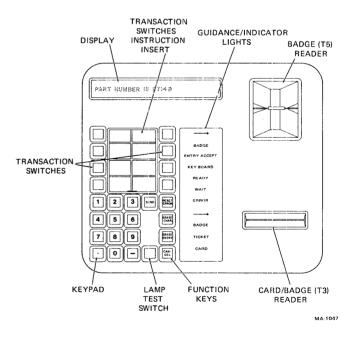
Figure 3-4 RT805 Controls and Indicators
