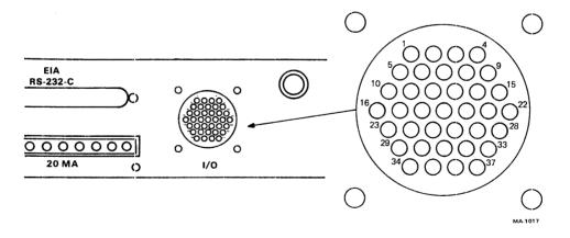
Figure 2-19 I/O Connector Pin Designations
