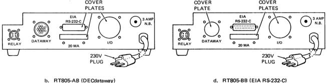
Figure 1-22 RT805 Basic Model Connector Panel Configurations
