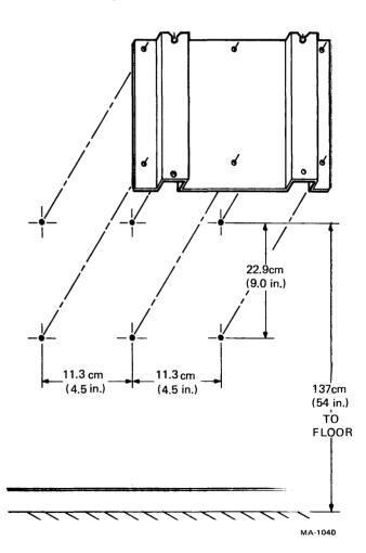
Figure 2-2 Wall-Mount Hole Location Data
