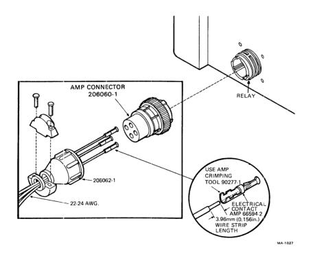
Figure 2-4 External Control Circuit Connector Details
