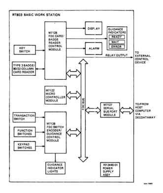
Figure 1-17 RT803-AA/AB (DECdataway) - Block Diagram
