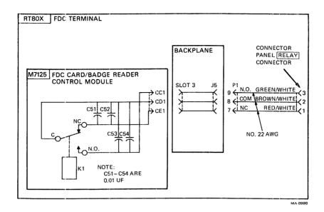
Figure 2-3 External Control Circuit - Schematic Diagram
