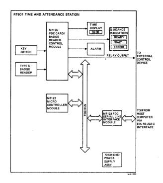
Figure 1-15 RT801-BA/BB with EIA RS-232-C Interface --Block Diagram
