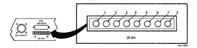
Figure 2-14 20 mA Connector Pin Designations
