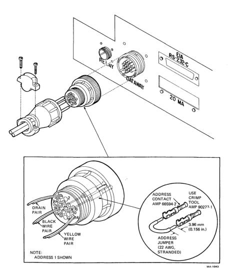
Figure 2-5 DECdataway Connector Addressing Details
