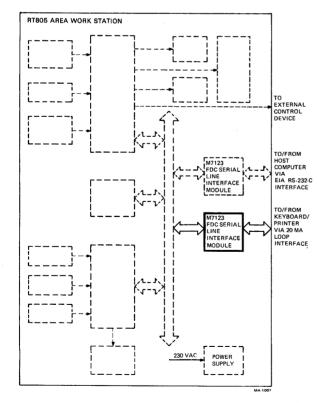
Figure 1-26 RT805-BA/BB (EIA RS-232-C) with XC (20 mA) Option — Block Diagram
