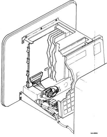
Figure 2-17 RT805-XD (Digital I/O) Option Location
