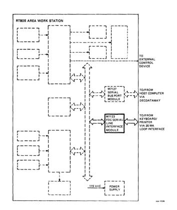
Figure 1-23 RT805-AA/AB (DECdataway) with XC (20 mA) Option -- Block Diagram
