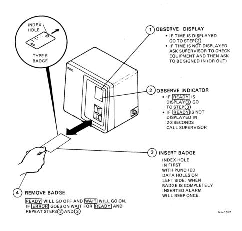
Figure 3-5 Typical RT801 Operating Procedure
