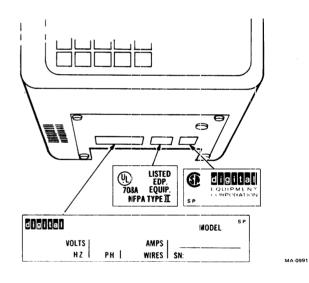
Figure 1-13 Electrical Data Plates
