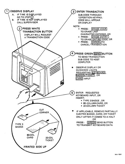
Figure 3-6 Typical RT803 Operating Procedure
