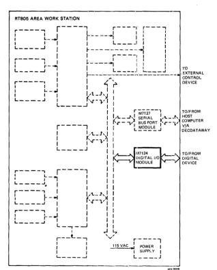
Figure 1-24 RT805-AA/AB (DECdataway) with XD (I/O) Option – Block Diagram
