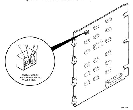
Figure 2-13 Baud Rate Switch Details
