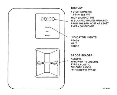
Figure 1-7 RT801 Operator's Panel
