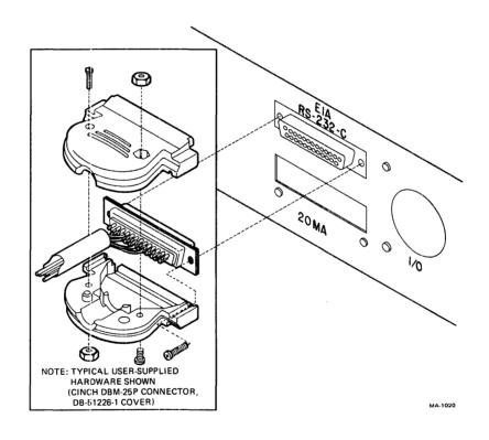
Figure 2-7 Typical EIA RS-232-C Cable Connection
