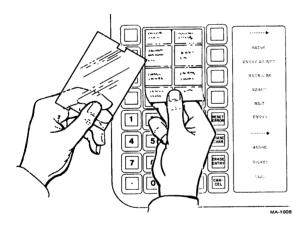
Figure 1-11 RT805 Transaction Switches Instruction Insert
