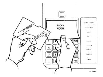
Figure 1-10 RT803 Transaction Switch Instruction Insert
