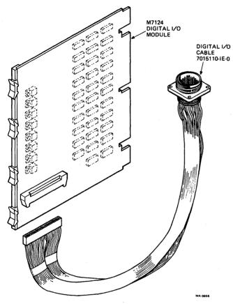
Figure 2-16 RT805-XD (Digital I/O) Option Kit
