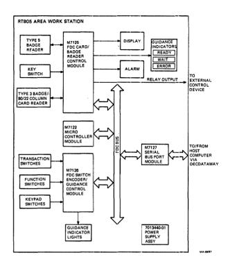
Figure 1-20 RT805-AA/AB (DECdataway) - Block Diagram
