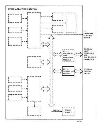
Figure 1-27 RT805-BA/BB (ÈIA RS-232-C) with XD (I/O) Option — Block Diagram
