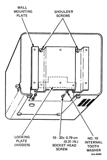
Figure 2-1 Wall-Mounting Hardware Details
