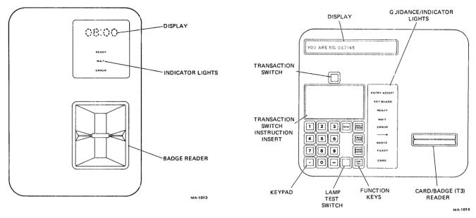
Figure 3-1 RT801 Controls and Indicators
