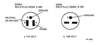
Figure 1-12 Power Plug Configurations
