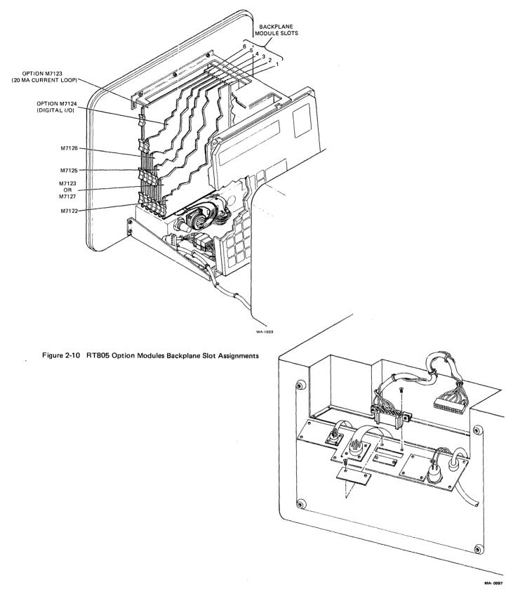
Figure 2-11 RT805-XC (20 mA Current Loop) Cable Installation
