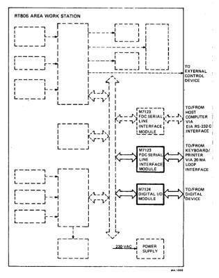
Figure 1-28 RT805-BA/BB (EIA RS-232-C) with XC (20 mA), XD (I/O) Options – Block Diagram
