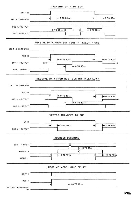
Figure B-8 DC005 Timing Diagram
