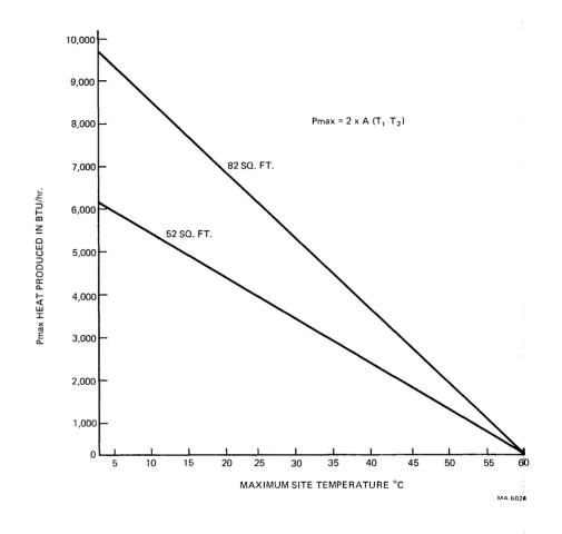
Figure 2-2 Cabinet Heat vs Site Temperature
