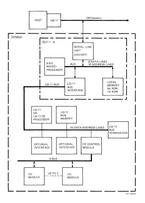
Figure 1-3 The ISV11-A in a DPM50 Subsystem
