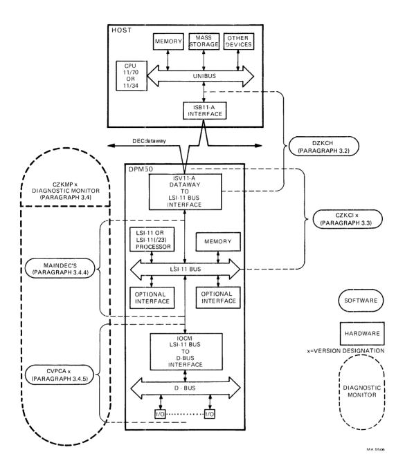
Figure 3-1 DPM50 Maintenance Software / Firmware Hierarchy
