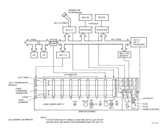
Figure 1-4 DPM50-Ax, -Cx Physical Layout
