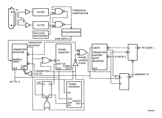
Figure 4-3 Receiver Simplified Block Diagram
