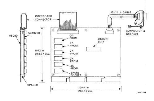
Figure 2-3 ISV11-A Physical Configuration
