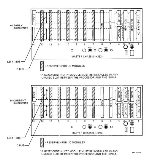
Figure 2-6 DPM50-AA, -AB, -CA, -CB, LSI-11 Module Placement
