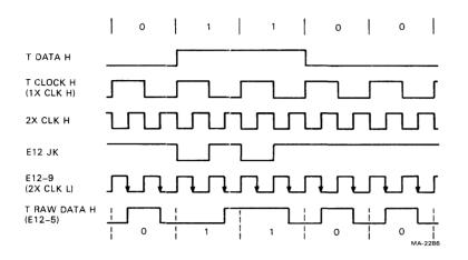
Figure 4-2 Transmitter Timing
