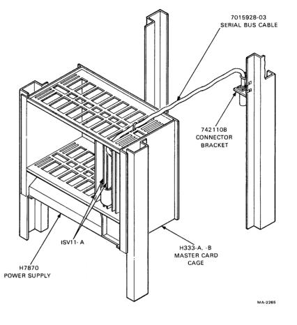
Figure 2-1 DECdataway Connector Mounting
