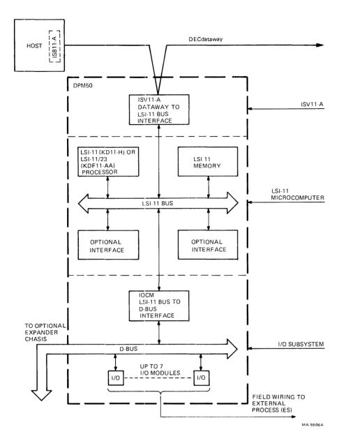
Figure 1-2 DPM50 Detailed Functional Diagram
