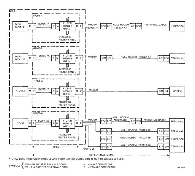
Figure 2-8 DPM50 Serial Line Filter Configuration - EIA (RS232C)
