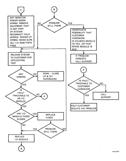
Figure 3-7 Troubleshooting Flowcharts Chart 2 DPM50 Subsystem Procedure, Part B
