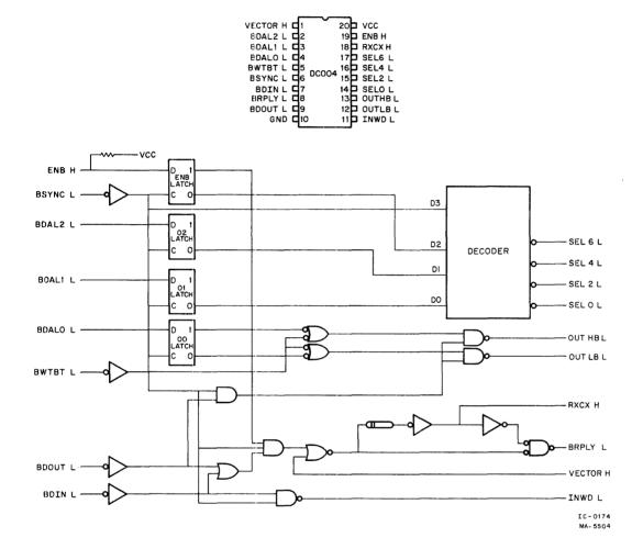
Figure B-4 DC004 Simplified Logic Diagram
