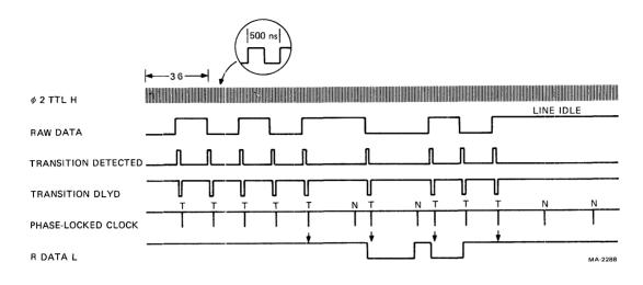
Figure 4-4 Receiver Timing
