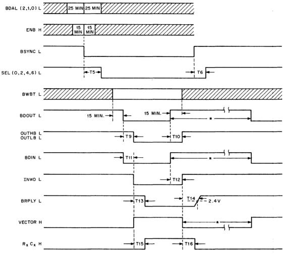
\* TIME REQUIRED TO DISCHARGE  $R_x C_x$  FROM ANY CONDITION ASSERTED = 150 ns
