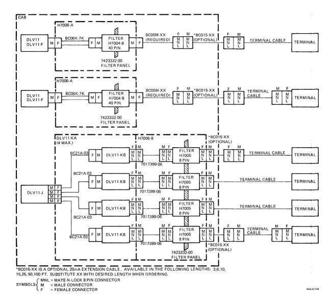
Figure 2-9 DPM50 Serial Line Filter Configuration – 20 mA Current Loop
