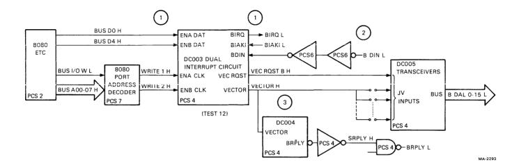
Figure 4-9 ISV11-A Interrupt Request To LSI-11
