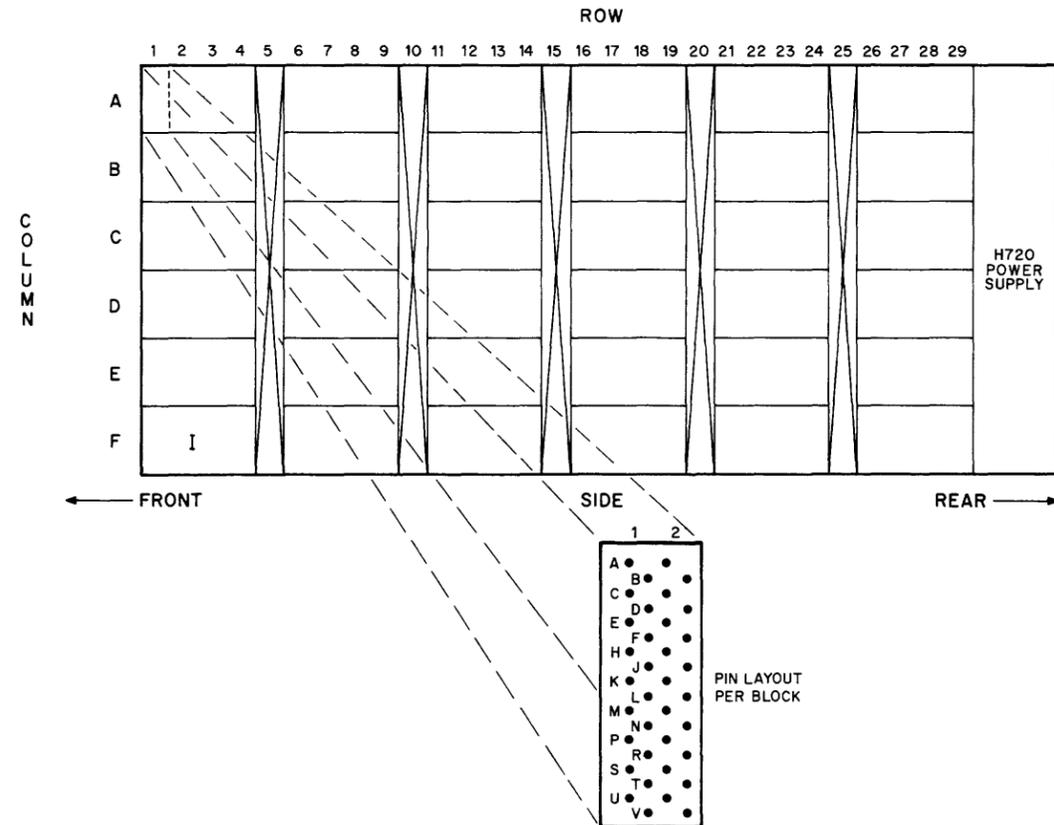
Figure A-1 Typical System Layout
