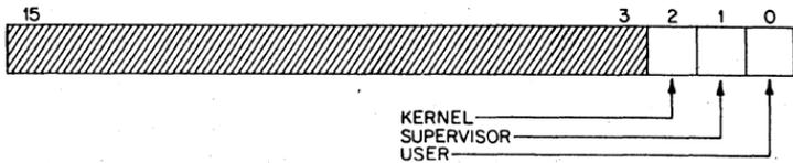
Figure 10-10 Format of Status Register #3 (SR3)
