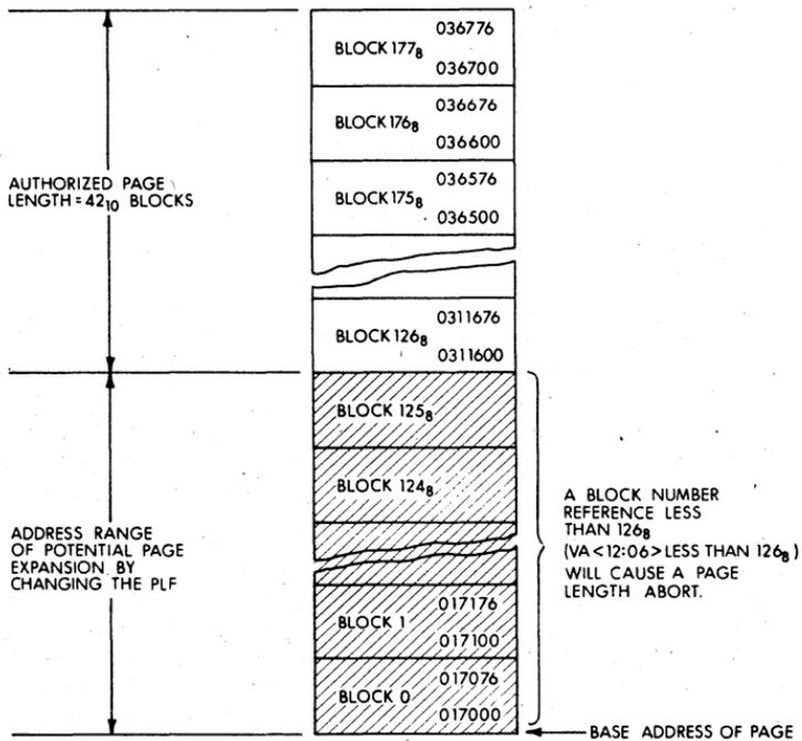
Figure 8-7 Example of a Downward Expandable Page
