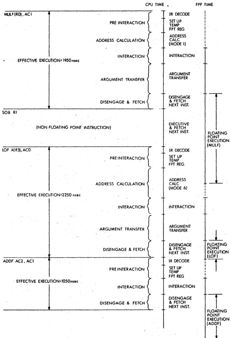
Figure B-3 Calculation of Effective Execution Times for Load Class Instructions
