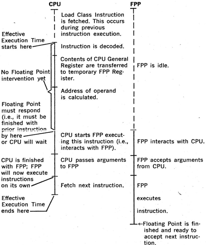
Figure B-1 Load Class Floating Point Instruction.
