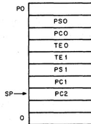
6. Subroutine A is running and uses stack for temporary storage.
