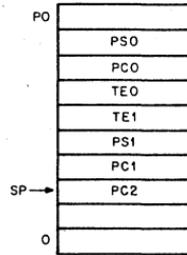
8. Subroutine A returns control to process 2 with an RTS R7,PC is reset to PC2.
