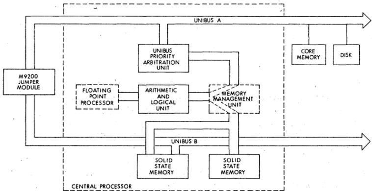
Figure 9-1 PDP-11/55, PDP-11/45 System Block Diagram
