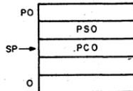
11. Process 1 completes its operation with an RTI, PC is reset to PC0, and status is reset to PS0.
