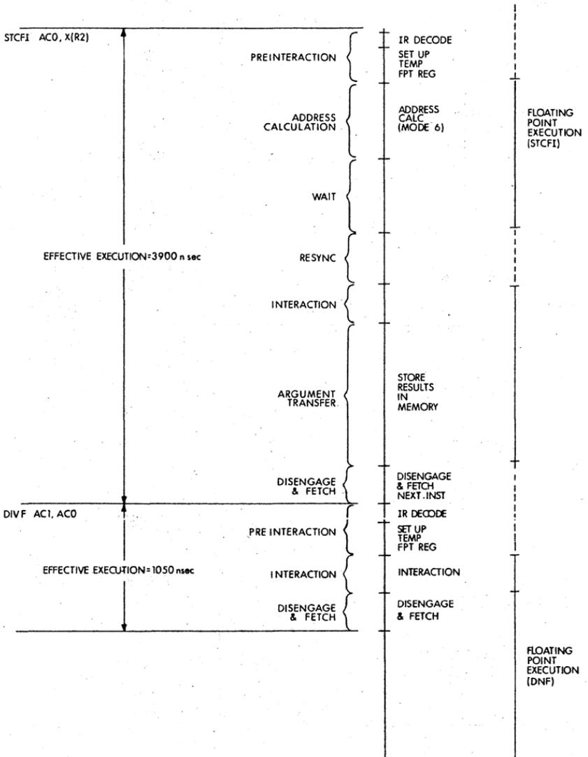
Figure B-4 Calculation of Effective Execution Time for Store Class Instructions
