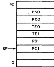
9. Process 2 completes with an RTI instruction (dismisses interrupt) PC is reset to PC(1) and status is reset to PS1; process 1 resumes.
