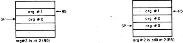
Figure 5-13: Constant Index Base Using "R6 Copy"
