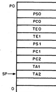
7. Subroutine A releases the temporary storage holding TA1 and TA2.
