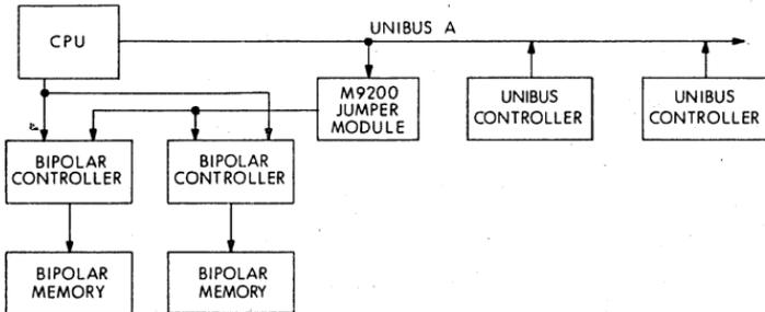
4. The two MS11 solid state memory controls are connected to a single UNIBUS (UNIBUS-B) that can be easily separated from the 11/45 CPU UNIBUS (UNIBUS-A) by removing a simple jumper module (M9200), thus facilitating dual UNIBUS systems. UNIBUS B does not have its own Unibus arbitration control logic; thus, a second PDP-11 CPU is required for other than NPR transfers from a single device.
