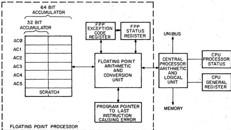
Figure 11.1 Floating Point Processor
