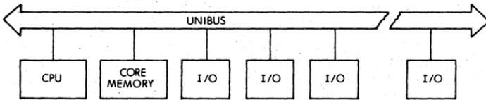
Figure 2-1 PDP-11 System Simplified Block Diagram
