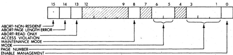
**Figure 8-11 Format of Status Register #0 (SR0)**
