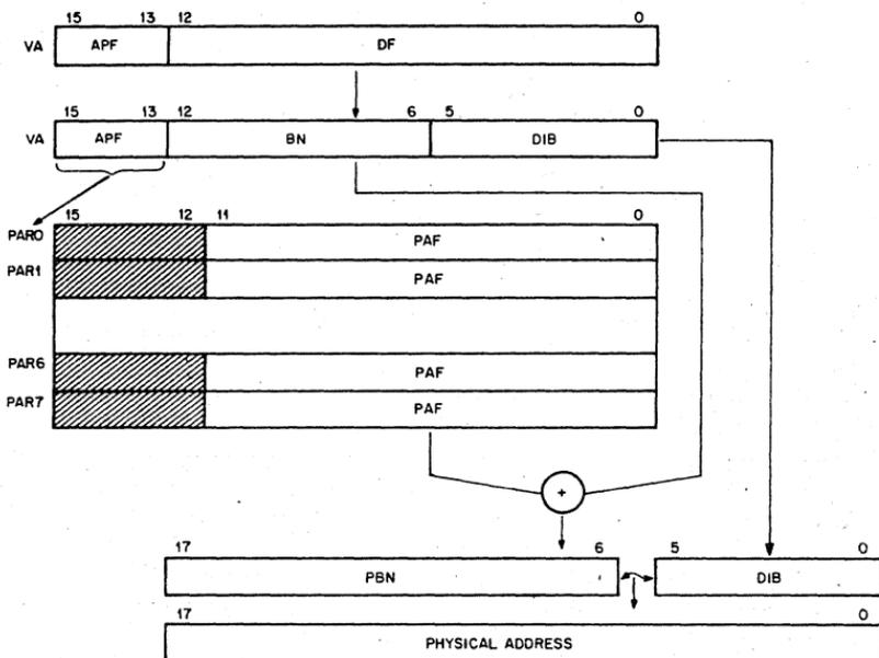
Figure 10-4 Construction of a Physical Address
