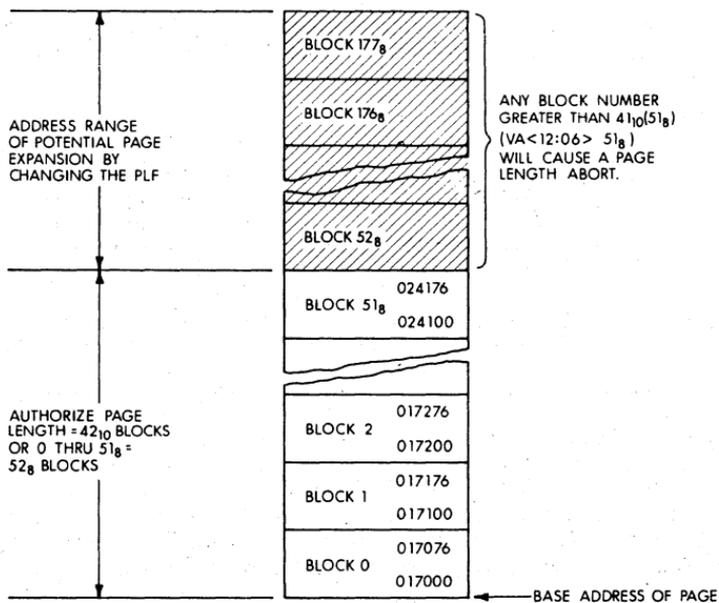
Figure 8-6 Example of an Upward Expandable Page
