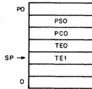
4. Process 1 interrupted with PC = PC1 and status = PS1; process 2 is started
