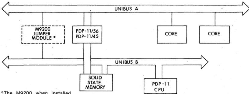
\*The M9200 when installed, connects Unibus A to Unibus B. If two CPU's are utilized, the M9200 must be removed.
