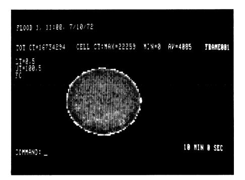
Figure 9-2 Resulting Flood Correction Matrix (M=50%)
