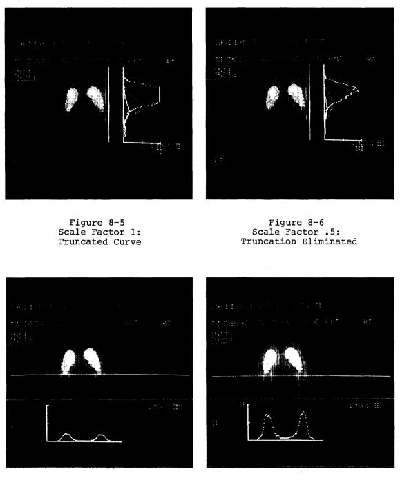
Figure 8-7 Scale Factor 1: Low Contour Curve Figure 8-8 Scale Factor 2: Contour Enhanced .
