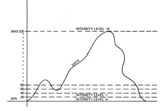
The data acquired under count change 20 is at intensity level 1. Data between 20-40 is at intensity level 2, 40-60 is at 3, etc. The data at level 300-320 has the highest intensity level, 15. Please note that data acquired at count change 0 is at intensity level 0. Therefore, the 16 levels of intensity range from 0 to 15.
