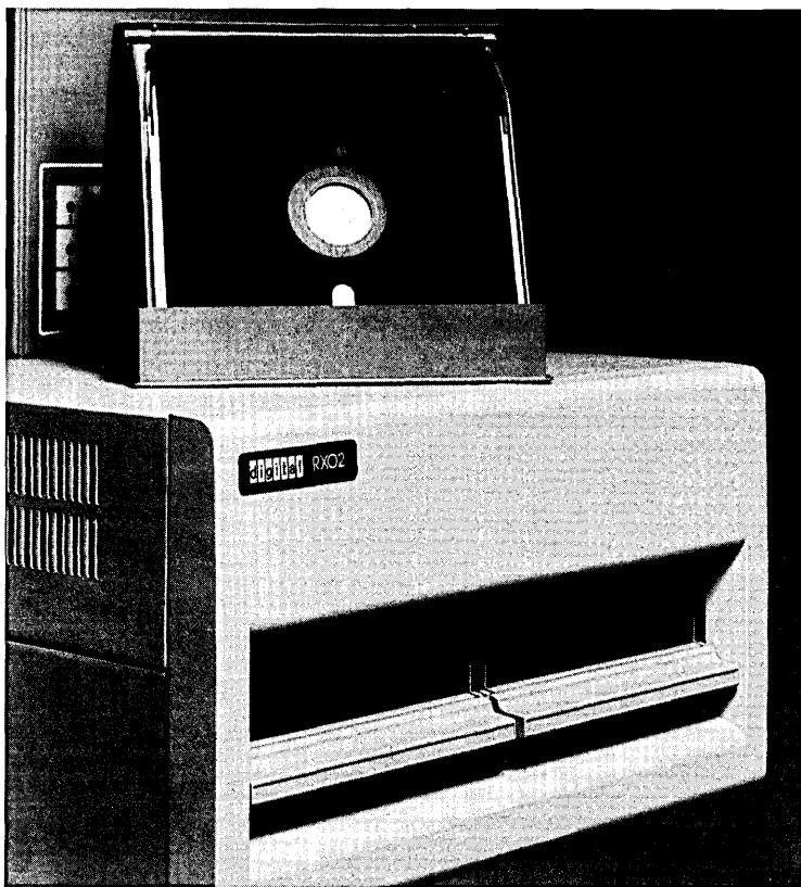
The RX02 double-density floppy disk drive provides an industry-compatible format and highly reliable operation. Direct memory access (DMA) is used to provide rapid data transfer and efficient utilization of the host processor. These subsystems include two RX02 0.5 MB drives (for a total of one MB) and a controller with interconnect cabling. The dual drives are packaged as a cabinet-mountable or tabletop unit.
