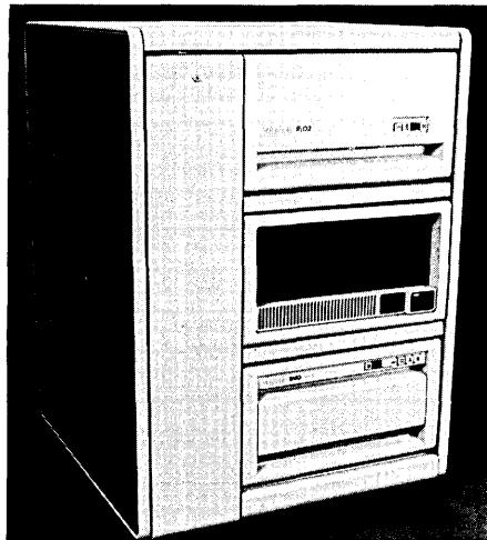
The PDP-11/24 RA80/RLO2 configuration provides all the standard features of the PDP-11/24-DC/DD box product and 121 MB fixed and 10 MB removable disk storage.
