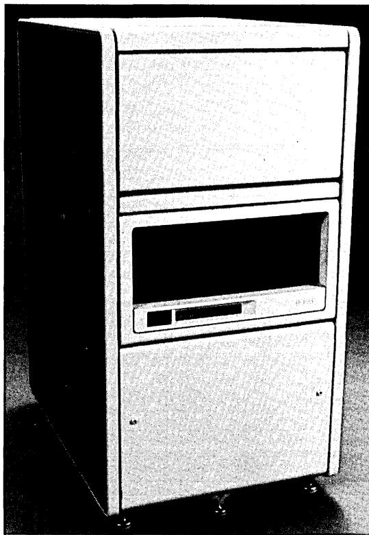
The PDP-11/44 is available in a cabinet-mounted variation. This configuration is built around the 11/44-DA(DB) box product and housed in an H9642 CPU cabinet. The kernel is intended to provide a foundation for building system configurations tailored for unique applications.
