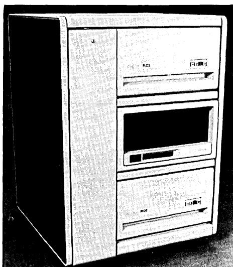
The PDP-11/44 Dual RL02 system configuration provides all the standard features of the PDP-11/44-DA(DB) and 20.8 MB of removable mass storage capacity.
