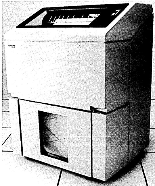
The LP27 is a 132-column, fully formed character, impact lineprinter. It includes both 64 and 96 character American print bands as standard on all versions. Maximum print throughput is 1200 lines per minute using the 64 character band or 800 lines per minute with the 96-character band.
