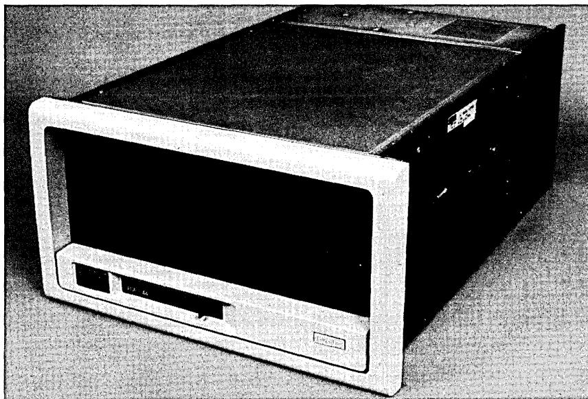
The PDP-11/44 is available in a 26.6 cm (10.5 in) rack-mountable version. It offers memory expansion up to 4 MB in the four pre-wired slots in the CPU backplane. The PDP-11/44 computer provides ample power and expansion space for configuration flexibility.
