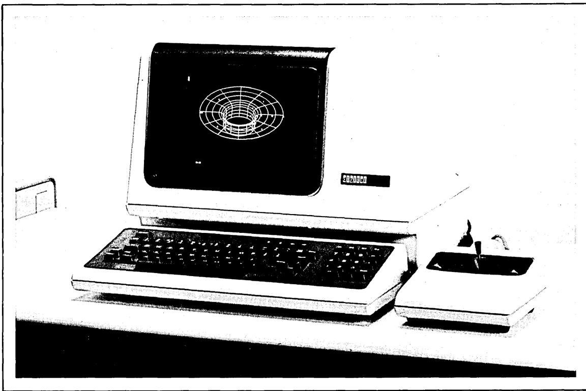
The VS11 is a high-performance, 16-color graphics system. It features a versatile graphics instruction set, bit-slice architecture, switch-selectable resolution and intensity for interlaced or non-interlaced operation.
