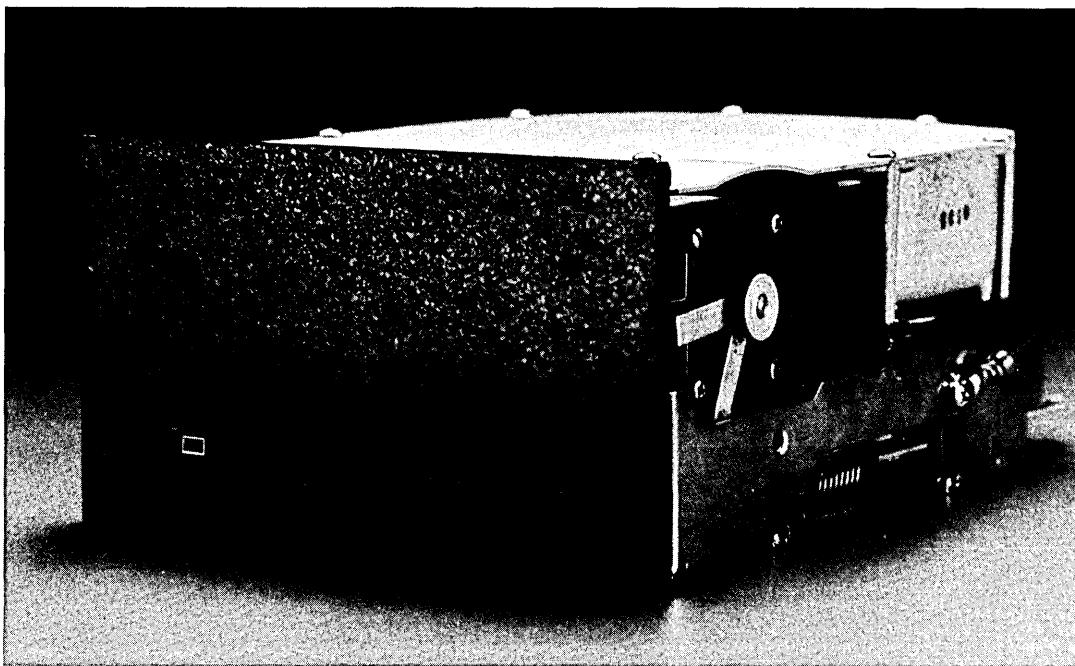
The RD51 is a 10-MB, non-removable disk drive, utilizing state-of-the-art Winchester technology. The drive mechanism is packaged in a single compact housing, which conforms to the industry standards for 5.25-in disk media. The sealed head/disk assembly (HDA) contains two platters, four read/write heads and positioning arm. The sealed HDA helps to increase drive reliability and ensure data integrity.
