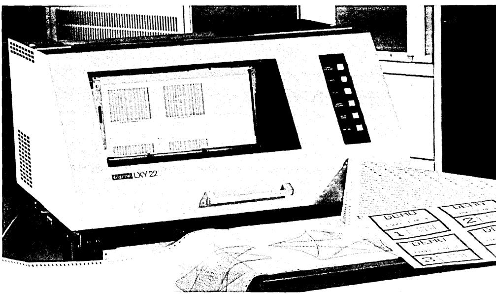
The LXY12 and LXY22 graphics lineprinters are versatile dot-matrix printers that combine the benefits of a line printer and a plotter in one product. These printers are compatible with all other Digital lineprinters, requiring no special software to use them as lineprinters.
