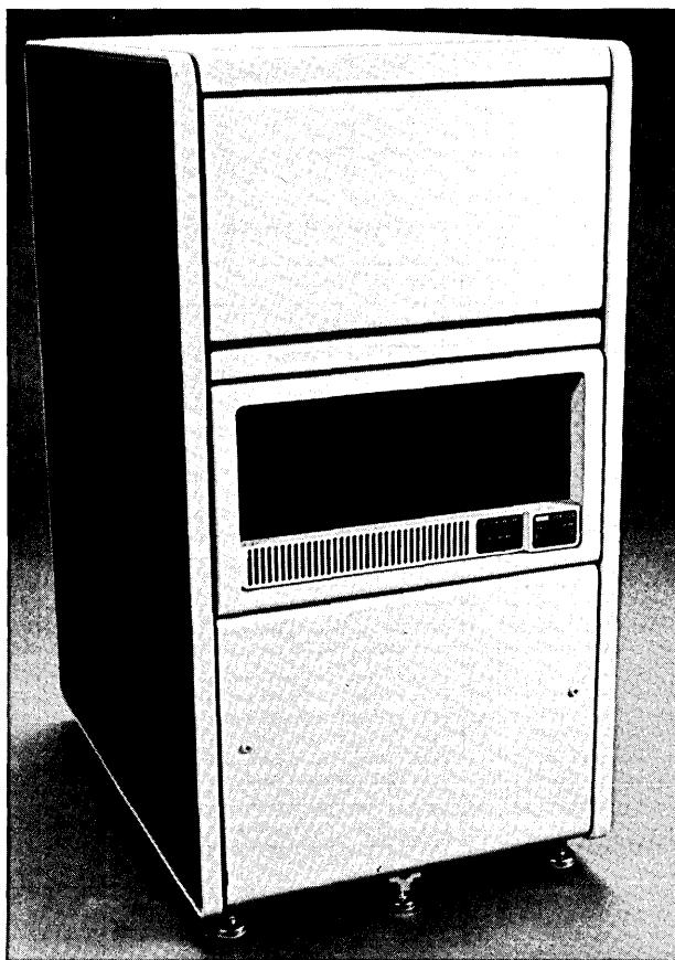
The PDP-11/24 is available in a cabinet-mounted model. It provides a foundation for building tailored system configurations and includes the 11/24-DC(DD) box product housed in an H9642 CPU cabinet.
