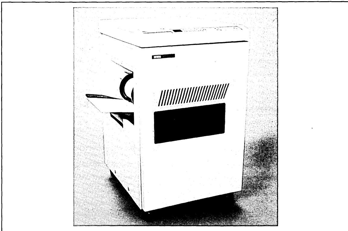
The LNO1 page printer is a high-quality nonimpact printer that employs laser technology. The LNO1 provides the speed of a lineprinter with exceptional print quality. Using electrophotographic imaging and xerographic printing, the LNO1 prints one page at a time, twelve pages per minute. The print resolution of 300 x 300 dots per square inch produces perfectly formed characters of even density and alignment. Since every page is an original, every copy is as crisp and clear as the first.
