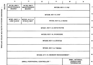
\*\* IF NO OPTION IS PRESENT IN THE SMALL PERIPHERAL CONTROLLER SLOT. A G727 GRANT CONTINUITY MODULE MUST BE INSERTED INTO ROW D.
