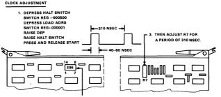
2. PLACE SCOPE PROBE ON E96 PIN 9 WHICH IS THE SECOND PIN FROM THE LEFT ON THIS IC LOOKING AT IT AS IT IS INSTALLED IN THE BACKPLANE.
