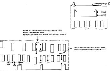
CUT W1 THROUGH W9 WHEN INSTALLING KT11-D
