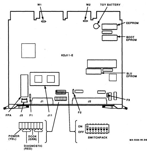
Figure 2–1 KDJ11-E Jumper and DIP Switch Locations
