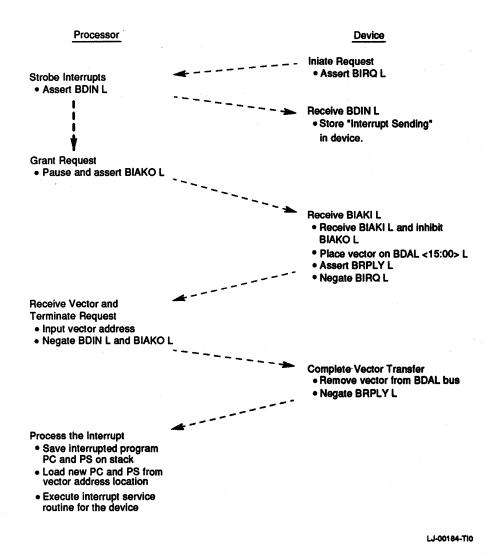
Figure 5–9 Interrupt Request/Acknowledge Sequence
