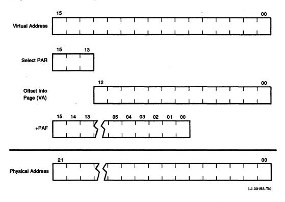
Figure 1–11 Construction of a Physical Address
