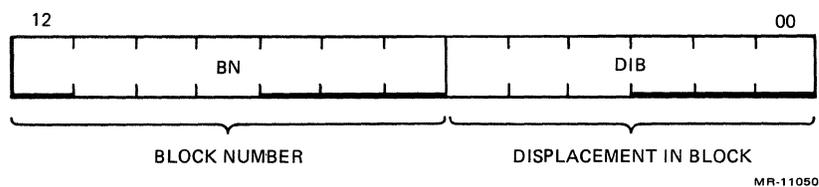
Figure 1-12 Displacement Field of a Virtual Address
