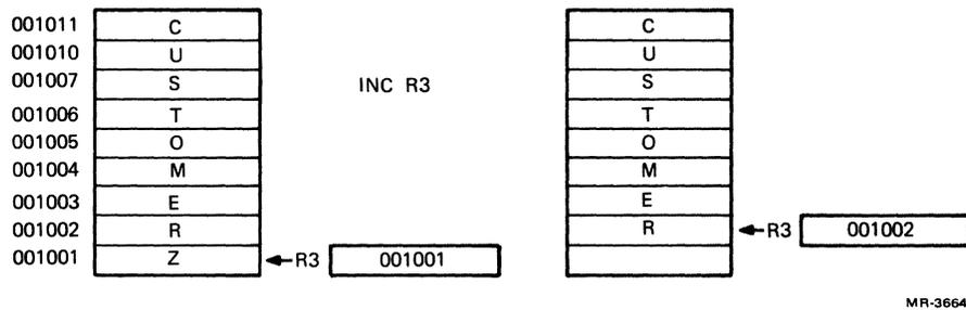
Figure 8-3 Byte Stack Used as a Character Buffer
