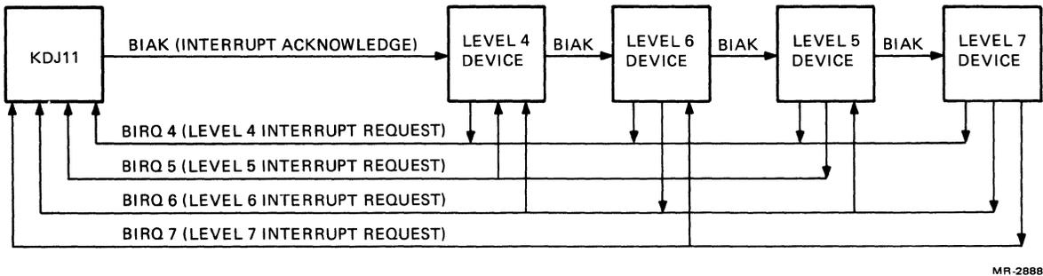
Figure 5-13 Position-Independent Configuration
