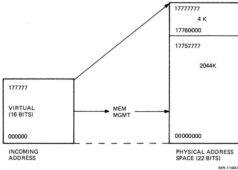
Figure 1-9 22-Bit Mapping
