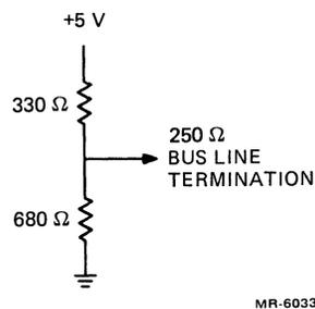
Figure 5-16 Bus Line Termination
