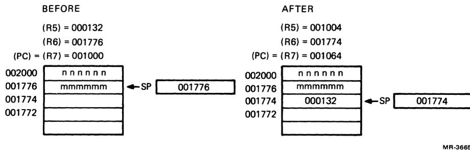
Figure 8-4 JSR Stack Condition Example
