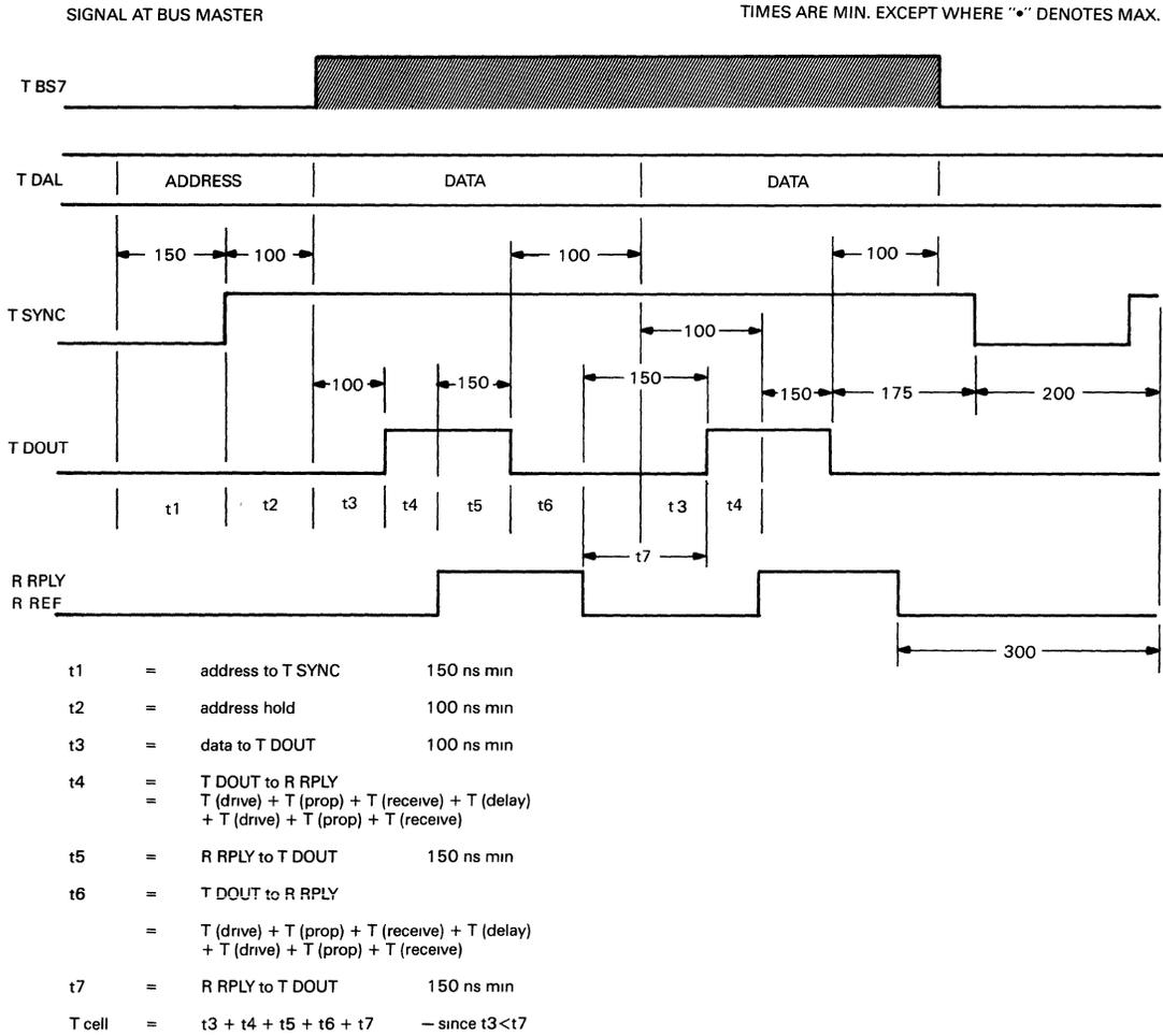
Figure 5-8 DATBO Bus Cycle Timing
