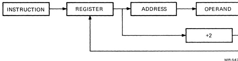
Figure 6-20 Mode 3 Autoincrement-Deferred
