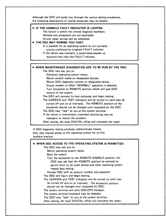
Figure 5-1 Remote Diagnosis Hardware Failure Reporting Procedure (Sheet 2 of 3)
