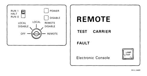
Figure 2-1 Electronic Console Panel Controls and Indicators
