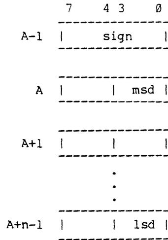
A zero length separate string occupies a single byte of memory which contains the sign. When used as a source, zero length strings provide operands with zero magnitude; when used as a destination, they can only reflect a result of zero magnitude without indicating overflow; the sign of the result is stored.
