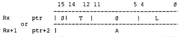
The encodings (in binary) for the NUMERIC string data type field are:
