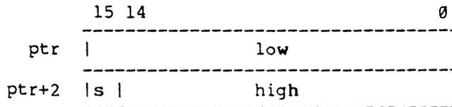
Note that these two representations of long integers differ. There is no single representation of long integer among EAE, EIS, FPP and software. The "register form" was selected to be compatible with EIS; the "in-line form" was selected to be compatible with current standard software usage.
