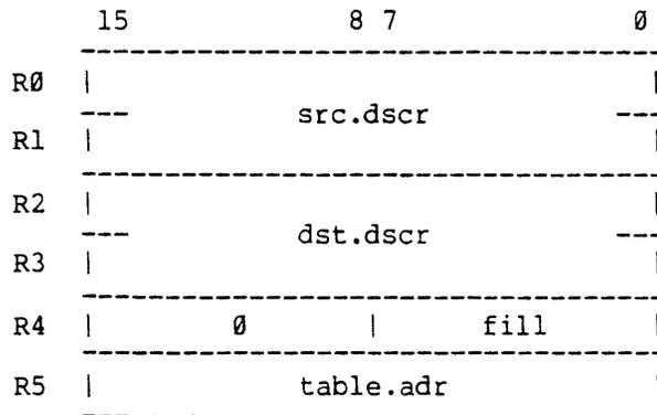
When the instruction is completed, R0 contains the number of unmoved source string characters, and R1 through R3 are cleared:
