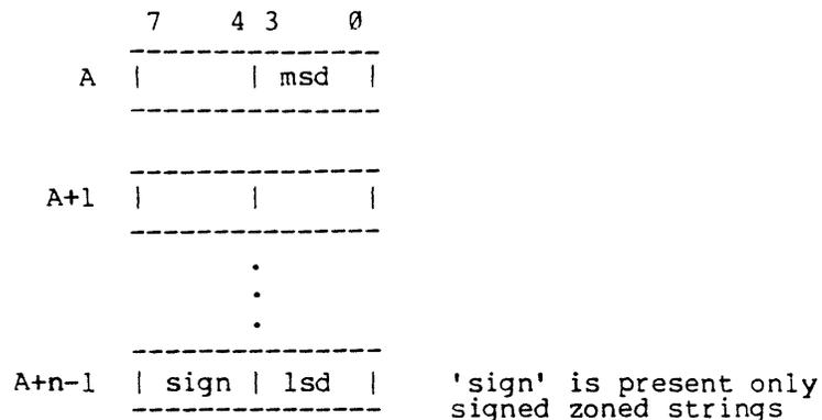
A zero length zoned string does not occupy memory; the address portion of its descriptor is ignored. When used as a source, zero length strings provide operands with zero magnitude; when used as a destination, they can only accurately reflect a result of zero magnitude (the sign of the operation is lost). An attempt to store a non-zero result will be indicated by setting overflow.
