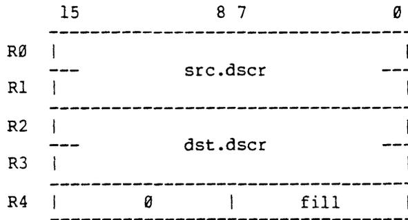
When the instruction is completed, R0 contains the number of unmoved source string characters, and R1 through R3 are cleared:
