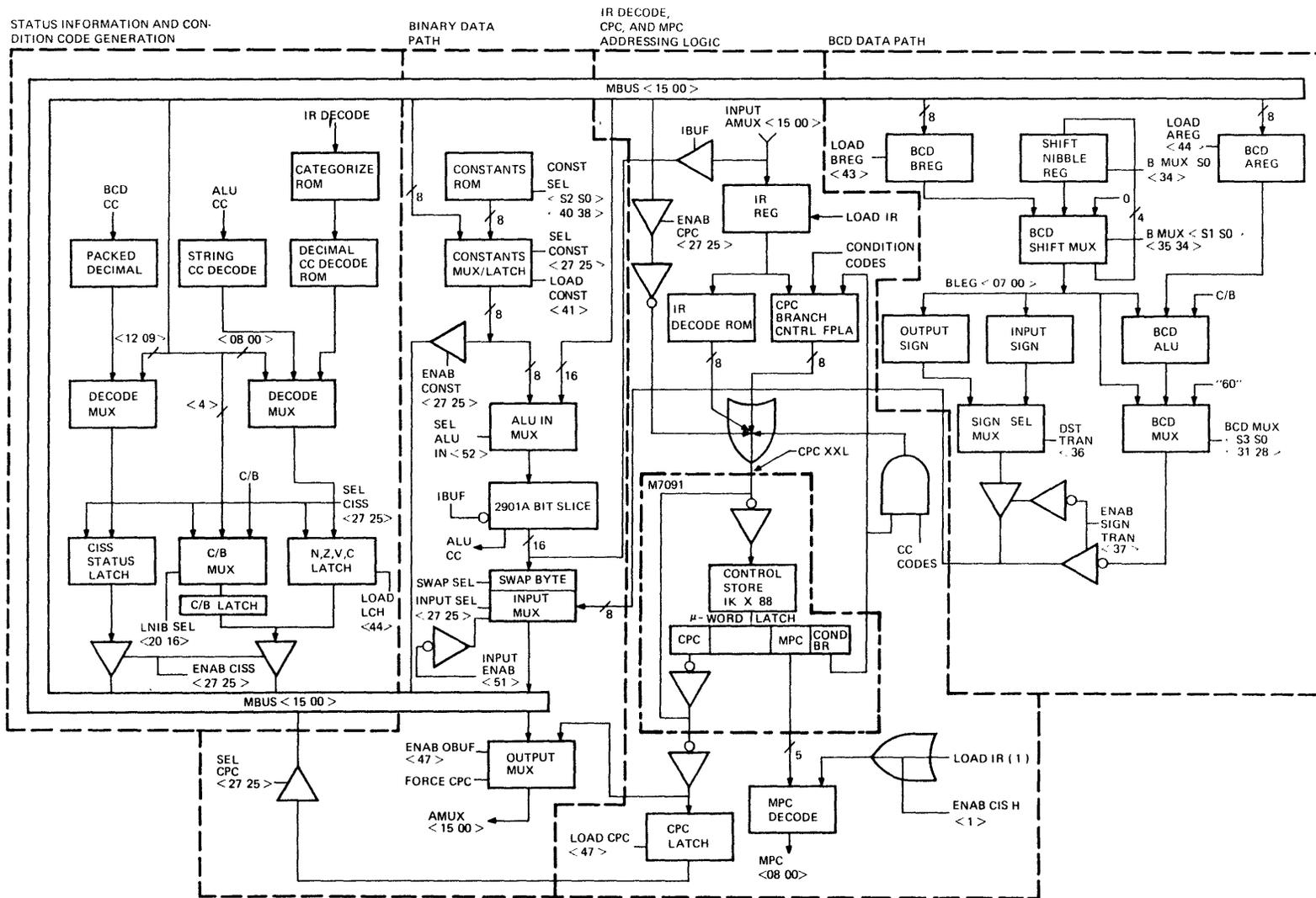
Figure 3-1 KE44-A Block Diagram
