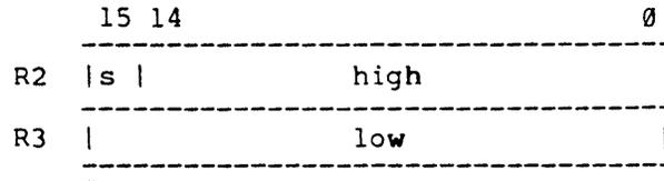
The in-line form of decimal convert instructions reference the long integer by a word address pointer which is part of the instruction stream:
