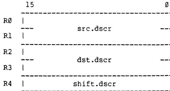
When the instruction is completed, the source descriptor registers and shift descriptor register are cleared:
