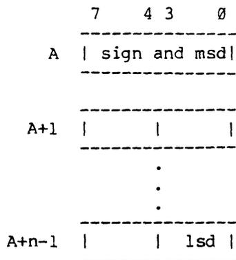
A zero length overpunch string does not occupy memory; the address portion of its descriptor is ignored. When used as a source, zero length strings provide operands with zero magnitude; when used as a destination, they can only accurately reflect a result of zero magnitude (the sign of the operation is lost). An attempt to store a non-zero result will be indicated by setting overflow.
