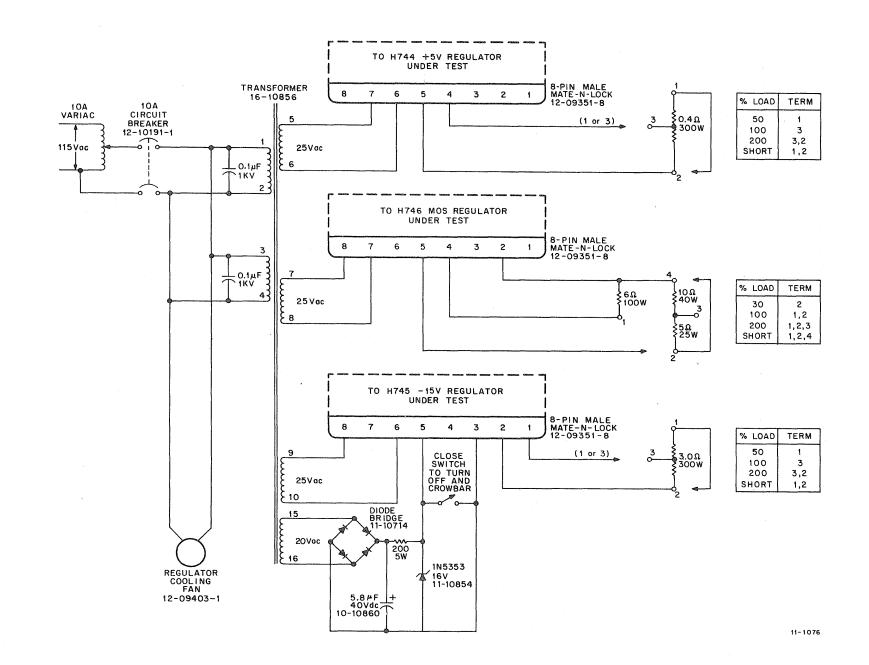
Figure 7-1 Voltage Regulator Test Bench Source and Loads
