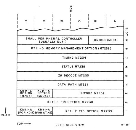
Figure 6-3 Module Allocation - KD11-A Processor, Basic (\*) and Options
