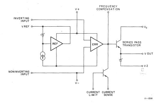
Figure 6-10 Simplified Diagram of Precision Voltage Regulator E1
