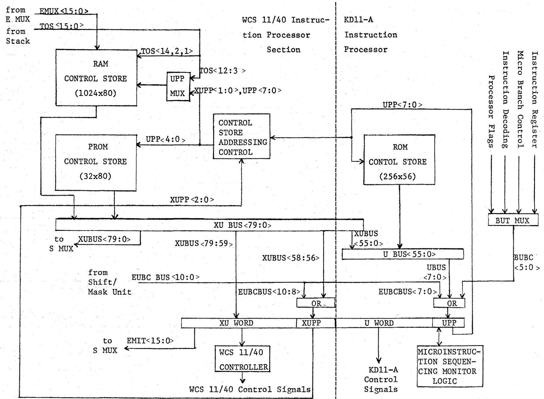
11-bit EUBC BUS into XUPP<2:0> and UPP<7:0>, respectively. Furthermore, the basic microbranch codes, BUBC, as selected by BUT MUX are Ored into UPP<5:0>.
