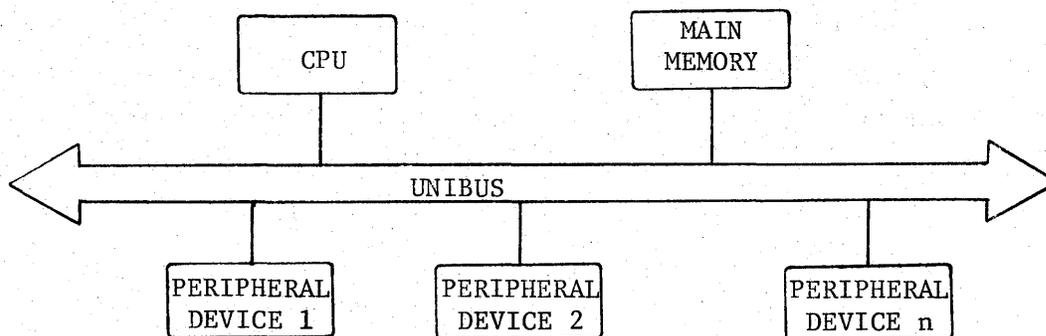
Figure 2: PDP-11 System Block Diagram
