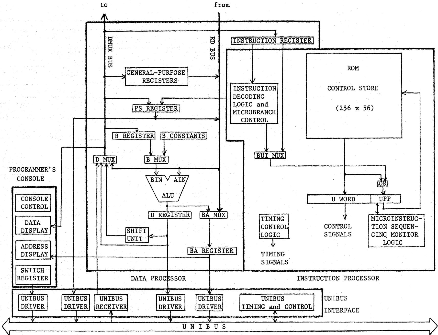
Figure 5: KD11-A Processor Register-Transfer Diagram
