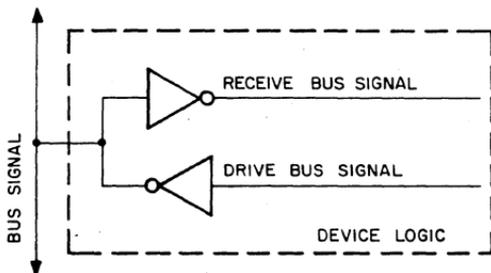
Figure 8-1 Bidirectional Nature of the Bus
