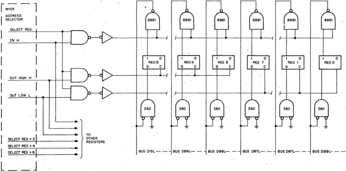
Figure 9.7 Typical Peripheral Device Register
