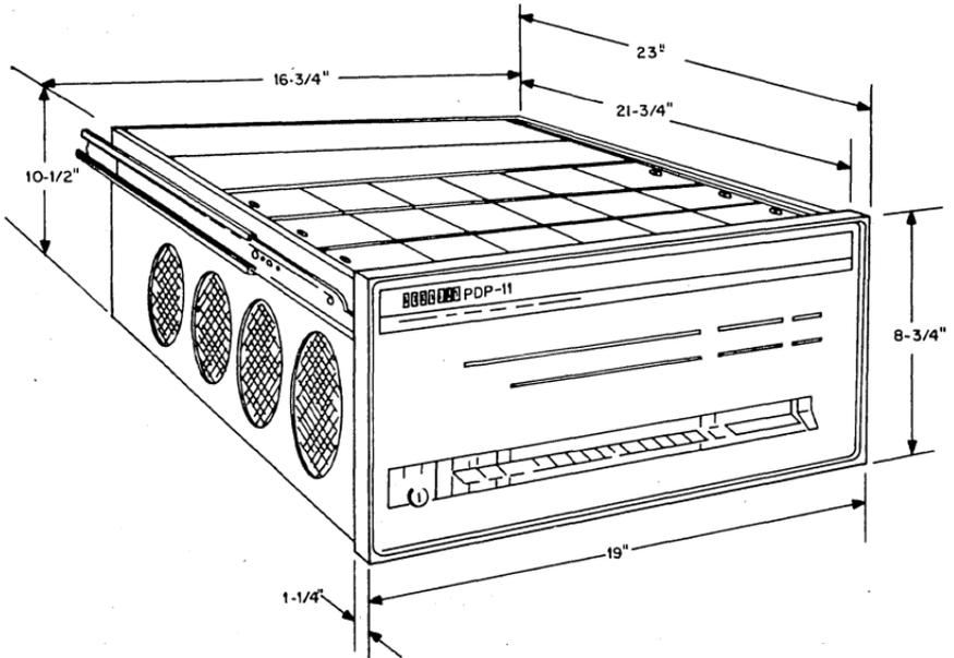
Figure 10.3 Rack Mountable PDP-11 Dimensions
