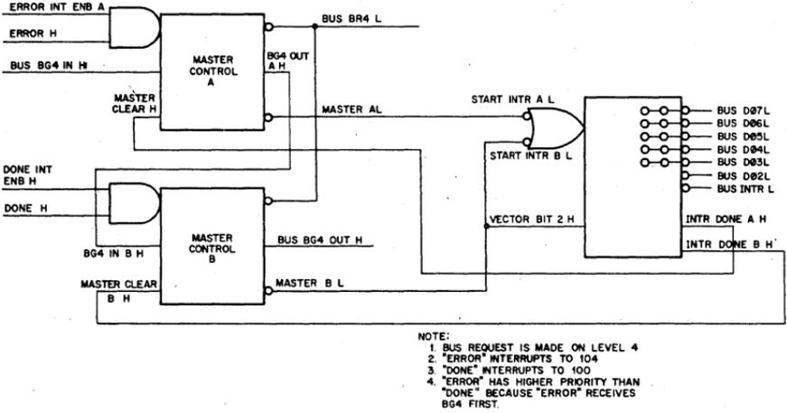
Figure 9.9 Typical Interconnection of M782 Interrupt Control
