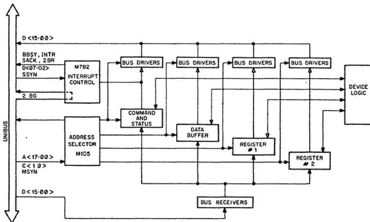
Figure 9.1 Typical Peripheral Device Interface
