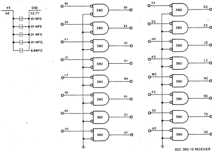
Figure 9.4 M784 Unibus Receivers
