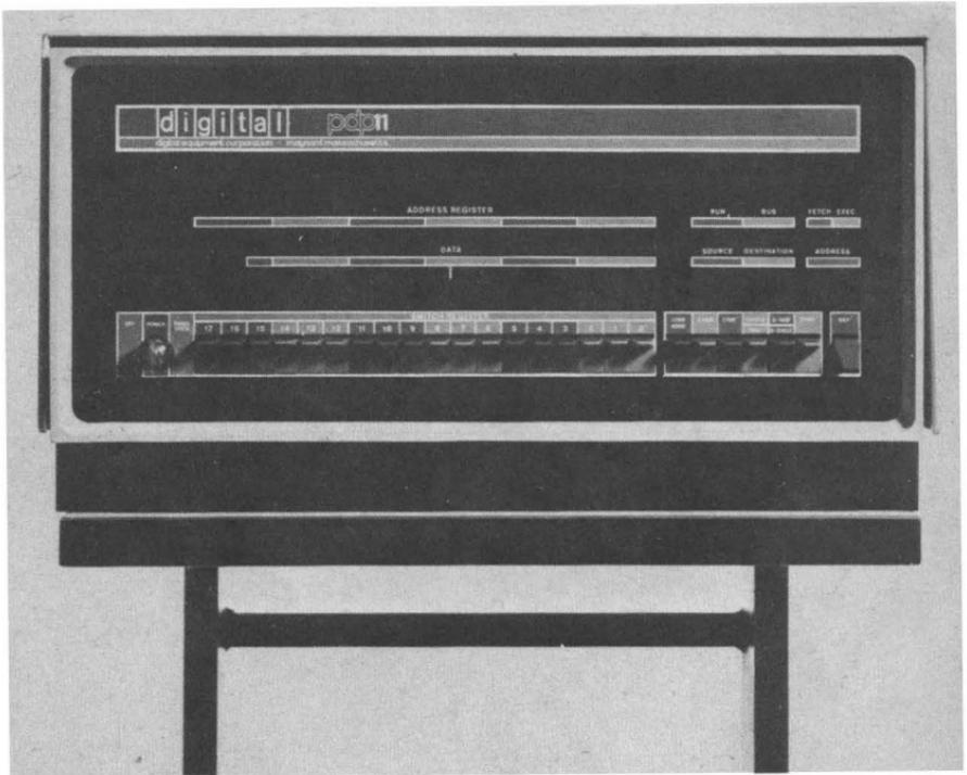
The PDP-11 is available in two versions—PDP-11/10 and PDP-11/20. The basic PDP-11/10 contains 1,024 words of read only memory in conjunction with 128 words of read/write memory and the basic PDP-11/20 includes 4,096 words of read/write memory.
