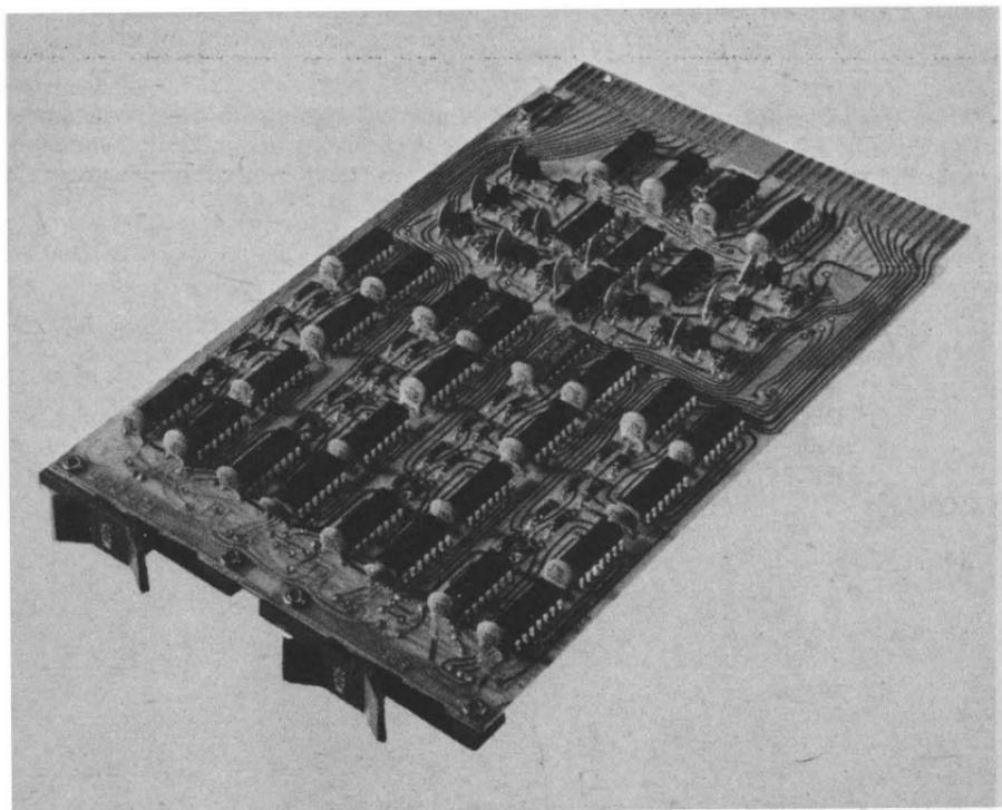
The DIGITAL M225 module contains multiple high speed general-purpose registers. The M225 general registers provide program flexibility when used as accumulators, index registers, and pointers to data words.
