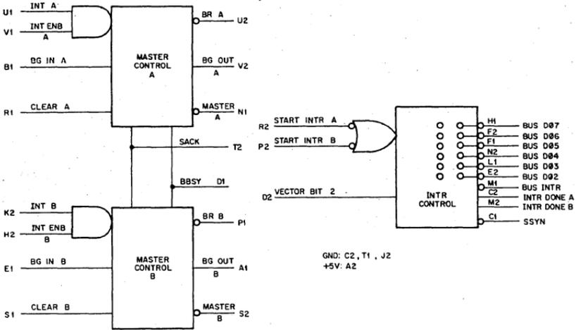
Figure 9.8 M782 Interrupt Control
