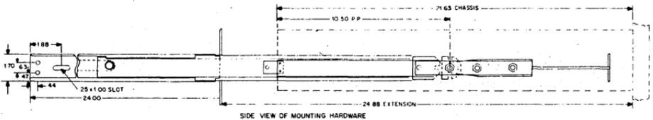
Figure 10.5 Side View of Mounting Hardware
