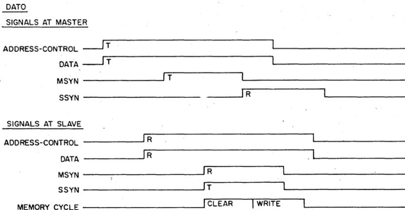
Figure D-2 DATO Operation
