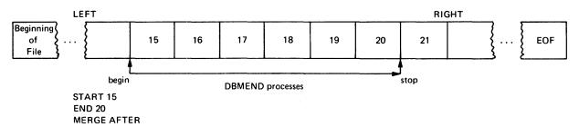
Figure 6-2 DBMEND Boundaries on Forward Processing
