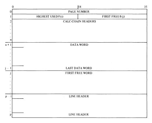
Figure D-1 Format of a Page Header
