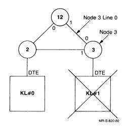
Figure 5-3: Dual-Processor Nodes
