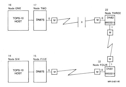
Figure 5-2: Loading an M9301-Equipped Remote Node
