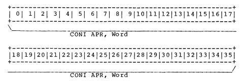
The CMAPRW word is the storage area provided for reading the Arithmetic Processor flags. The CONI APR, instruction puts the status of the error and sweep flags here. (For more information on the Arithmetic Processor, refer to the DECsystem-10/DECSYSTEM-20 Processor Reference Manual.)
