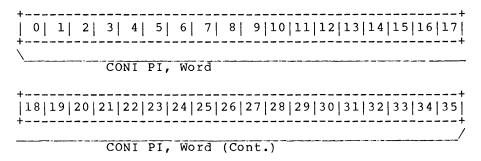
The CMPIWD word is the storage area provided for reading the Priority Interrupt system conditions. The CONI PI, instruction will place the PI status information here. (For more information on the Priority Interrupt system refer to the DECsystem-10/DECSYSTEM-20 Processor Reference Manual.)
