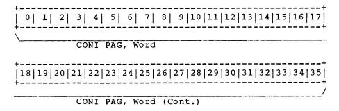
The CMPGWD word is the storage area provided for reading the system status of the Pager. The CONI PAG, instruction puts the status information here. (For more information on the Pager refer to the DECsystem-10/DECSYSTEM-20 Processor Reference Manual.)
