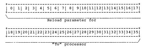
This word contains a copy of the "To" processor's reload word. The copy is saved by the owning processor in case the "To" processor crashes.
