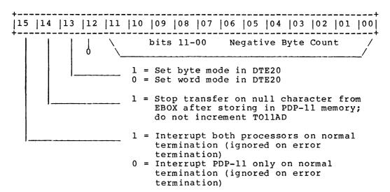
TO11BC When the PDP-11 loads this register (the TO-11 byte count) with the number of bytes to be transferred, the DTE20 begins the TO-11 transfer operation.
