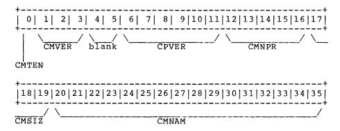
The PIDENT word provides information about the owning processor and its area. The separate fields in PIDENT are described below.
