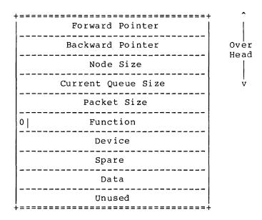
The first four words of the packet are not transfered to the KL. They contain information necessary to manage the queue in PDP-11 memory. The packet that is actually transfered across the DTE20 during a direct transfer is always at least 12 (octal) bytes and consists of words beginning with Packet Size and ending with the Data word.
