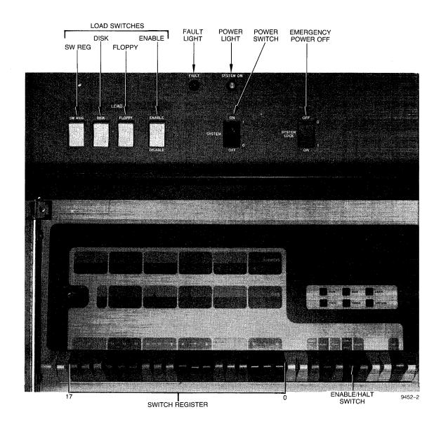
Figure 5-1: Load Switches and Switch Register for KL with Floppy Disks
