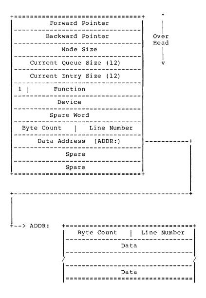
An indirect transfer takes place in two parts; first the header portion and then the data. Not all of the header shown above is transfered across the DTE20. The Header transfer always consists of 12 (octal) byte starting with the function word and ending with the data address word.
