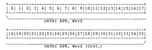
The CMDAPR word is the storage area provided for reading the current break conditions from the Arithmetic Processor. The DATAI APR, instruction puts the information here. (For more information on break conditions and the Arithmetic Processor, refer to the DECsystem-10/DECSYSTEM-20 Processor Reference Manual.)
