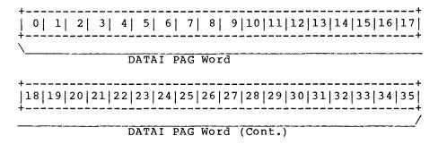
The CMPDWD word is the storage area provided for reading the process status of the Pager. The DATAI PAG, instruction puts the status information here. (For more information on the Pager refer to the DECsystem-10/DECSYSTEM-20 Processor Reference Manual.)
