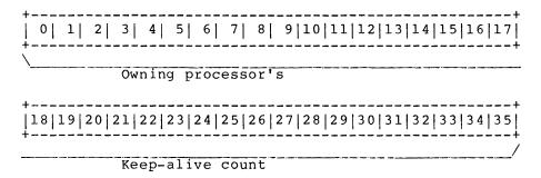
The CMKAC word contains the owning processor's Keep-Alive count. This word is incremented periodically, and is also checked periodically to make sure that it has changed. The Keep-Alive count should be incremented at least once a second by the owning processor, and the monitoring processor should allow the count to remain unchanged for at least six seconds before declaring the owning processor to be dead.
