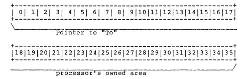
The CMPPT word contains a pointer to the area in the Communications Region that is owned by the "To" processor.
