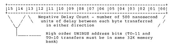
DLYCNT Since the DTE20 is clocked from the EBUS clock module, which runs at a different rate from the PDP-11 clock, a compromise in timing must be effected in order to transfer data over the DTE20. Therefore, the PDP-11 sets this register to notify the DTE20 of the speed at which to carry out byte transfer operations. The register contains the number of 500 nanosecond units of delay that should come between two consecutive byte transfers.
