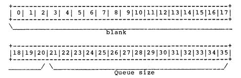
This word contains the number of eight-bit bytes written into the current packet by the transmitting processor. The packet can contain more than one message; this word does not contain a count of the number of messages, only of the number of bytes.
