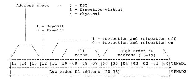
TENAD1-2 The PDP-11 uses these two registers in examine and deposit operations to specify the KL address. When the PDP-11 writes TENAD2 the deposit/examine operation is initiated; thus, all necessary data must be written to DEXWD1-3 before TENAD2 is written.
