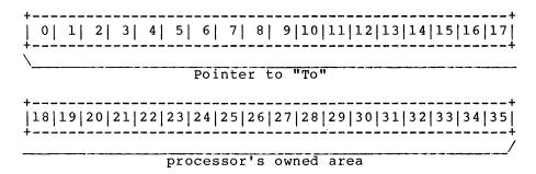
This word contains the owning processor's copy of the "To" processor's Keep-Alive count for purposes of comparison with the continuously updated copy kept by the "To" processor.
