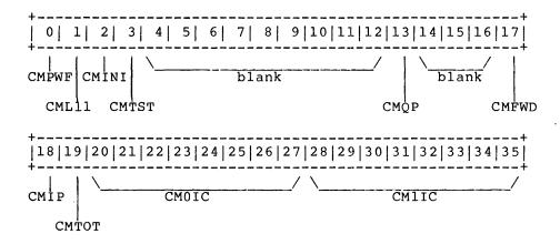
The STATUS word is intended to be the only word a processor has to examine when it receives a doorbell interrupt. The STATUS word contains the following status bits and counters:
