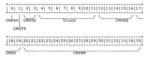
The TOPID word is the first location in each "To" processor area. This word contains information on the connections between the owning processor and the "To" processor.
