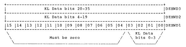
DEXWD1-3 During a deposit or examine operation, the data being deposited or examined appear in these three registers. However, DEXWD1 must always contain zeros in the high-order bits.
