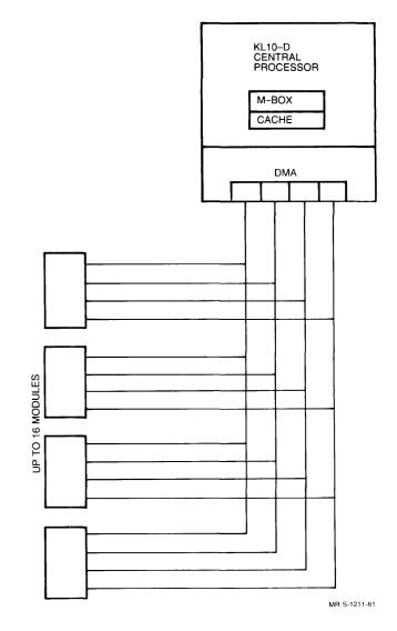
Figure 5–16 KL10–D Memory Bus Structure
