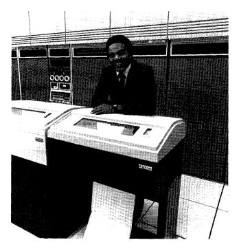
Up to 132 characters can be stored in a print line buffer and, upon command from the data source, the LP05 prints the contents of the buffer and advances the forms as specified by the command. It signals the data source when it is ready for the next line of print data or forms motion command.
