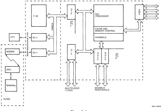
Figure 5–1 KL10–D Central Processing Unit
