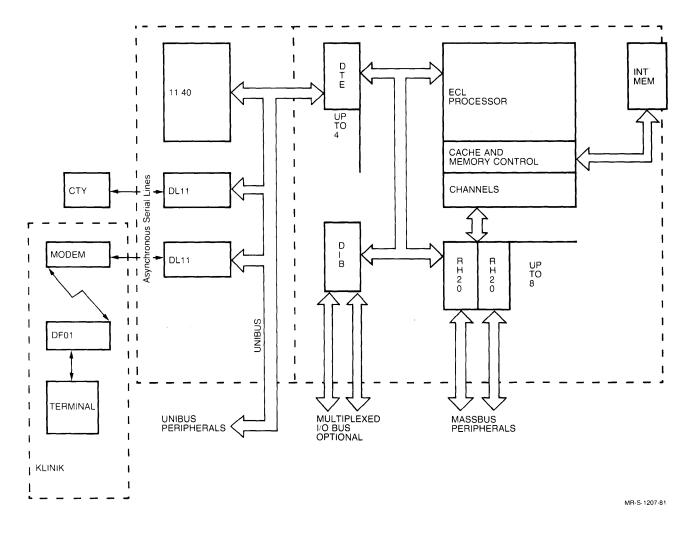
Figure 5–2 KL10–E Central Processor Unit
