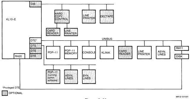
Figure 5–20 KL10–E Unibus and I/O Bus Peripheral Devices
