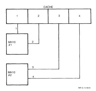
Figure 5–7 MH10 Memory Interleaving Concept
