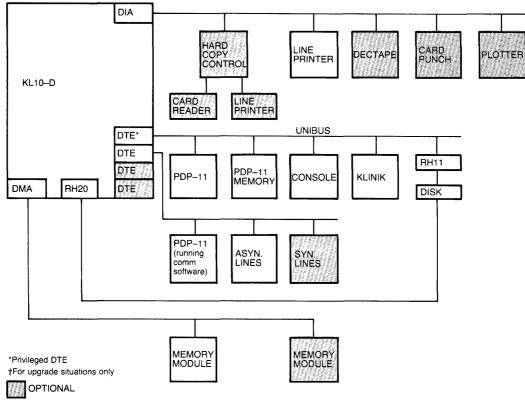
Figure 5–19 KL10–D Unibus and I/O Bus Peripheral Devices
