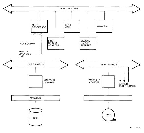
Figure 6–1 KS10 System Architecture
