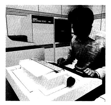
The local operator controls the KS10 with a set of commands typed at the console terminal (CTY). The CTY connects directly to the microprocessor-based console hardware over a serial line interface (USART). A second serial line operating in parallel with the first can also be connected to the console hardware, allowing the KS10 to be controlled by a remote diagnosis link.
