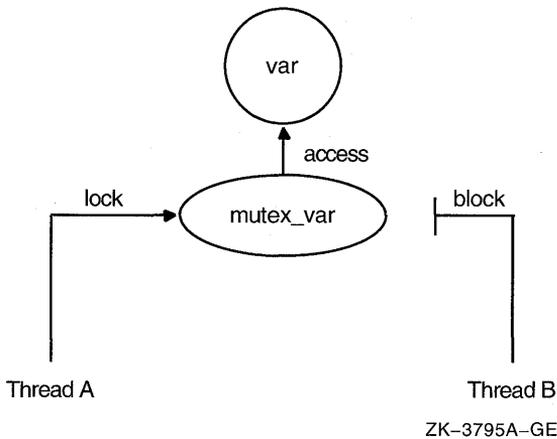
Each mutex must be created. (To create mutexes as part of your program's one-time initialization code, see Section 2.5.) To create a mutex, use the `cma_mutex_create` or `pthread_mutex_init` routine. These routines allow you to specify an attributes object, which allows you to specify the mutex type. The types of mutexes are described in the following sections.
