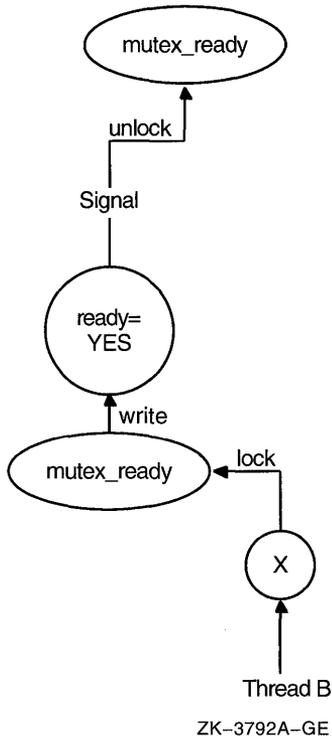
Thread B releases its lock on the shared variable's mutex. As a result of the signal, Thread A wakes up, implicitly regaining its lock on the condition variable's mutex. It then verifies that the predicate is in the correct state, and proceeds to execute Task Y (see Figure 2-4).
