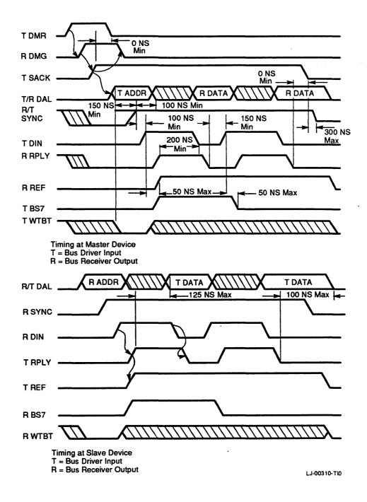
Figure A-9 DATBI Bus Cycle Timing
