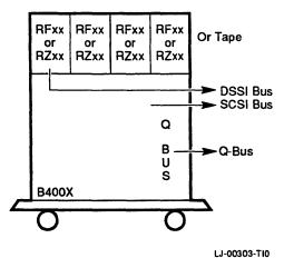
Figure 5–3 BA400x Q-Bus and Disk Expansion Enclosure
