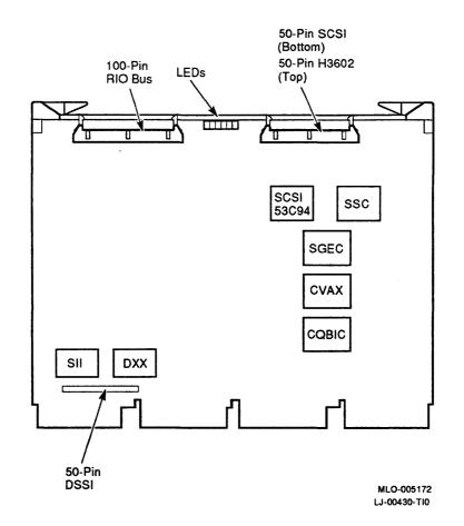
Figure 1–5 KN220-AA I/O Module Layout
