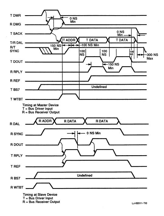
Figure A–10 DATBO Bus Cycle Timing
