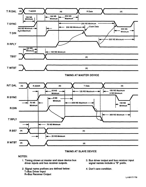
Figure A-2 DATI Bus Cycle Timing
