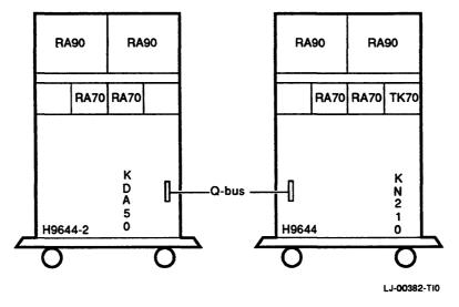
Figure 5–9 DU-55xxx RA Base System with H9644 Expansion Cabinet
