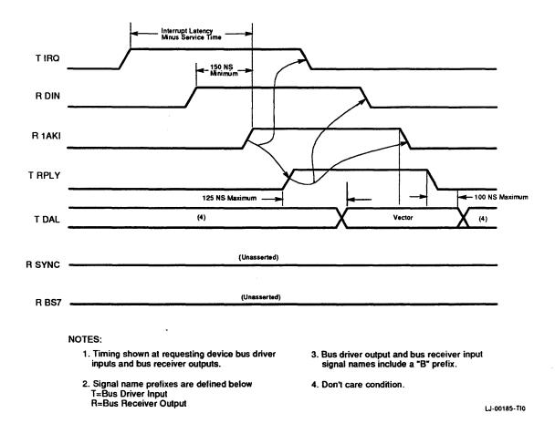
Signal timing must be considered carefully when implementing four-level interrupts (Figure A-12).
