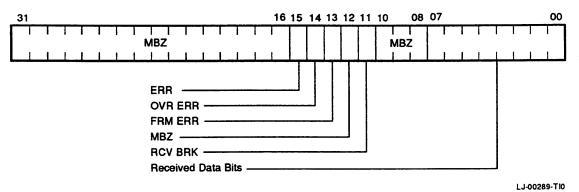
Figure 3–32 Console Receiver Data Buffer
