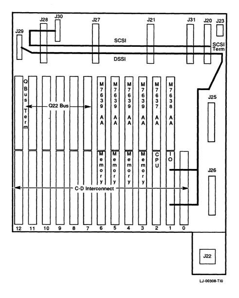
Figure 5–13 BA430 Enclosure Backplane Layout
