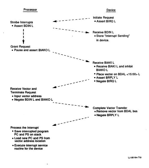
Figure A–11 Interrupt Request/Acknowledge Sequence
