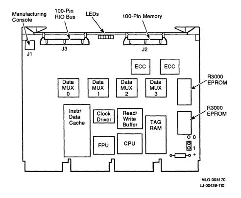
Figure 1–4 KN220-AA CPU Module Layout
