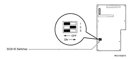
Table 3-5 shows the setting of the SCSI ID switches on the RX23 FDI board for the valid SCSI ID addresses.
