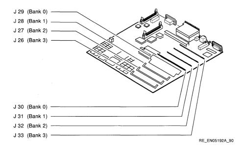
6 Insert the first MS44 memory module, with the side containing the bar code label facing up, into the connector on the system module. Gently press down on the module, until the tabs on the connector snap, locking the module into position.
