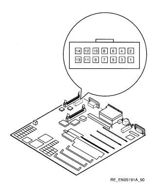
Table 2-3 **System Module Power Connector Voltages**
