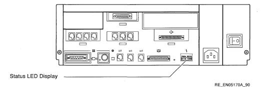
During the power-up self-test, or when running extended self-test diagnostics (see Chapter 2), LEDs 7, 6, 5, 4, and 2 on the status LED display show a binary code. If the system detects an error, it halts and displays a code indicating the number of the test that failed.
