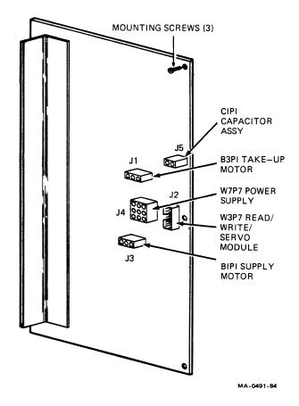
Figure 10 Power Amplifier Module
