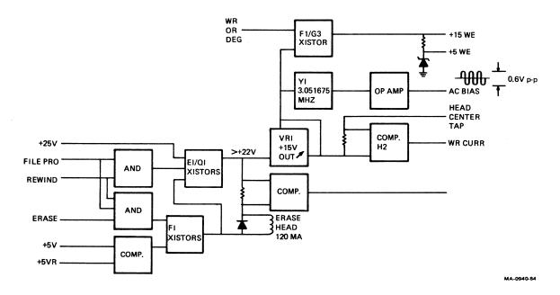
Figure 19 Write Driver Block Diagram
