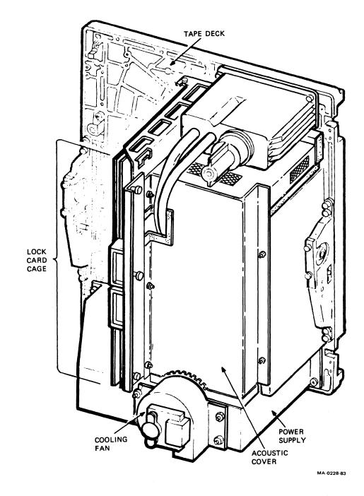
Figure 16 TU8Ø Transport Components (Bottom)
