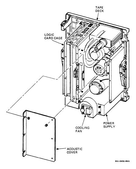
Figure 8 Transport Components (Bottom)
