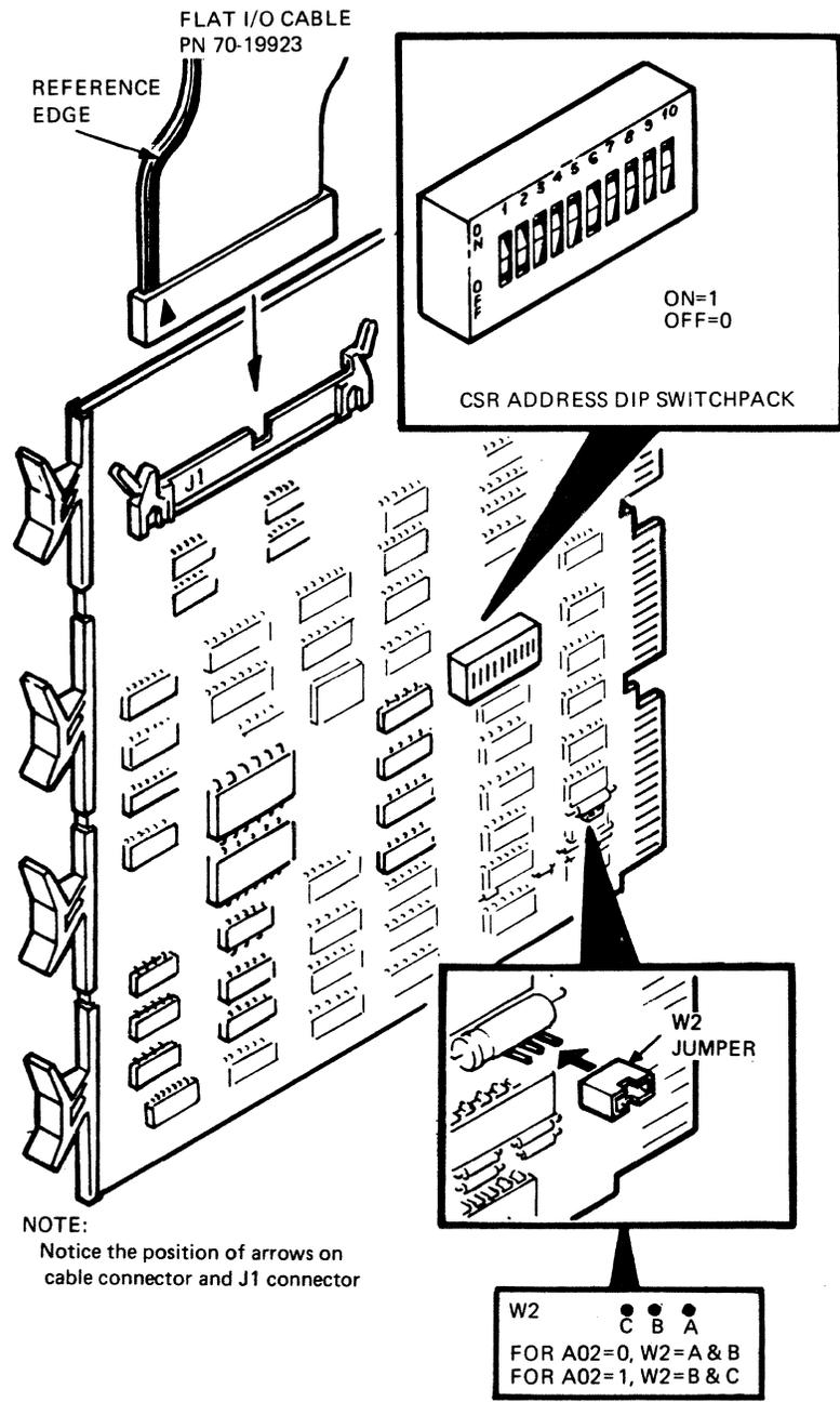
Figure 13 LESI UNIBUS Adapter Module
