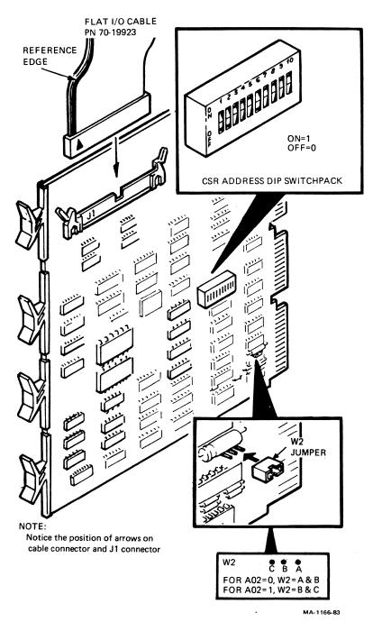
Figure 13 LESI UNIBUS Adapter Module
