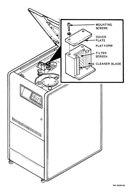
Figure 2 Tape Cleaner Removal
