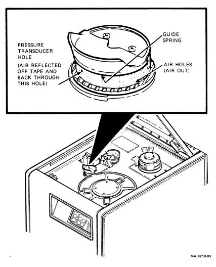
Figure 5 Air Bearing
