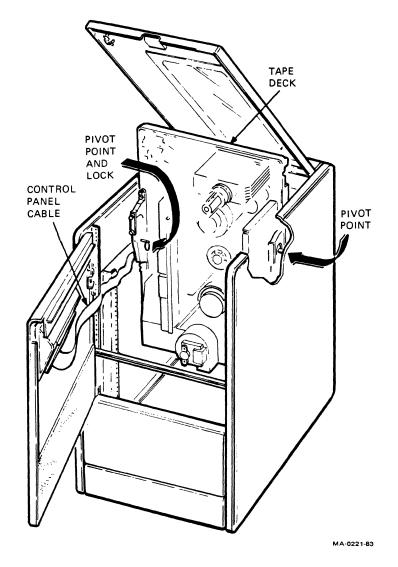
Figure 7 Rotating the Tape Deck
