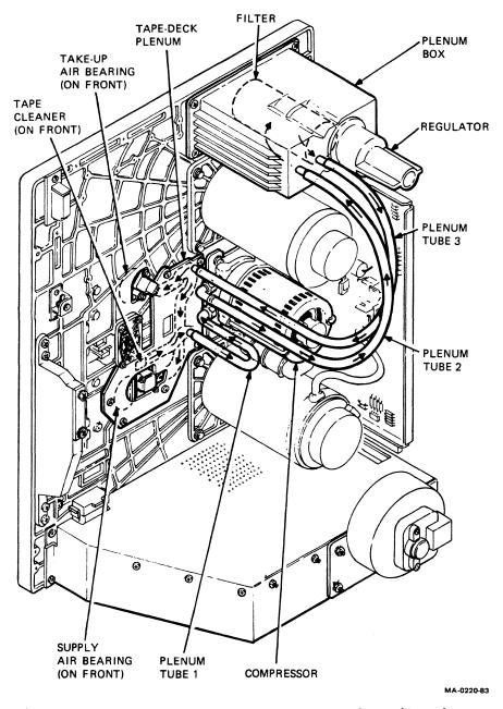
Figure 21 Vacuum and Pressure Distribution
