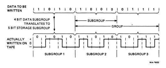
Figure 5 GCR Representation of Data Written on Tape
