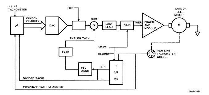
Figure 16 Velocity Servo
