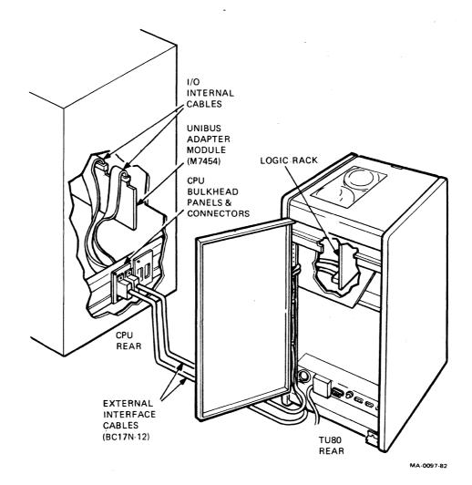
Figure 20 TU80 Interface Cabling
