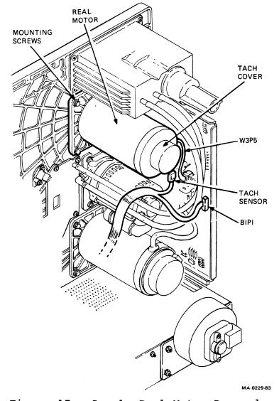
Figure 17 Supply Reel Motor Removal
