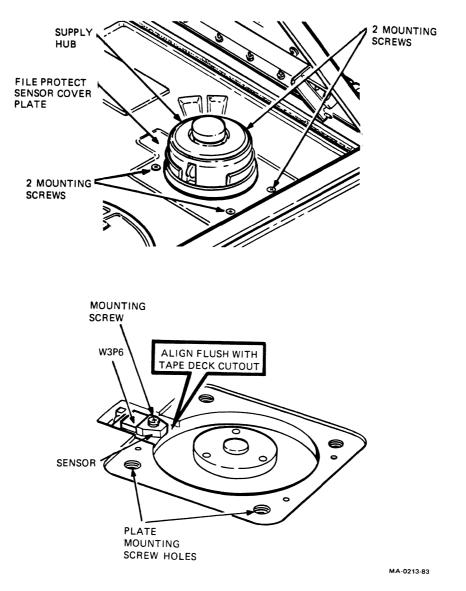
Figure 3 File Protect Sensor Removal
