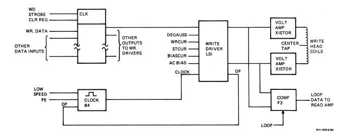
Figure 18 Write Control Block Diagram
