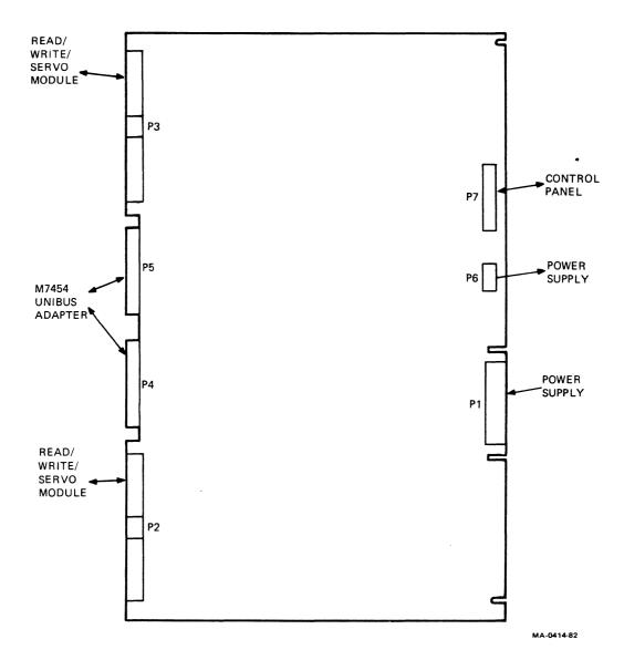
Figure 18 Formatter/Control Module
