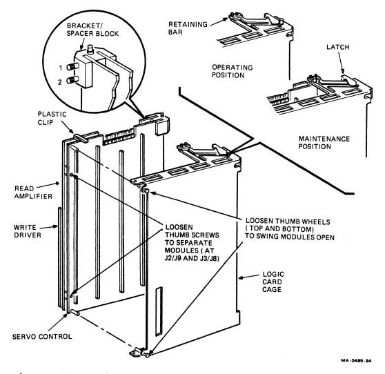
Figure 6 Write Driver/Read Amplifier/Servo Control Modules
