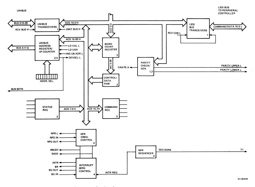
Figure 10 M8739 LESI Adapter Block Diagram
