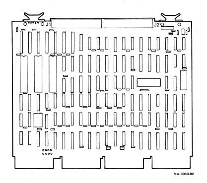
Figure 19 M7454, UNIBUS Adapter Module
