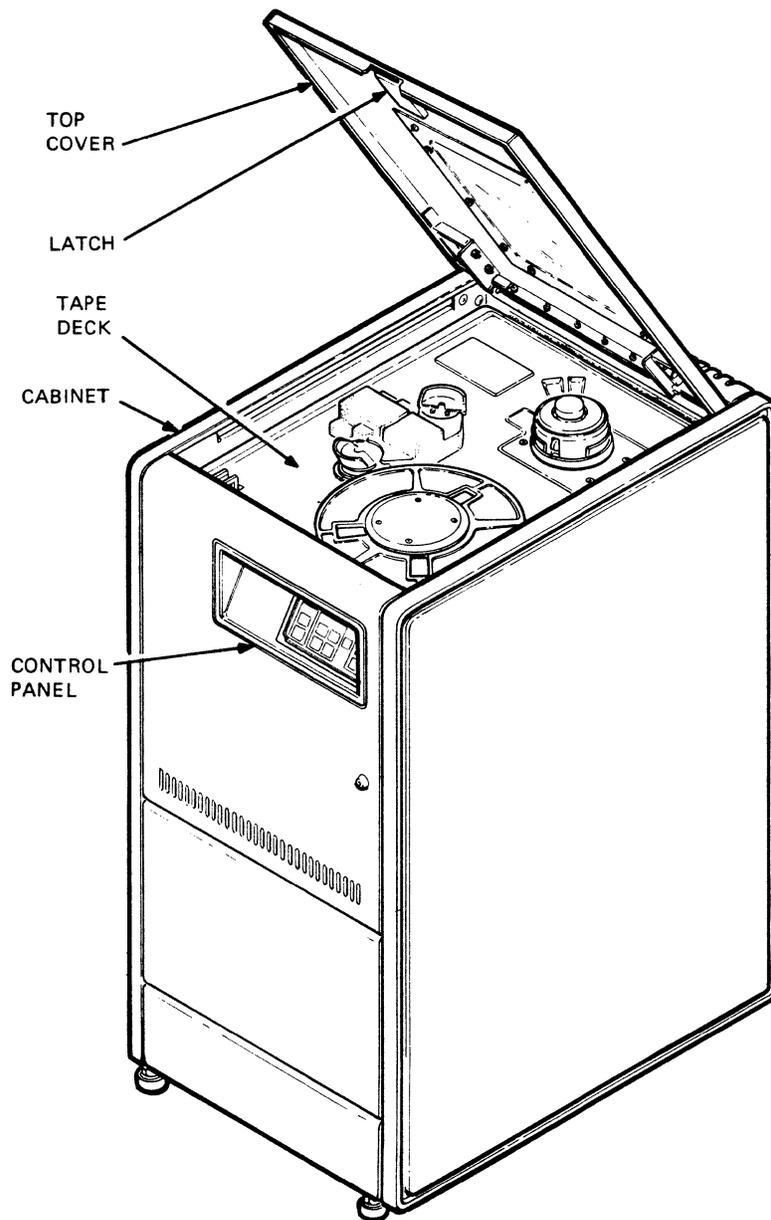
TAPE DECK COMPONENTS & CONTROL PANEL = TRANSPORT
