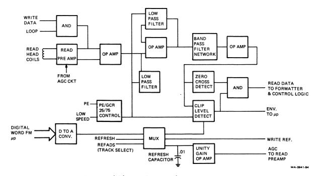
Figure 20 Read Amplifier Block Diagram
