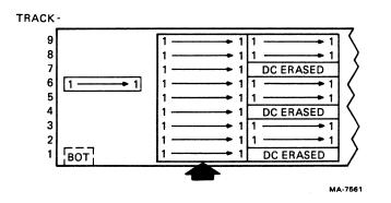
Figure 1 Group Coded Recording (GCR Tape)
