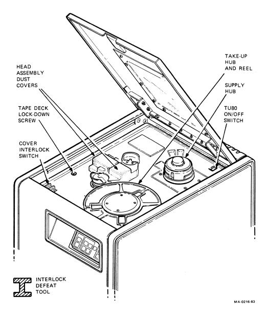
Figure 3 Transport Components (Top)
