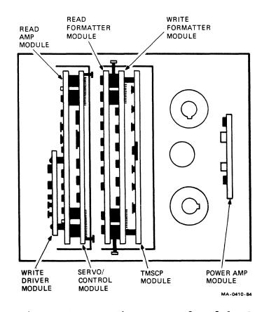
Figure 4 Logic Cage and Module Locations
