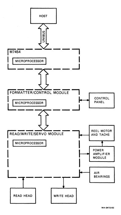
Figure 21 TU80 Basic Block Diagram
