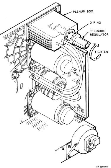
Figure 18 Pressure Regulator Removal
