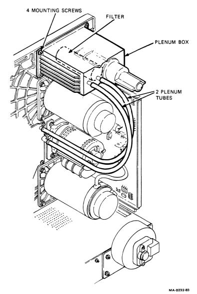
Figure 19 Plenum Box and Air Filter Removal
