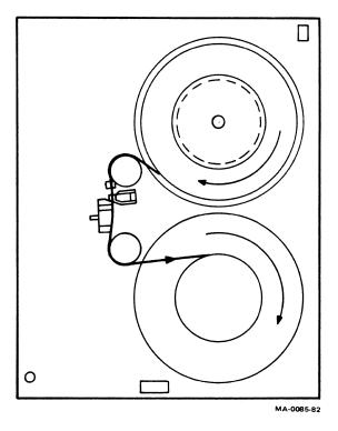
Figure 6 Threading Tape
