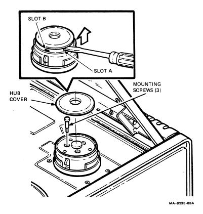
Figure 16 Supply Hub Assembly Removal
