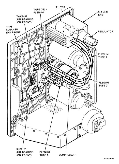
Figure 11 Vacuum/Pressure Air System
