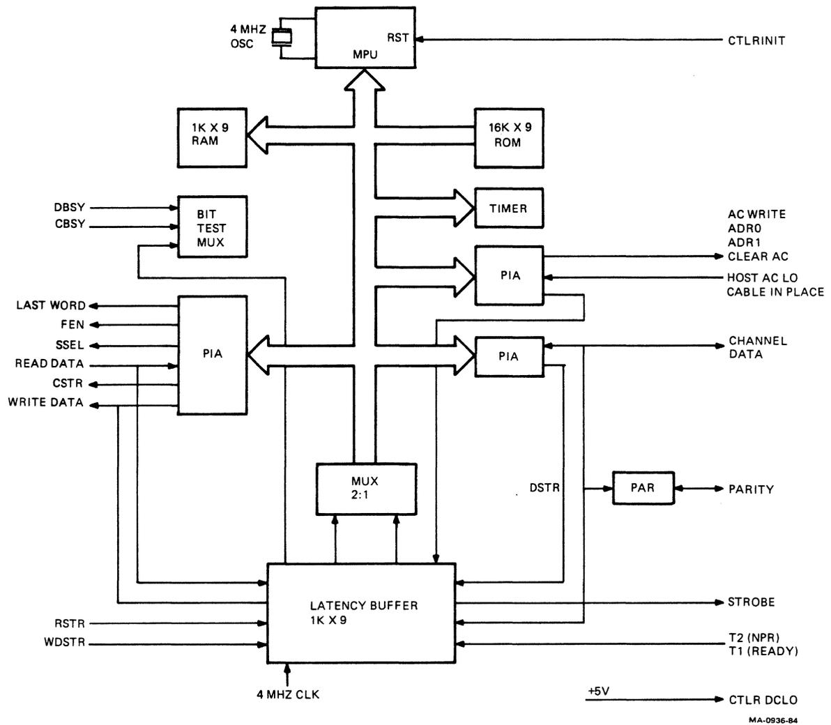
Figure 12 TMSCP Controller Block Diagram
