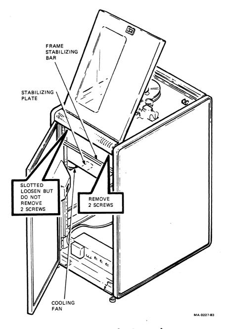
Figure 21 Power Supply Removal
