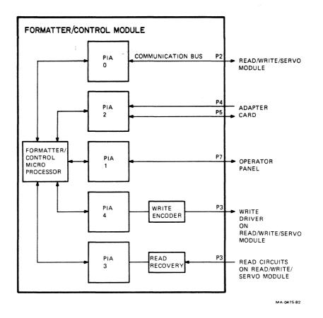
Figure 25 DIA Interfacing (Formatter/Control Module)
