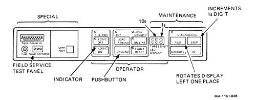
Figure 7 Control Panel With Field Service Tests Loaded
