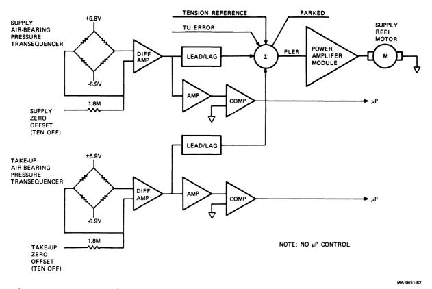
Figure 17 Tension Servo
