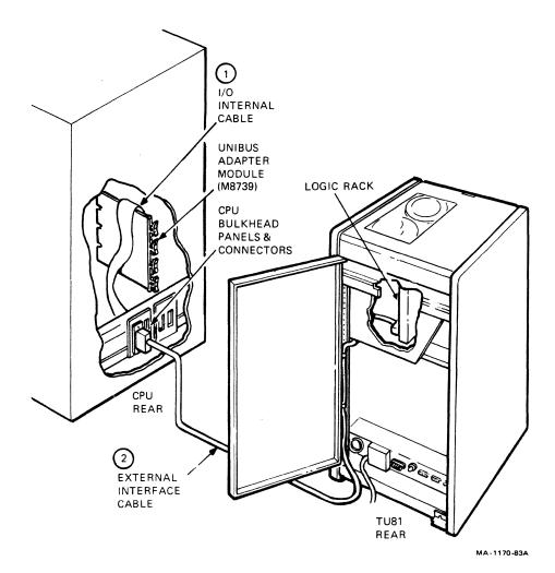
Figure 1 Interface Cabling
