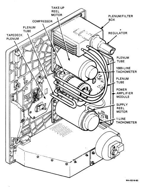
Figure 9 Transport Components (Cover Removed)
