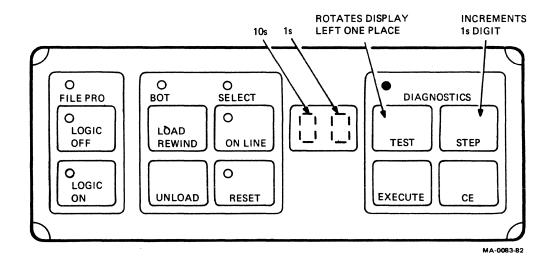
Figure 7 TU8Ø Control Panel
