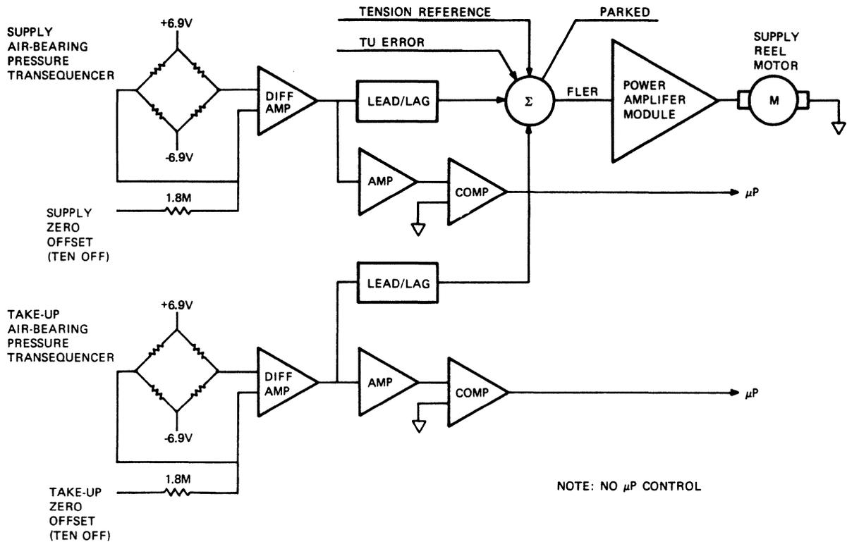
Figure 17 Tension Servo
