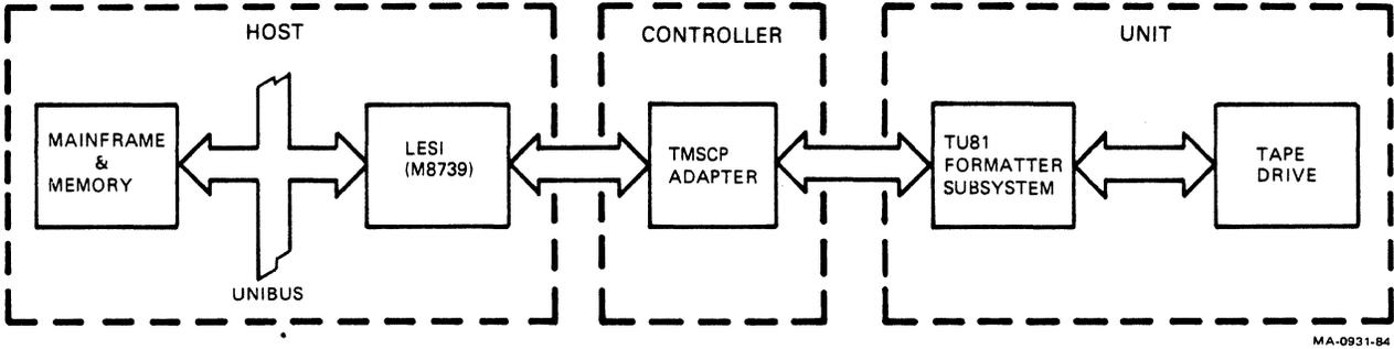
Figure 7 TU81 System Block Diagram
