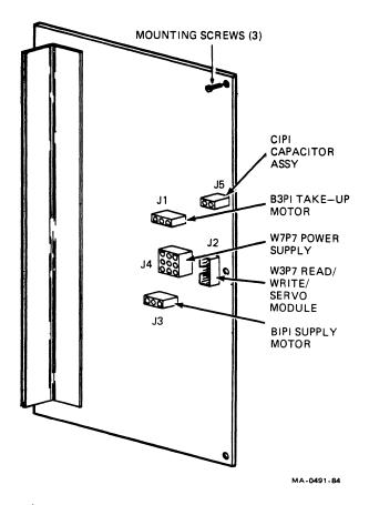
Figure 20 Power Amplifier Module
