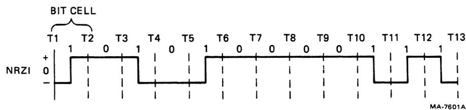
Figure 3 NRZI (Non-Return to Zero Inverted Recording)
