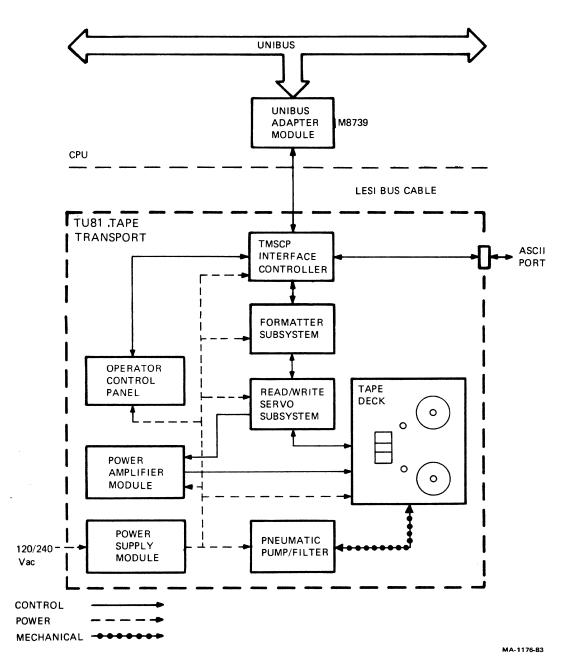
Figure 15 TU81 Basic Block Diagram
