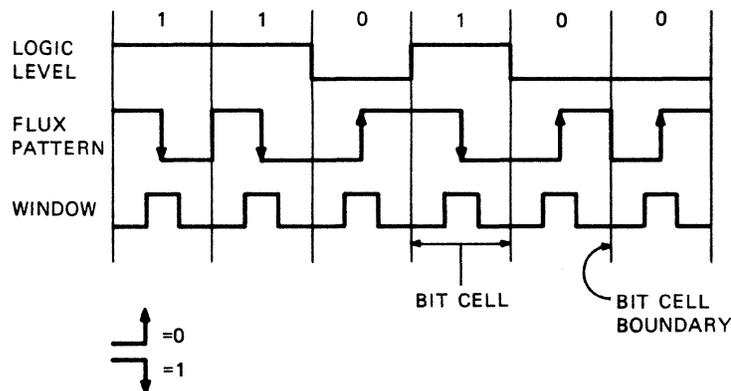
Figure 1 Phase Encoded (PE) Recording
