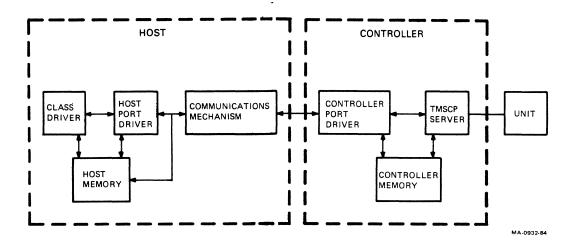
Figure 8 Software/Firmware Block Diagram
