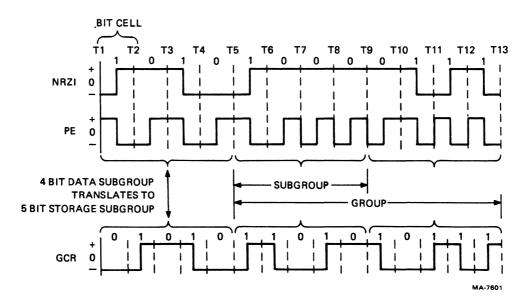
Figure 2 Tape Recording Formats
