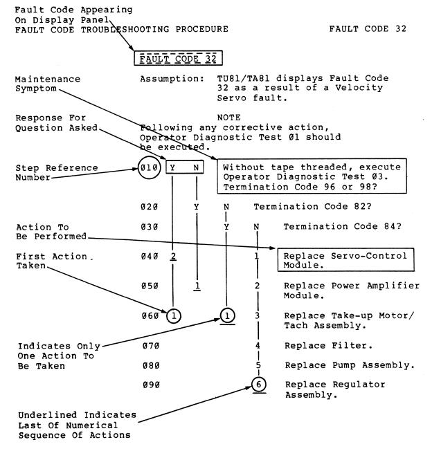
Figure 2 Pathfinder Fault Code Troubleshooting Procedure
