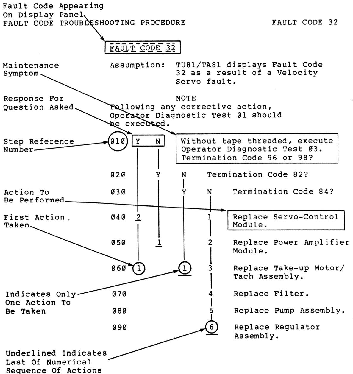
Figure 2 Pathfinder Fault Code Troubleshooting Procedure
