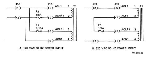
Figure 23 Voltage Select Module
