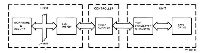
Figure 7 TU81 System Block Diagram
