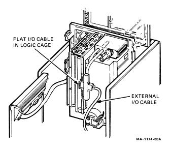
Figure 8 Internal I/O Cabling
