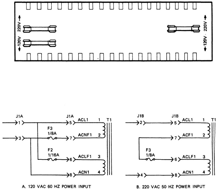
Figure 23 Voltage Select Module
