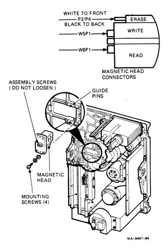
Figure 11 Magnetic Head Removal
