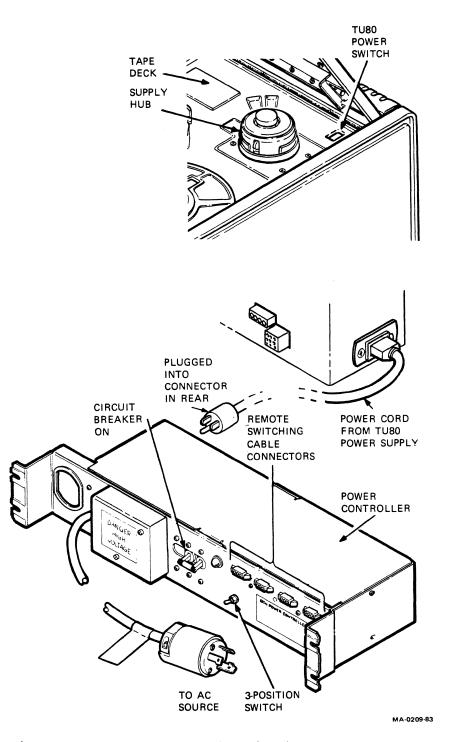
Figure 4 TU81 Power-Up Checks
