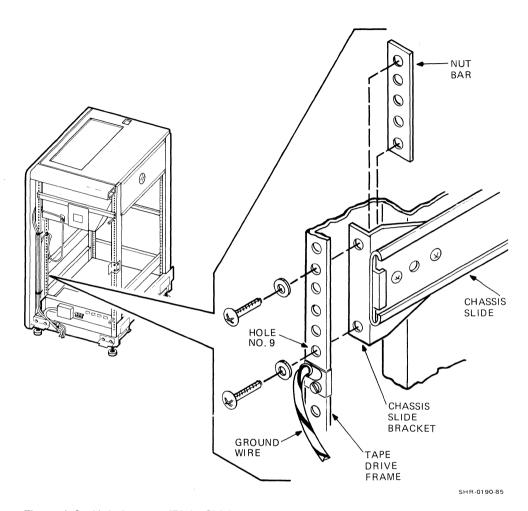
Figure A-9 Hole Locator (Right Side)
