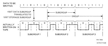
Figure 1-4 GCR Representation of Data Written On Tape
