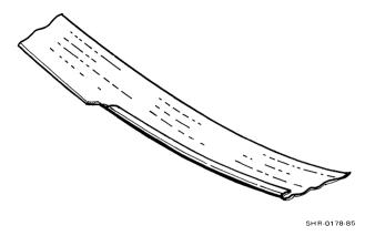
Figure 4-3 Tape End Damage
