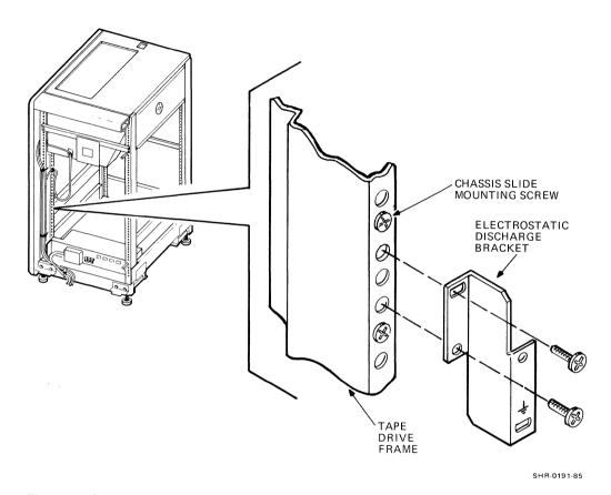
Figure A-10 Mounting the Left Electrostatic Discharge Bracket
