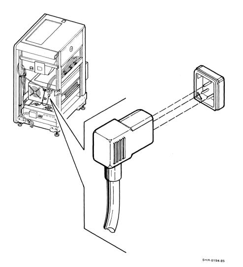
Figure A-14 Plugging in the Disk Drive Power Cord
