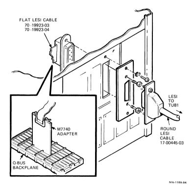
Figure 5-15 M7740 Module and TU81 Bulkhead Mounting
