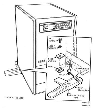
Figure 5-9 Rear Stabilizer Installation
