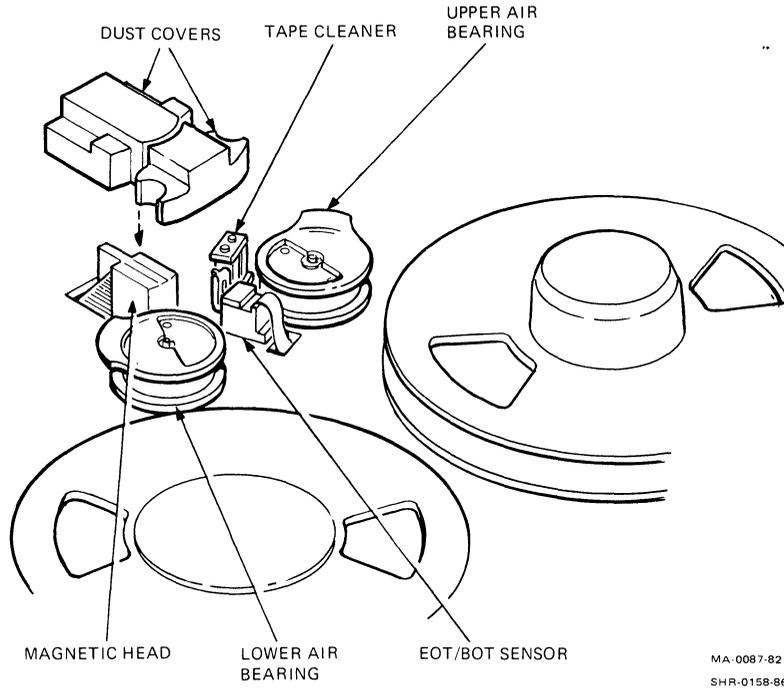
Figure 4-7 Magnetic Head/Tape Path Components
