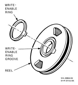
Figure 2-4 Write-Enable Ring
