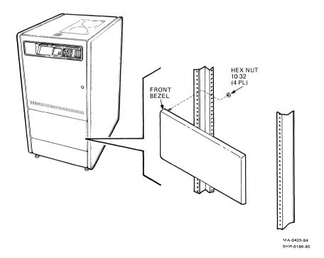
Figure A-6 Removing Front Bezel
