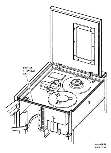
Figure 5-5 Removing the Front Shipping Bar
