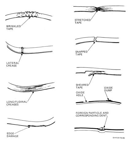
Figure 4-1 Tape Damage
