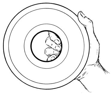
Figure 4-2 Correct Tape Handling
