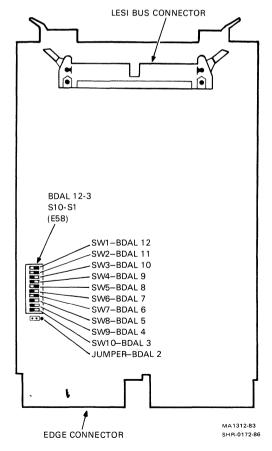
Figure 5-16 M7740 KLESI Q-Bus Adapter Module
