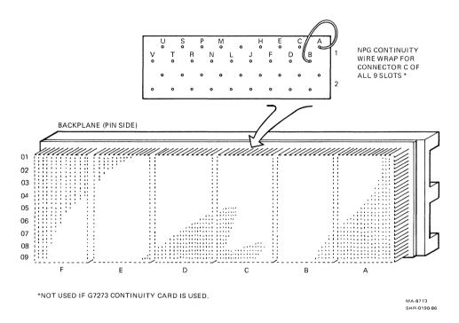
Figure 5-22 Unibus NPG Jumper
