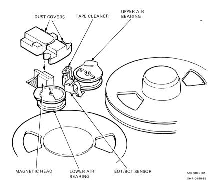
Figure 4-7 Magnetic Head/Tape Path Components
