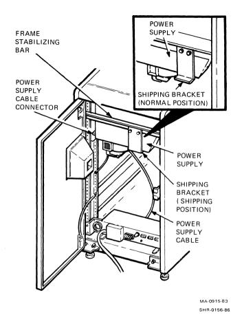
Figure 5-4 Rear Shipping Bracket
