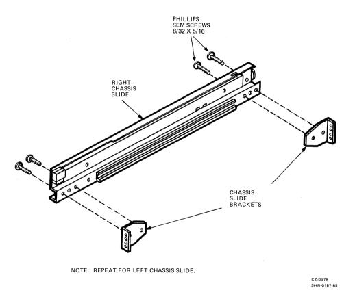
Figure A-7 Mounting the Chassis Slide Brackets to the Right-Side Chassis Slide
