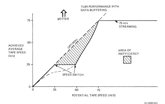
Figure 1-5 Adaptive Speed Control and Buffering
