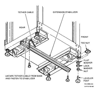
Figure 5-6 Cabinet Leveler Feet Assembly and Extension Stabilizer
