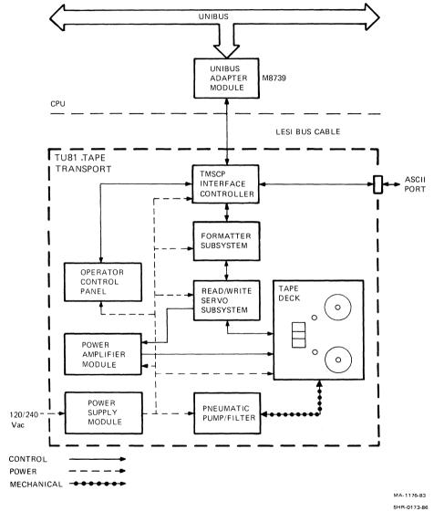
Figure 1-6 TU81 and TA81 Transport Functional Block Diagrams (Part A)
