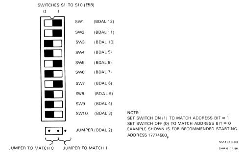
Figure 5-17 M7740 Module Jumpers and Switches
