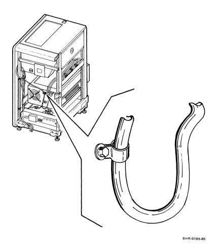
Figure A-15 Routing the Disk Drive Power Cord
