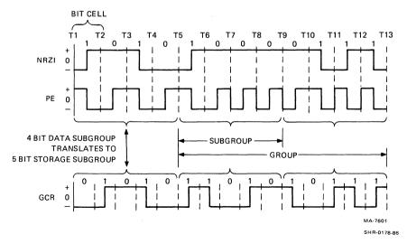
Figure 1-3 Tape Recording Formats
