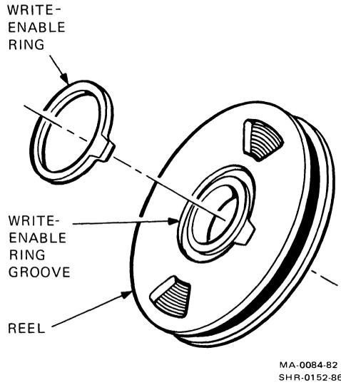
Figure 2-4 Write-Enable Ring
