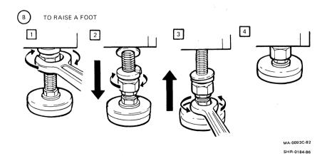
Figure 5-7 Leveler Feet Adjustments
