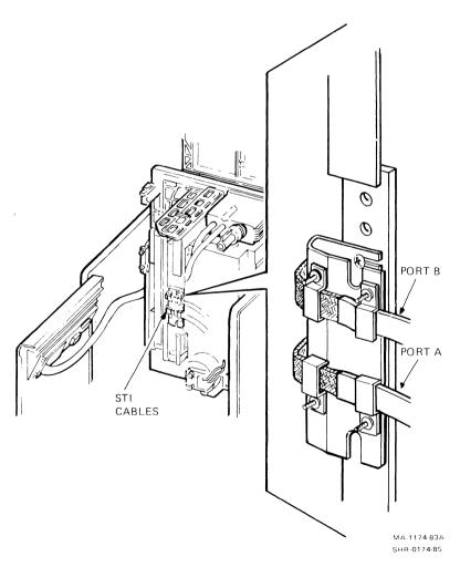
Figure 5-26 TA81 Tape Deck Access and Internal Cabling
