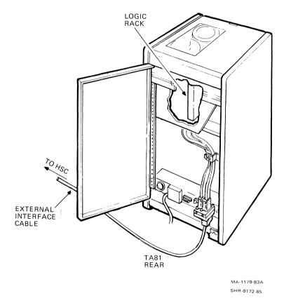
Figure 5-24 TA81 Interface Cabling
