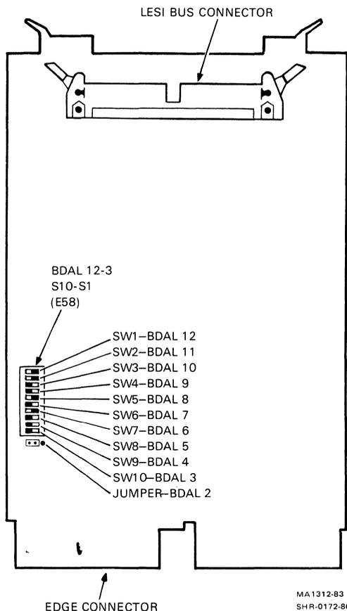
Figure 5-16 M7740 KLESI Q-Bus Adapter Module
