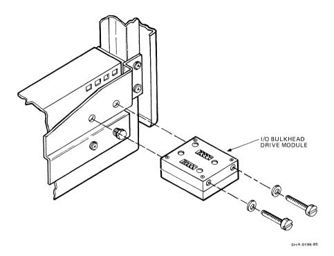
Figure A-16 Mounting the I/O Bulkhead Module
