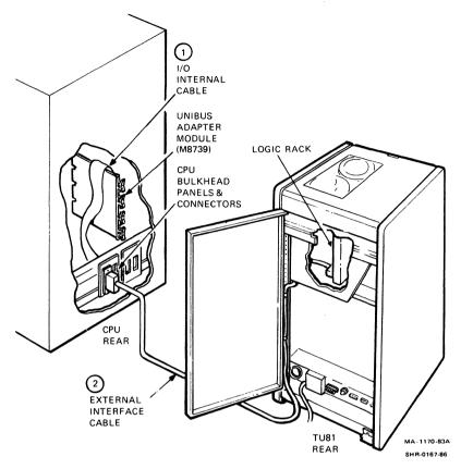
Figure 5-12 Interface Cabling
