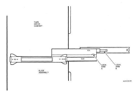
Figure A-11 Extended Locked Chassis Slides
