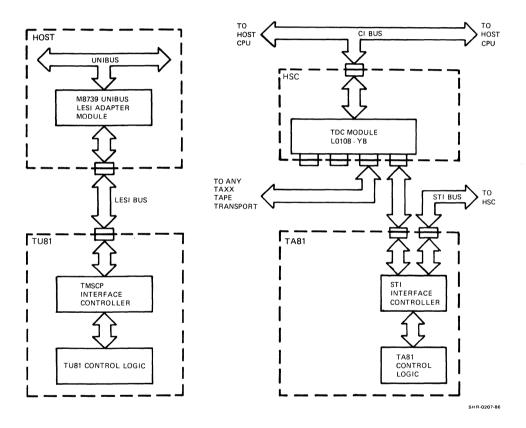
Figure 1-2 TU81 and TA81 Subsystem Block Diagrams
