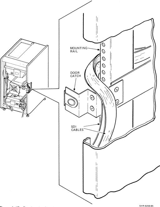
Figure A-17 Routing the SDI Cables
