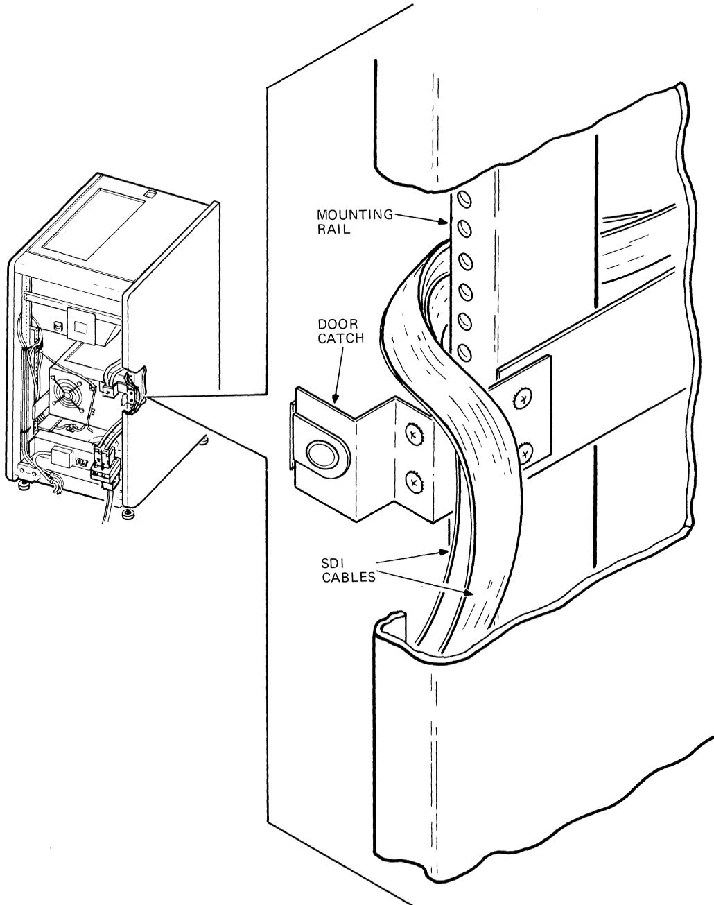
Figure A-17 Routing the SDI Cables
