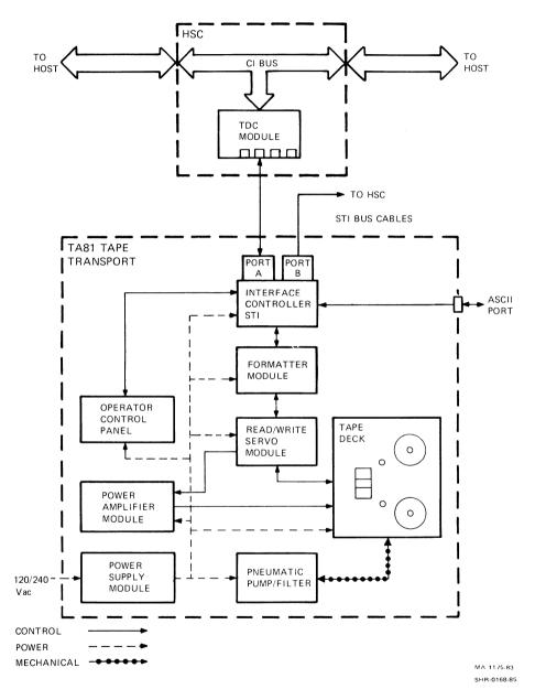
Figure 1-6 TU81 and TA81 Transport Functional Block Diagrams (Part B)
