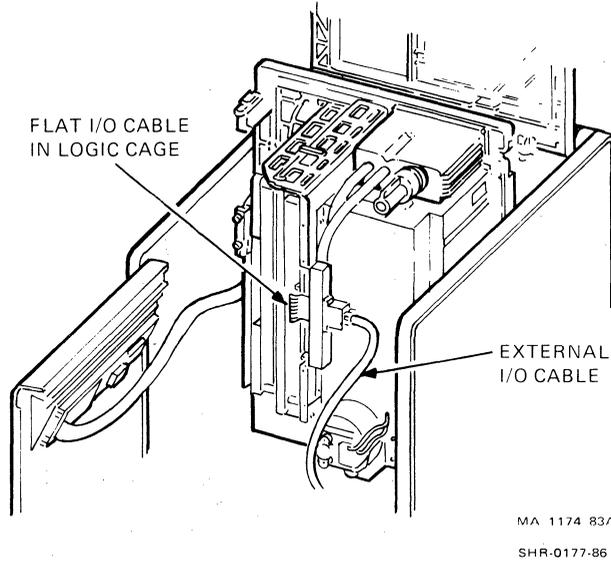
Figure 5-14 Tape Deck Access and Internal Cabling
