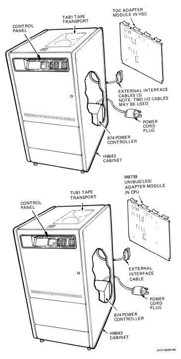
Figure 1-1 TU81 and TA81 Tape Subsystems
