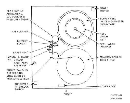
Figure 1-7 **Tape Deck Components**
