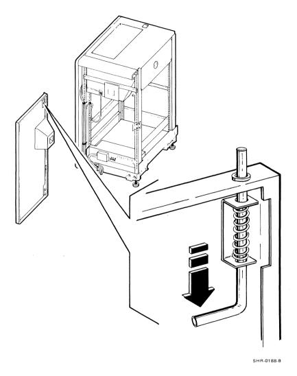
Figure A-5 Releasing Pivot Pin to Remove Rear Door
