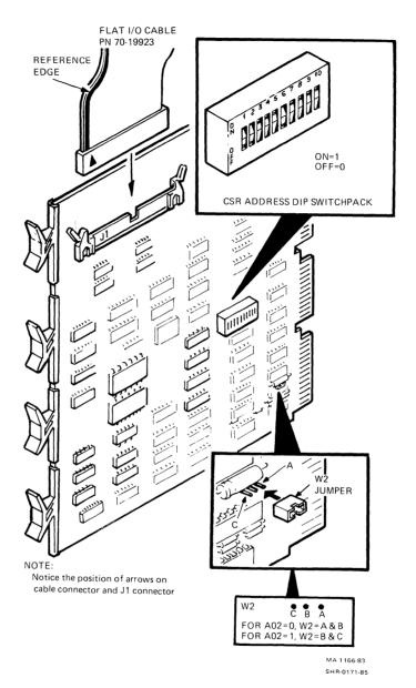
Figure 5-19 M8739 Module (Style B)
