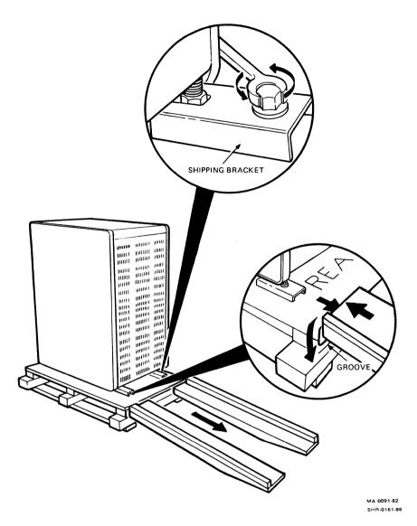
Figure 5-3 Transport Removal From Shipping Pallet With Ramps
