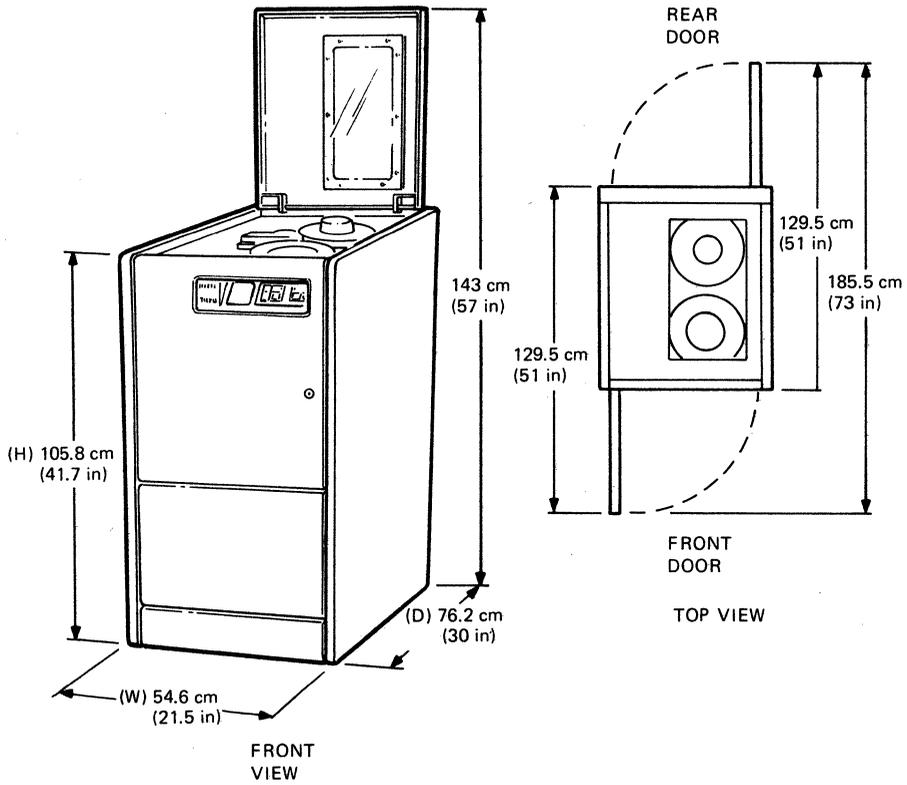
NOTE: WITH H9544-MJ FOOT INSTALLED, THE UNIT WIDTH IS 91.2 cm (34.25 in).
