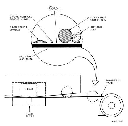
Figure 4-4 Relative Size of Tape Contaminants
