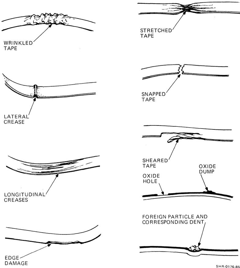
Figure 4-1 Tape Damage
