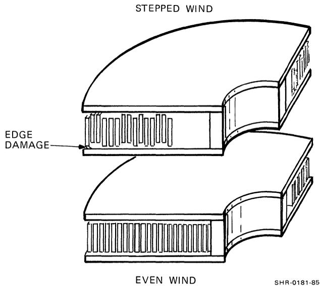
Figure 4-8 Uneven (Stepped) and Even Wind
