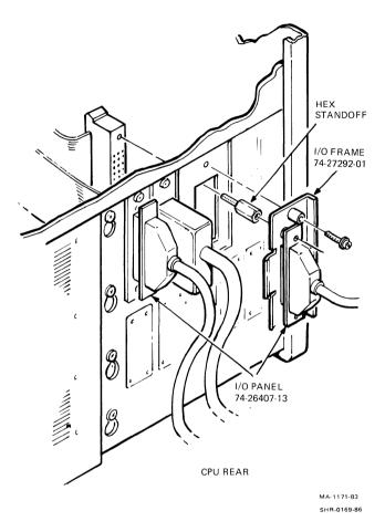
Figure 5-23 I/O Cable Installation on CPU Bulkhead
