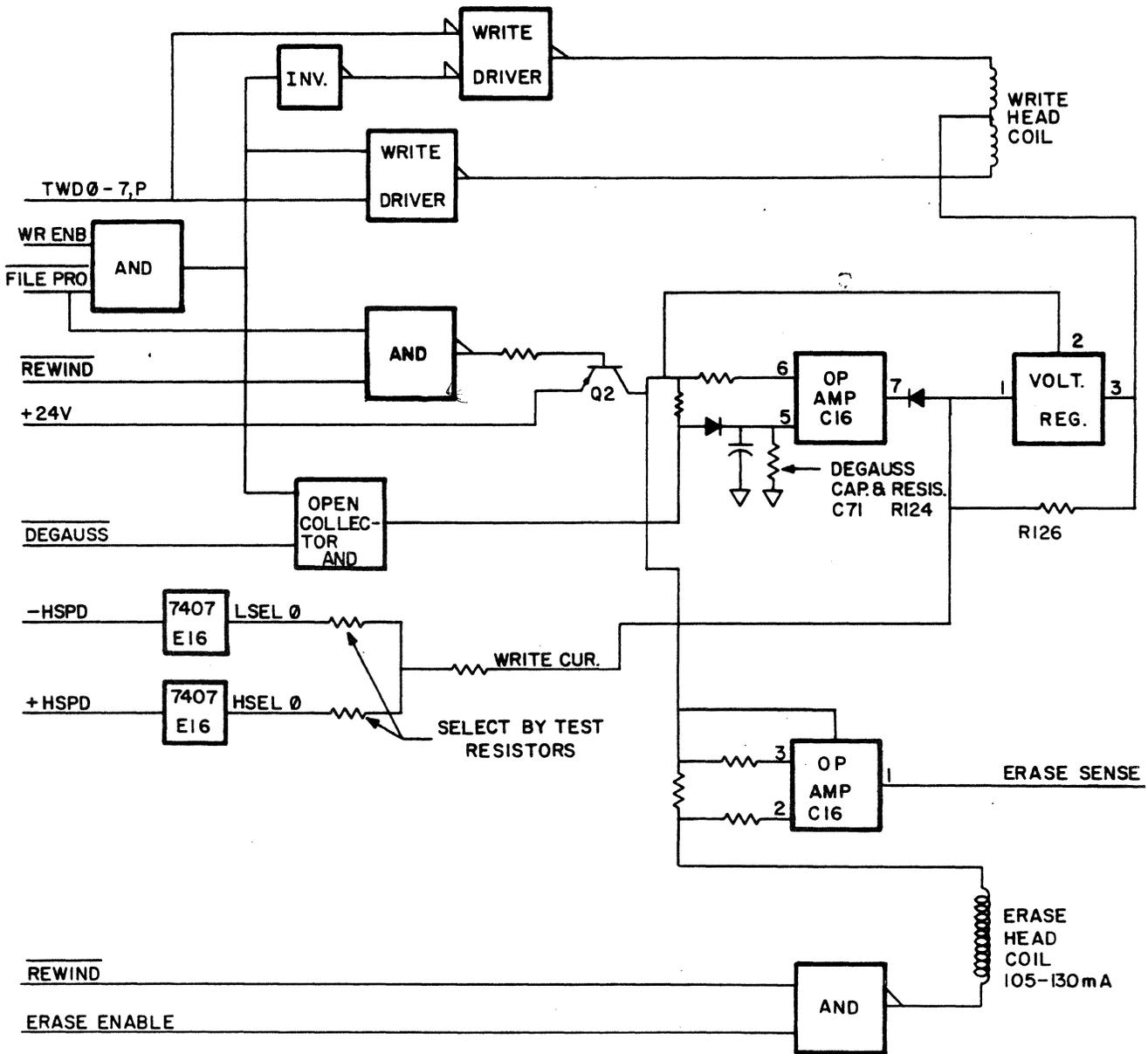
Figure 4-15. WRITE/ERASE BLOCK DIAGRAM
