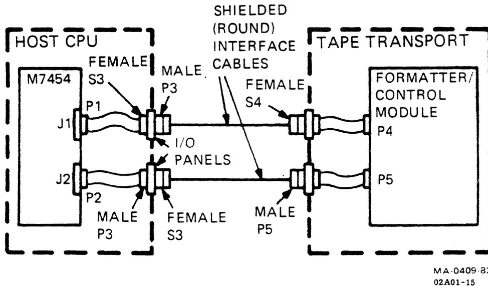
Figure 2-10. PLUG-TO-PLUG INTERFACE CABLE CONNECTIONS
