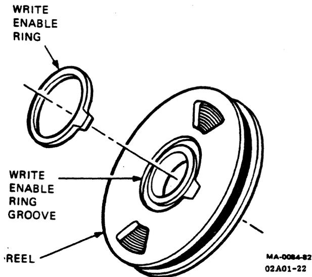
Figure 3-2. WRITE ENABLE RING
