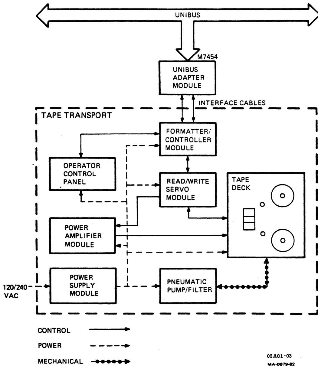
Figure 1-2. TU80 TAPE SUBSYSTEM BLOCK DIAGRAM
