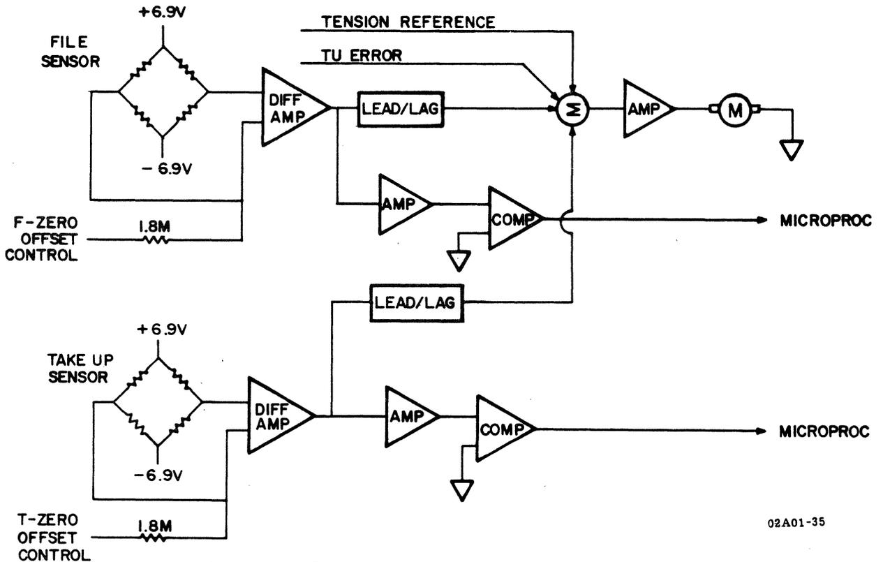
Figure 4-13. TENSION SERVO - SIMPLIFIED
