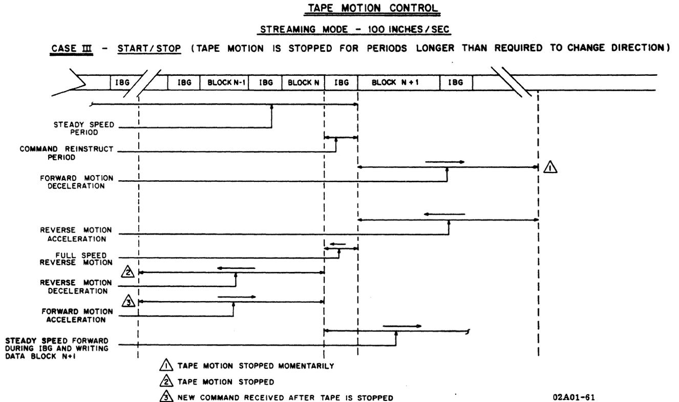
Figure 4-39. TAPE MOTION CONTROL - CASE 3 (Cont'd)
