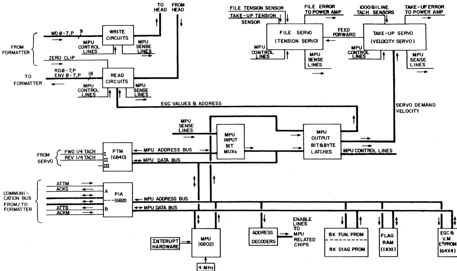
Figure 4-12. READ/WRITE/SERVO MODULE BLOCK DIAGRAM
