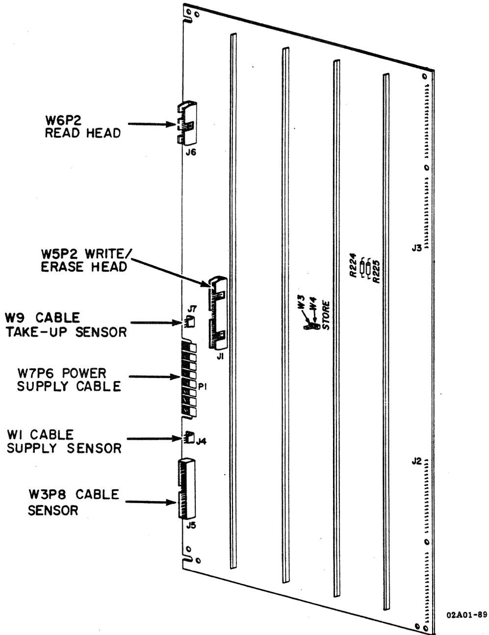
Figure 5-23. READ/WRITE/SERVO MODULE
