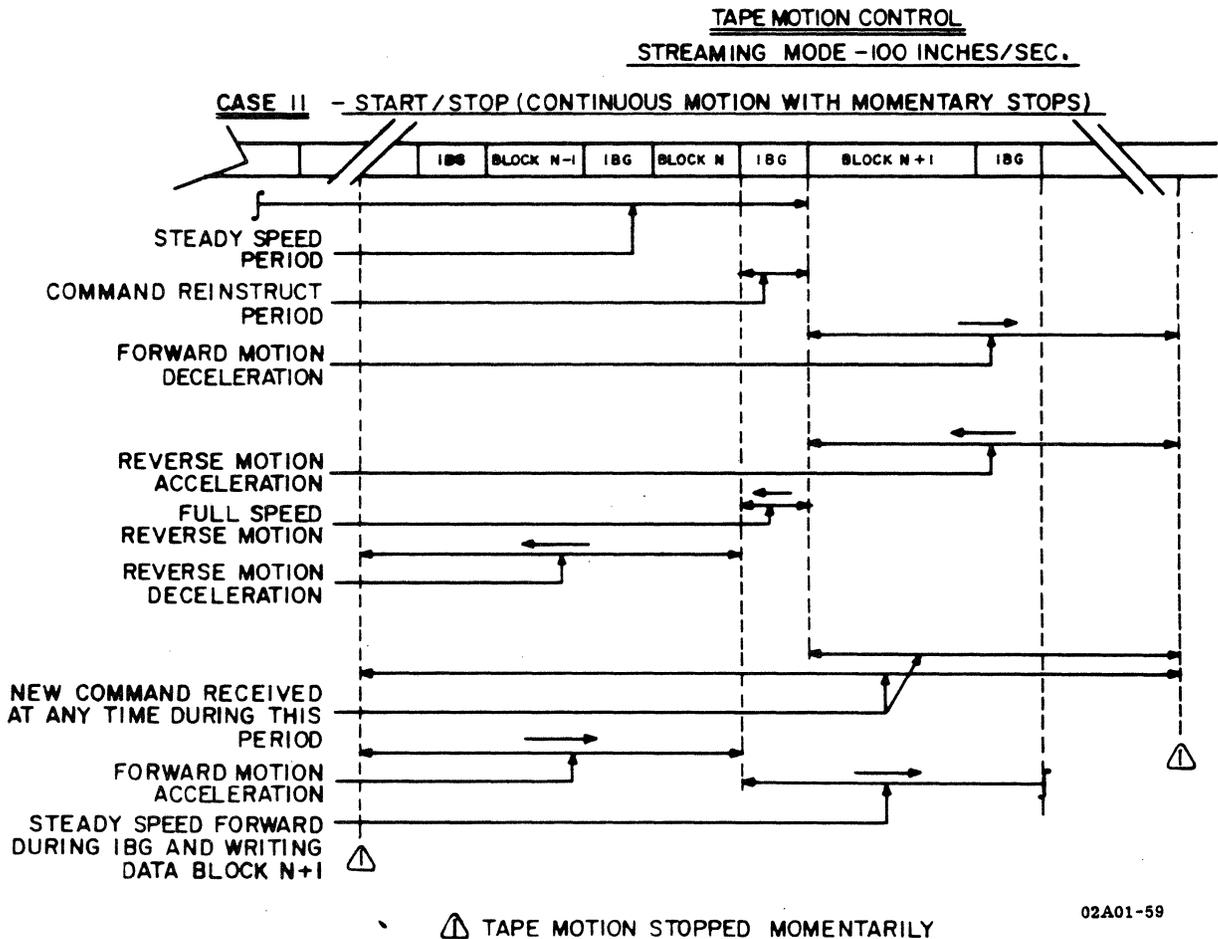
Figure 4-37. TAPE MOTION CONTROL - CASE 2 (Cont'd)
