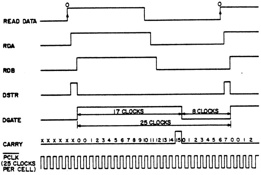
Figure 4-24. PE RECOVERY - DATA CELL TIMING
