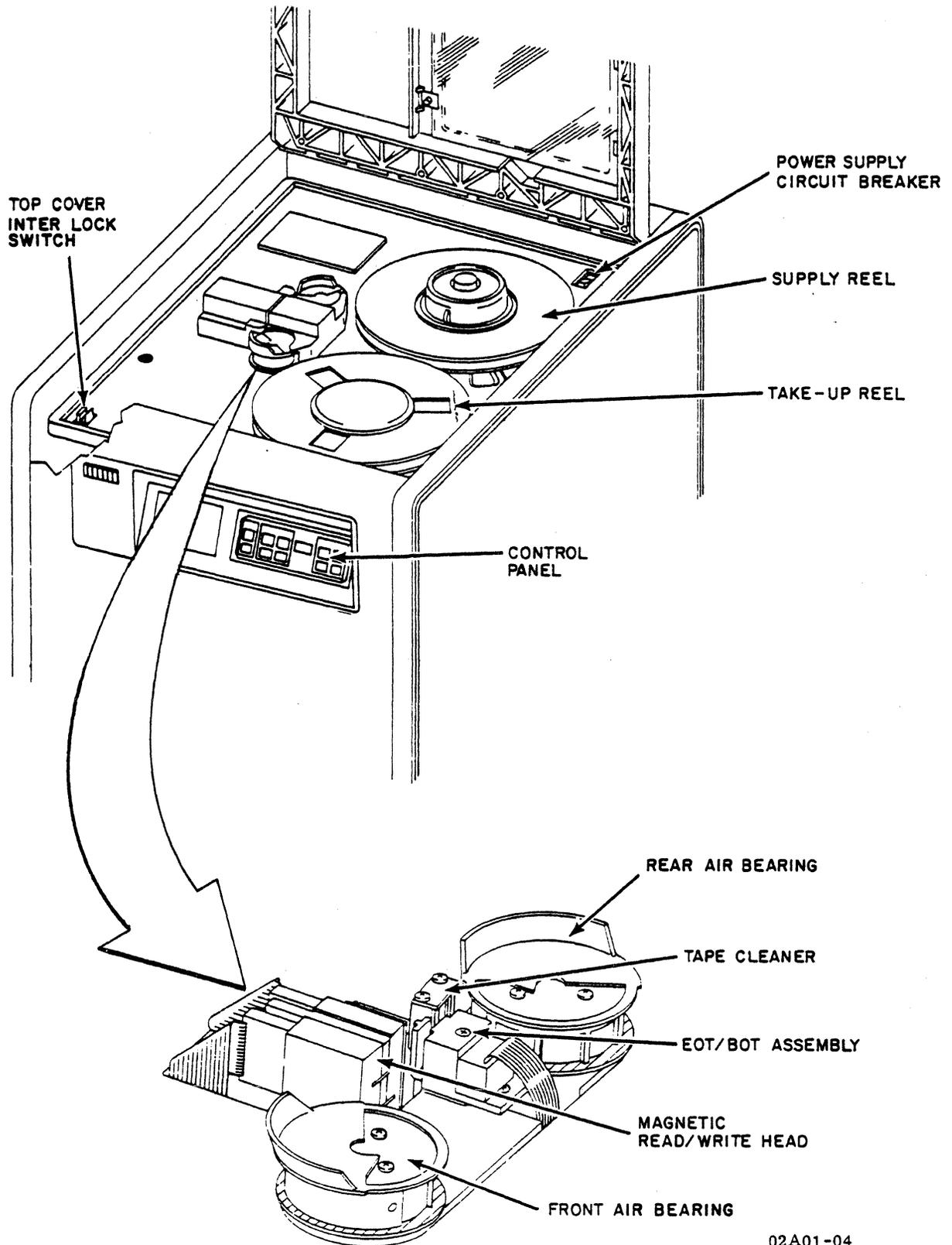
Figure 1-3. TAPE DECK COMPONENT LOCATIONS, TOP VIEW
