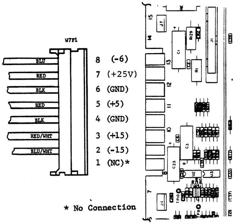
Figure 5-22. DC VOLTAGE CHECKS
