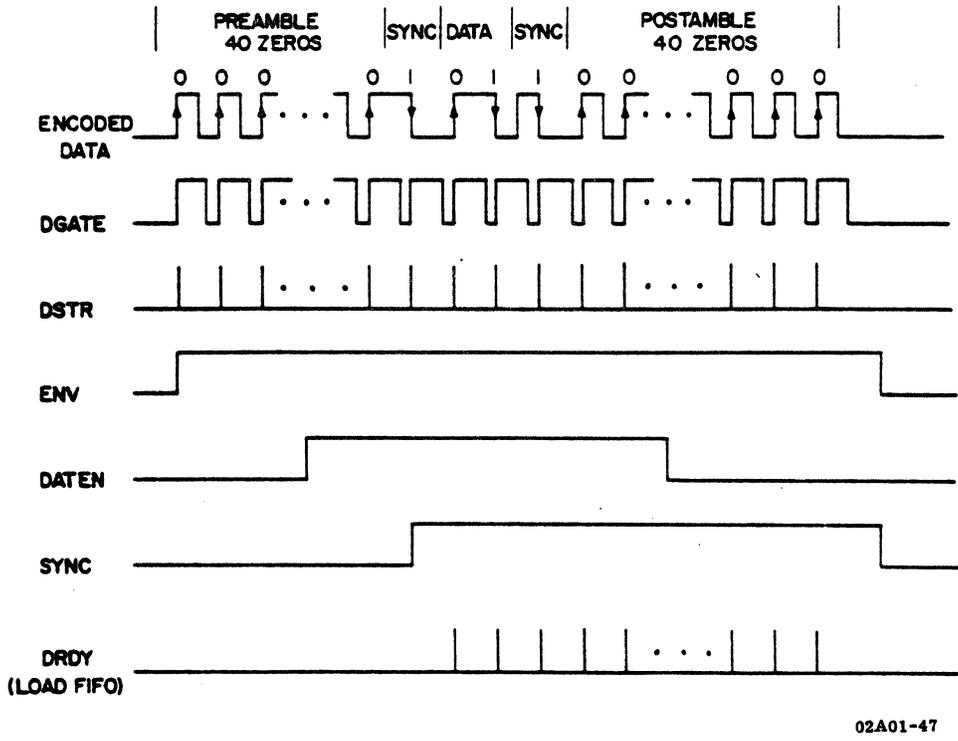
Figure 4-25. PE READ RECOVERY TIMING
