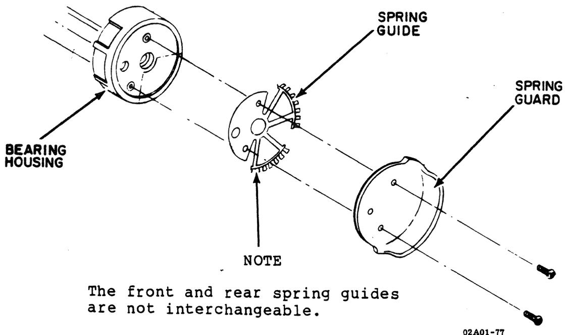
Figure 5-11. AIR BEARING SPRING GUIDE
