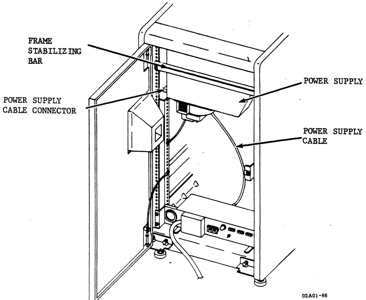
Figure 5-20. POWER SUPPLY (REAR CABINET VIEW)
