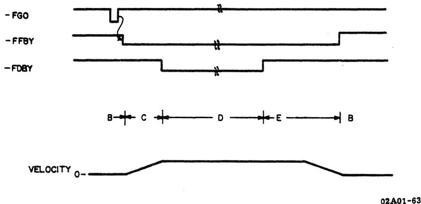
Figure 4-41. START/STOP - NO NEW COMMAND RECEIVED
