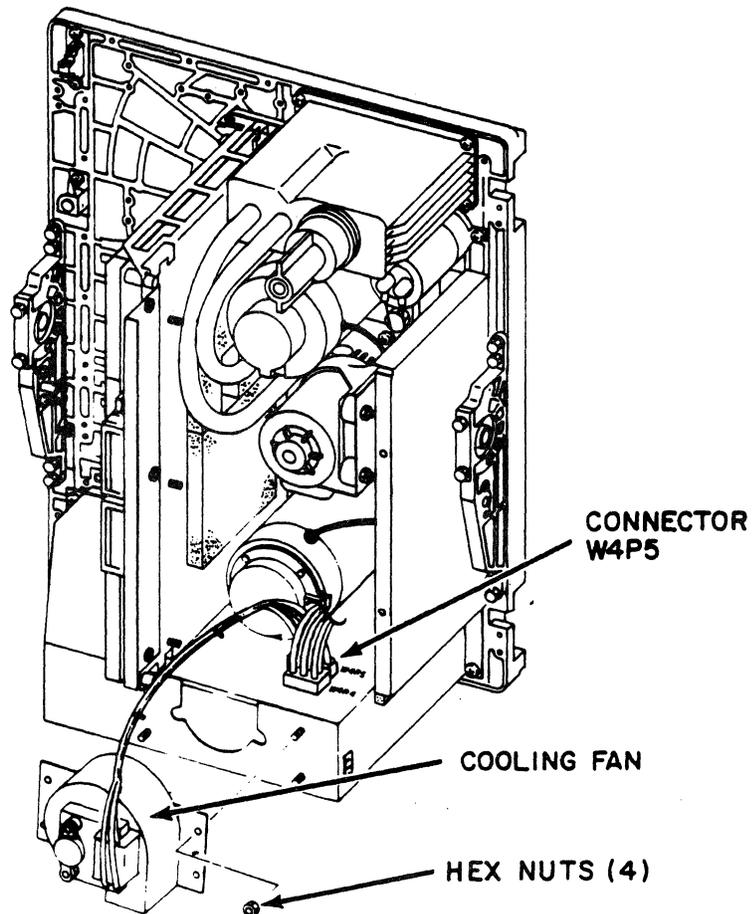
Figure 5-18. COOLING FAN ASSEMBLY 02A01-84
