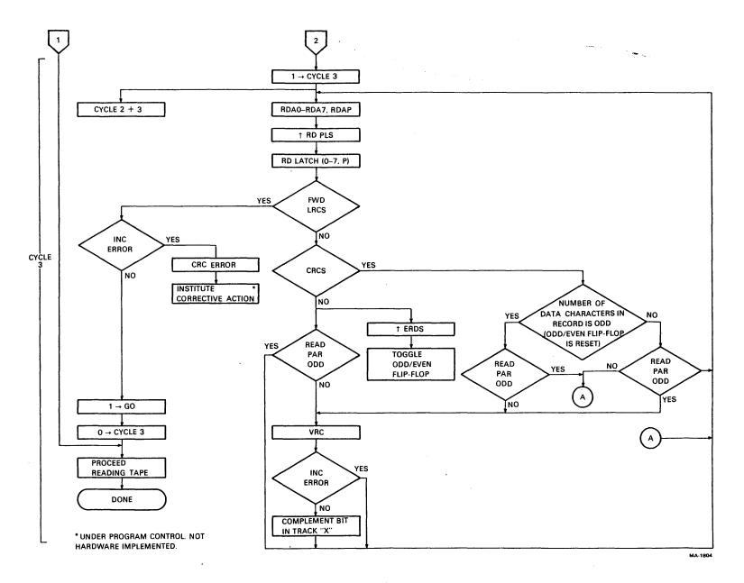
Figure 4-38 NRZI Error Correction Cycle Flow Diagram (Sheet 2 of 2)
