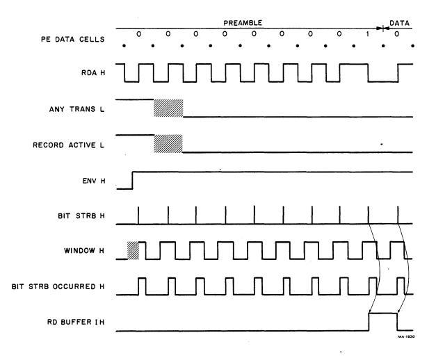
Figure 4-34 Data Discriminator Timing Diagram
