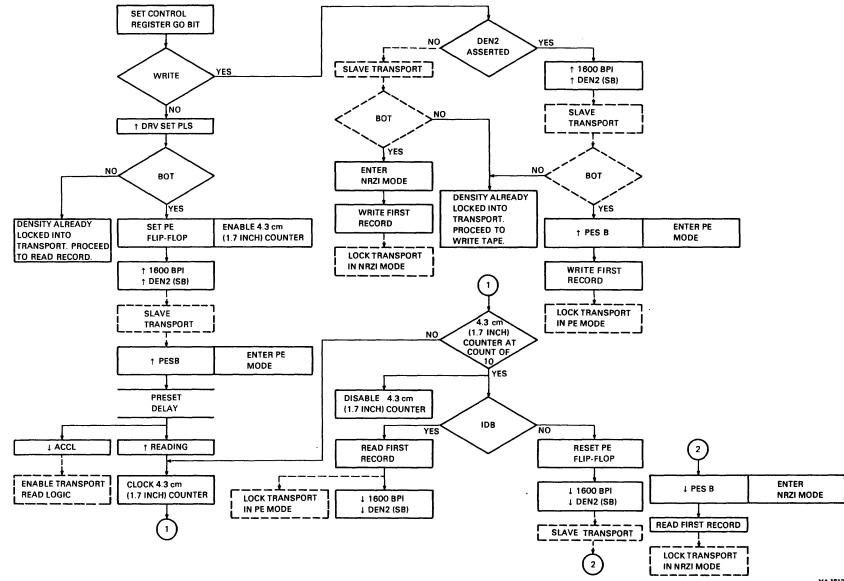
Figure 4-27 Density Select Flow Diagram
