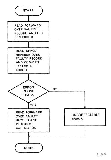
Figure 2-9 Simplified NRZI Error Correction Flow Diagram
