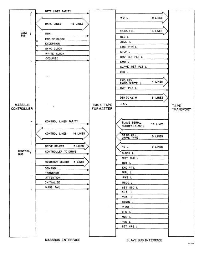
Figure 4-1 TM03 Interface Signals
