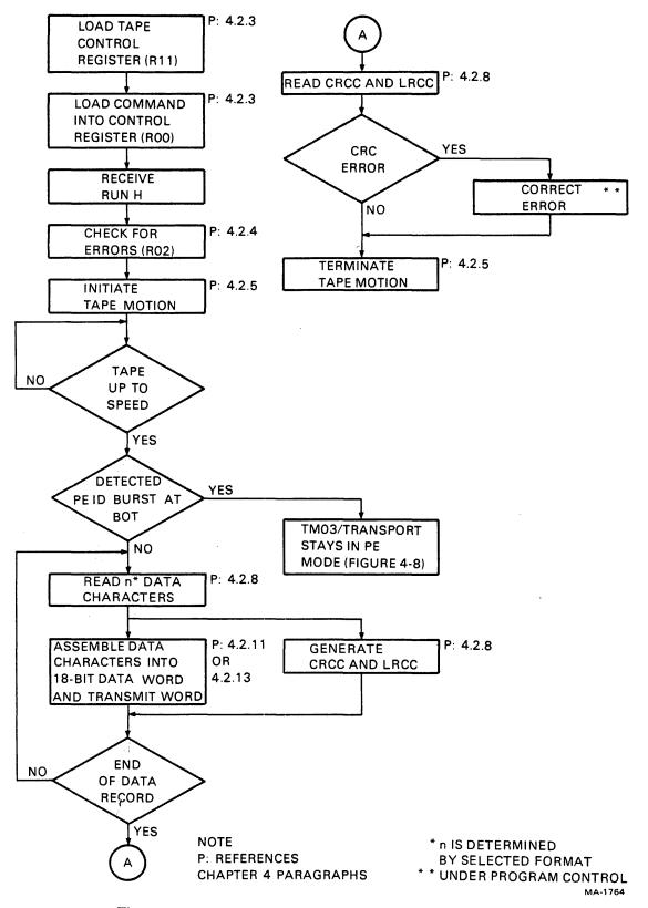
Figure 4-9 NRZI Read (Forward) Operational Flowchart
