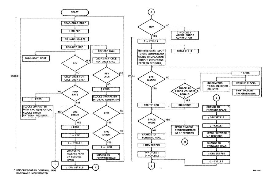
Figure 4-38 NRZI Error Correction Cycle Flow Diagram (Sheet 1 of 2)
