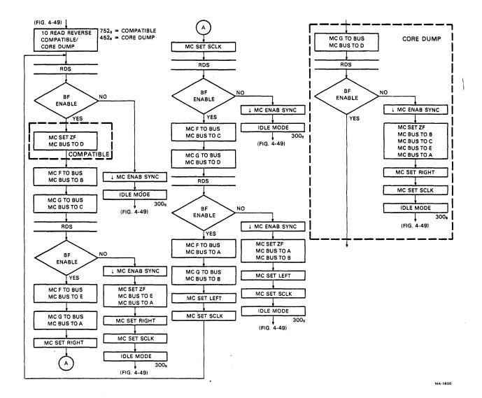
Figure 4-56 PDP-10 Read Reverse Flow Diagram
