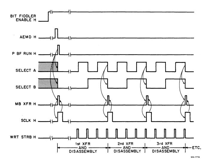
Figure 4-62 Bit Fiddler Write Operation in Core Dump Mode
