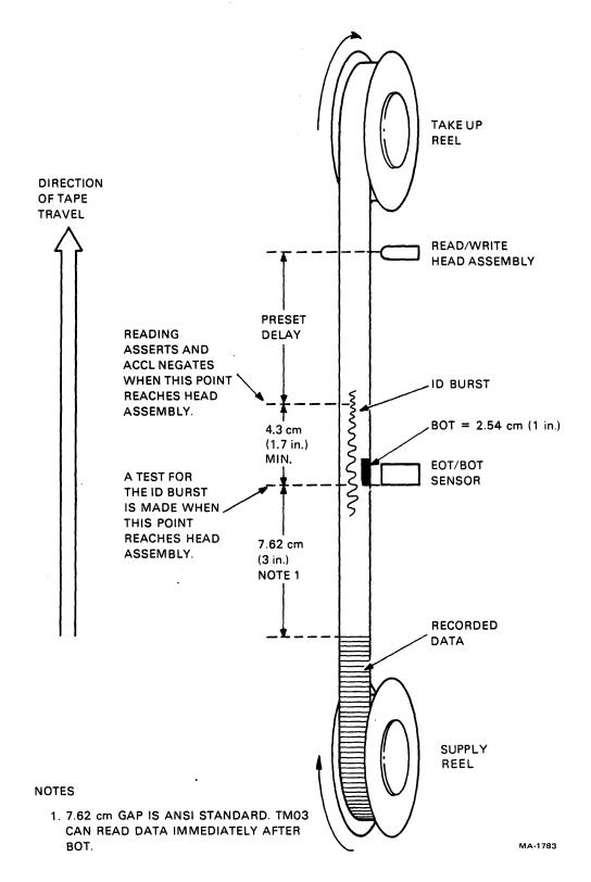
Figure 4-26 Magnetic Tape Positioned at BOT
