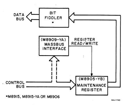
Figure 4-16 Formatter Read Wrap-Around (WRP3)
