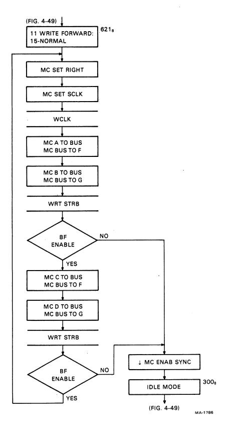
Figure 4-51 PDP-11 Write Forward: (15-Normal) Flow Diagram
