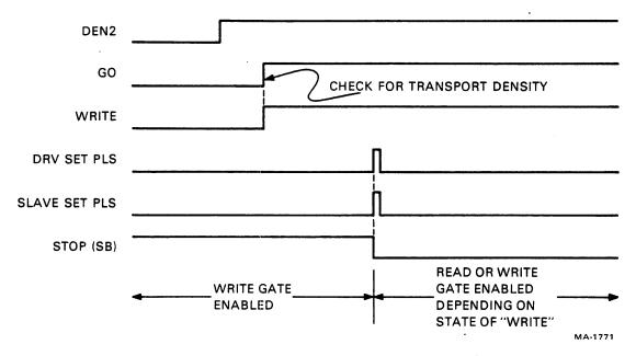
Figure 4-29 Density Select Timing
