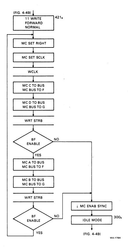
Figure 4-50 PDP-11 Write Forward Normal Flow Diagram
