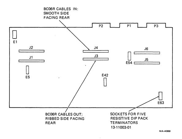
Figure 3-8 Cable Orientation on M8940 MTA Module
