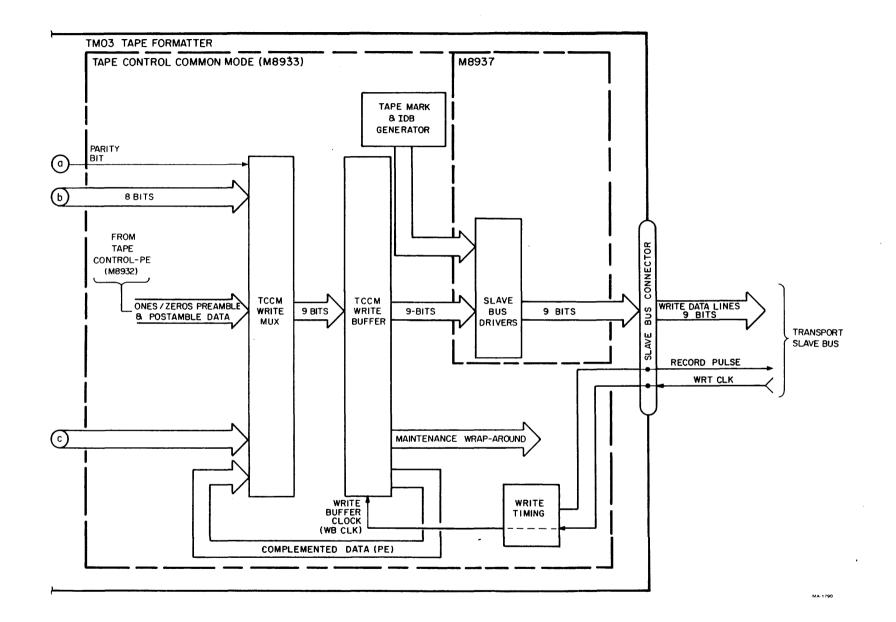
Figure 4-2 Write Data Path (Sheet 2 of 2)
