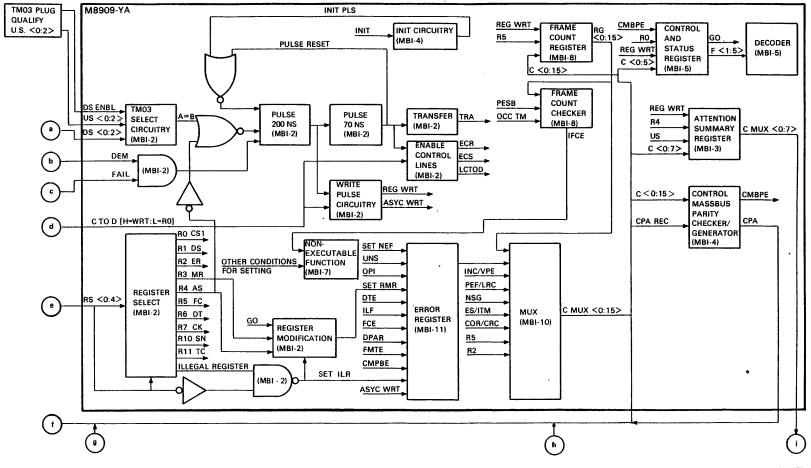
Figure 4-21 TM03 Register Read/Write (Sheet 2 of 3)
