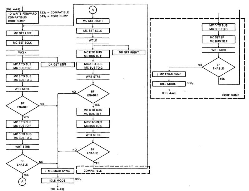
Figure 4-54 PDP-10 Write Forward Flow Diagram
