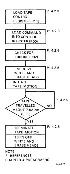
Figure 4-7 Erase Operational Flowchart
