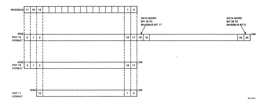
Figure 4-45 Processor Data Word Formats on Massbus
