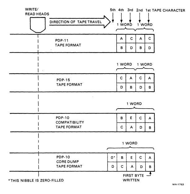
Figure 4-44 Tape Recording Formats
