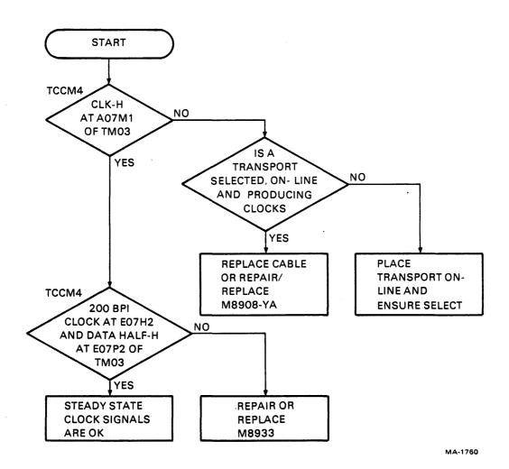
Figure 5-8 Steady State Clock Trouble Analysis
