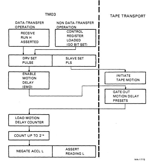
Figure 4-24 Tape Motion Initiation Flowchart
