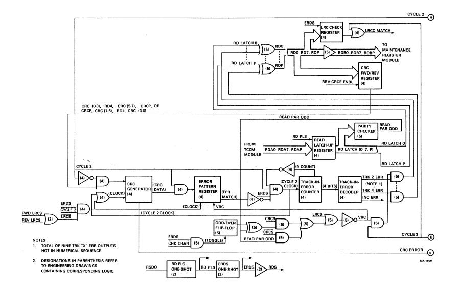
Figure 4-39 NRZI Error Correction Block Diagram (Sheet 1 of 2)
