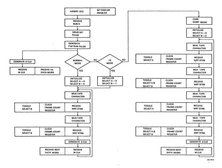
Figure 4-59 M8906 Bit Fiddler Write Operation Flowchart
