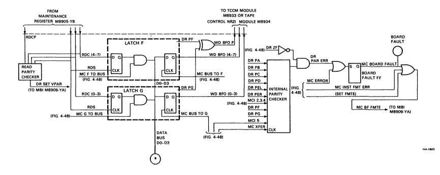
Figure 4-47 Write/Read Data Paths (Sheet 1 of 2)
