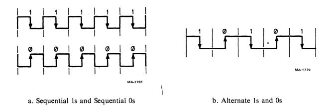
Figure C-2 PE Waveforms
