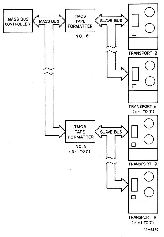
Figure 1-1 TM03 Tape Transport System Configuration
