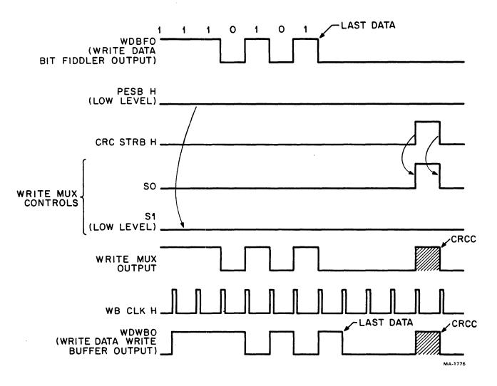
Figure 4-41 TCCM Write Operation Timing (NRZI, 1 of 9 tracks)
