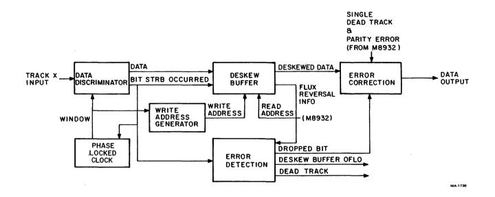
Figure 4-32 One Section of the Data Sync Module
