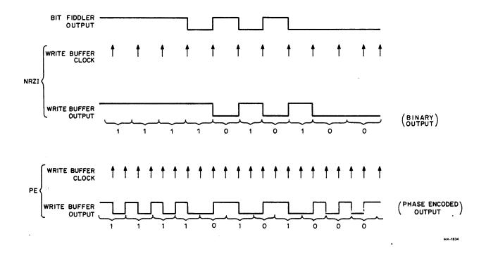
Figure 4-3 TCCM Write Timing
