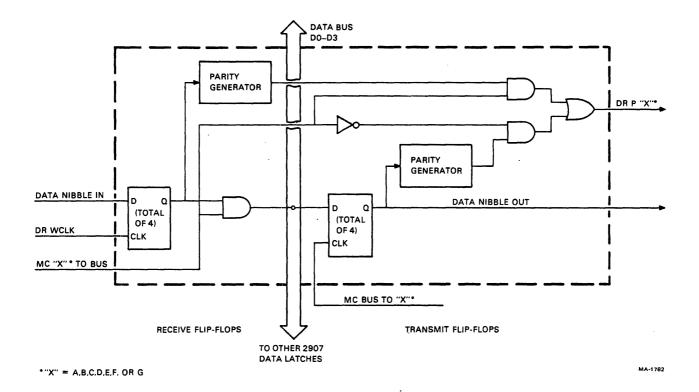
Figure 4-46 2907 Latch Logic
