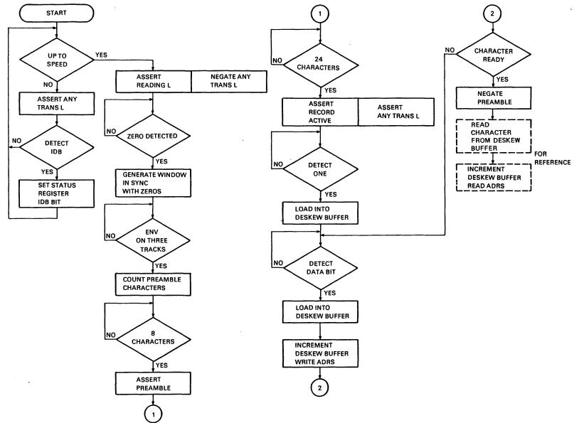
Figure 4-35 Preamble/IDB Detection Flowchart
