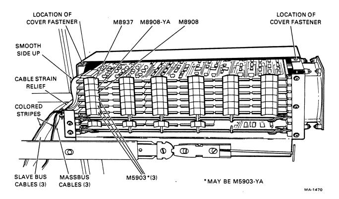
Figure 3-1 TM03 Formatter with Cover Removed
