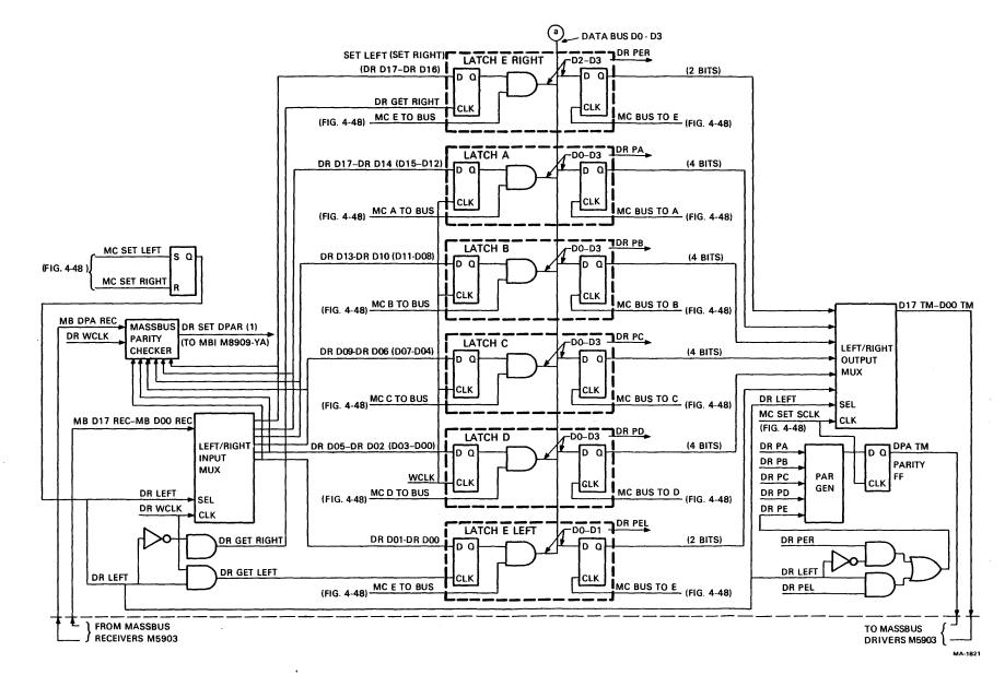
Figure 4-47 Write/Read Data Paths (Sheet 2 of 2)
