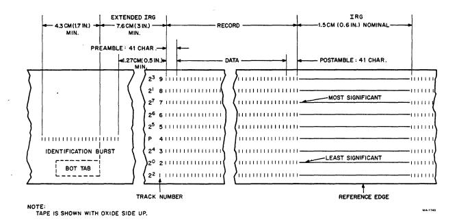
Figure C-4 PE Recording Format
