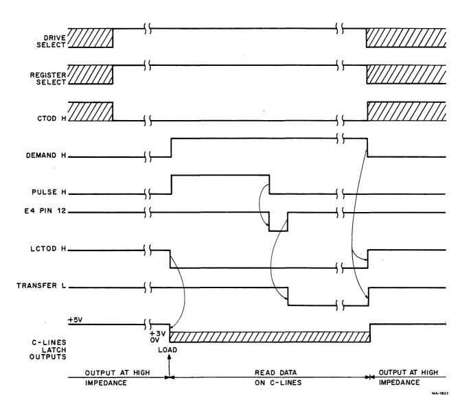
Figure 4-20 Register Read Timing Diagram
