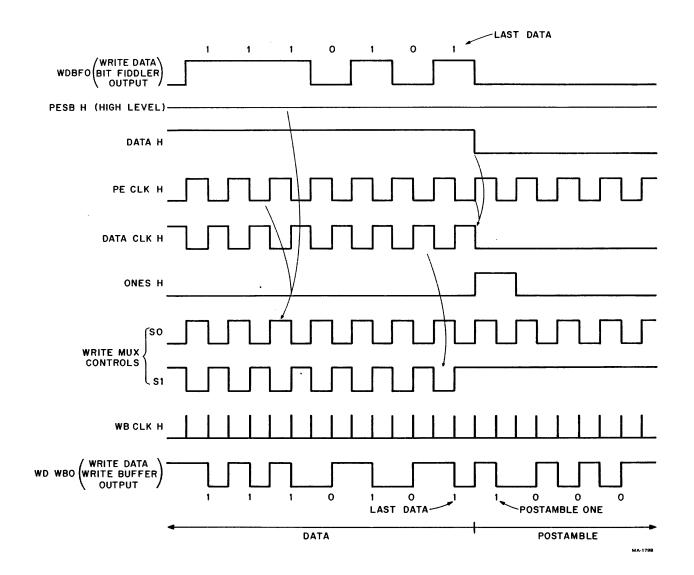
Figure 4-40 TCCM Write Operation Timing (PE)
