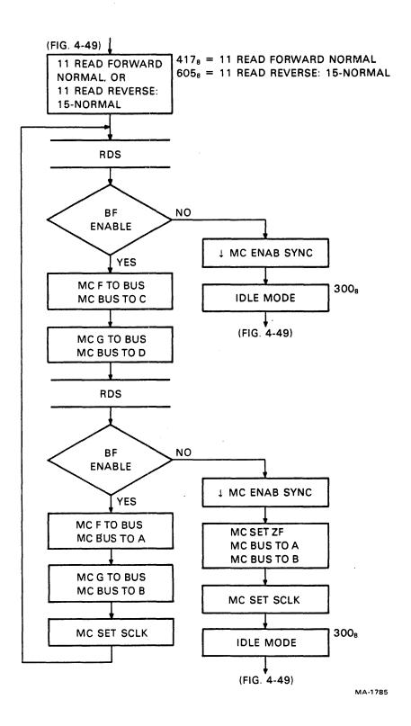
Figure 4-52 PDP-11 Read Forward Normal/PDP-11 Read Reverse (15-Normal) Flow Diagram
