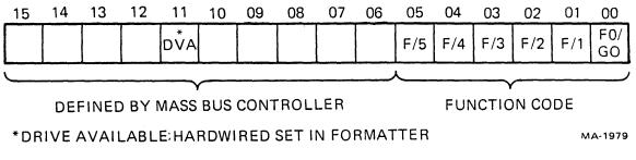
Figure 2-1 Control Register Format
