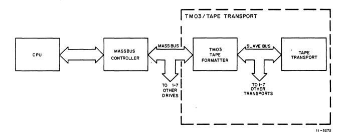
Figure 1-6 TM03 in a System Configuration
