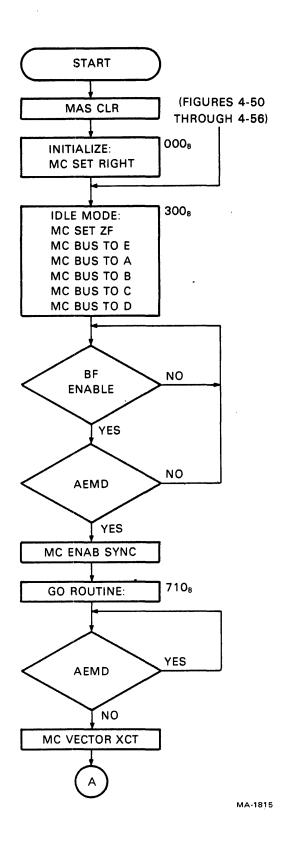
Figure 4-49 Program Startup Flow Diagram (Sheet 1 of 2)
