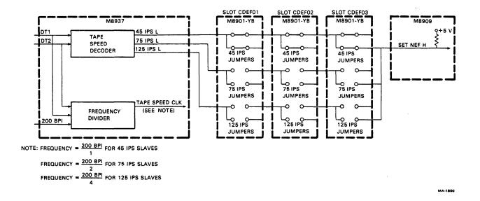
Figure 4-30 Tape Speed Selection Block Diagram
