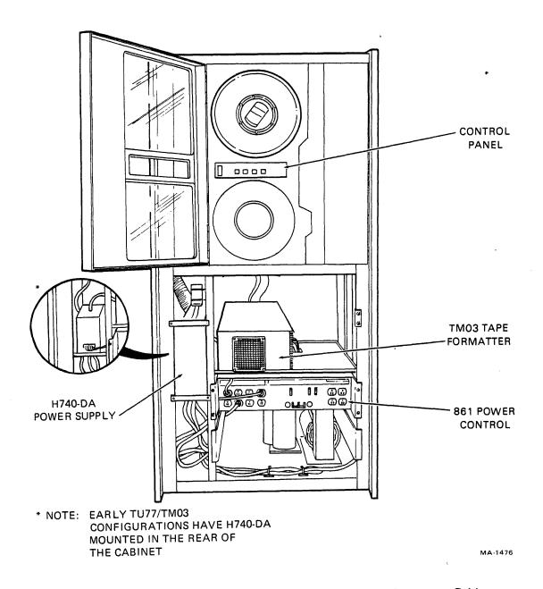
Figure 1-4 TM03 with TU77 Tape Transport in H9500 Corporate Cabinet
