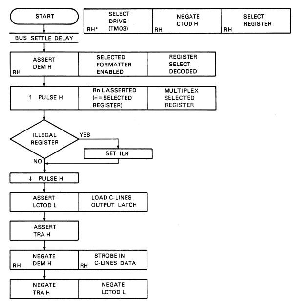
\* RH INDICATES THAT THE OPERATION IS PERFORMED BY THE MASSBUS CONTROLLER.
