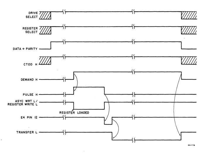
Figure 4-18 Register Write Timing Diagram
