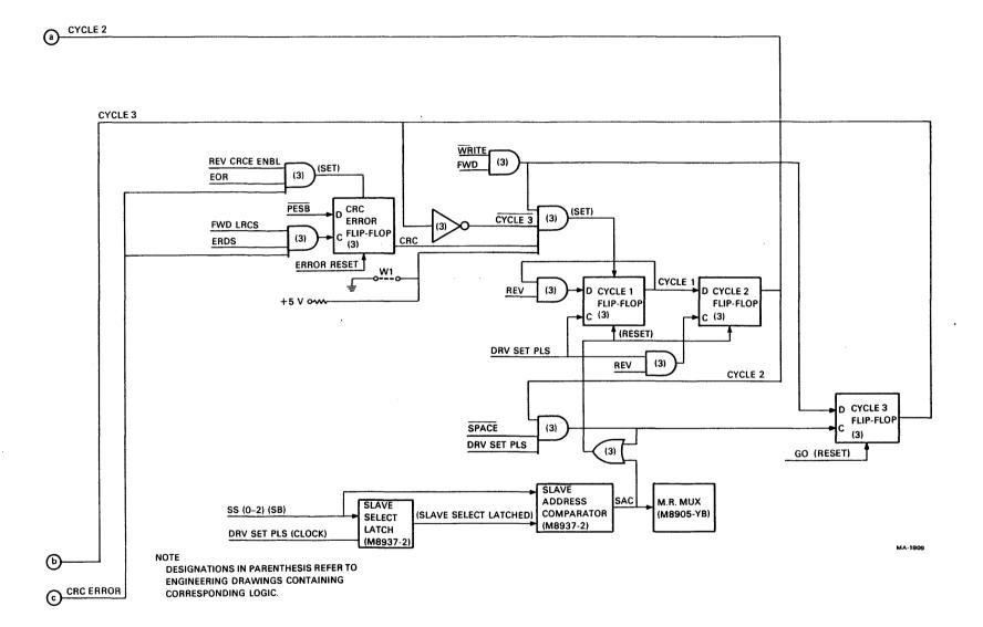
Figure 4-39 NRZI Error Correction Block Diagram (Sheet 2 of 2)
