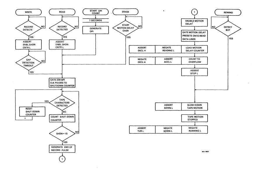
Figure 4-25 Tape Motion Termination Flowchart
