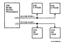
Figure 6-3 Memory Chip Select Lines (MP-2059, CS, Sheets 2 and 3)
