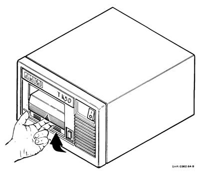
Figure 3-7 Lifting Cartridge Insert/Release Handle
