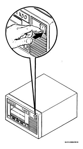
Figure 3-14 Turning Off Power
