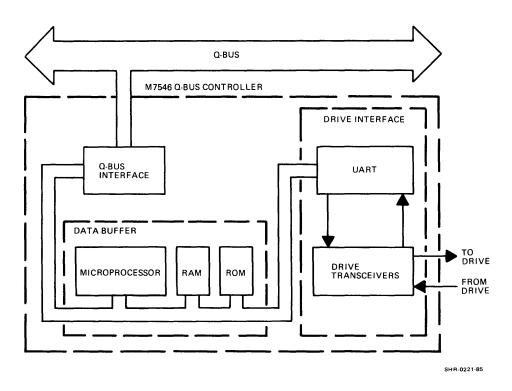
Figure 5-1 TQK50 High Level Block Diagram
