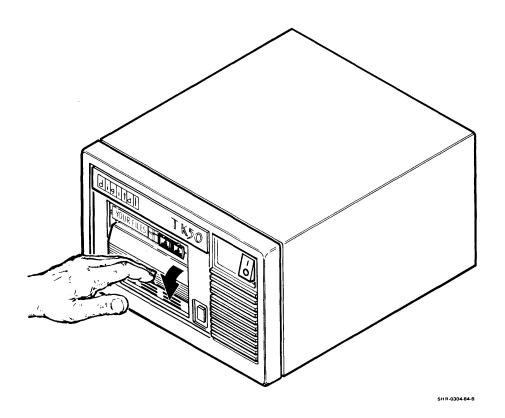
Figure 3-9 Lowering Cartridge Insert/Release Handle
