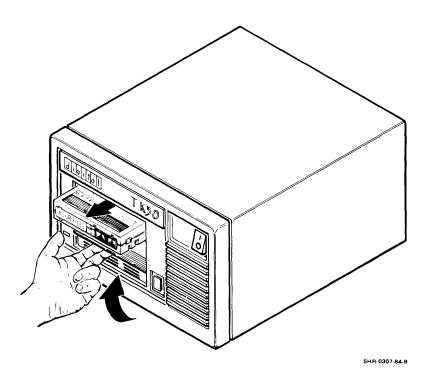
Figure 3-12 Ejecting Tape Cartridge (After Rewind)
