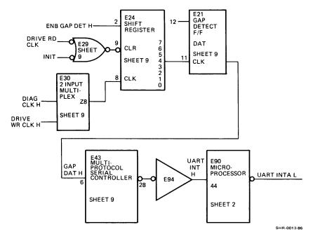
Figure 6-7 Enable Gap Detect Circuit (MP-2059, CS, Sheets 2 and 9)
