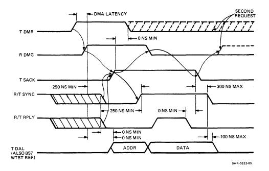
Figure 5-2 Q-bus Timing
