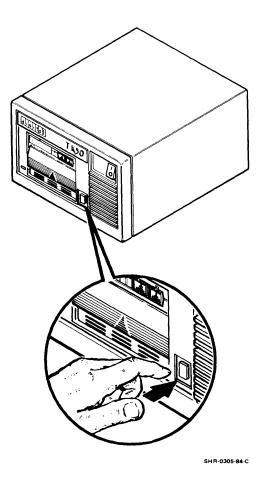
Figure 3-10 Setting Load/Unload Switch to Load
