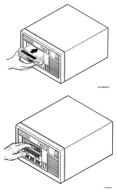
Figure 3-8 Inserting Tape Cartridge
