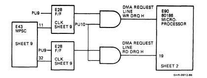
Figure 6-6 DMA Channel (MP-2059, CS, Sheets 2 and 9)
