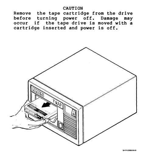
Figure 3-13 Removing Tape Cartridge
