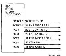
Figure 6-4 Peripheral Chip Select Lines (MP-2059, CS, Sheet 2)
