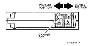
Figure 3-3 Write-Protecting Tape
