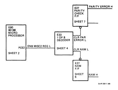
Figure 6-5 FPLS Interrupt (MP-2059, CS, Sheets 2,4,6,&7)
