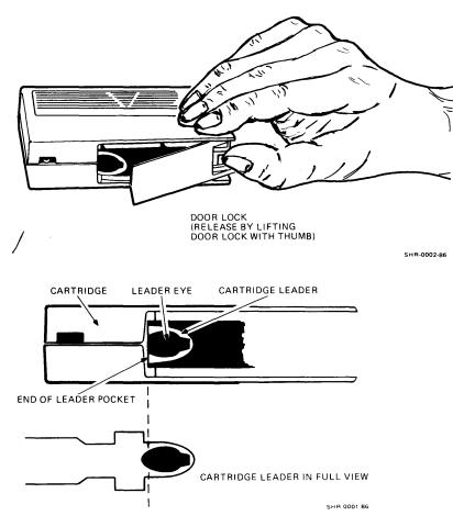
Figure 3-1 Inspecting Tape Cartridge
