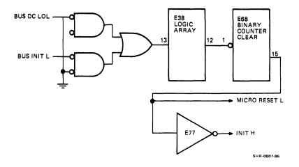
Figure 6-1 Power Up Reset Circuitry
