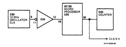
Figure 6-2 Microprocessor Timing Circuit (MP-2059, CS, Sheet 2)
