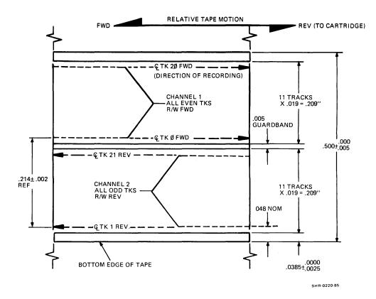
Figure 2-8 Recording Direction
