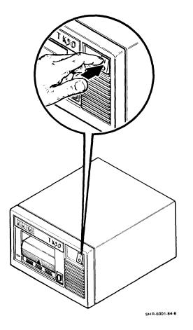
Figure 3-6 Turning on Power
