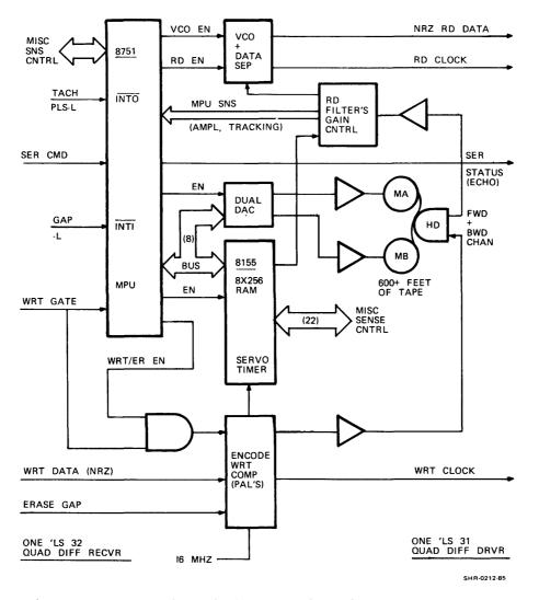
Figure 2-3 Simplified Logic Diagram: TK50 Tape Drive
