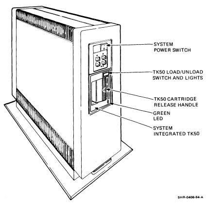
Figure 2-1 System Integrated TK50
