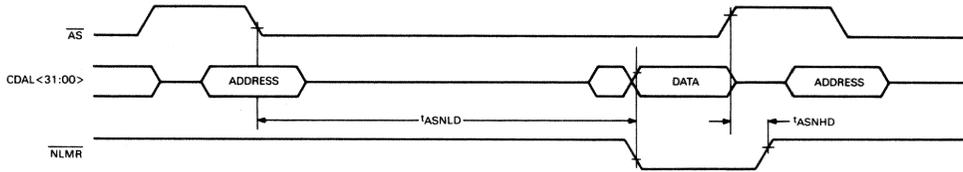
Figure 38 • CVAX 78588 DMA Address Miss Timing (NOP)
