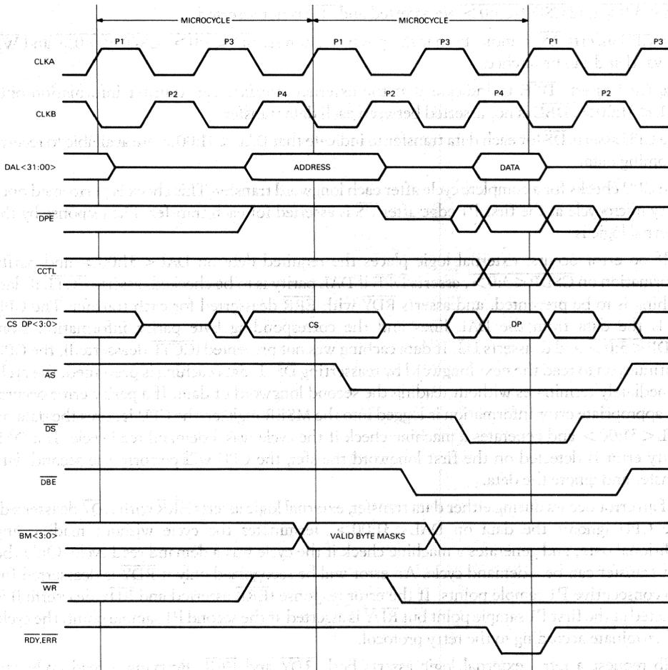
Figure 41 • CVAX 78034 Single Transfer CPU Read Cycle
