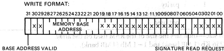
Figure 4 • CVAX 78588 Configuration Registers (CSR0-CSR15) Write Format
