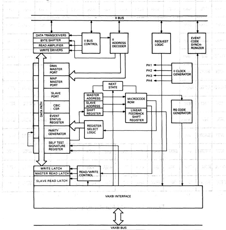
Figure 1 • DC514 VAXBI Bus Interface Chip Block Diagram
