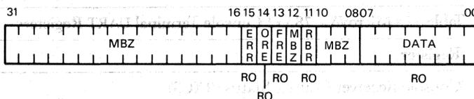
Figure 9 • MicroVAX 78332 Receiver Data Buffer (CSR/RXDB) Register Format
