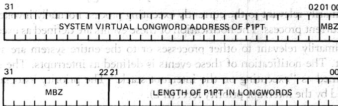
Figure 25 • CVAX 78034 P1 Region Mapping Registers Format
