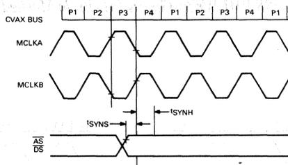
Figure 34 • CVAX 78588 Synchronizer Timing for Asynchronous DMA Operations
