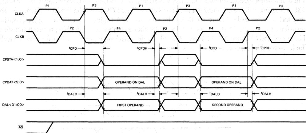
Figure 65 • CVAX 78034 Double-precision CPU to CFPA Transfer Timing
