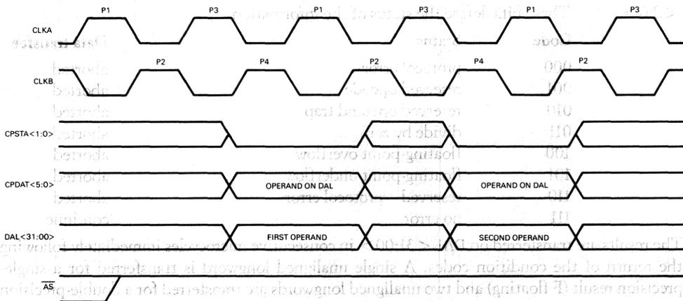
Figure 49 • CVAX 78034 Double-precision CPU to CFPA Transfer
