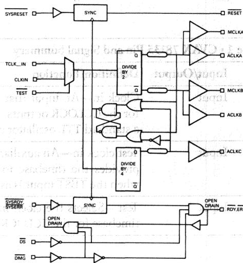
Figure 1 • CVAX 78135 Clock Generator Logic Diagram
