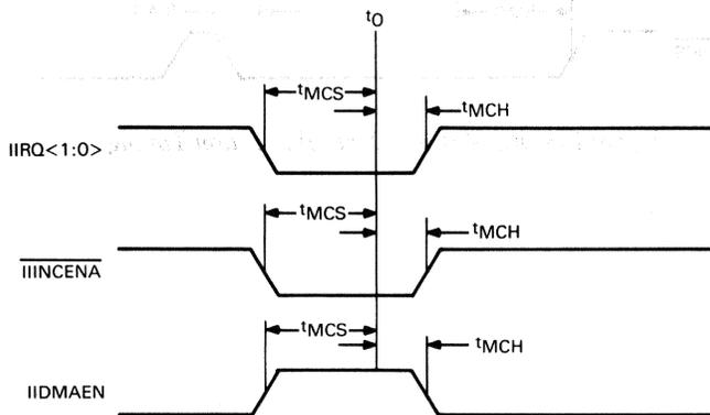
Figure 20 • DC514 Master-port Control Signal Timing
