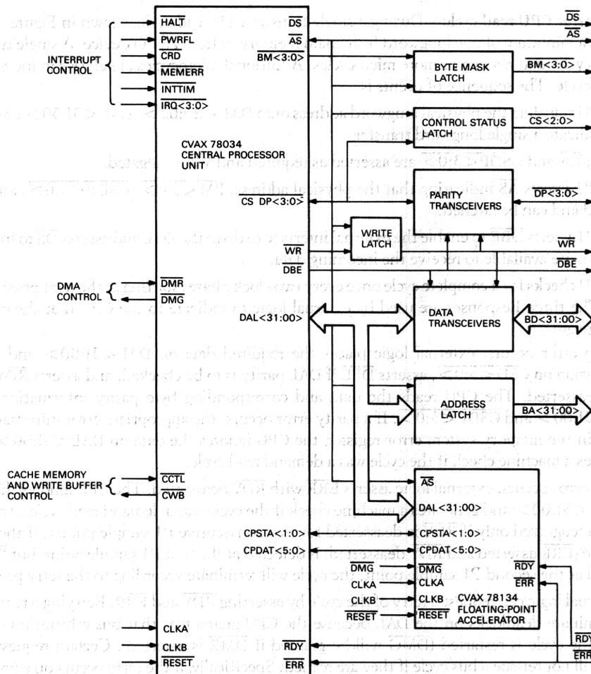
Figure 39 • CVAX 78034 CPU Bus Connections
