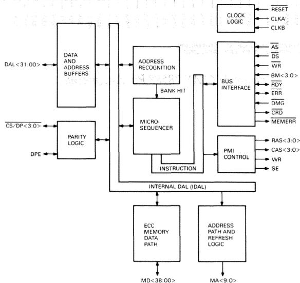
Figure 1 • CVAX 78588 Memory Controller Functional Block Diagram
