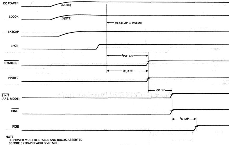
Figure 15 • CVAX 78711 Unsequenced Powerup (ac Power Normal) Timing
