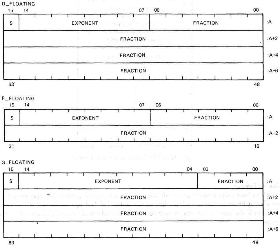
Figure 12 • CVAX 78034 Floating-point Data Types
