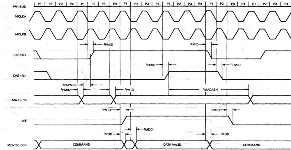
Figure 27 • CVAX 78588 PMI Write Timing (Single Unmasked Transfer)
