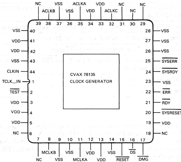
Figure 2 • CVAX 78135 Pin Assignments
