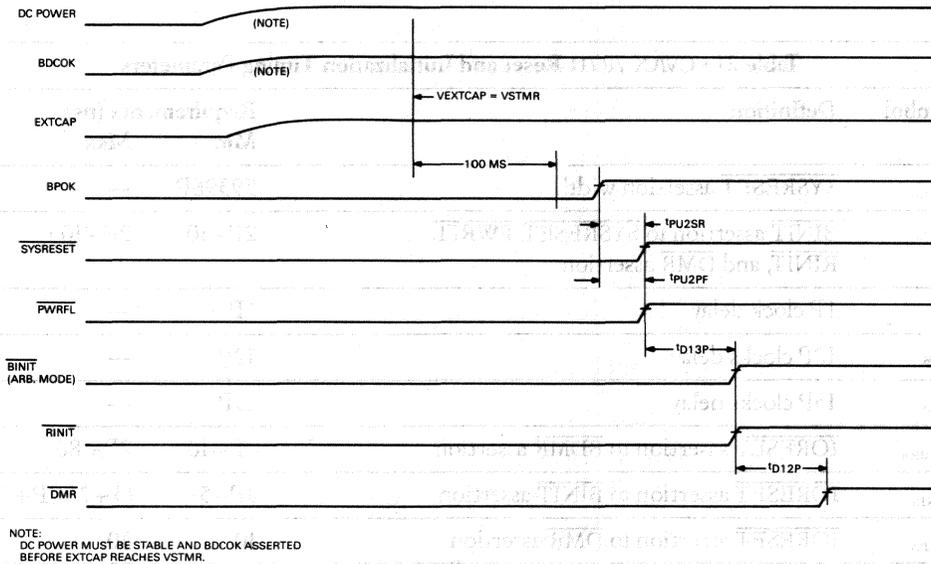
Figure 16 • CVAX 78711 Unsequenced Powerup (ac Power Failure) Timing
