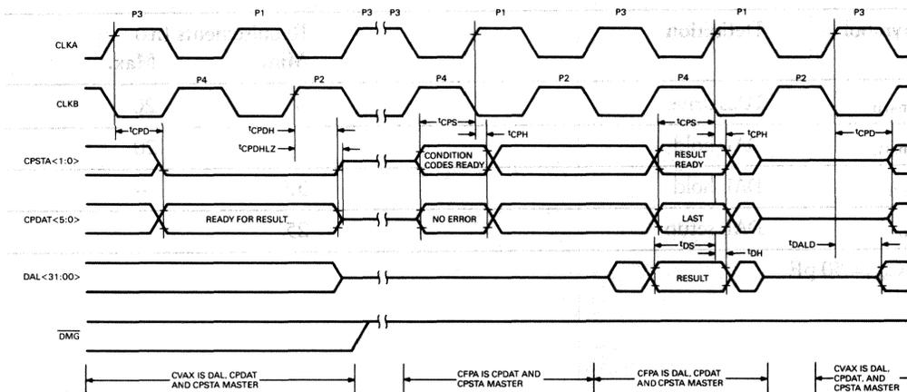
Figure 66 • CVAX 78034 Single-precision CFPA to CPU Transfer Timing
