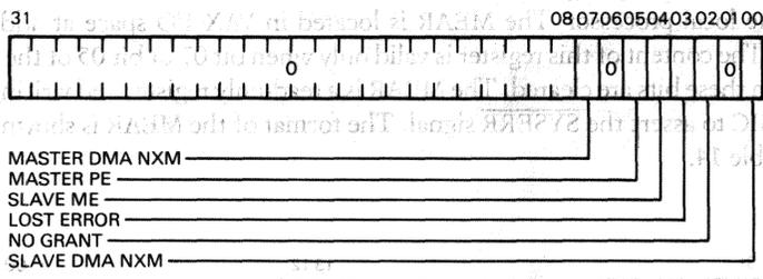
Figure 7 • CVAX 78711 DMA System Error Register Format
