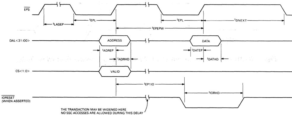
Figure 29 - MicroVAX 78332 MicroVAX EP Write Command and Write Data Transaction Timing
