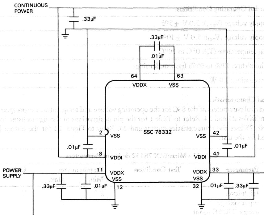
Figure 22 • MicroVAX 78332 Power Supply Connections
