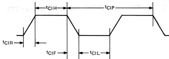
Figure 24 • MicroVAX 78332 Clock Input Waveform
