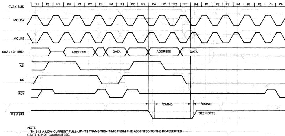
Figure 22 • CVAX 78588 CPU Write Timing (Single—Unmasked)
