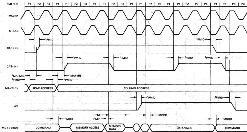
Figure 28 • CVAX 78588 PMI Write Timing (Single Masked Transfer)
