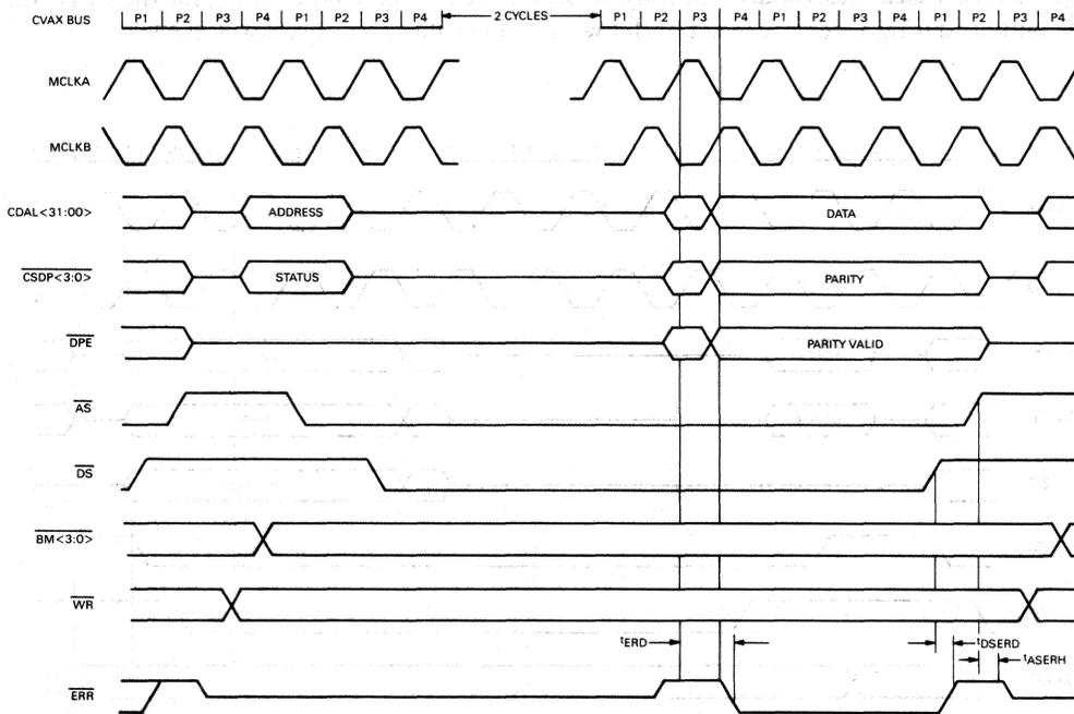
Figure 17 • CVAX 78588 CPU or Synchronous DMA Read Timing
