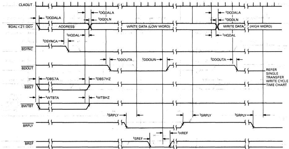
Figure 46 • CVAX 78711 CQbic to Q22-bus Block-mode Write Timing
