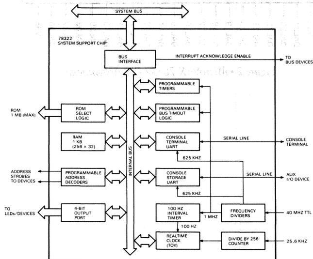
Figure 1 • MicroVAX 78332 SSC Functional Block Diagram
