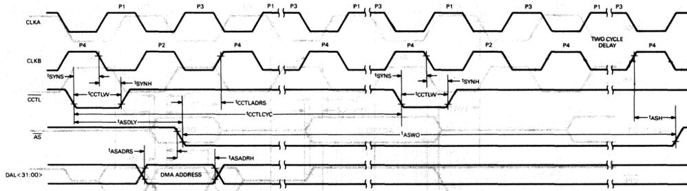
Figure 59 • CVAX 78034 Octaword Cache Invalidate Cycle Timing
