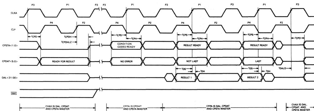
Figure 67 • CVAX 78034 Double-precision CFPA to CPU Transfer Timing
