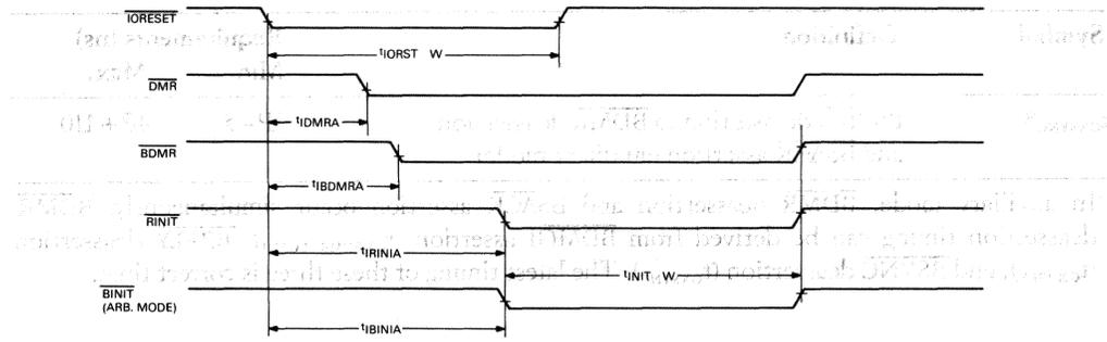
Figure 19 • CVAX 78711 I/O Reset Signal Timing
