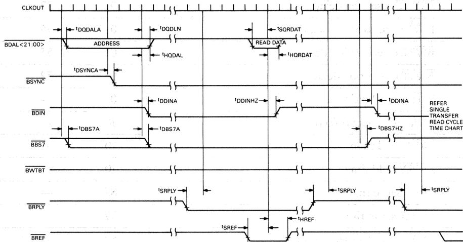
Figure 43 • CVAX 78711 Q22-bus Block-mode Multiple Transfer Read Timing
