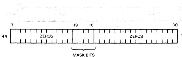
Figure 10 • DC514 Slave-port Mask Register Format
