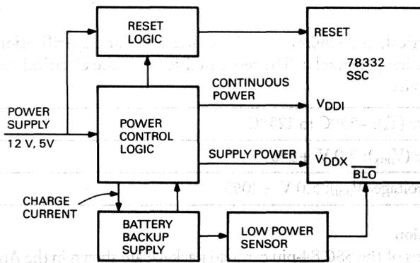
Figure 21 • MicroVAX 78332 Power Supply Interconnection
