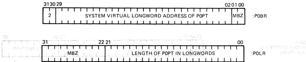
Figure 23 • CVAX 78034 P0 Region Mapping Registers Format
