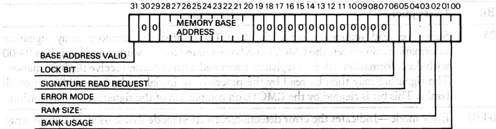
Figure 3 • CVAX 78588 Configuration Registers (CSR0-CSR15) Read Format
