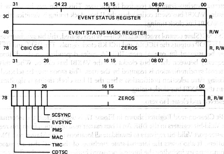
Figure 16 • DC514 Control and Status Register Format
