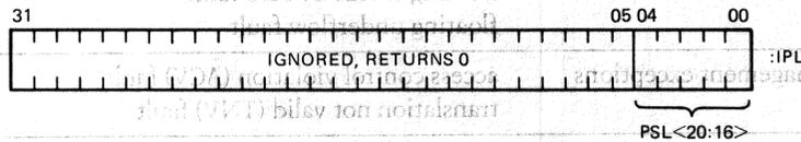
Figure 29 • CVAX 78034 Interrupt Priority Level Register Format
