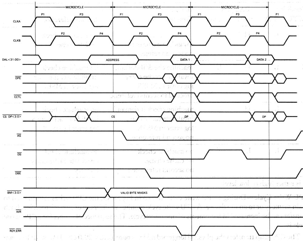
Figure 42 • CVAX 78034 Multiple Transfer CPU Read Cycle
