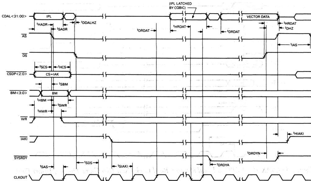
Figure 32 • CVAX 78711 CPU to CQBIC IAK Cycle Timing
