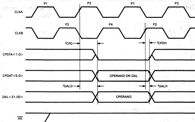
Figure 64 • CVAX 78034 Single-precision CPU to CFPA Transfer Timing
