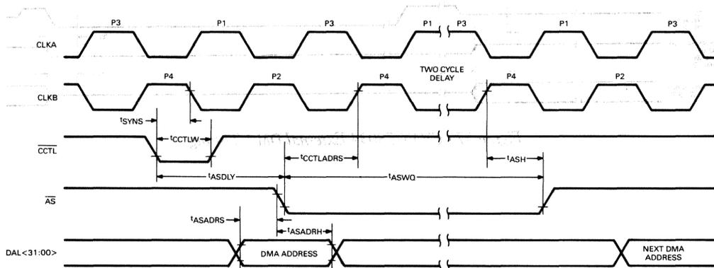
Figure 58 • CVAX 78034 Quadword Cache Invalidate Cycle Timing
