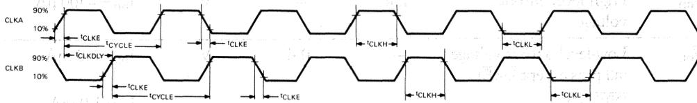
Figure 53 • CVAX 78034 Clock Input Timing
