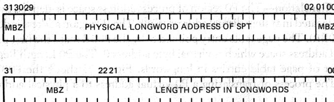
Figure 21 • CVAX 78034 System Mapping Registers Format
