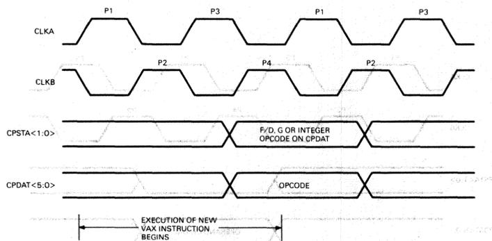
Figure 47 • CVAX 78034 Opcode Transfer Cycle
