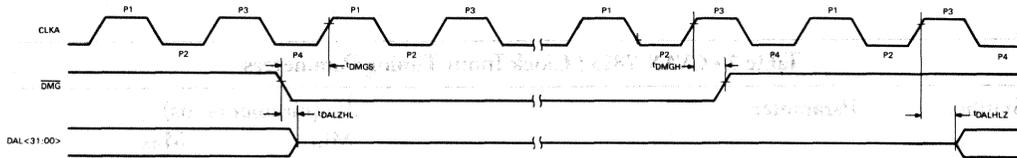
Figure 7 • CVAX 78134 External DMA Timing
