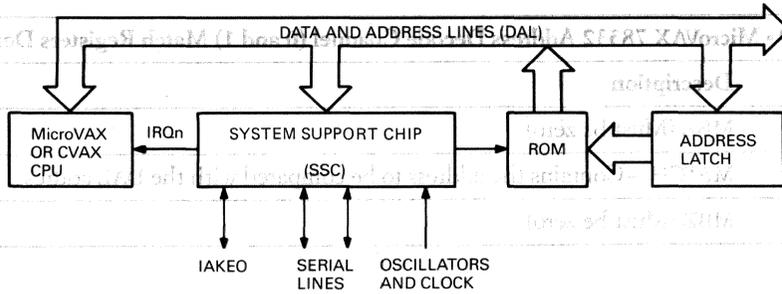
Figure 18 • MicroVAX 78332 CPU to SSC Interface System Configuration
