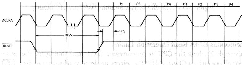
Figure 12 • CVAX 78588 Initialization Timing (Synchronous Operation)
