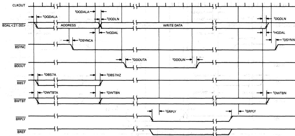
Figure 45 • CVAX 78711 Q22-bus Single Transfer Write Timing
