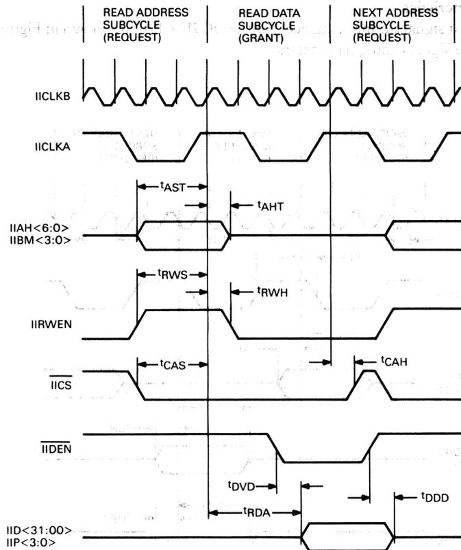
Figure 19 • DC514 II Bus Read Transaction Timing
