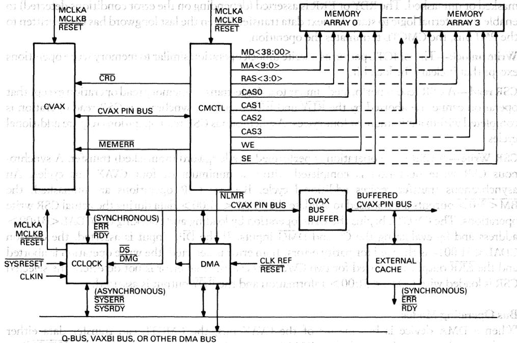
Figure 9 • CVAX 78588 CPU System Interface Diagram
