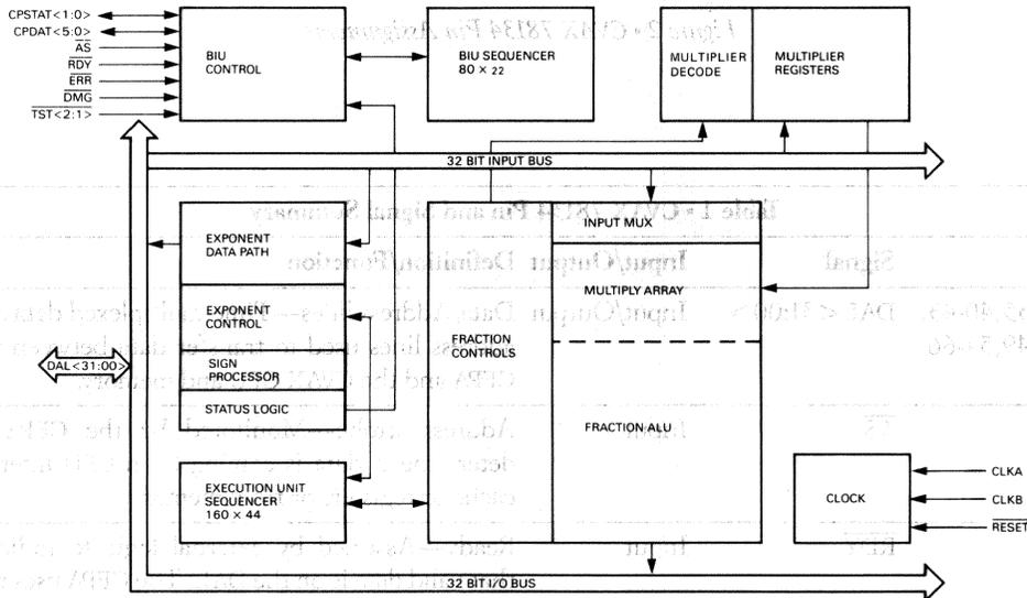
Figure 1 • CVAX 78134 Floating-point Accelerator Block Diagram
