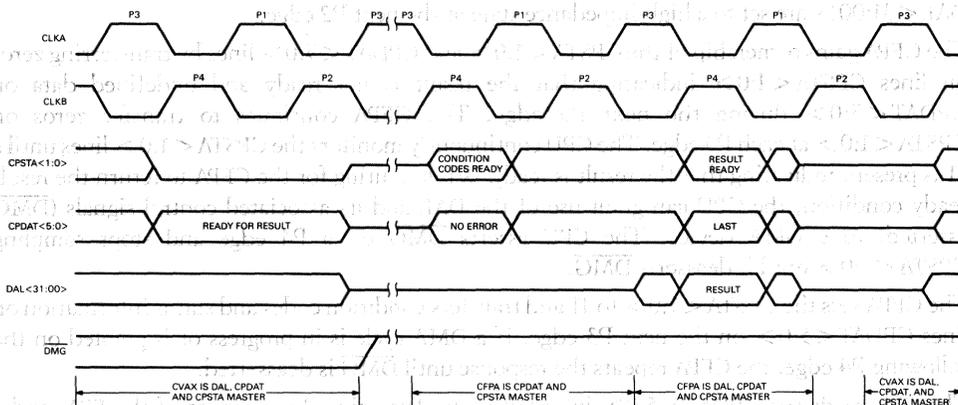
Figure 50 • CVAX 78034 Single-precision CFPA to CPU Transfer
