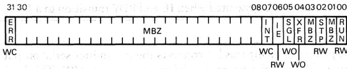
Figure 12 • MicroVAX 78332 Timer Control Registers (0 and 1) Format
