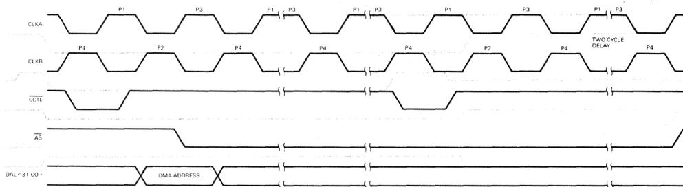
Figure 46 • CVAX 78034 Octaword Cache Invalidate Cycle
