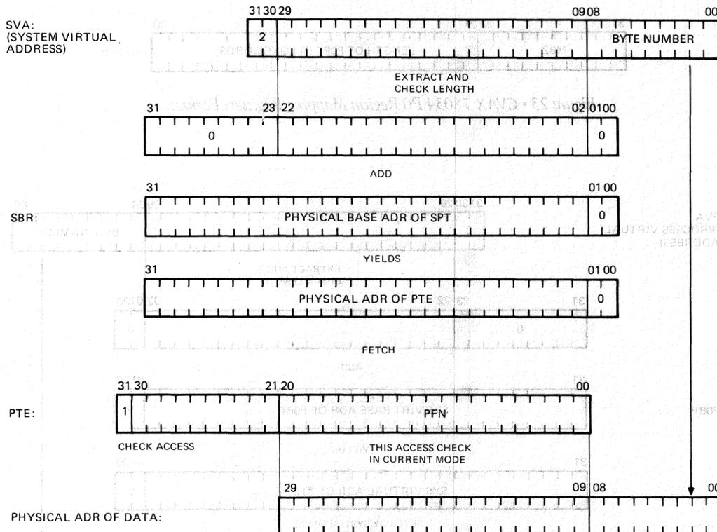
Figure 22 • CVAX 78034 System Virtual-to-physical Address Translation
