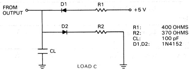
Figure 23 • MicroVAX 78332 dc Output Load Circuits
