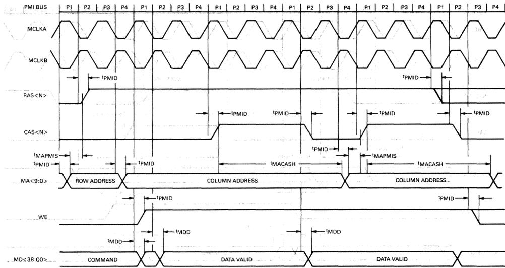
Figure 29 • CVAX 78588 PMI Write Timing (Multiple Unmasked Transfer)
