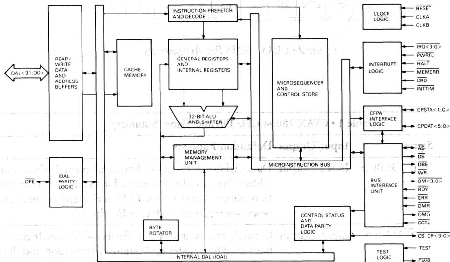
Figure 1 • CVAX 78034 Microprocessor Block Diagram
