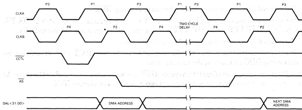
Figure 45 • CVAX 78034 Quadword Cache Invalidate Cycle
