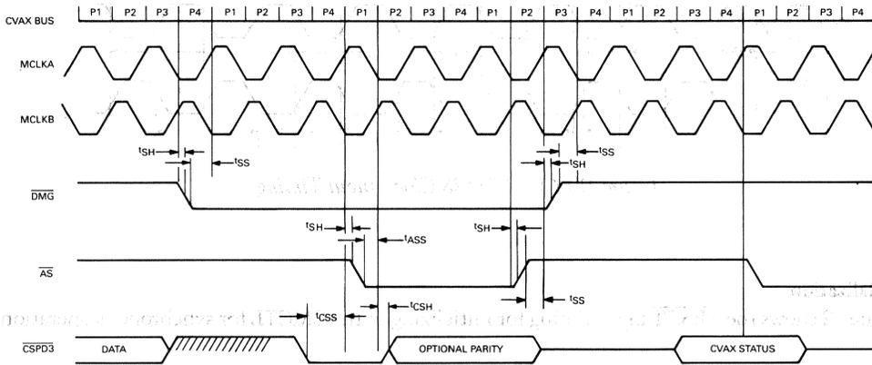
Figure 14 • CVAX 78588 Synchronous  $\overline{DMG}$  and  $\overline{AS}$  Timing
