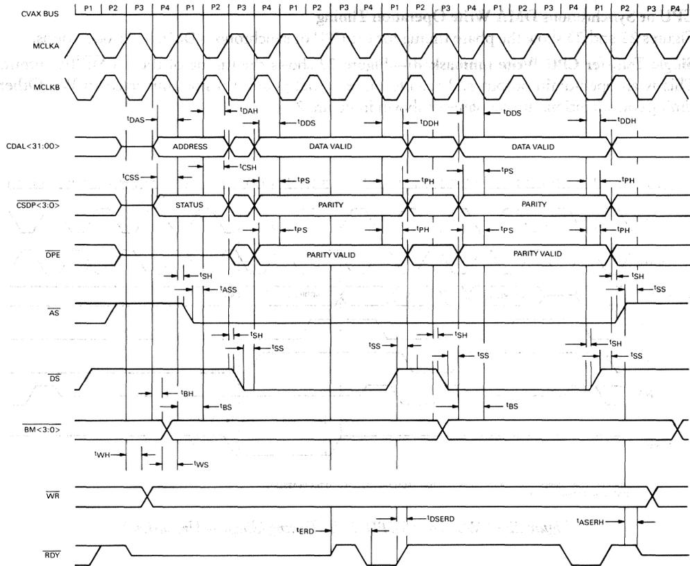
Figure 23 • CVAX 78588 Synchronous DMA Write Timing (Quadword—No Error)
