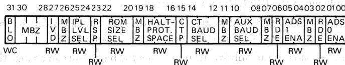
*Figure 4 • MicroVAX 78332 Configuration Register Format*
