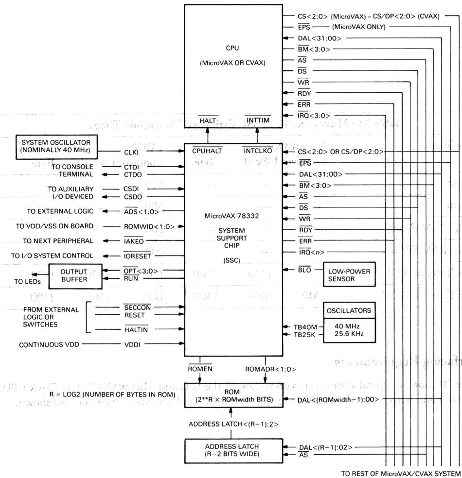
Figure 20 • MicroVAX 78332 SSC to CPU Typical Interconnections
