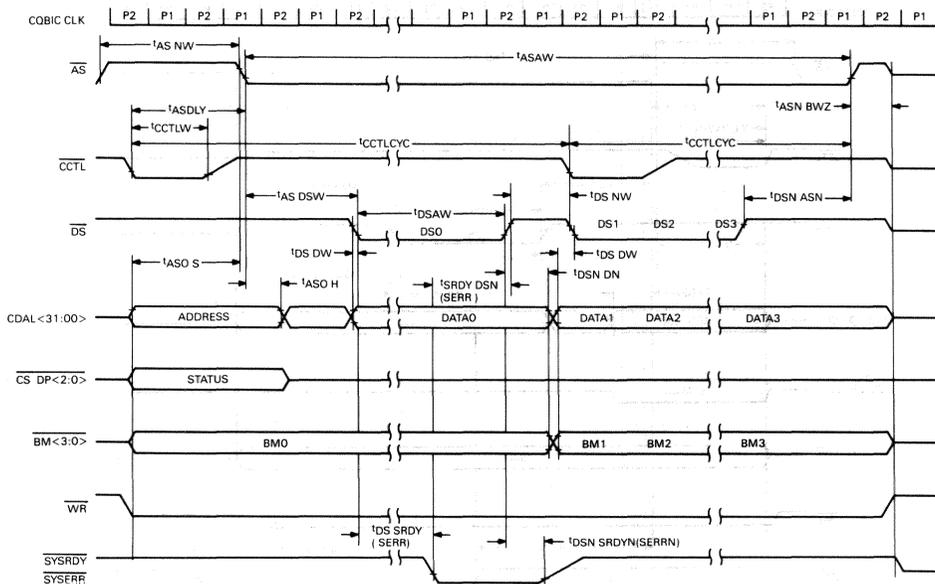
Figure 39 • CVAX 78711 QCBIC to Local Memory Write Timing
