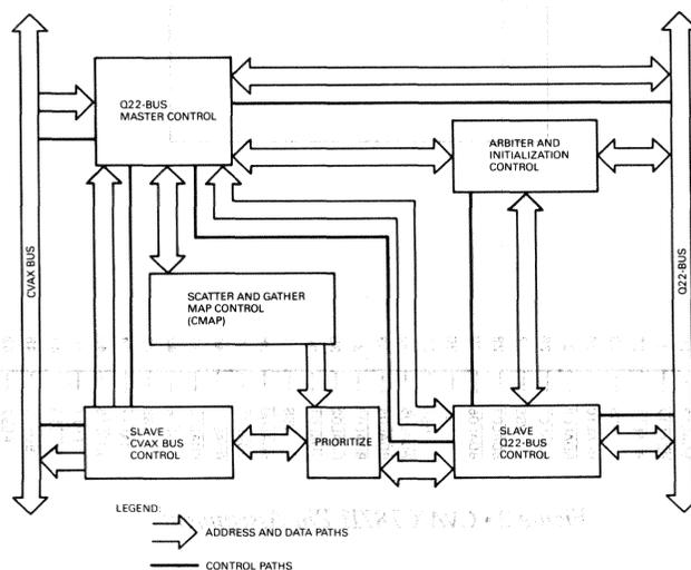
Figure 1 • CVAX 78711 Q22-bus Interface Block Diagram
