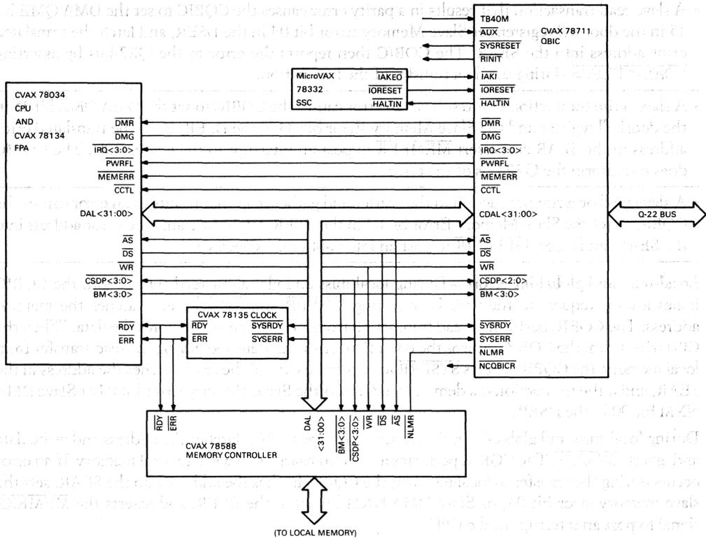
Figure 12 • CVAX 78711 System Interconnect Diagram
