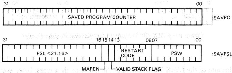
Figure 9 • CVAX 78034 Console Saved Register Formats
