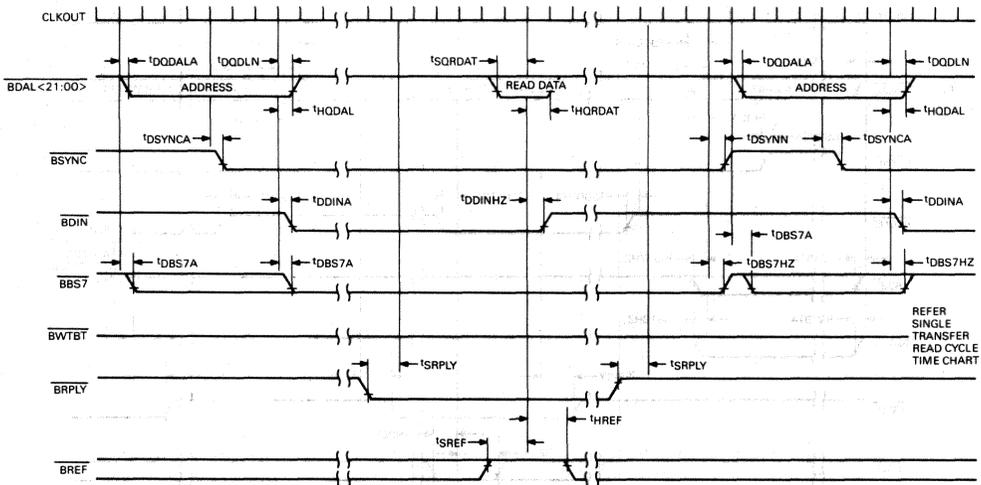
Figure 44 • CVAX 78711 Q22-bus Nonblock-mode Multiple Transfer Read Timing
