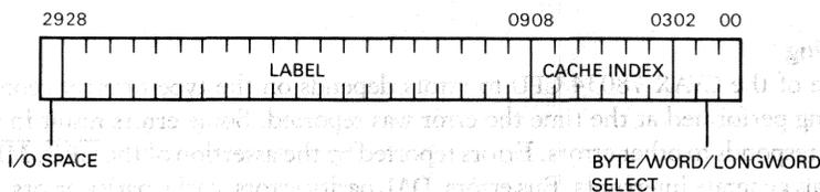
Figure 36 • CVAX 78034 Physical Address for Cache Access
