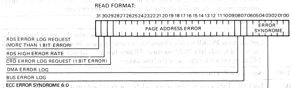
Figure 5 • CVAX 78588 System Error Status Register Read Format
