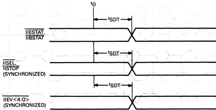
Figure 21 • DC514 Master- and Slave-port Status Signal Timing
