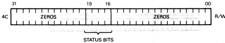
Figure 11 • DC514 Slave-port Status Register Format
