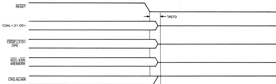
Figure 13 • CVAX 78588 CVAX Bus Reset Timing
