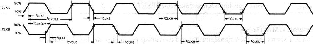
Figure 5 • CVAX 78134 Clock Input Timing
