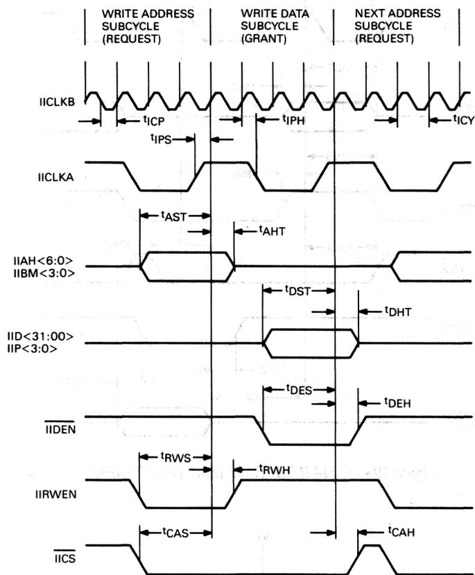
Figure 18 • DC514 II Bus Write Transaction Timing
