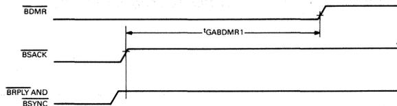
Figure 21 • CVAX 78711 Q22-bus Mastership (Arbiter Mode) Timing
