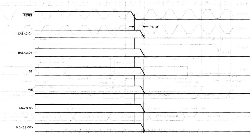
Figure 24 • CVAX 78588 PMI Reset Timing
