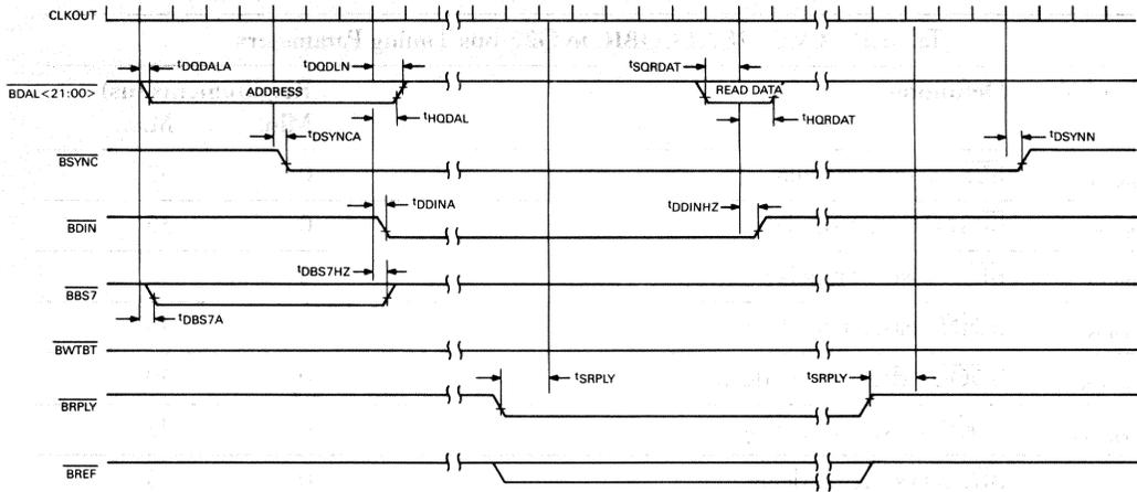
Figure 42 • CVAX 78711 Q22-bus Single Transfer Read Timing
