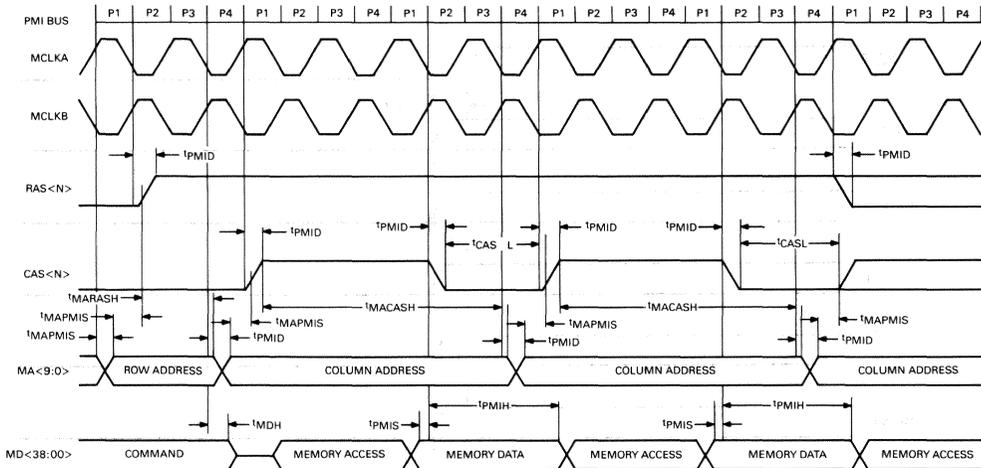
Figure 26 • CVAX 78588 PMI Read Timing (Multiple Transfer)
