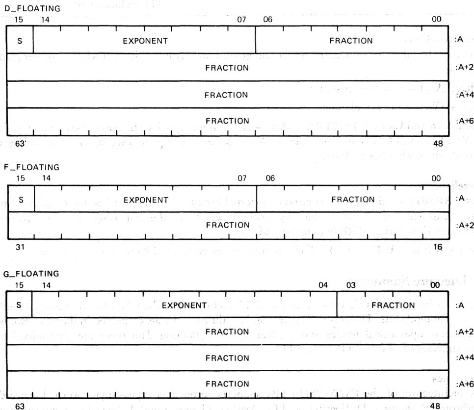
Figure 4 • CVAX 78134 Floating-point Data Types
