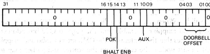
*Figure 6 • CVAX 78711 System Configuration Register Format*
