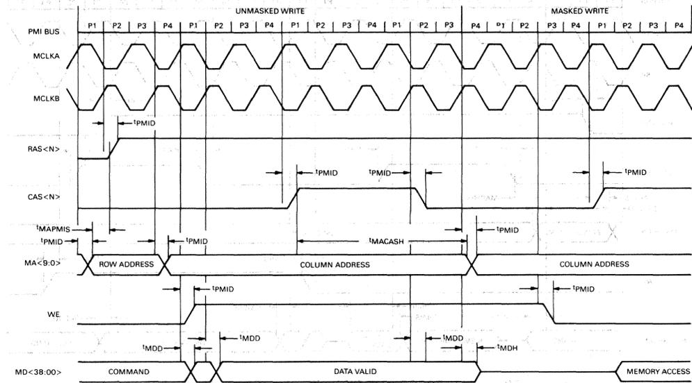
Figure 30 • CVAX 78588 PMI Write Timing (Multiple Unmasked and Masked Transfer)
