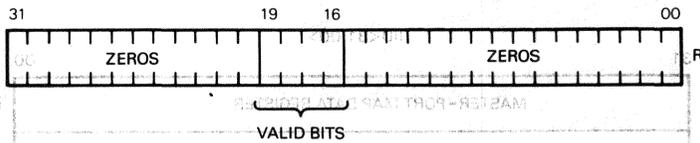
Figure 5 • DC514 Master-port Valid-bit Register Format
