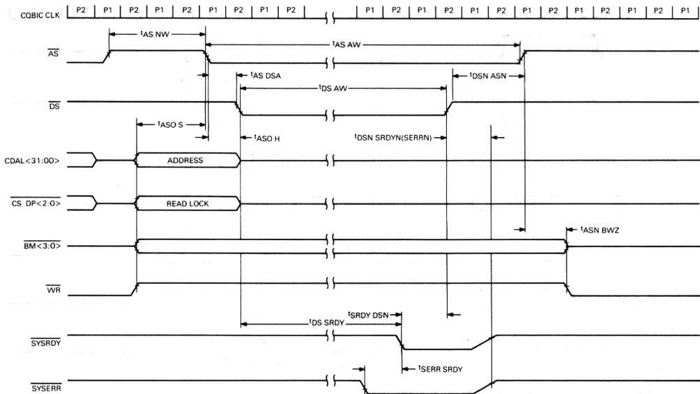
Figure 40 • CVAX 78711 CPU Retry Timing
