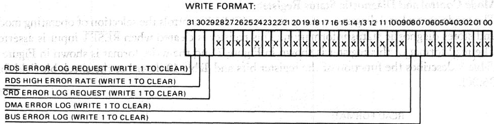
Figure 6 • CVAX 78588 System Error Status Register Write Format
