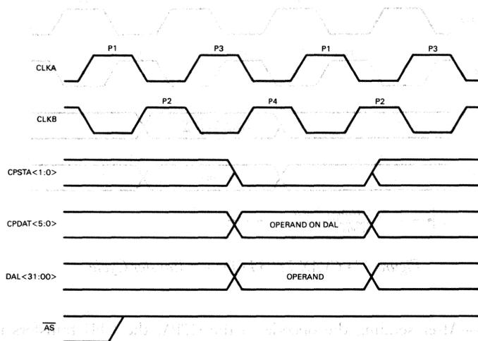
Figure 48 • CVAX 78034 Single-precision CPU to CFPA Transfer
