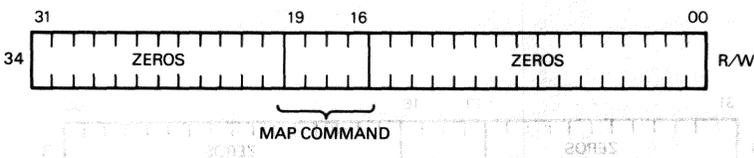
Figure 8 • DC514 Master-port Map Command Register Format
