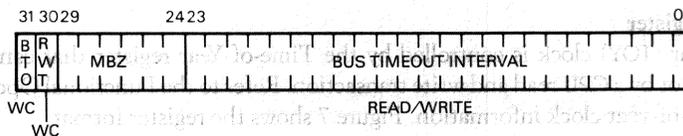
Figure 5 • MicroVAX 78332 Bus Timeout Control Register Format
