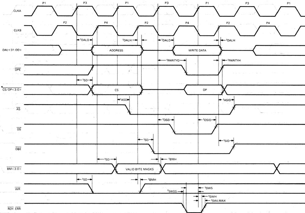
Figure 62 • CVAX 78034 CPU Write Bus Cycle Timing
