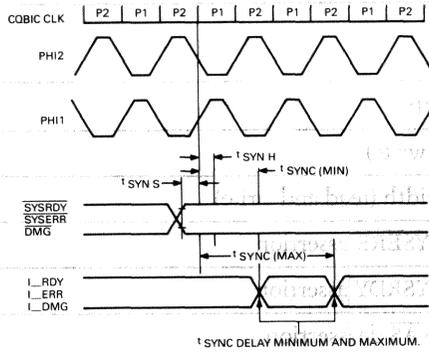
Figure 36 • CVAX 78711 CQBIC Clock to Internal Timing Synchronization
