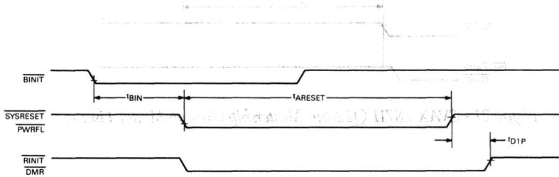
Figure 20 • CVAX 78711 Q22-bus Initialize (Auxiliary Mode) Timing
