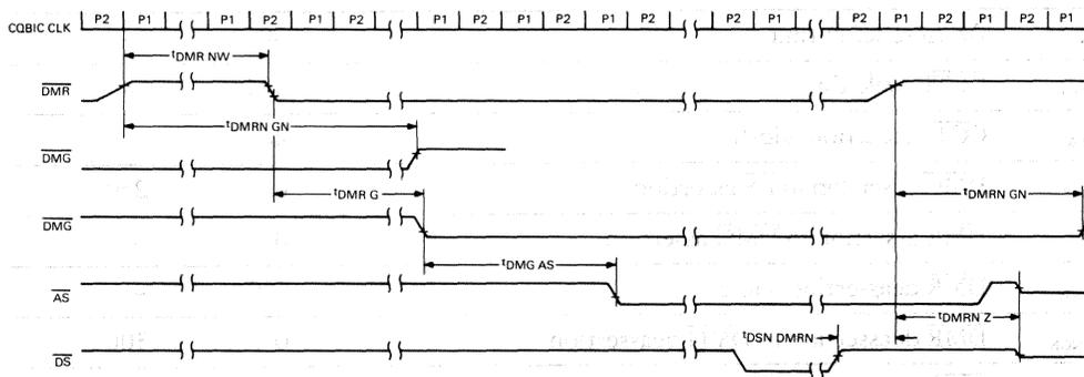
Figure 37 • CVAX 78711 Bus Arbitration Timing
