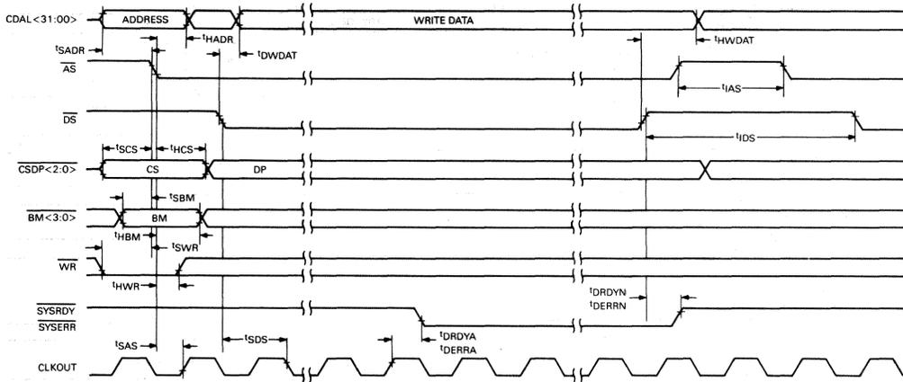
Figure 30 • CVAX 78711 CPU to CQBIC Write Cycle Timing
