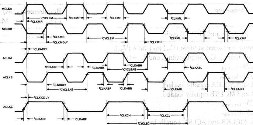
Figure 5 • CVAX 78135 Clock Output Timing
