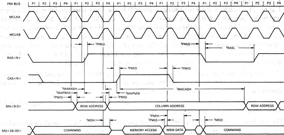
Figure 25 • CVAX 78588 PMI Read Timing (Single Transfer)
