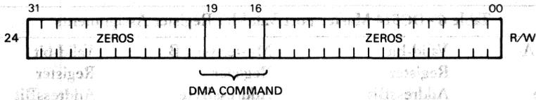
Figure 4 • DC514 Master-port DMA Command Register Format
