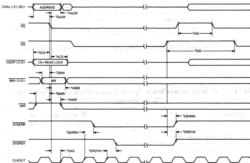
Figure 33 • CVAX 78711 CPU to Local Memory Read Lock Cycle (No Q22-Bus Mastership Retry) Timing
