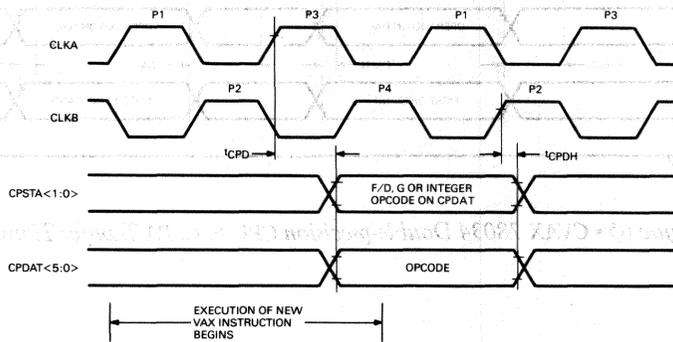
Figure 63 • CVAX 78034 Operand Transfer Cycle Timing
