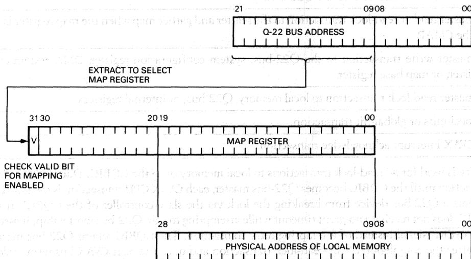
Figure 11 • CVAX 78711 Q22-Bus to Local Memory Address Mapping
