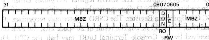
*Figure 8 • MicroVAX 78332 Receiver Control and Status (CSR/RXCS) Registers Format*
