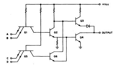
Figure 9 TTL AND/NOR Gate Simplified Schematic
