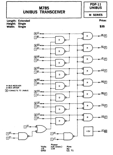
The M785 consists of eight drivers and eight receivers for use as a device interface with the PDP-11 UNIBUS. Pin U1 provides +3 volts and has an output capability of 10 TTL loads. Driver gates have open collectors and are capable of sinking 50 mA with a collector voltage of less than 0.8 volts.
