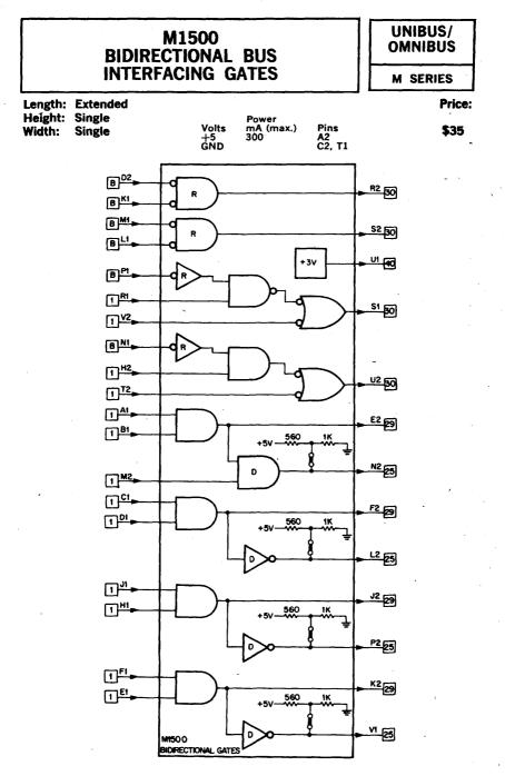
This module provides gating arrangements useful for interfacing to the PDP-8/e, PDP-8/m and PDP-11 computers. It is designed specifically to provide additional gating and output drive when using the M1501-M1502 Input/Output modules. Examples are shown in Figures 1 and 2.
