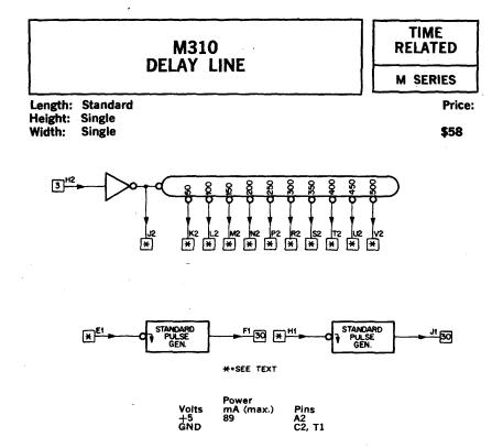
The M310 consists of a tapped delay line with associated circuitry and two pulse amplifiers. The total delay is 500 nanoseconds with taps available at 50 nanosecond intervals.
