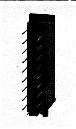
This is a 36 pin single slot connector. It is provided for M-Series modules but can be used with modules or connector boards in the K and W Series. Uses include mounting in confined or irregular spaces. Often the H807 is used to terminate a connector board at a remote location. The H807 is available only with wire wrap pins.
