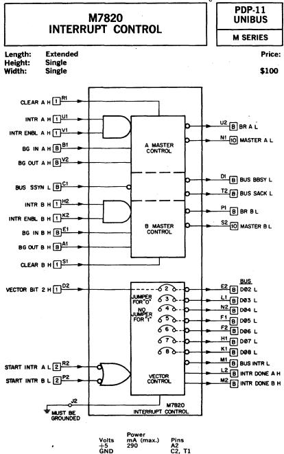
The M7820 is used in PDP-11 device interfaces. It consists of logic circuits that can be divided into three functional sections: Master Control A, Master<sup>></sup> Control B, and INTR Control.
