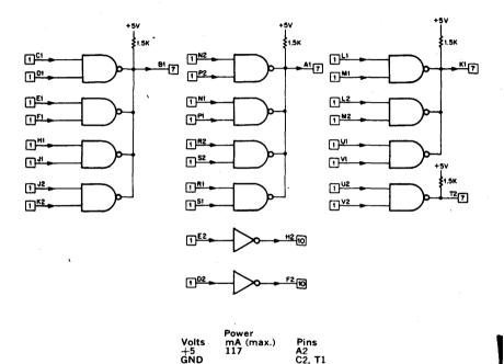
This module provides NAND/OR gates arranged in four groups consisting of 4, 4, 3, and 1 two-input NAND gates respectively. The outputs in each group are connected together to provide a wired OR for low levels. The function of these gates can be shown as:
