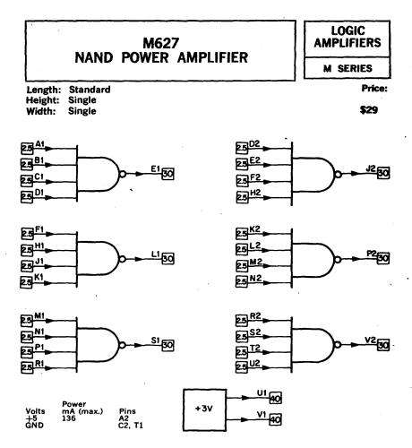
The M627 provides six 4-input NAND gates that combine power amplification with high-speed gating.
