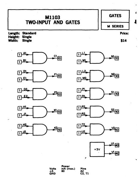
The M1103 contains ten 2-input AND gates. Unused inputs on any gate must be returned to a source of logic HIGH for maximum noise immunity. Two pins are provided (U1 and V1) as a source of +3 volts for this purpose.
