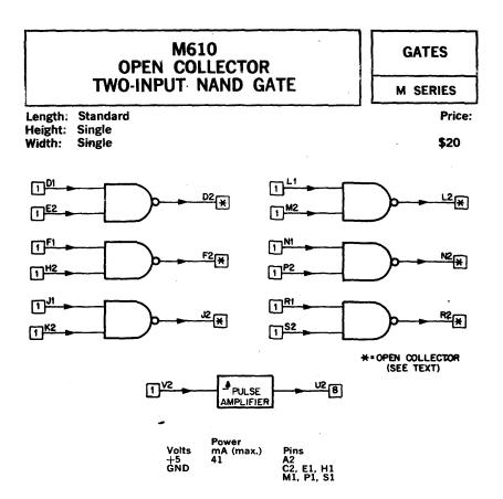
The M610 contains 8 two-input NAND gates with open collector outputs. It also contains a pulse amplifier which does not have an open collector output.
