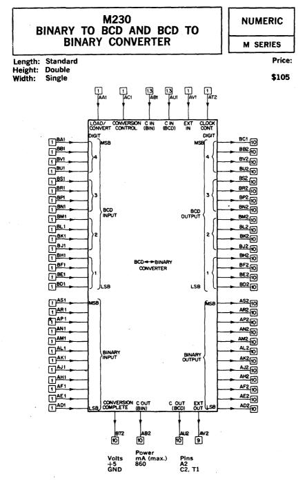
The M230 converts a binary number to its binary coded decimal equivalent or a binary coded decimal number to its binary equivalent.
