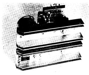
The H710 power supply is ruggedly built, low cost, regulated, floating output, five volt power supply that can be mounted in an H920 chassis drawer or used as a free standing unit. Remote sensing to correct for loss due to long lines is provided. When shipped from the factory, the remote sensing inputs are jumpered to their respective outputs. Especially useful in systems that require maximum repeatability from K303 timers in the millisecond region.
