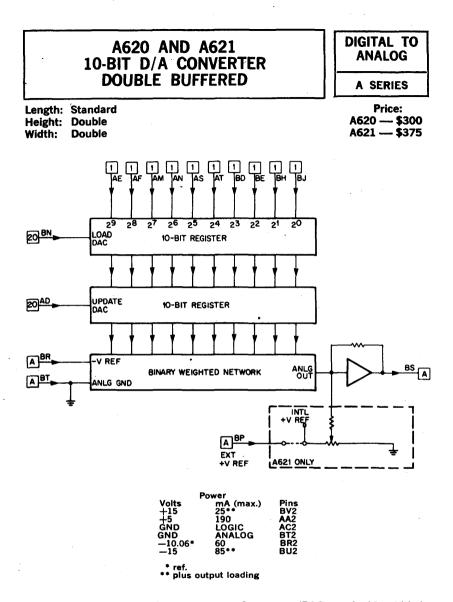
The A620 and the A621 Digital-to-AnalogConverters (DAC) are double-width in the lower (B section) half. The converters are complete with two 10-bit buffer registers, level converters, a precision divider network, and a current summing amplifier, capable of driving external loads up to 10 mA. The reference voltage is externally supplied for greatest efficiency and optimum scale-factor matching in multi-channel-application.
