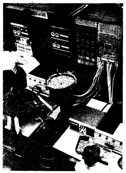
All incoming integrated circuits undergo computer controlled testing, with 40 dc and 16 ac tests performed in 1.1 seconds. This 100% inspection speeds production by minimizing the diagnosis of component failures in module test.
