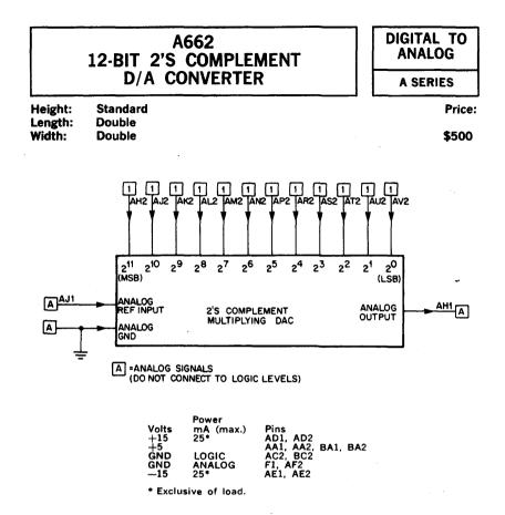
The A662 is a precision 12 bit multiplying digital to analog converter whose output is the product of the external analog reference voltage supplied and digital code presented.
