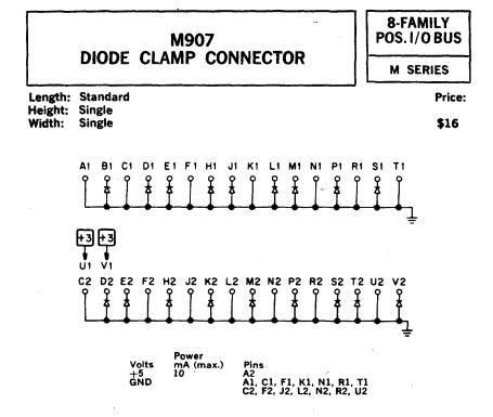
The M907 is used to provide proper undershoot ground clamps for positive I/O bus signals not using M103 or M101 inputs.
