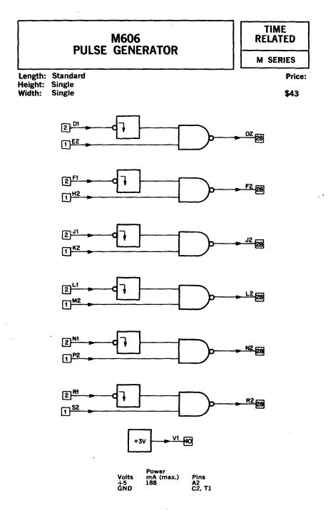
The M606 contains six pulse generators.
