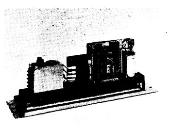
The H726 power supply provides +5 volts at 7 amps with over-voltage protection. A convenience outlet as well as an off switch for the 5 V supply are supplied; both may be operated in parallel. This power supply is built into a systems unit mounted via the two mounting screws in the systems unit. The H014 mounting plate may be used to mount the supply horizontally in a 19" rack.
