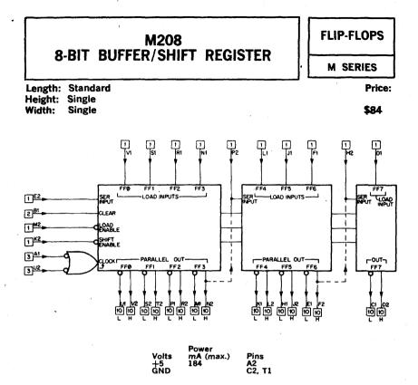
The M208 is an internally connected 8-bit buffer/shift register. Provisions are made for gated single-ended parallel load, bipolar parallel output, and serial input. The shift register is divided into three segments:
