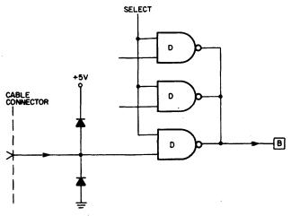
Figure 2. Typical Input Circuit
