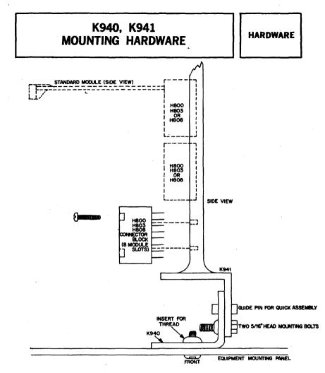
This convenient mounting hardware permits logic connector pin wiring to be done before logic is installed in the enclosure.
