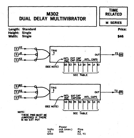
The M302 contains two delays (one-shot multivibrators) which are triggered by a level change from HIGH to LOW or a pulse to LOW whose duration is equal to or greater than 50 ns. When the input is triggered, the output changes from LOW to HIGH for a predetermined length of time and then returns to LOW.
