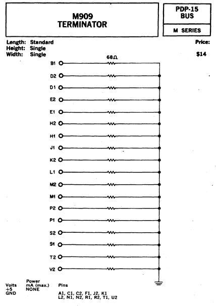
The M909 module contains eighteen 68 ohm resistors tied to ground through a common bus.
