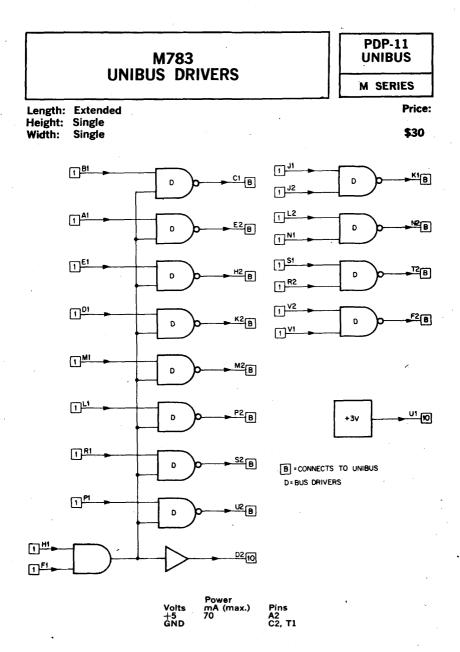
The M783 consists of 12 drivers to be used as an input interface to the UNIBUS of the PDP-11. Pin U1 provides +3 volts as a source of logic HIGH for 10 TTL loads.
