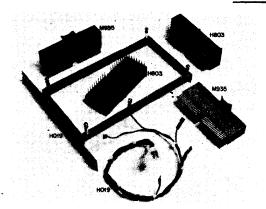
**H019 Mounting Bar**—an aluminum casting with the power bus board and power wiring harness. It also includes four mounting spacers for mounting in an 8/e chassis. Up to ten connector blocks of any type may be accommodated by this frame.
