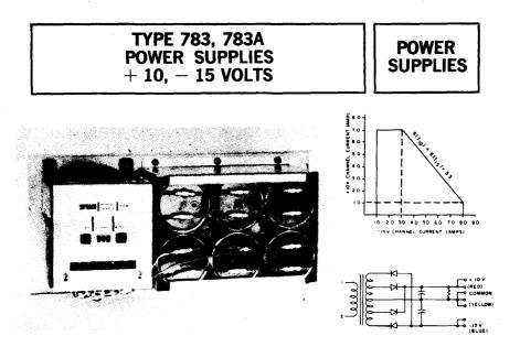
The Type 783 Power Supply (+10, -15 v) is a simple, rugged supply capable of withstanding wide line and load variation for general system use. The graph above shows the permissible region of operation when both outputs are used. When used singly, the 10-v output can supply 0 to 7.5 amp, or the 15-v output can supply 1.0 to 8.5 amp. It is designed for mounting in a standard 19-in. rack. The Type 783A is a 783 Power Supply with a 50-cps transformer.
