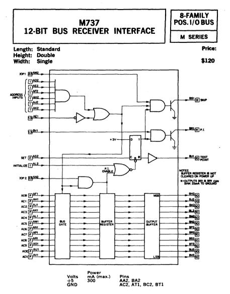
The M737 12-Bit Bus Receiver Interface is completely contained on a double height, single width module.
