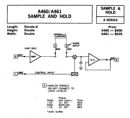
The A460 and A461 are one-channel sample and hold modules used to sample the value of a changing analog signal at a particular point in time and store this information as a stable analog voltage level. The A460 is without input buffering; the A461 includes a unity-gain input buffer amplifier. When the A461 is used an external jumper is required between pins BH2 and AR2.
