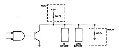
Pull-up resistors of 68 ohms to +5.0 V (supplied on M910) must be tied to the output and the last device should terminate all lines to ground with a 68-ohm resistor (supplied on M909).
