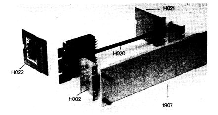
Pairs of brackets. H001 provides  $\frac{3}{4}$ " standoff to mount 1907 over mounting panel wiring. H002 provides a 2" setback so a control panel with switches, lamps, etc. can be mounted flush with mounting rack or cabinet in front of logic wiring.
