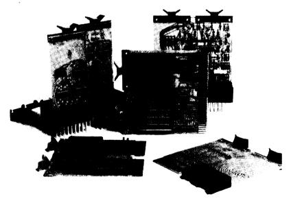
The A Series additions are DTL and TTL compatible and compatible with DEC K and M Series modules, computers, control systems and standard instrumentation.
