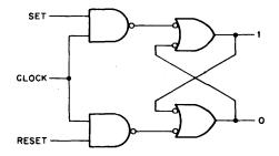
Figure 13 Clocked NAND Gate Flip-Flop
