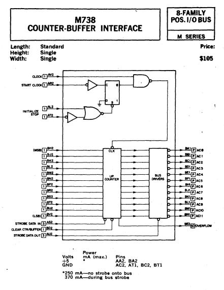
The M738 provides a 12-bit binary up-counter that can be read to the positive external I/O bus of a PDP-8/I or PDP-8/L. The counter can be cleared or preset to a starting value by a jam transfer from an external device. When a count enable flag is set, the counter operates as an up-counter in response to external clock pulses. The content of the counter can be strobed to the I/O bus through data gates under program control.
