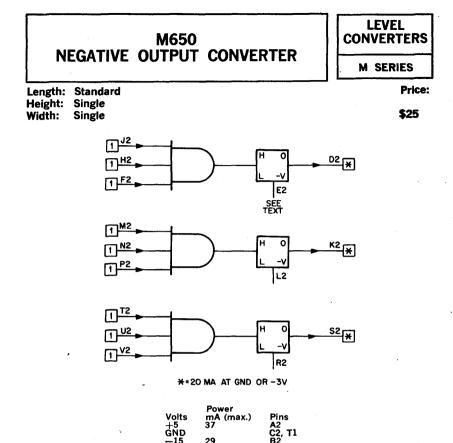
The M650 contains three noninverting signal converters which can be used to interface the positive logic levels or pulses (of duration greater than 100 ns) of K and M Series to digital negative logic levels of -3 volts and ground. These converters provide current drive at a low output impedance so that unterminated cables or wires can be driven with a minimum of ringing and reflections.
