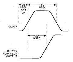
Figure 19. D Type Flip-Flop Timing
