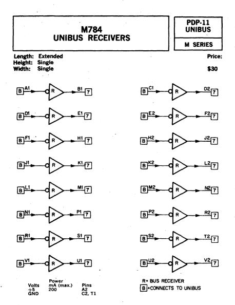
The M784 consists of 16 inverting receivers that are used as an output interface from the UNIBUS of the PDP-11.
