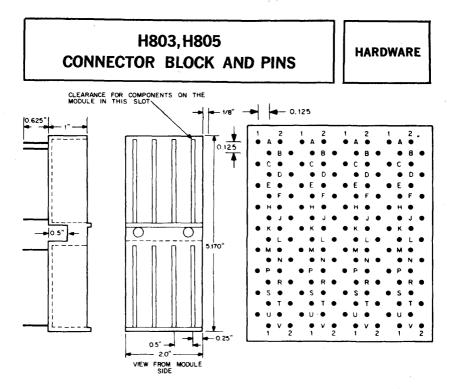
The H803 is the 8-module molded Connector Assembly used in the H911 mounting panels. For each of the eight modules, it provides a 36-pin connector with the wirewrap pins forming a 0.125-inch staggered grid as shown above. This connector is designed to be used with M Series modules; however, it can also be used with all other series listed in this handbook.
