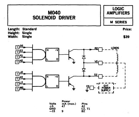
The M040 contains two identical high-voltage driver circuits. Each consists of a 4-input positive NAND gate that controls a PNP transistor switch. The switch is capable of sinking up to 600 ma of current from an external power supply of up to -70 volts. One terminal of the load device (relay, etc.) must be connected to the external voltage, the other to the driver output. The positive terminal of the external supply connects to the module ground.
