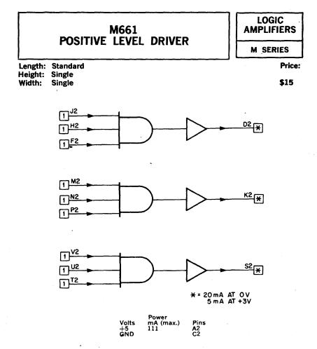
The M661 contains three AND circuits which may be used to drive low impedance unterminated cable with M Series logic levels or pulses of duration greater than 100 ns.
