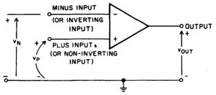
$v_{OUT} = A(v_P - v_N)$ , WHERE A IS THE AMPLIFIER GAIN
