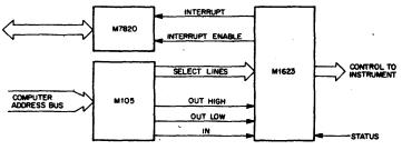
Figure 1. Typical PDP-11 Interface
