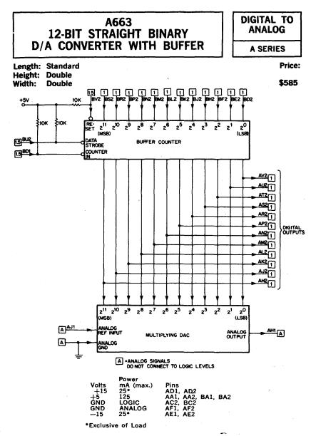
The A663 is a precision 12 bit multiplying digital to analog converter whose output is the product of the external analog reference voltage supplied and digital code presented. A 12 bit Buffer Counter provides input to the D/A Converter and external digital outputs.
