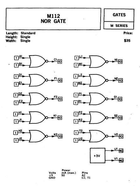
The M112 contains ten positive NOR gates, each performing the function A + B. Pins U1 and V1 provide two separate logic HIGH sources (+3V) each capable of holding up to 40 unused M Series inputs HIGH.
