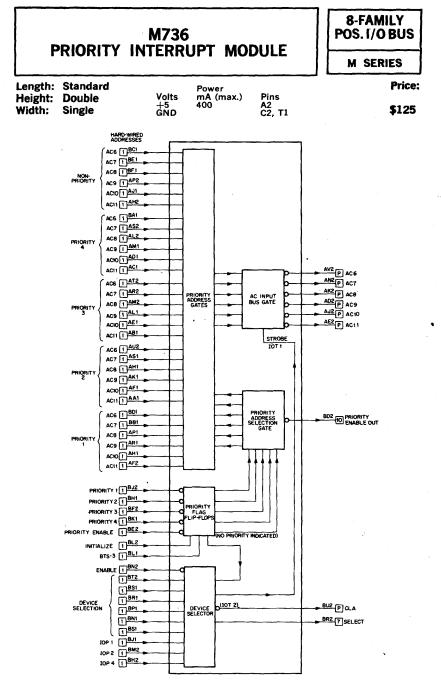
The M736 is used in conjunction with the PDP8/I or 8/L to provide the capability of assigning priorities to various I/O devices connected to the I/O bus of the computer. The M736 can be used to assign priorities for one thru four external devices. Priority assignment may be provided for more than four devices by using additional M736 modules for each additional group of four devices. All M736's in a particular priority system would utilize the same device code.
