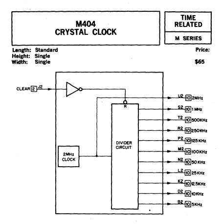
The M404 clock contains a 2 MHz crystal oscillator and frequency dividers.
