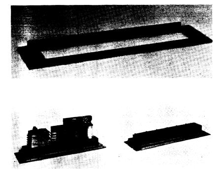
The H014 is a  $5.\frac{1}{4}$ " mounting panel for a standard 19" rack or cabinet. The H014 may be used to mount the H726 power supply or an H933 systems unit casting. When the H933 systems unit casting is mounted on an H014, the back plane pins are available behind the H950-P bezel cover panels.
