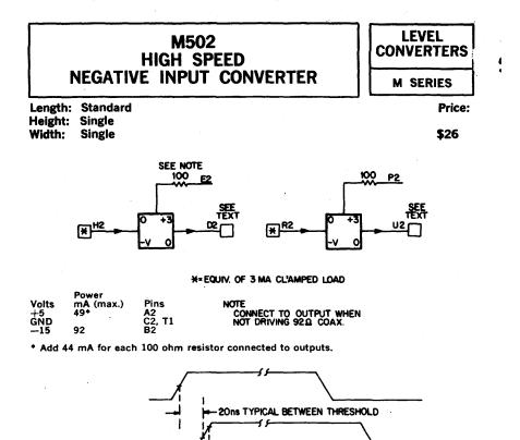
The M502 contains two non-inverting high-speed signal converters which interface standard negative (-3 volts and ground) logic levels or pulses with M and K Series positive logic modules. These converters provide sufficient current drive at a low output impedance for system interconnections by means of terminated 92-ohm coaxial cable.
