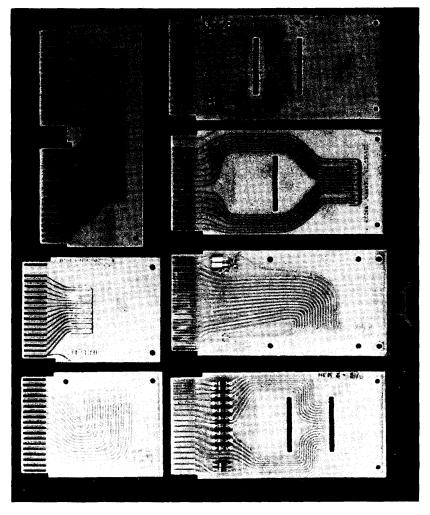
TYPICAL MYLAR FLEXPRINT CABLE CONNECTORS
