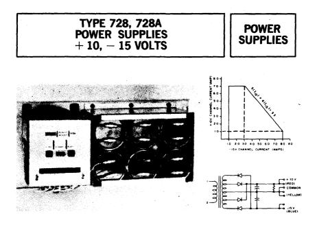
The Types 728 and 728A (+10, -15 v) Power Supplies are capable of withstanding wide line and load variations for general system use. When used singly, the 10-v channel can supply 0 to 7.5 amp, or the 15-v channel can supply 1.0 to 8.5 amp. The 728 Power Supply is electrically identical to the 783 but is made on a shorter chassis specifically designed for mounting on the plenum door of a DEC computer cabinet.
