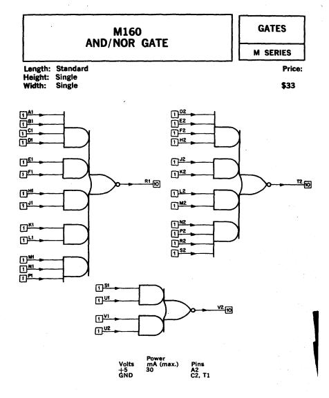
The M160 module contains three general-purpose AND/NOR gates which perform functions similar to those of the M121.
