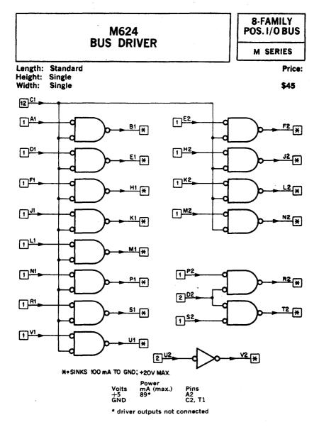
The M624 contains 15 bus drivers intended for convenient driving of the positive input bus of either the PDP-8/I or PDP-8/L. Twelve of the drivers have a common gate line for selecting data. There are three additional drivers, two sharing a common gate line and the third without a gate line. These three additional drivers were intended to accommodate the functions of PROGRAM INTERRUPT, IO SKIP and CLEAR AC.
