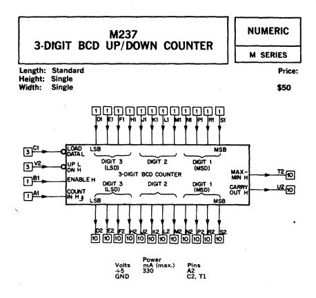
The M237 is a 3-digit synchronous BCD up/down counter. It has a single control input that can switch the counting mode from up to down without disturbing the contents of the counter. The M237 is fully cascadable and programmable. Cascading simply involves paralleling the respective ENABLE, LOAD DATA, and UP/DOWN signals while one MAX/MIN signal drives the ENABLE input of the next M237.
