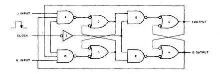
Figure 15. Master-Slave J-K Flip-Flop
