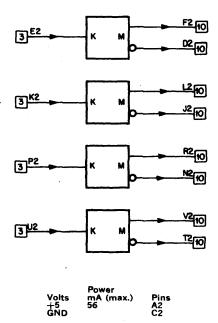
The M521 K Series to M Series Converter contains four circuits which can convert any K Series input to complementing M Series outputs.
