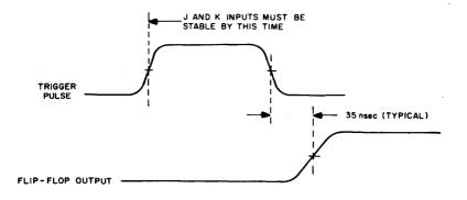
Figure 20. J-K Flip-Flop Timing
