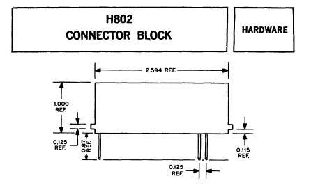
This is an 18 pin connector block for a single FLIP CHIP® module. It can be used to mount all modules except those with pins on both sides of the board. Pin dimensions are .031 inches by .062 inches and may be of the wire wrap type only. Number 24 wire should be used with this connector.
