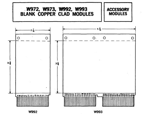
Type W992 and W993 are single side copper clad boards. The diagrams above indicate the copper clad area that is usable for etching purposes. The identifying numbers are etched from the clad using a minimum of etchable area. Type W972 and W973 are equivalent to the above types but have copper clad on both sides.
