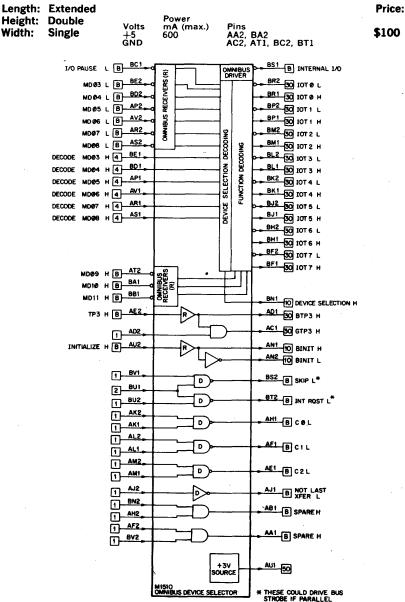
The M1510 Bus Device Selector is designed for use with the PDP-8/e and PDP-8/m computers. It provides a convenient and efficient method of decoding the device code for an interface system. The M1510 decodes the six device selection bits to produce a device selection level. It also decodes the three function selection bits to produce a one-of-eight function level output.
