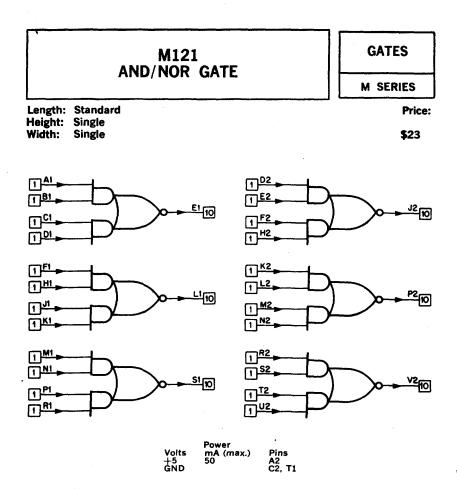
The M121 module contains six AND/NOR gates which perform the function (AB + CD). By proper connection of signals to the AND inputs, the exclusive OR, coincidence, and NOR functions can be performed.
