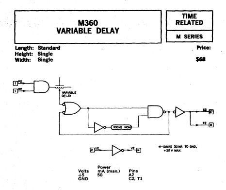
The M360 contains an adjustable delay line with a standardizing amplifier. The delay is adjustable between the limits of 50 ns to 300 ns by means of a slotted screw which is accessible from the handle end of the module.
