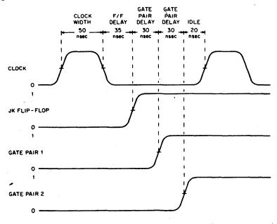
Figure 22. Delays Determining System Operating Frequency
