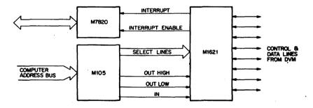
Figure 1. Typical PDP-11 Interface
