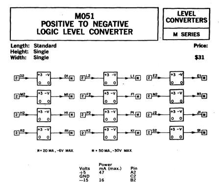
The M051 contains twelve level converters that can be used to shift M and K Series logic levels to negative logic levels of ground and -3 volts.
