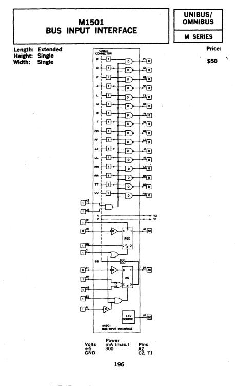
The M1501 contains 16 bus drivers for interfacing parallel input data to a bidirectional data bus structure such as the PDP-11 UNIBUS or the PDP-8/e OMNIBUS. The module includes two control flags that can be used for interrupt request and enable. Data inputs from an external device enter a 40-pin flat cable connector mounted on the module itself. All inputs are diodeclamped to ground and +5 volts.
