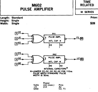
The M602 contains two pulse amplifiers which provide power amplification, standardize pulses in amplitude and width, and transform level changes into a standard pulse.
