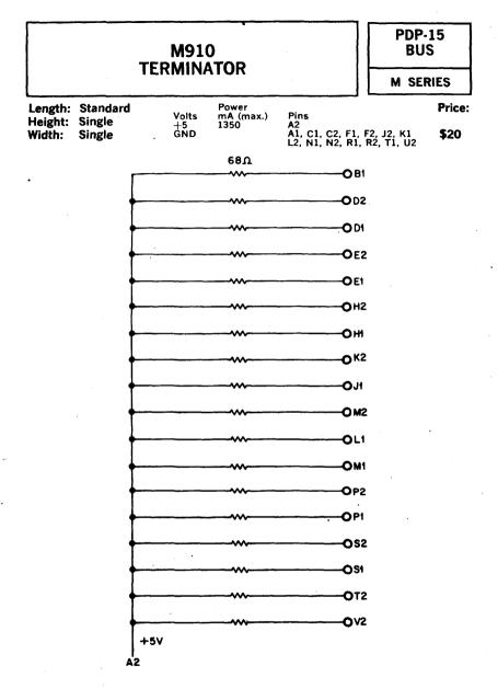
The M910 module contains eighteen 68-ohm resistors tied to a common  $\pm 5$  volt bus.
