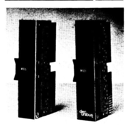
**UNIBUS Jumper Module M920**—The M920 Module is a double module that connects the UNIBUS from one system unit to the next. The printed circuit cards are on one-inch centers. A single M920 Module carries all 56 UNIBUS signals and 14 grounds.
