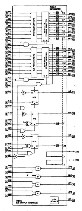
**Spare Lines:** Two additional lines are provided between the cable connector and the module for additional communication between the module and the external device. These lines are diode protected against voltage over shoot below -0.75 volts or above +5.75 volts.
