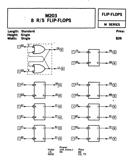
The M203 is made up of 8 R/S-type flip-flops. Each flip-flop is made up of two 2-input NAND gates with cross-coupled outputs.
