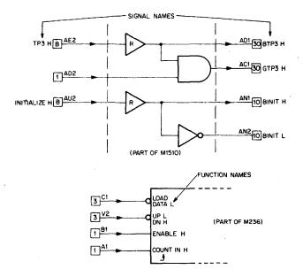
Figure 5. Signal and Function Names
