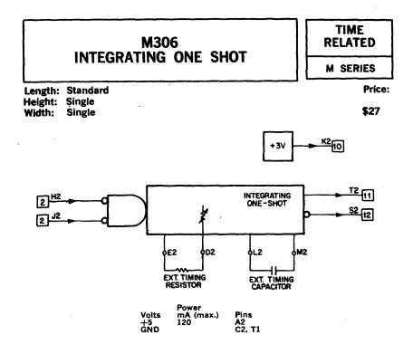
The M306 is a zero-recovery-time integrating monostable multivibrator with complementary outputs. The M306 has the ability to respond to an input even while in the active state, so that successive inputs above a preset frequency can postpone the return to the inactive state indefinitely.
