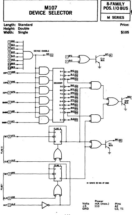
The M107 is a device selector which, by the use of extended decoding of the BMB lines 9 through 11, will provide seven discrete IOT pulses. Five additional IOT pulse outputs are provided to allow the user to reduce software requirements by the combining of IOT codes. The IOT instruction and the IOP times at which the various IOT pulses occur at the module pins are outlined in the following chart:
