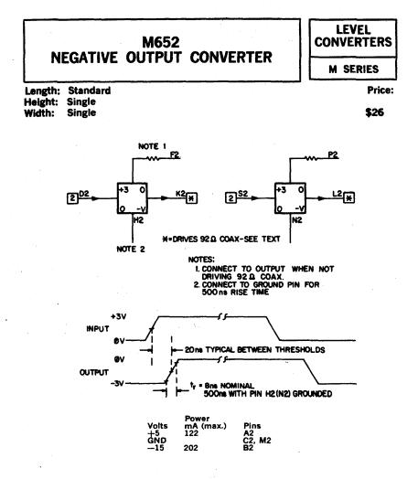
The M652 contains two noninverting high-speed signal converters which can be used to interface the positive logic levels or pulses of the K and M Series to digital negative logic levels of -3 volts and ground. These converters provide current drive at a low output impedance so that system interconnections can be made using terminated 92-ohm coaxial cable.
