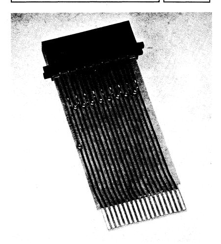
The W980 Module Extender allows access to the module circuits without breaking connections between the module and mounting panel wiring.
