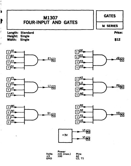
The M1307 contains six 4-input AND gates. Unused inputs on any gate must be returned to a source of logic HIGH for maximum noise immunity. Two pins are provided (U1 and V1) as a source of +3 volts for this purpose.
