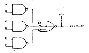
By using one of the two inverters provided, a true AND/OR function can be realized. A maximum of four groups of gates can be connected together. Connection is made by merely connecting output pins together.
