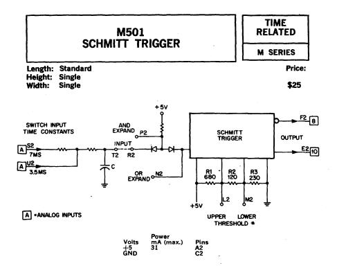
The M501 is a Schmitt Trigger with variable thresholds and complementary positive logic outputs.
