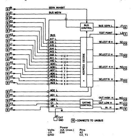
The M105 is used in PDP-11 device interfaces to control the flow of data between the device registers and the UNIBUS. It provides gating signals for up to four device registers that indicate a register is being referenced and three control signals that indicate the path for data flow.
