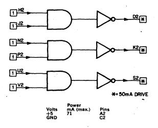
The M660 Cable Driver consists of three NAND gate circuits each of which will drive a 100-ohm terminated cable with M Series levels or pulses of duration greater than 100 ns.
