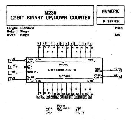
The M236 is a 12-bit synchronous binary up/down counter. It has a single control input that can switch the counting mode from up to down without disturbing the contents of the counter. The M236 is fully cascadable and programmable. Cascading simply involves paralleling the respective ENABLE, LOAD DATA, and UP/DOWN signals while one CARRY-OUT signal drives the COUNT IN input of the next M236.
