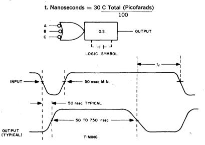
Figure 21. One-Shot Delay Timing and Logic Symbol
