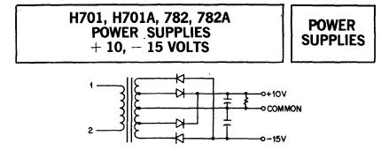
The 782 and 782A power supplies are ruggedly built, low cost units that fit into a standard 19-inch rack. The H701 and H701A are identical to these units, except they can be mounted on a chassis or panel in applications where space is added to an existing device. The basic supply can be mounted in various configurations and is identical to the power supplies used in models 700D and H900. The Types 782A and H701A are Power Supplies with 50 Hertz transformers. The Types 782 and 701 are 60 Hertz.
