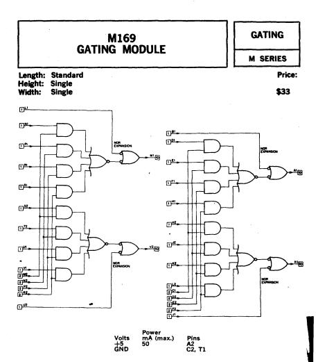
The M169 contains groups of 4-input AND/NOR gates prewired as four stages of a 4-input, 1-output multiplexer or similar gating function.
