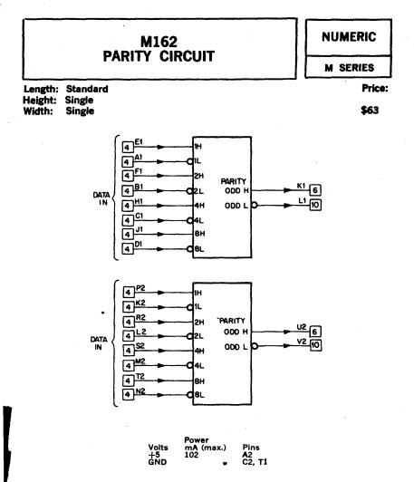
The M162 contains two parity detector circuits. Each circuit indicates whether the binary data presented to it contains an ODD or EVEN number of ONES. The data and its complement are required as shown.
