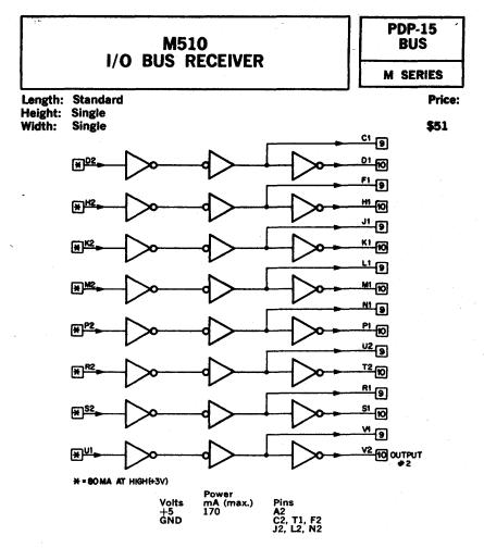
The M510 is a positive input/output receiver card for use with the PDP-15. It contains 8 high-impedance input circuits of at least 27K ohms and input switching thresholds of about +1.5 V. Each receiver has two outputs, one of the same polarity as the input, the other, the complement of the input. The receiver card can be used anywhere on the PDP-15 I/O Bus.
