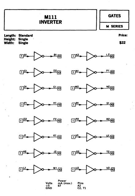
Sixteen Inverters with input/output connections as shown.
