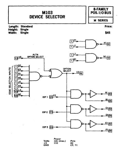
The M103 is used to decode the six device bits transmitted in complement pairs on the positive bus of the PDP8/I and PDP8/L. Selection codes are obtained by selective wiring of the bus signals to the code select inputs D2, E2, F2, H2, J2, and K2. This module also includes pulse buffering gates for the IOP signals found on the positive bus of the above computers. Two two-input NAND gates are also provided for any additional buffering that is required.
