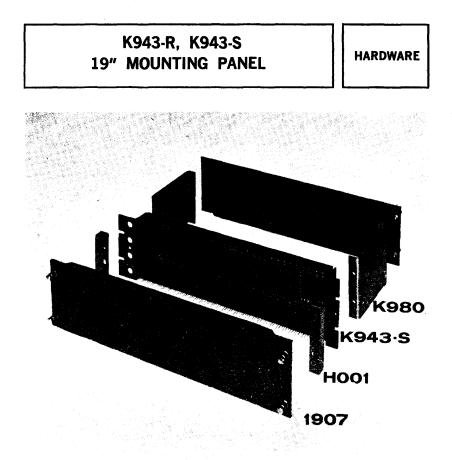
These low cost, 19" panels have sixty-four 18 pin connector sockets with either wire wrap (S) or solder fork (R) contact pins. Shipped with connector blocks installed and pins A and C bussed.
