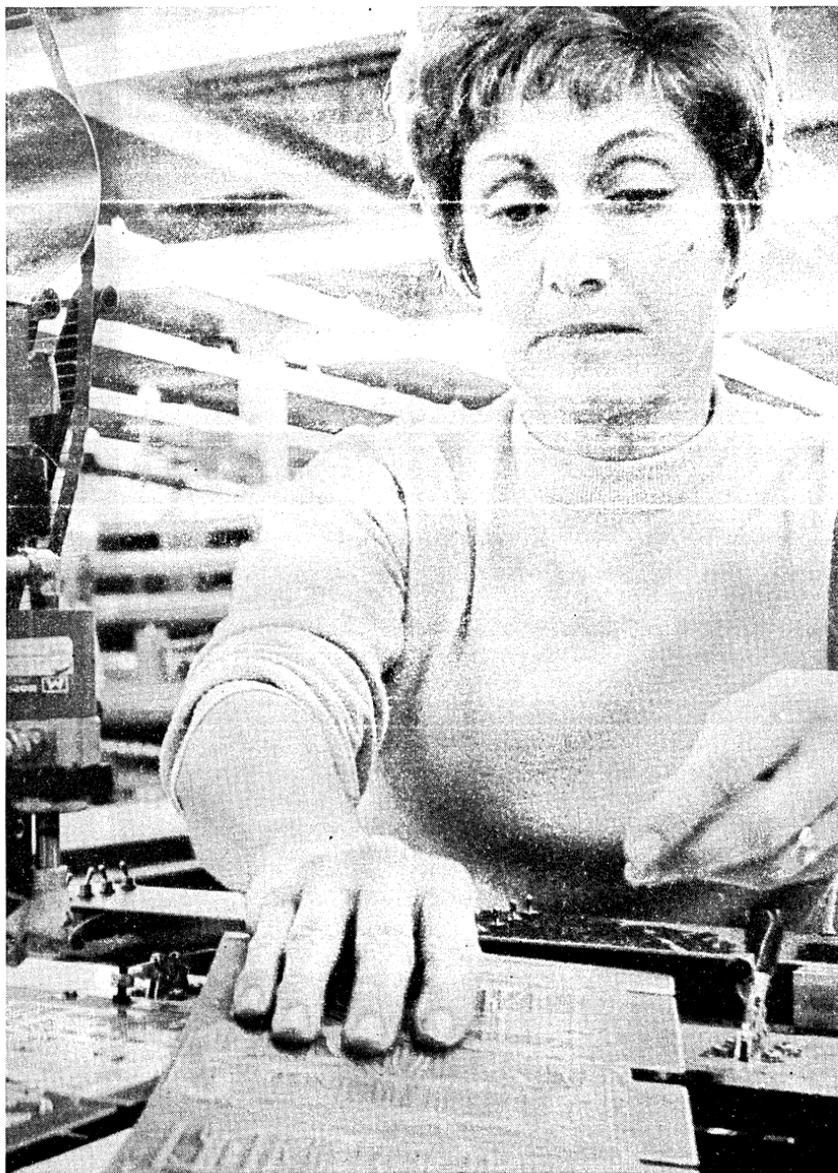
Discrete components for DIGITAL Modules are positioned and crimped in place at rates up to 2,200 per hour on pantograph controlled inserting machines. Board layouts are placed in rows, minimizing the effort required to follow the template. Several templates for each module type are generated by numerically controlled milling machines.
