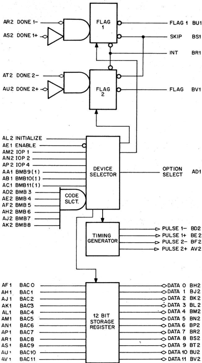
Figure 2. M731 8/I BUS-NEGATIVE OUTPUT INTERFACE
