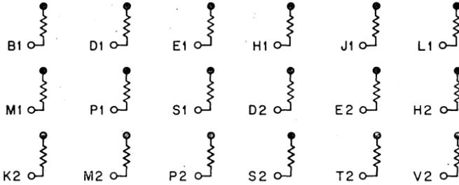
The M906 cable terminator module contains 18 load resistors which are clamped to prevent excursions beyond +3V and ground. It may be used in conjunction with M623 to provide cable driving ability similar to M661 using fewer module slots.
