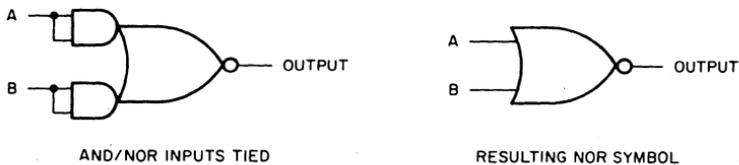
Figure 11 NOR Connection of AND/NOR Gate
