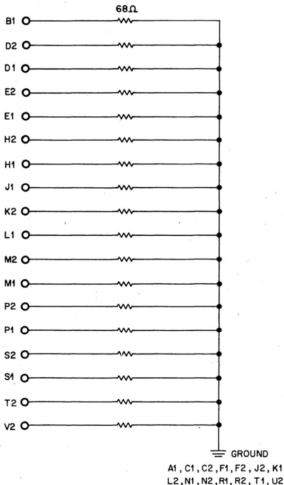
The M909 module contains 18  $68\Omega$  resistors. All 18 resistors are tied to ground through a common bus.
