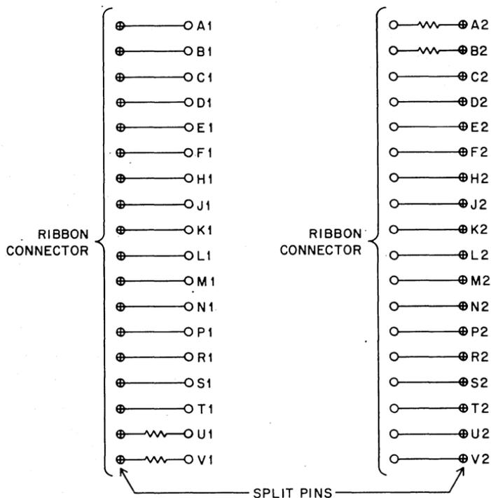
The M908 cable connector consists of a single sized, double sided board which contains thirty-six split pins which allows the connection of thirty-six separate wires. All connections are made on the component side of the module. The 10 ohm,  $\frac{1}{4}$  watt resistors connected in series with module pins A2, B2, U1 and V1 are provided to afford some measure of protection in the event that these pins are inadvertently connected to a source of supply voltage.
