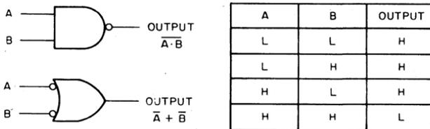
Figure 8 NAND Gate Logic Symbol and Truth Table
