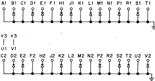
The M907 is used to provide proper undershoot ground clamps for PDP8/I positive bus signals not using M103 or M101 inputs.
