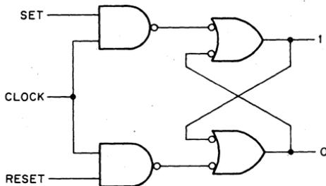
Figure 13 Clocked NAND Gate Flip-Flop
