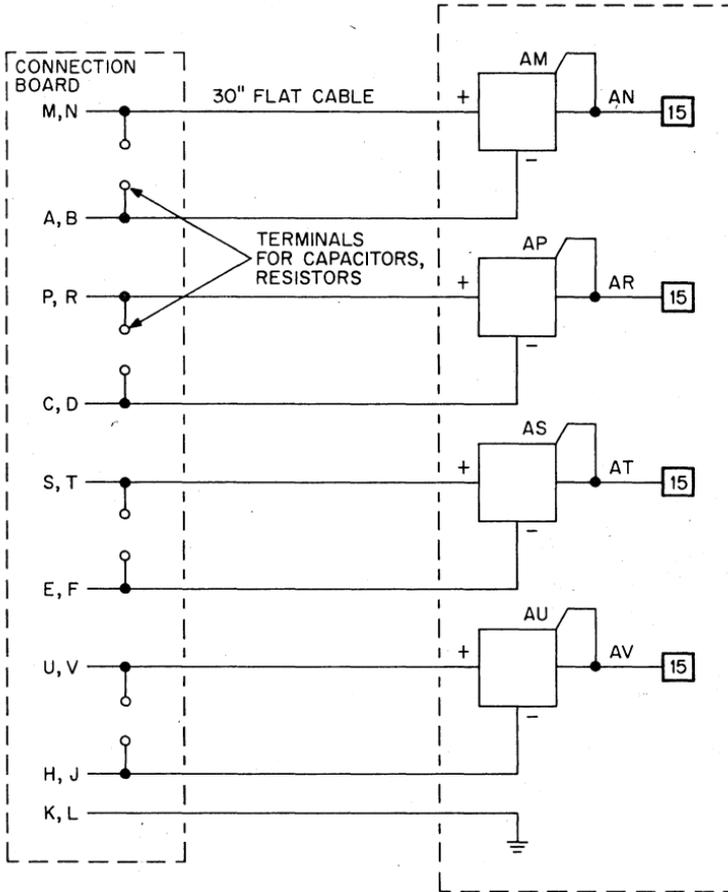
Basically a noise-rejecting, threshold sensing differential voltage amplifier, the K524 is readily adapted to sensing threshold points in DC analog signals, AC signals, and pulses. It can also be biased to sense resistance thresholds. The differential amplifying technique permits flexible grounding and shielding methods to accommodate floating signal generators and minimize noise.
