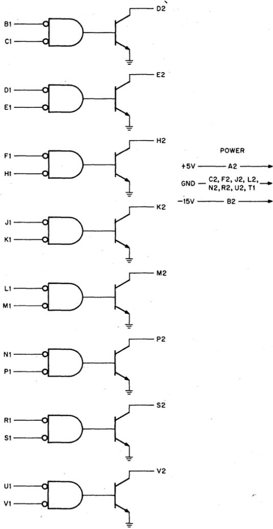
The M622 contains eight two input AND gate bus drivers for convenient driving of the positive input bus of the PDP-15. The output consists of an open collector NPN transistor.
