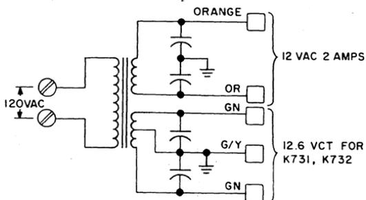
These hash-filtered, 50/60 Hz transformers supply K731 Source and K732 Slave Regulator modules. The K743 also provides an auxiliary winding for use with K580 Dry Contact Filters, K681 or K683 Lamp Drivers (requires additional bridge rectifier, and the K730 Supply and Control Module. Type 914 Power Jumpers are convenient for connecting to tab terminals on these transformers and on the K732 and K943. Both transformers have holes at the corners of the chassis plate for mounting on K980 endplates:
