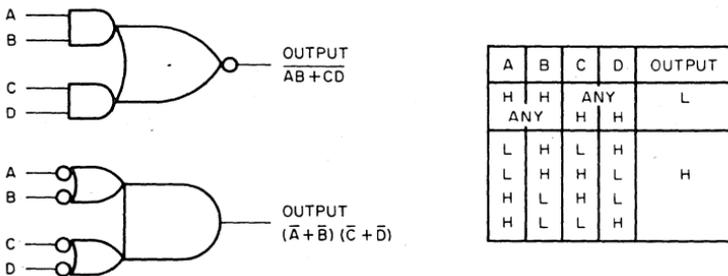
Figure 10 AND/NOR Gate Logic Symbols and Truth Table
