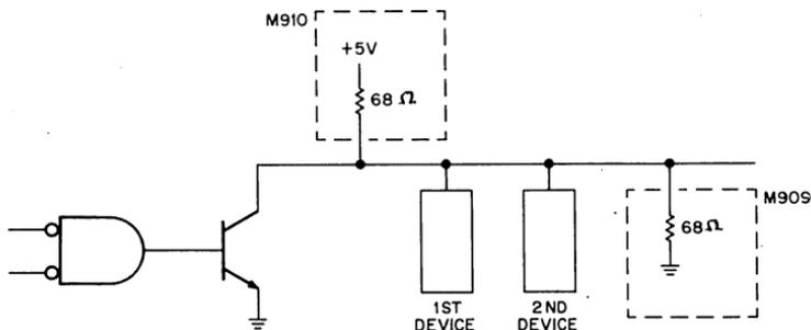
Pull up resistors of  $68\Omega$  to +5.0 volts (supplied on M910) must be tied to the output and the last device should terminate all lines to ground with a  $68\Omega$  resistor (supplied on M909).
