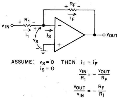
Fig. 2, Inverting Amplifier
