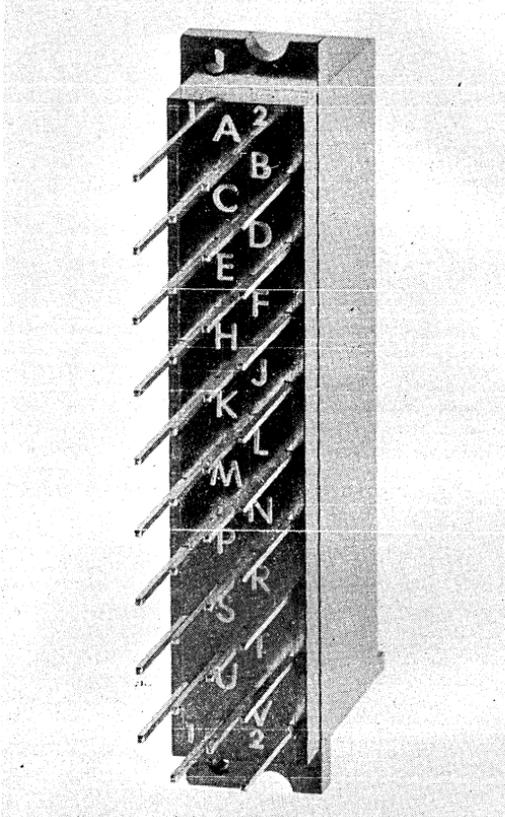
This is a 36 pin single slot connector. It is provided for M-Series modules but can be used with modules or connector boards in the K and W Series. Uses include mounting in confined or irregular spaces. Often the H807 is used to terminate a connector board at a remote location. The H807 is available only with wire wrap pins. Number 30 wire should be used with this connector.
