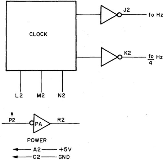
The M410 is a free-running contactless-resonant-reed-tuned clock which provides stable timing signals for a system using the M706 and M707 teletype converter modules. Overall frequency stability of the outputs is better than .1% in the temperature range 0°C-70°C. Available clock frequencies are listed below. A pulse amplifier is provided for the generation of nominal 150 nsec pulses.
