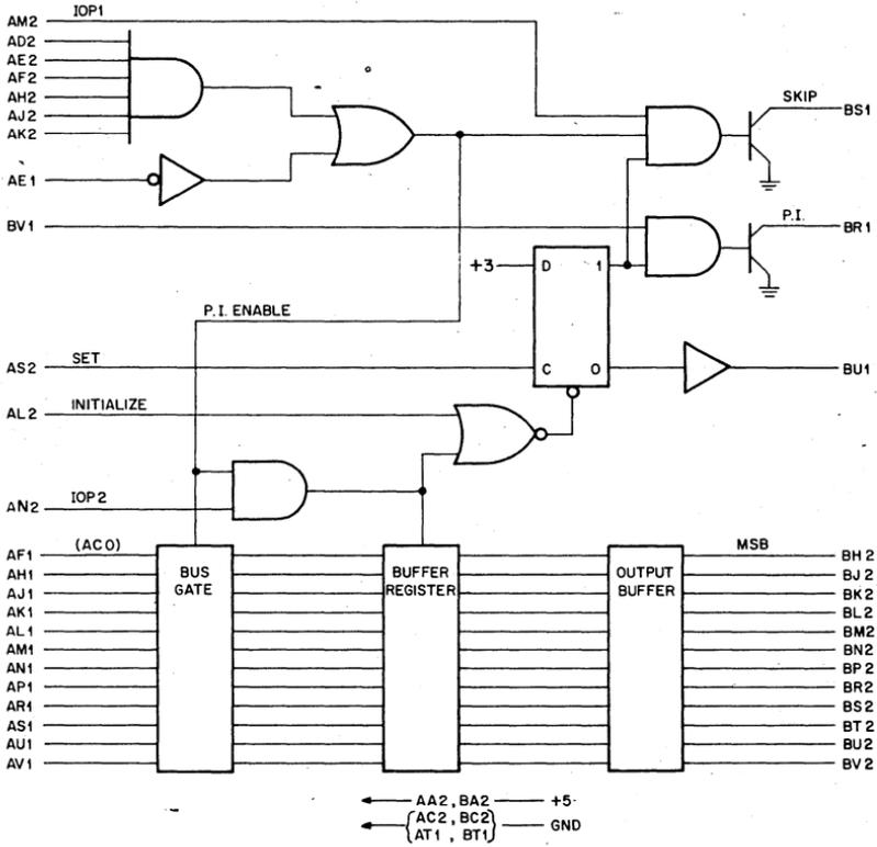
The M737 12-Bit Bus Receiver Interface is completely contained on a double height, single width module.
