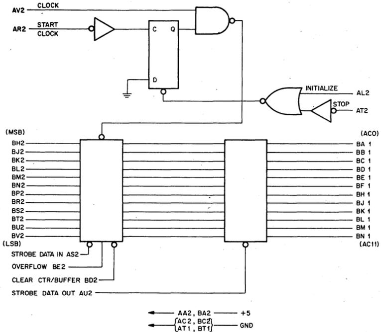
The M738 Counter-Buffer Interface is contained on a double height, single width module.
