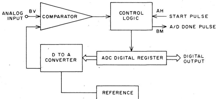
A811 10-BIT ANALOG-TO-DIGITAL CONVERTER
