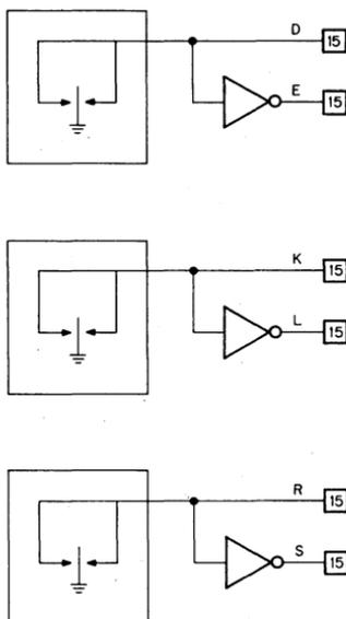
The K420 uses three 3-position Toggle switches. Only when the Toggle is in the center position will pins D, K, and R be high. The switch acts like a SPST Toggle in one direction and a spring returned push button in the other direction. Built in switch filters and Schmitt Triggers remove all switch contact bounce. Both inverted and uninverted outputs for each switch can drive 15 unit loads. Outputs are unslowed and may be used to drive M Series inputs directly.
