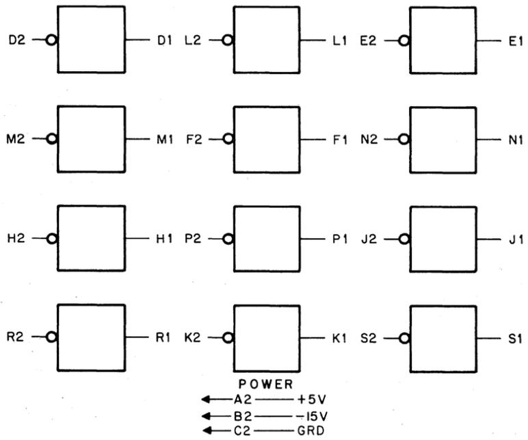
The M051 contains twelve level converters that can be used to shift M and K Series logic levels to negative logic levels of ground and -3 volts. A grounded input on the driver generates a grounded output.
