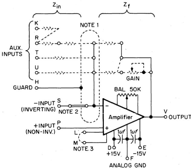
NOTE 1. Mounting holes are provided on the module so that input and feedback components can be added. Components shown with dashed lines are not included with the module.
