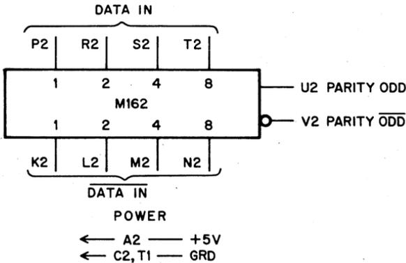
The M162 is a parity detector and contains two Parity Circuits. Each circuit indicates whether the Binary Data presented to it contains an ODD or EVEN number of ONES. The DATA and its complement are required as shown.
