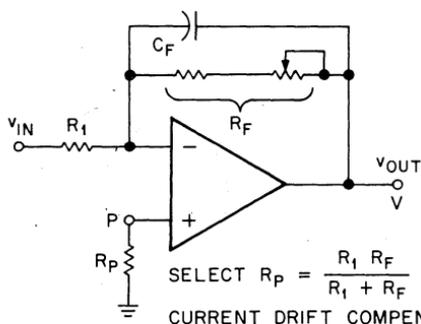
$$\frac{v_{OUT}}{v_{IN}} = -\frac{R_F}{R_1}$$
