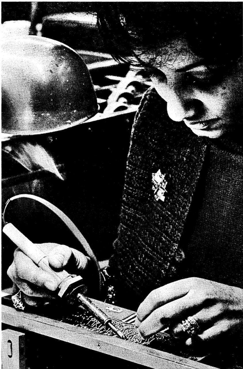
After the modules are flow-soldered, they undergo a visual inspection to insure that all solder points and runs are properly made. If needed, additional solder is added.
