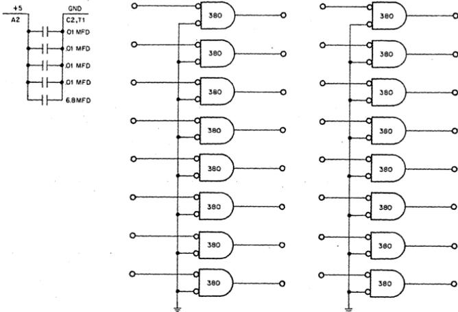
Figure 4 M784 Unibus Receivers\*
