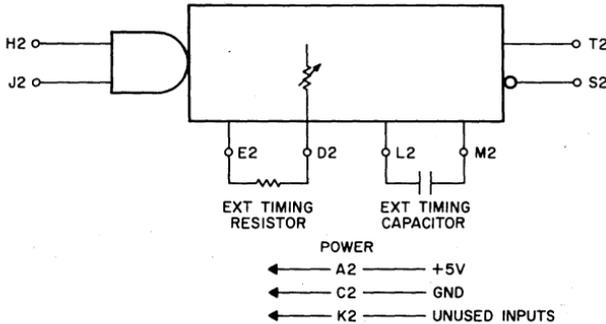
The M306 contains one integrating monostable multivibrator mounted on a single fiip-chip™ module.
