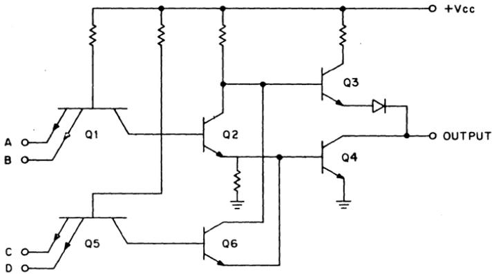
Figure 9 TTL AND/NOR Gate Simplified Schematic
