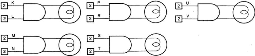
The K410 indicator lamp module provides a convenient way to build binary, decimal, octal, or bi-quinary displays. Lamps and lamp drivers receive their supply voltage through fast-on tab connectors. Any 12.6 V c. t. transformer may be used as a voltage supply provided the center tap is grounded.
