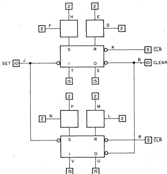
This superslow memory simplifies sequencing of machine motions, and finds other applications where the ultimate in noise isolation is needed and speed is no problem. Its 1 KHz maximum repetition rate makes this flip-flop noticeably more resistant to extremely noisy surroundings than faster types like K202, K210, etc. So noise immune, in fact, that several yards of wire may be connected to K201 outputs even in severely noisy areas without errors.
