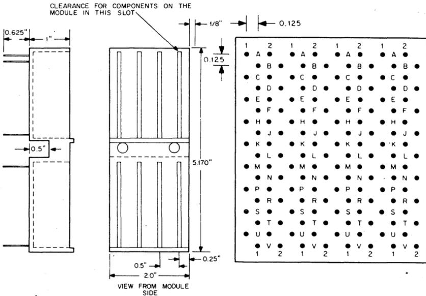
The H803 is the 8-module molded Jacket Assembly used in the H910 and H911 mounting panels. For each of the eight modules, it provides a 36-pin connector with the wirewrap pins forming a 0.125-inch staggered grid as shown above. This connector is designed to be used with M Series modules; however, it can also be used with all other series listed in this handbook.
