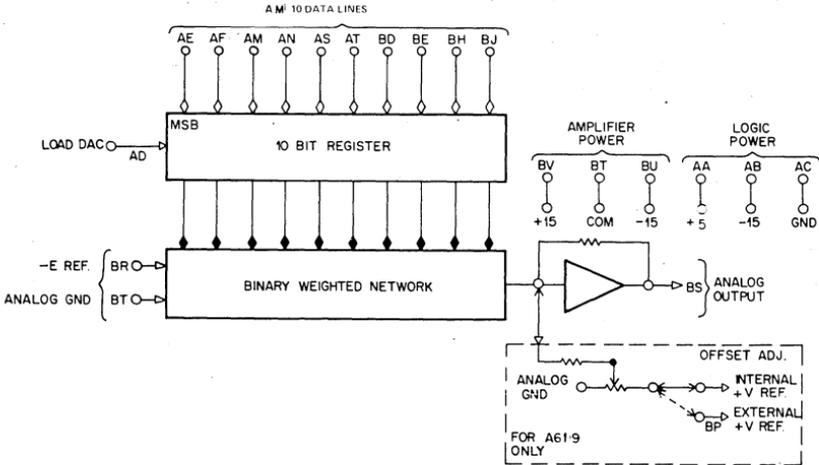
The A618 and the A619 Digital to Analog Converters (DAC) are contained on one DEC double Flip-Chip™ Module. These modules are also double width in the lower (B section) half. The converters are complete with a 10-bit buffer registers, level converters, a precision divider network, and a current summing amplifier capable of driving external loads up to 10 ma. The reference voltage is externally supplied for greatest efficiency and optimum scale factor matching in multi-channel applications.
