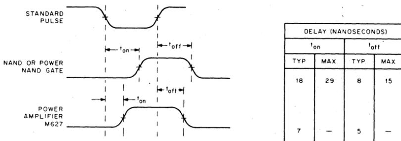
Figure 18. NAND Gate and Power Amplifier Delays
