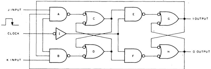
Figure 15. Master-Slave J-K Flip-Flop
