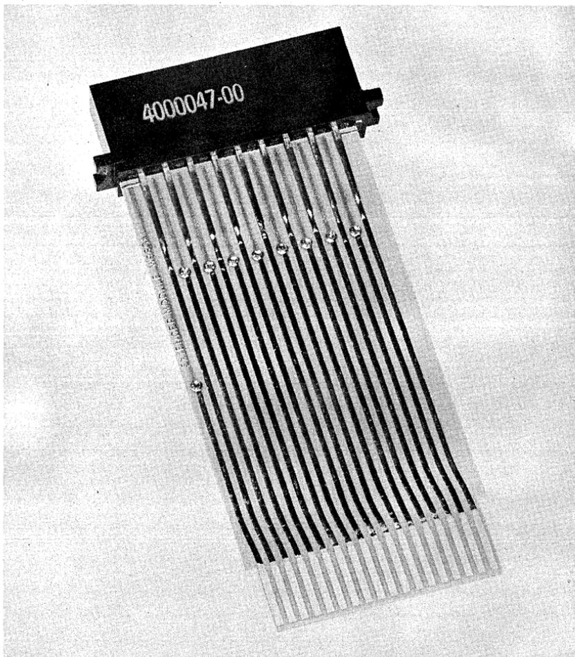
The W980 Module Extender allows access to the module circuits without breaking connections between the module and mounting panel wiring.
