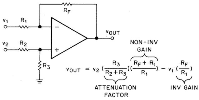
Fig. 9, Differential Gain
