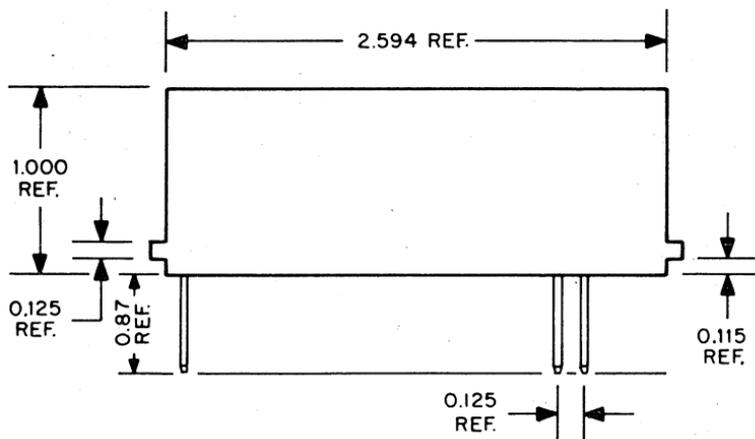
This is an 18 pin connector block for a single FLIP CHIP module. It can be used to mount all modules except those with pins on both sides of the board. Pin dimensions are .031 inches by .062 inches and may be of the wire wrap type only. Number 24 wire should be used with this connector.
