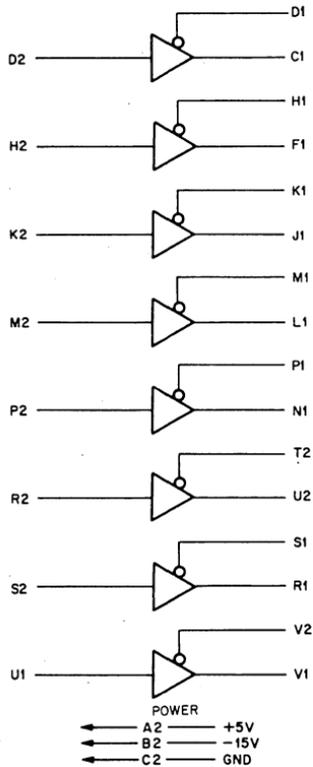
The M500 module is used to convert negative input signals to positive output signals. Each card contains 8 converters and is pin compatible with the M510 positive receiver card.
