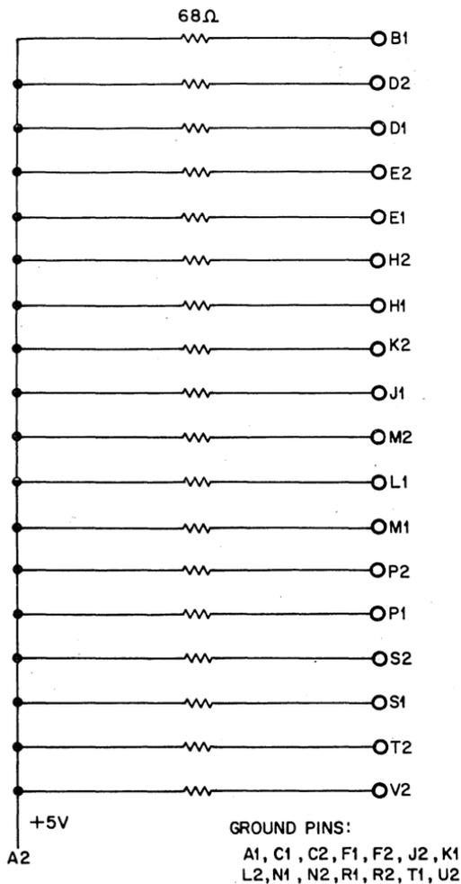
The M910 module contains 18-68Ω resistors. All resistors are tied to a common +5 volts bus.
