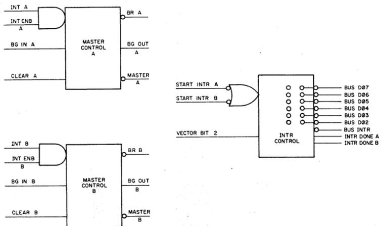
Figure 8 M782 Interrupt Control
