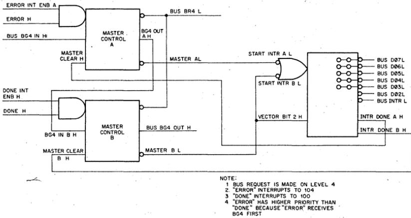
Figure 9. Typical Interconnection of M782 Interrupt Control
