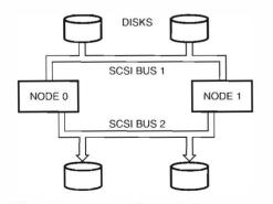
**Figure 5** Typical ASE Configuration
