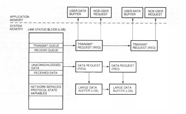
Figure 4 Link Status Block and Associated Data Structures
