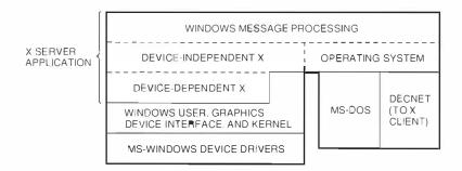
Figure 4 eXcursion X Server Internal Architecture
