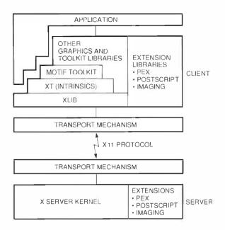
Figure 2 X Client-Server Architecture
