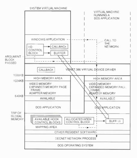
Figure 3 Invoking the Network Process
