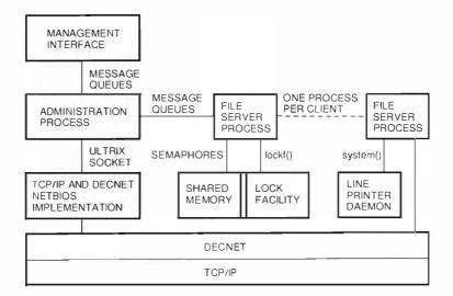
Figure 1 PATHWORKS for ULTRIX Process Model
