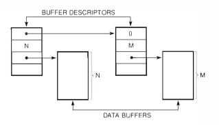
Figure 3 LASTDRIVER Buffering Model
