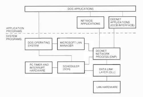
Figure 1 PATHWORKS Client Components
