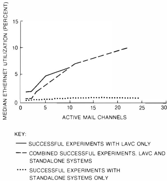
Figure 7 Median Ethernet Utilization versus Mail Load
