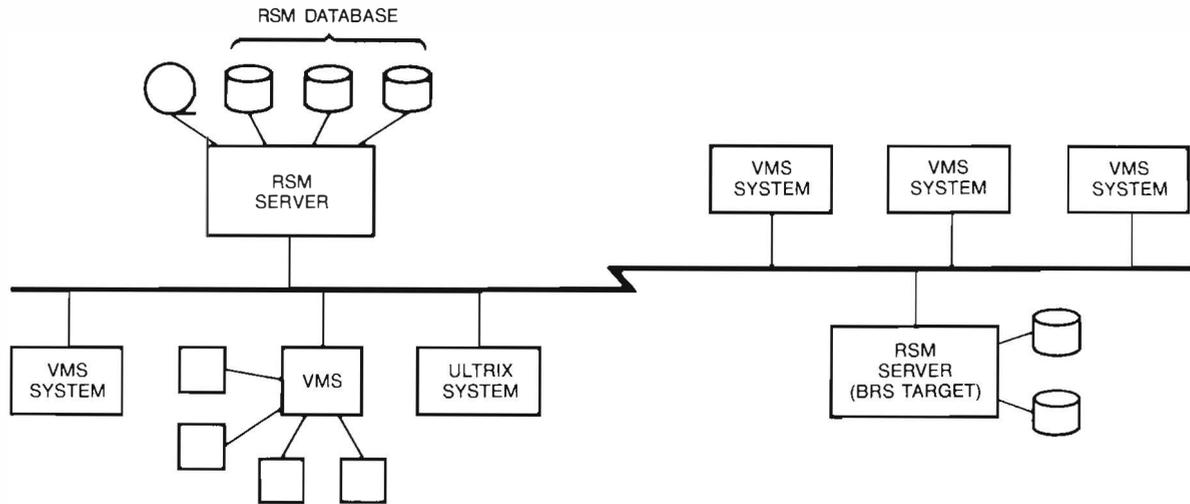
Figure 2 RSM Configured in a Wide Area Network
