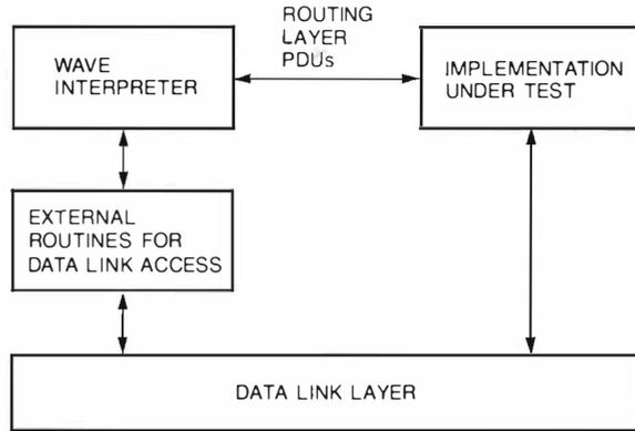
Figure 3 Routing Tester Configuration
