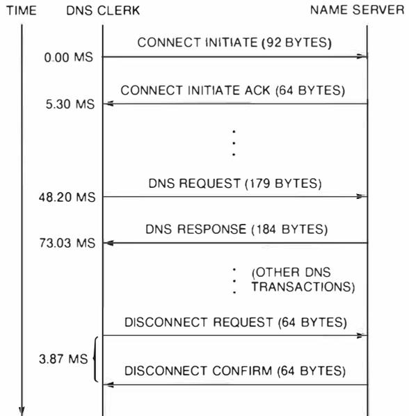
Figure 6 Message Trace for a DNS Operation
