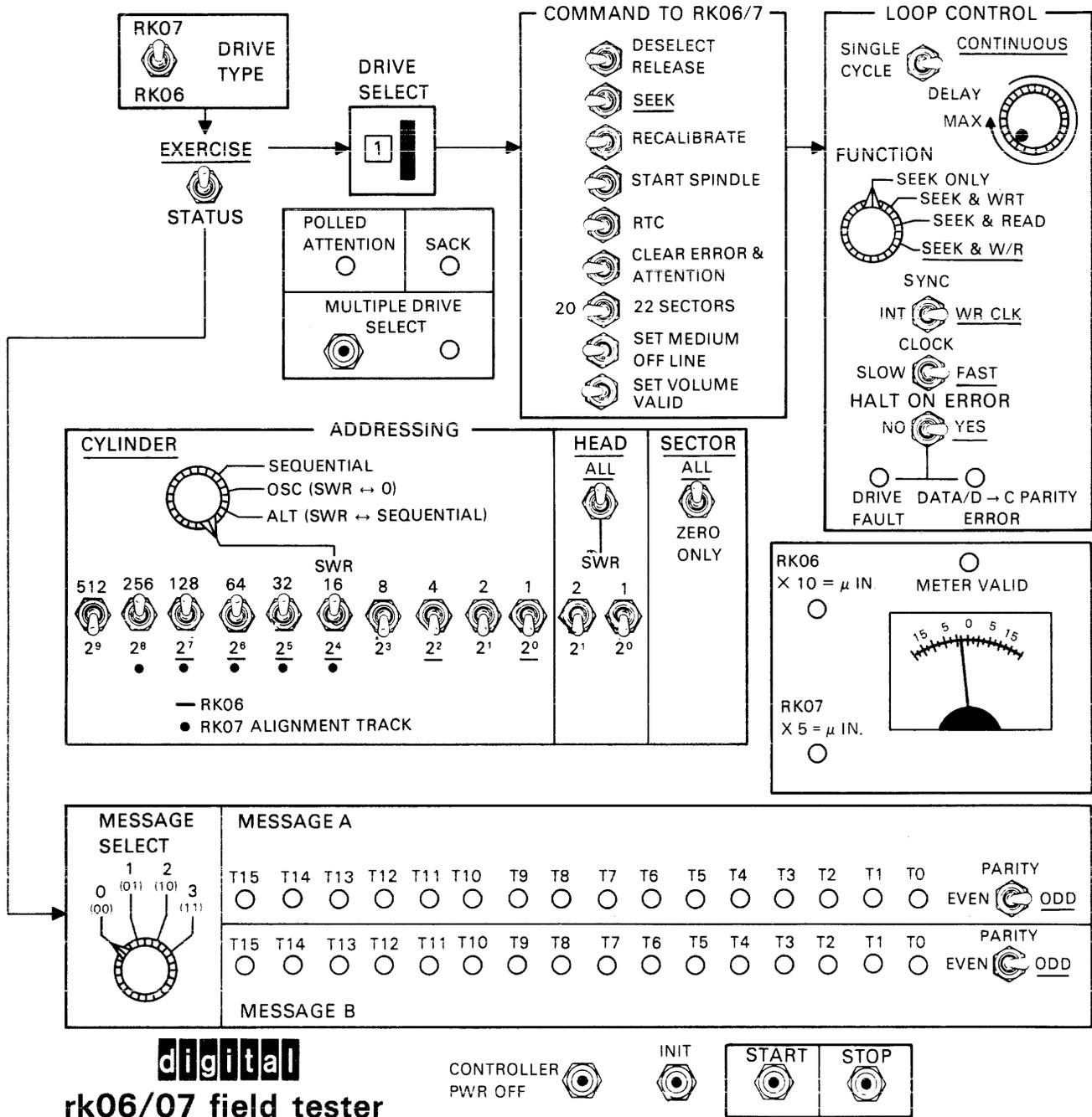
Figure 3-1 Field Test Box Controls and Indicators
