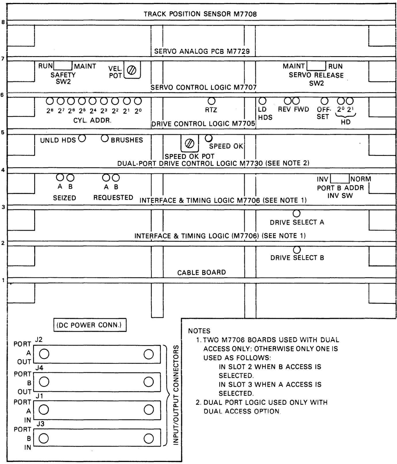
Figure 4-3A Drive Module/Slot Layout
