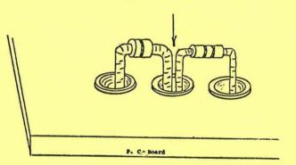
Leads must be able to fit in the same hole without using force.
