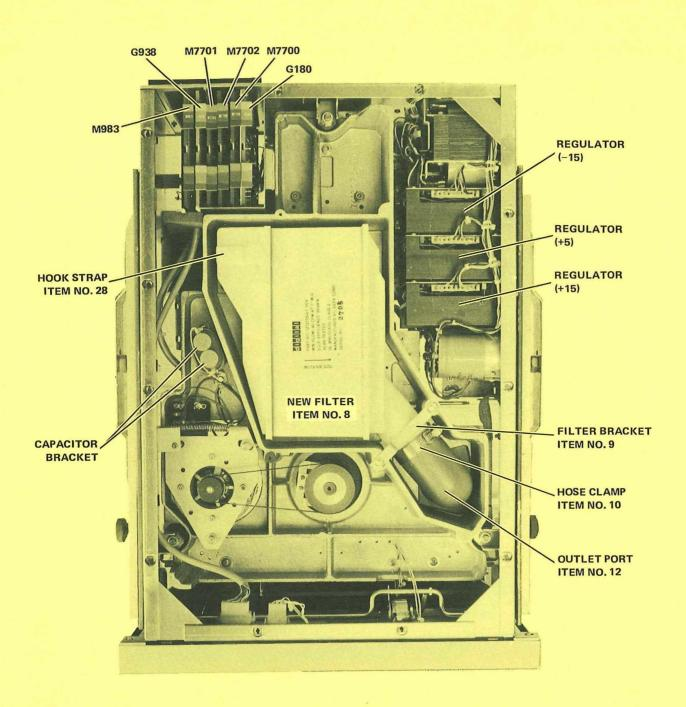
FIGURE NO. 7 NEW FILTER SYSTEM (BOTTOM VIEW)
