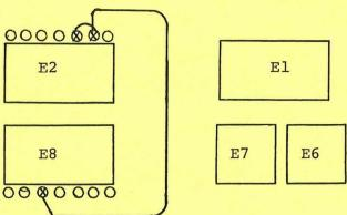
TRY TO PLACE WIRE AS SHOWN BUT DO NOT CEMENT UNTIL ALL WIRES ARE INSTALLED.
