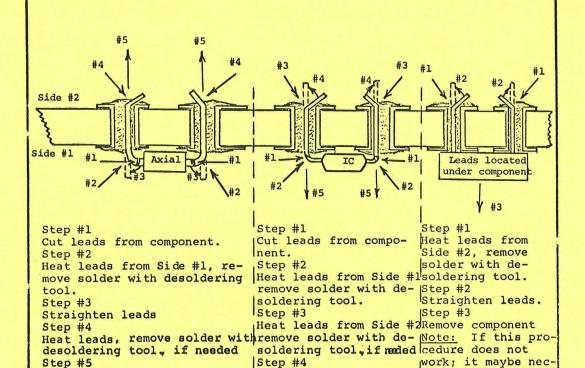
Remove leads from holes. | Straighten leads | Step #5 | Remove leads
