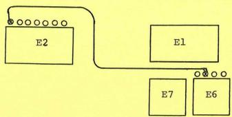
() 6. AT THIS TIME CHECK ETCH CUT AND WIRES ADDED FOR CORRECTNESS. IF THE WIRES ARE INSTALLED PROPERLY THEY CAN BE CEMENTED TO THE PRINTED CIRCUIT BOARD. THIS HELPS PREVENT ANY DAMAGE TO WIRES WHEN MODULE IS INSTALLED OR REMOVED FROM THE DRIVE.
