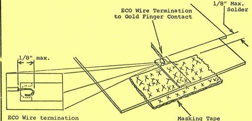
ECO Wire termination suggested, termination shape of strip portion, conductor. 1/8" from insulation to curved portion of the conductor.
