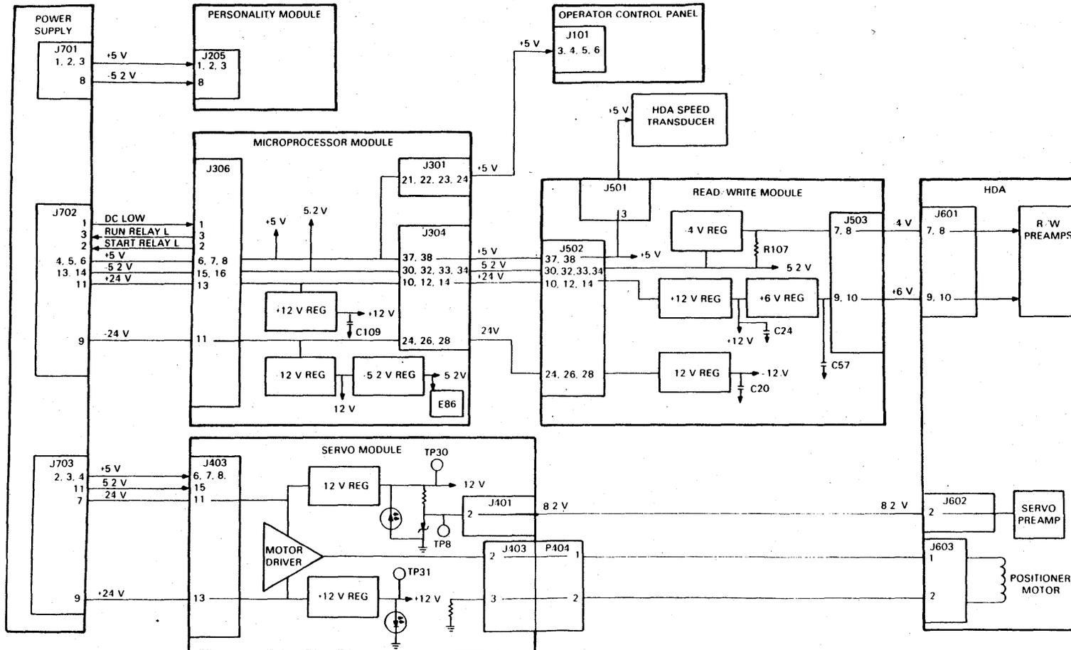
Figure 5-3 Power Distribution Diagram
