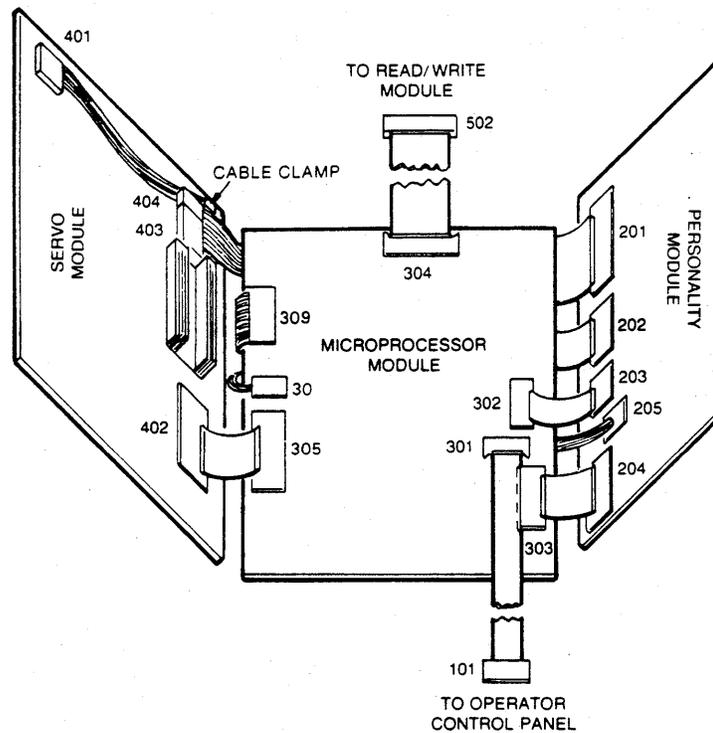
Figure 2-13 Module Connector Locations
