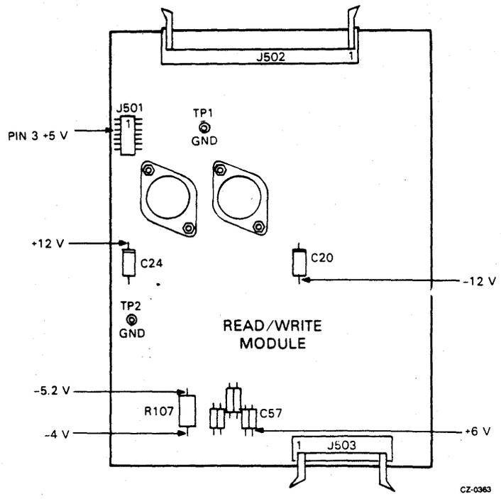
Figure 5-7 Read/Write Module Voltage Checkpoints
