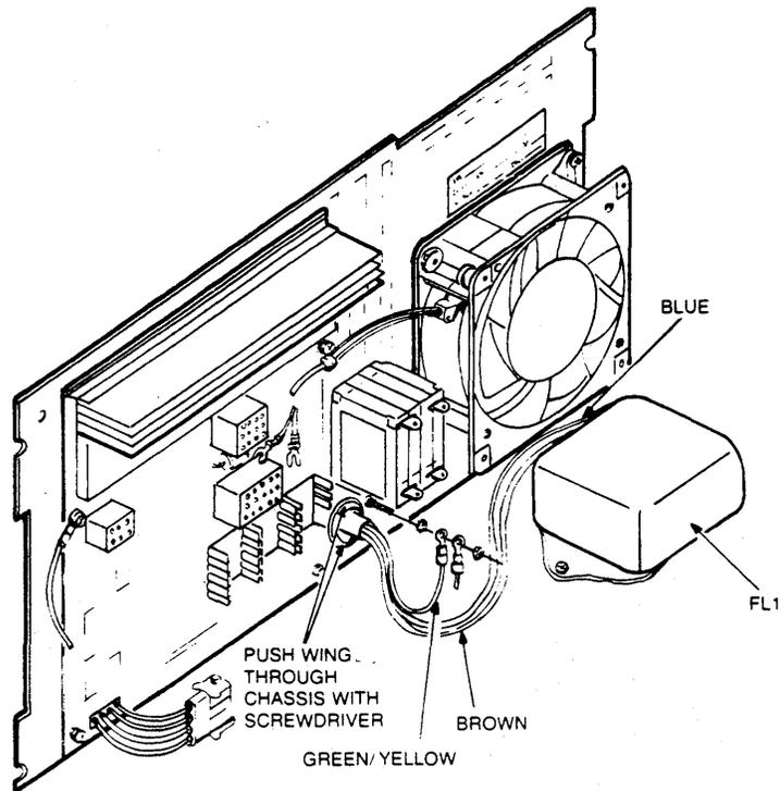
Figure 2-32 Drive AC Line Cord Replacement
