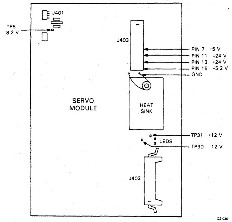
Figure 5-5 Servo Module Voltage Checkpoints
