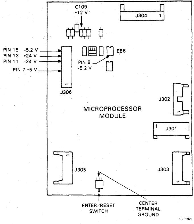
Figure 5-4 Microprocessor Module Voltage Checkpoints
