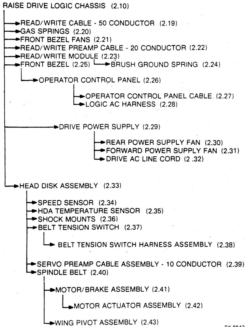
Figure 2-3 FRUs Accessed by Raising the Drive Logic Chassis
