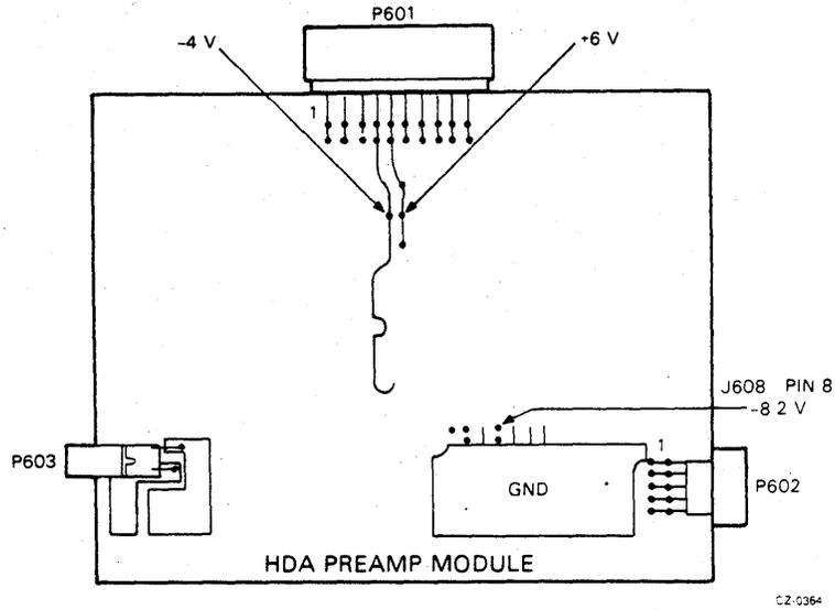
Figure 5-8 HDA Preamplifier Voltage Checkpoints
