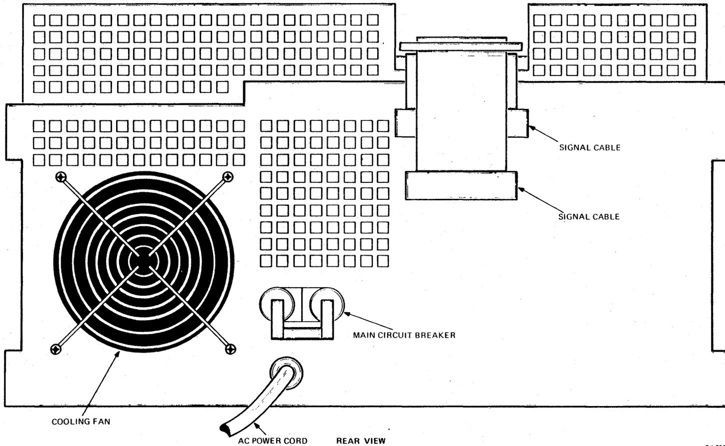
Figure 2-1 Location of Disk Drive Power Controls
