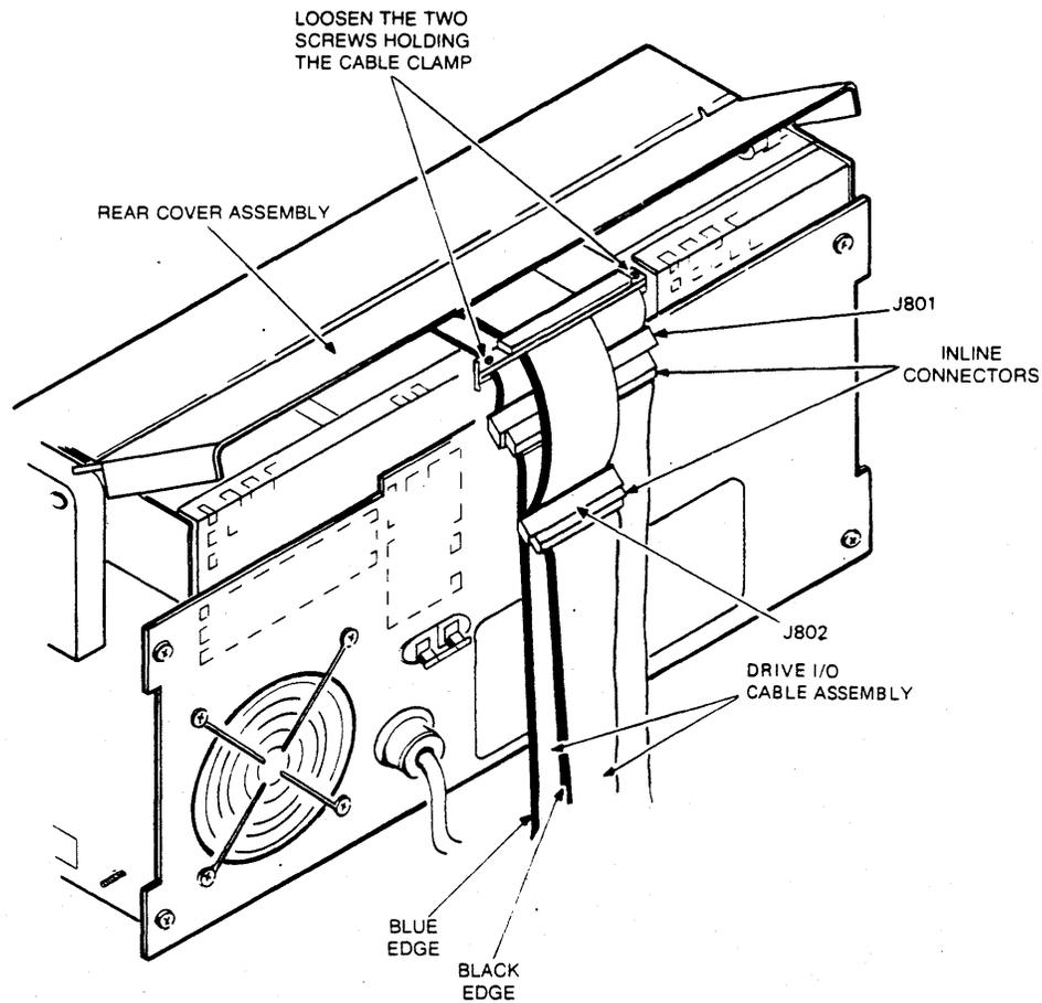
Figure 2-18 Drive I/O Cable Replacement
