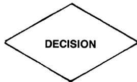
**DECISION** - A diamond indicates that a decision is made. For example, whether to go on with the following step or to “branch” to a different step.
