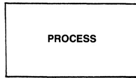
**PROCESS** - A rectangle indicates that the computer is performing a processing task such as an arithmetic calculation or other defined operation causing a change in value, form, or location of information.
