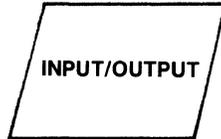
**INPUT/OUTPUT** - A parallelogram indicates the input or output of data; that is, it represents information available for processing (input), or the recording of processed information (output).
