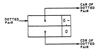
When a function returns a dotted pair (A.B) as its value it is returning a pointer to a cell as shown:
