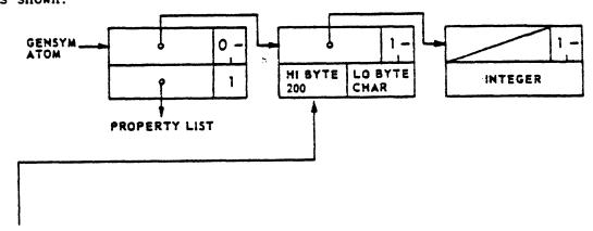
NOTE: Characters in strings and atom PNAMES are formed from 7-bit ASCII values; thus bit 15 can be used to signal a GENSYM atom. (This property is only needed on printout and is not checked or used by any other LISP functions besides GENSYM and PNAME.)
