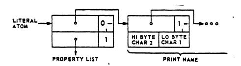
Given a pointer to a cell in RO: (1) if D is non-zero at (RO) then RO points to a number, (2) else if F at 2(RO) is zero then RO points to a dotted pair, (3) else if F at 2(RO) is 2 or 3 then RO points to a string atom, (4) else RO points to a literal atom.
