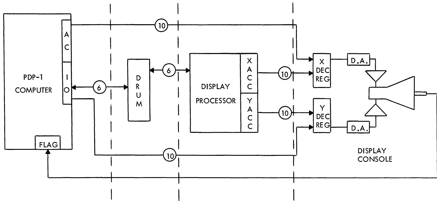
Figure 1 Display System Block Diagram
