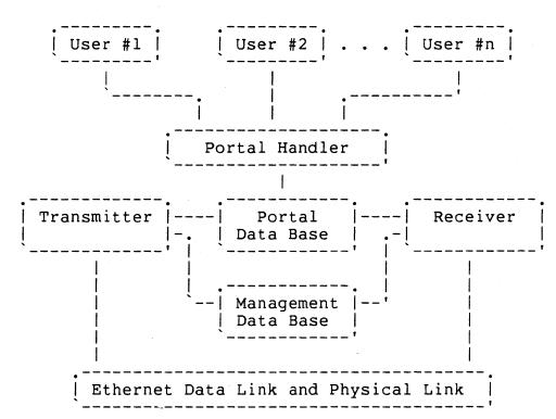
The Portal Handler maintains the Portal Data Base according to user requests through the User Interface. The Portal Handler communicates with the Transmitter and Receiver through the Portal Data Base. The Transmitter and Receiver send and receive frames through the DNA Ethernet Data Link User Interface and maintain counter and event information in the Management Data Base.
