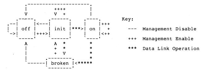
Network management can enable the channel. From the "off" or "broken" states, this enable causes a transition to "init". From the "on" state, enable has no effect.
