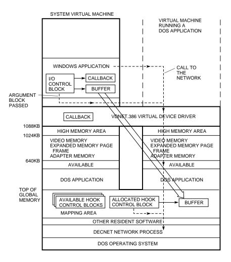
Figure 3 Invoking the Network Process
