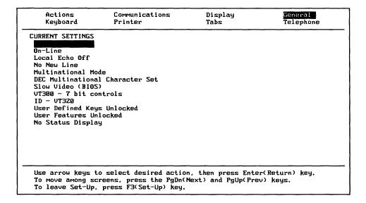
2. Use to move the video bar to the Multinational Mode choice in the CURRENT SETTINGS column. Two choices (NRC and Multinational Mode) appear in the SELECTIONS column, as shown in Figure 2–8.
