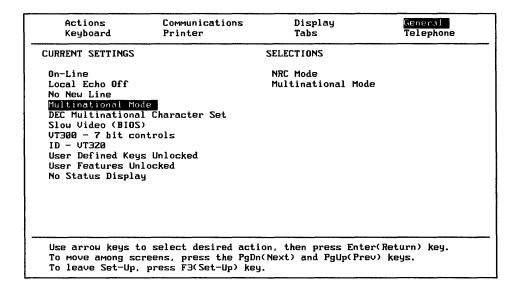
3. Use ⇒ to move to the SELECTIONS column. Then, use ⋒ and w to move the video bar to the NRC Mode option. After you highlight NRC Mode, press Return. To move back to the CURRENT SETTINGS column without making a selection, press ←.
