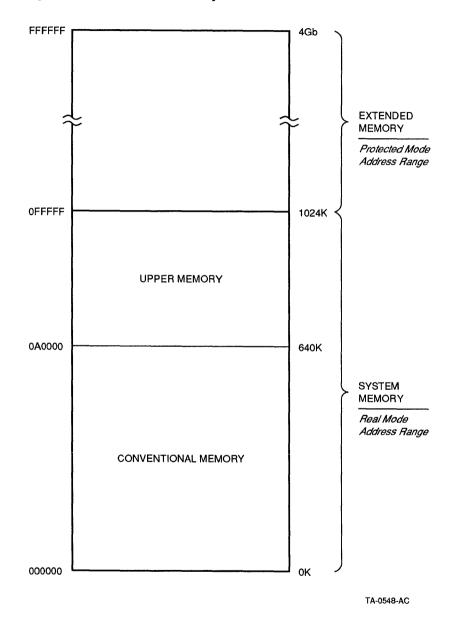
Figure 1–6 Extended Memory on a 80386 PC
