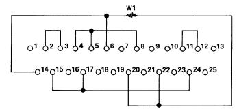
Use this connector to test DV, DUP, DZ, and DMC interfaces. When used with the DV11 interface, remove W1.
