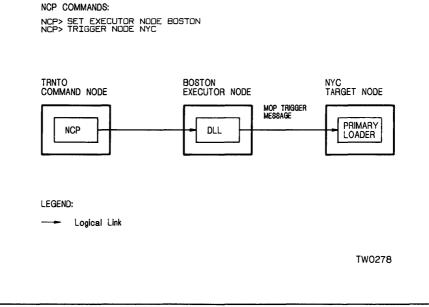
When you use the LOAD command, the executor node proceeds with the load operation according to the options specified in the initial load request. Any required information that has been defaulted is obtained from the volatile database. With this information, the executor is thereby able to control the load sequence.
