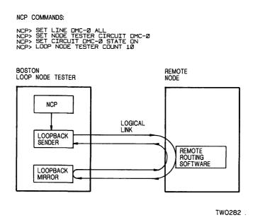
For this test, you first load the line and set a loop node name for the circuit to the adjacent node. Next, turn on the circuit. Finally, issue the LOOP NODE command using the loop node name, as shown in the following example:
