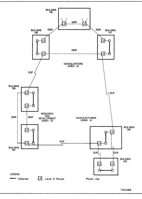
Each area is a complete level 1 network. When configuring each area, you must ensure that there are redundant paths to the level 2 routers in the area. Redundant paths help to maintain the availability of the other areas in the network.
