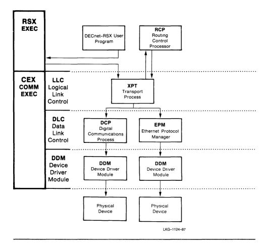
Figure 8–5: DECnet-RSX System Illustrating Routing
