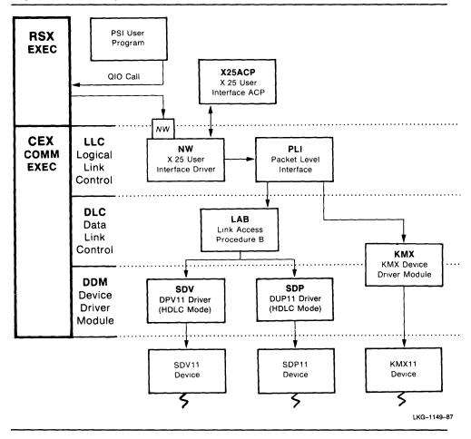
Figure 8-31: Physical Communications Devices for a PSI System
