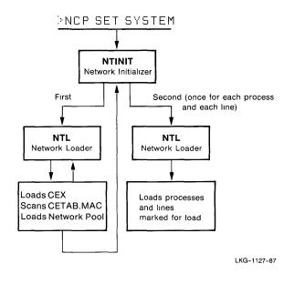
Figure 8–9 illustrates the process of turning on the network using the NCP SET EXECUTOR STATE ON command. The sequence of processing is:
