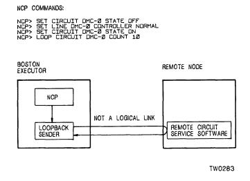
In the first step of this test, you turn the circuit off. Next, you set the controller to its normal operational mode and put the circuit in the ON state. Finally, you issue the LOOP CIRCUIT command. This sequence is shown in the following example:
