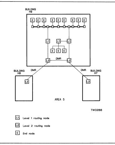
Once you have designed the network from the level 2 routers down to the end nodes, you should actually install the network in a bottom-up manner:
