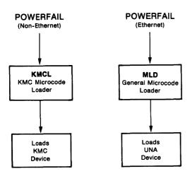
Figure 8-11: Loading KMC Devices with Microcode
