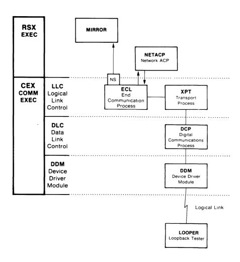
Figure 8-20: Node Level Loopback Testing
