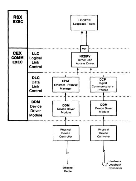
Figure 8-18: Hardware Loopback Circuit Testing
