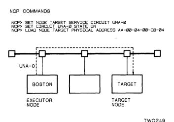
Figure 5-4: Operator-initiated Down-line Load over an Ethernet Circuit (NCP LOAD)
