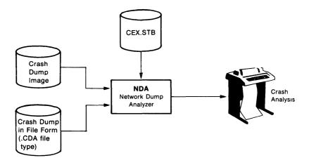
Figure 8-17: Network Crash Dump Analyzer
