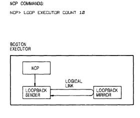
Figure 4-4: Local Loopback Test
