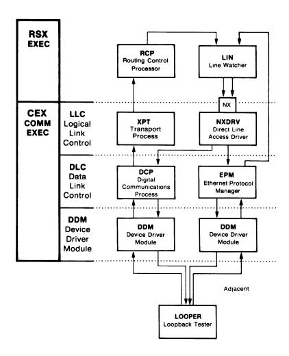
Figure 8-19: Circuit/Line Level Loopback Testing
