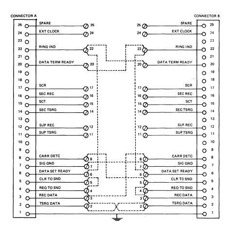
Figure 4-14: EIA Asynchronous Null Modem Wiring Diagram
