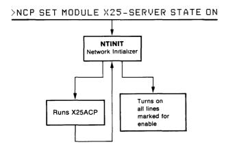
Figure 8-10: Turning On the X.25 Server
