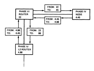
Figure 7-5: A Phase III Routing Node in a Phase IV Routing Path
