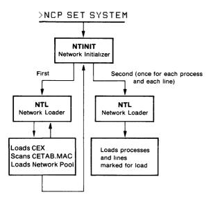
Figure 8-8: Loading the Network
