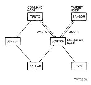
Figure 5-3: Operator-initiated Down-line Load over a DDCMP Circuit (NCP TRIGGER)
