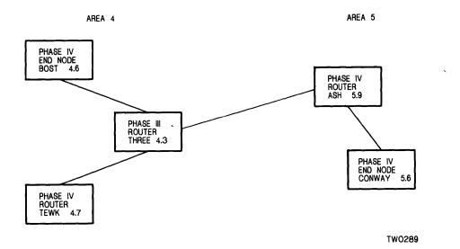
Figure 7-7: Area Leakage with Phase III Nodes
