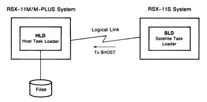
Figure 8-29: Down-line Task Loading
