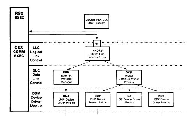
Figure 8-7: DECnet-RSX Operations with DLX
