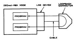
Figure 4-18: External Loopback Test Using a Loopback Connector
