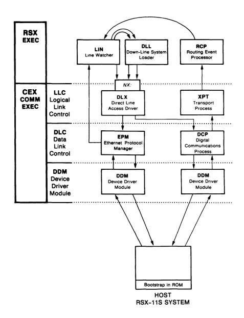
Figure 8-27: Down-line System Loading
