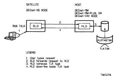
Figure 5-6: Down-line Task Loading an RSX-11S Task
