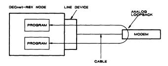
Figure 4-16: External Loopback Test Using a Modem
