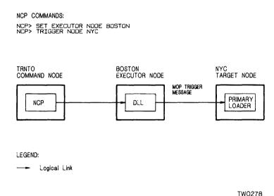
Figure 5-2: Operator-initiated Down-line Load
