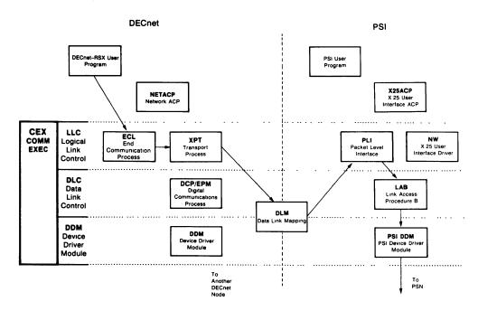
Figure 8-32: Combined DECnet-RSX/PSI System
