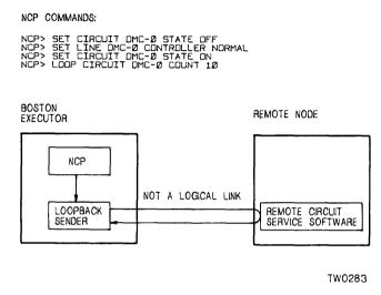
Figure 4-5: Circuit Level Software Loopback Test
