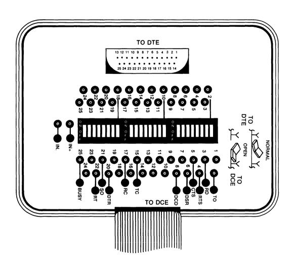
Figure 4-15: Typical Breakout Box
