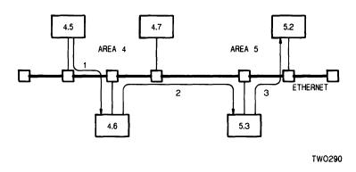
Figure 7-8: A Multiple Area Ethernet
