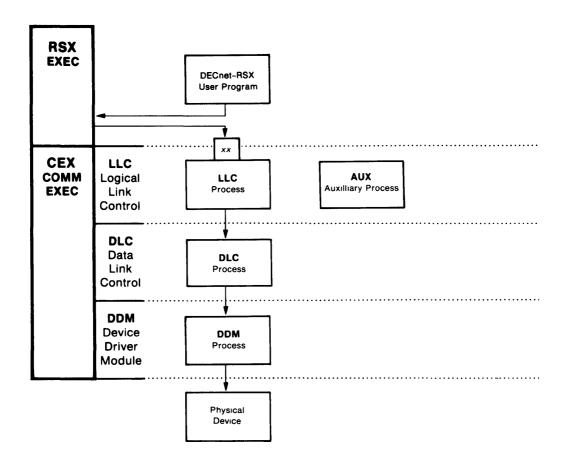
Figure 8-1: CEX Environment Illustrating Transmission
