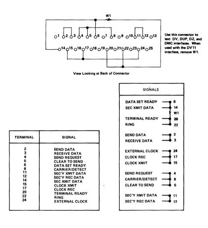
Figure 4-13: H325 Loopback Connector Wiring Diagram
