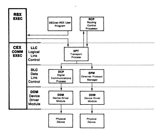
Figure 8-5: DECnet-RSX System Illustrating Routing
