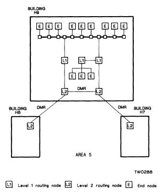
Figure 7-3: A Portion of the Level 1 Network in Area 5
