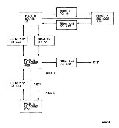
Figure 7-6: An Example of an Improperly Placed Phase III Node
