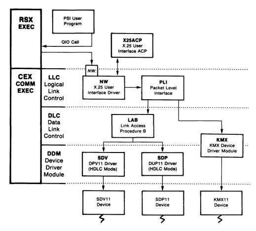
Figure 8-31: Physical Communications Devices for a PSI System
