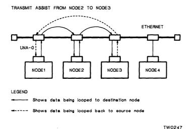
Figure 4-7: Loopback Test Using an Assistant Giving Transmit Assistance
