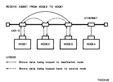
Figure 4-8: Loopback Test Using an Assistant Giving Receive Assistance
