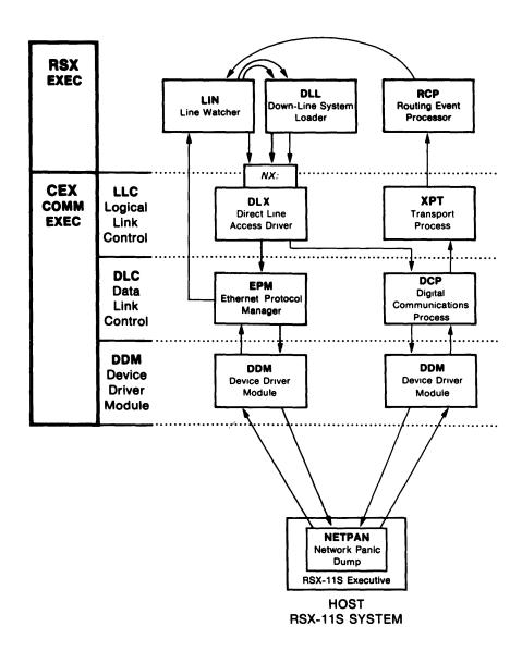
Figure 8-28: Up-line System Dumping
