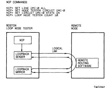
Figure 4-2: Local-to-remote Loopback Test Using a Loop Node Name
