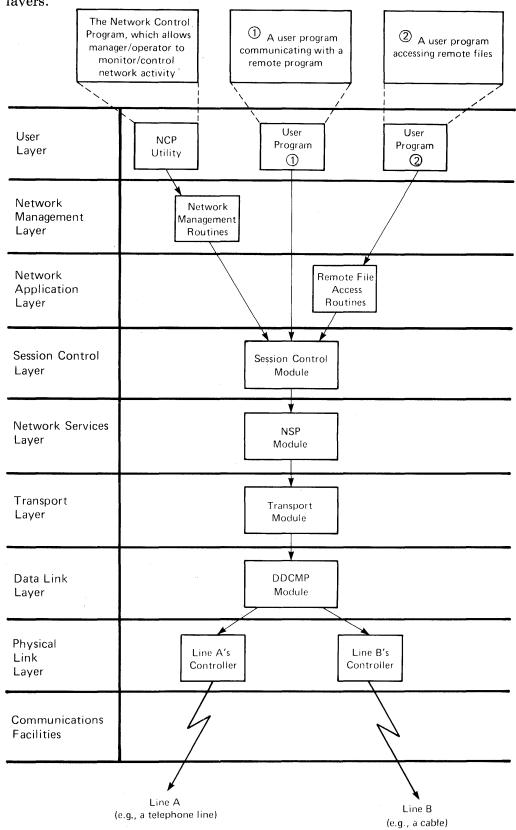
Figure 1–3 shows a typical DECnet node containing multiple modules in some layers.
