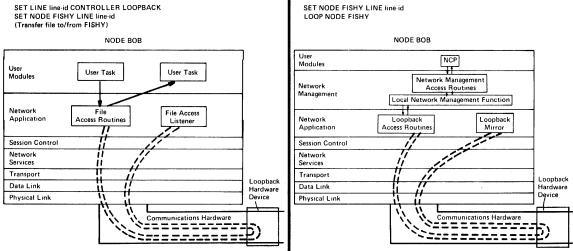
C. Local-to-Loopback Node Test, Two Nodes, using user task
