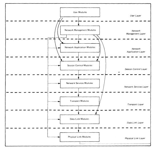
Black arrows show direct access for control and examination of parameters, counters, etc. Red arrows show interfaces between layers for normal user operations such as file access, down-line load, up-line dump, end-to-end looping, and logical link usage.
