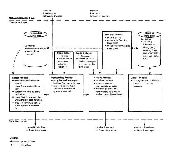
Figure 3-4: Transport Control Components and their Functions
