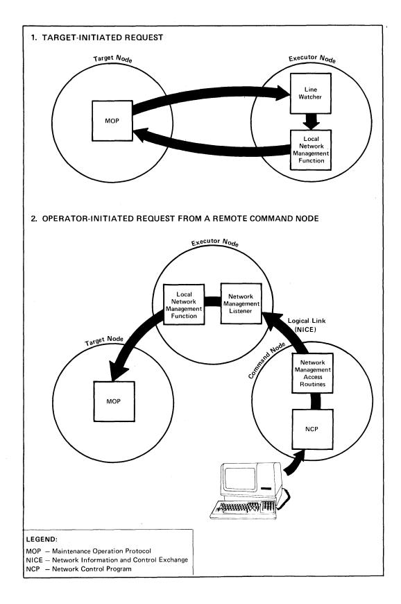
Figure 7-2: Down-Line Load Request Operation
