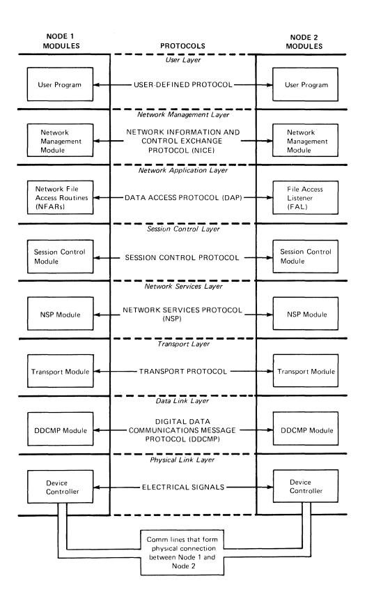
Figure 1-4: Protocol Communication between Two Nodes
