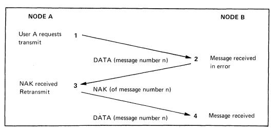
Figure 2-5: DDCMP Message Exchange, Showing Error Recovery
