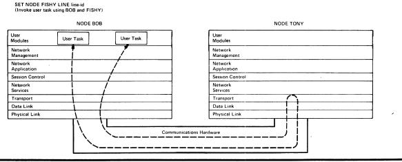
D. Local-to-Loopback Node Test, Two Nodes, using loopback mirror and test messages SET NODE FISHY LINE line id LOOP NODE FISHY
