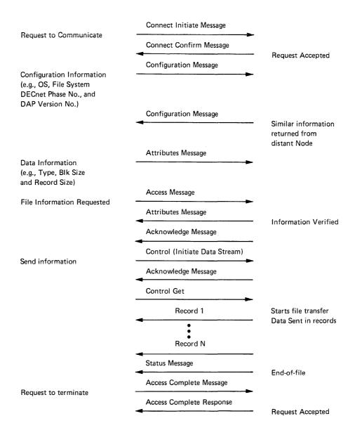
Figure 2-1. Typical DAP Message Exchange (Sequential File Retrieval)
