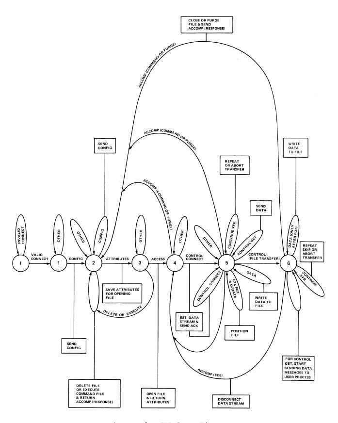
Figure B-l. FAL State Diagram
