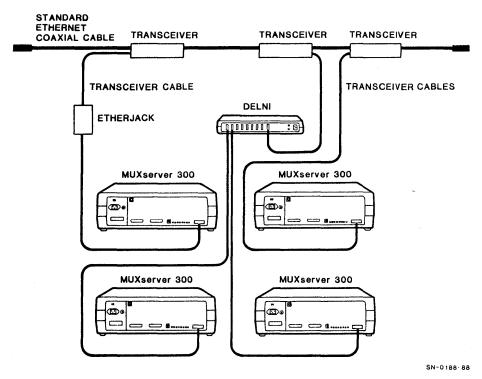
Figure 9 Standard Ethernet Coaxial Cable Connection
