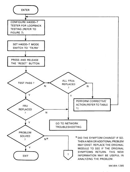
Figure 6 Troubleshooting Flow Diagram (Sheet 1 of 4)
