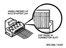
Figure 25 Cap Ridge in Connector Slot
