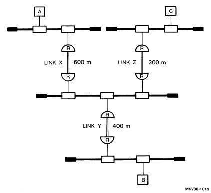
Figure 7 Multiple-Segment Ethernet with Remote Repeaters
