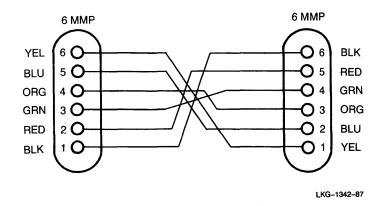
Figure 11 6MMP-to-6MMP Pin Diagram (DIGITAL/3 Foot)
