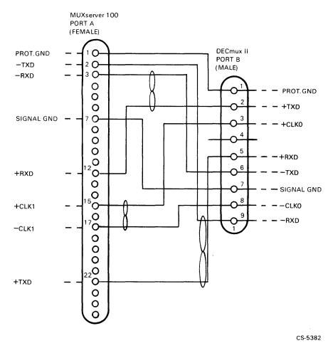
Figure 9 RS-422 DECmux II (Port B) to MUXserver 100 (Port A)
