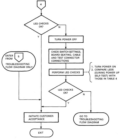
Figure 1 Installation Flow Diagram (Sheet 5 of 5)
