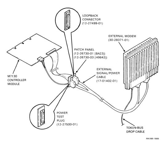
Figure 8 DTQNA External Installation in BA23A, BA123, and H9642 Systems (DTQNA-BB and -BE)
