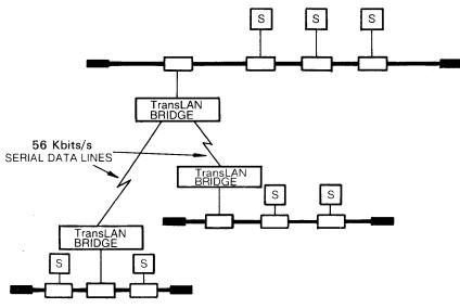
Figure 18 TransLAN Bridge Extended Network Configuration
