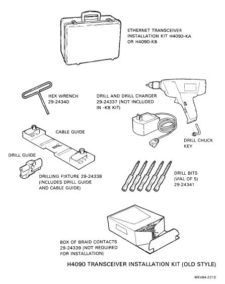
Figure 1 Transceiver Installation Kit Parts (Sheet 1 of 2)
