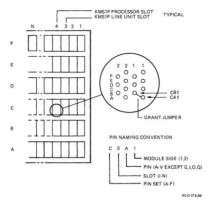
Figure 3 Locating the NPG Jumper
