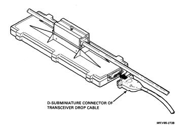
Figure 3 Ethernet H4000 Transceiver with Removable Tap Assembly
