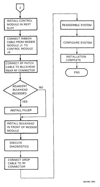
Figure 6 Installation Flowchart for DTQNA in BA2XX Systems (Sheet 3 of 3)
