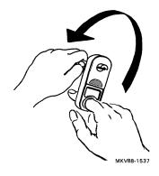
12. Pull the tool off the cable and remove any debris that remains inside the hole.
