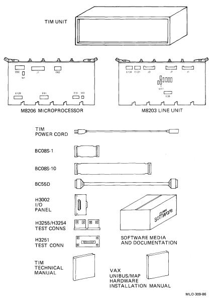
Figure 2 DTUNA Hardware Component Parts Diagram
