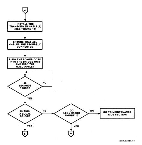
Figure 6 LAN Bridge 200 Installation Flow Diagram (Sheet 5 of 6)
