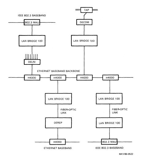
Figure 3 LAN Bridge 100 Connections
