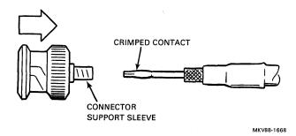
20. Slip the support sleeve under the braid and over the dielectric.
