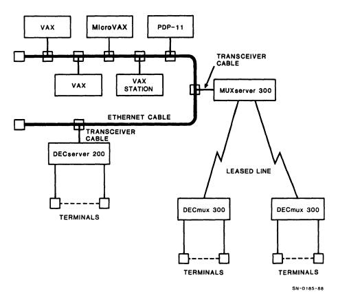
Figure 2 MUXserver/DECmux 300 Network
