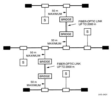
Figure 16 Extended Network with LAN Bridge 100 Remote Bridges
