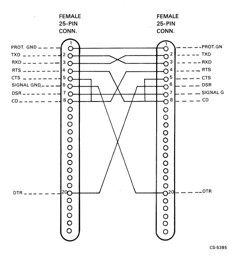
Figure 12 RS-232-C Asynchronous Null Modem Connection
