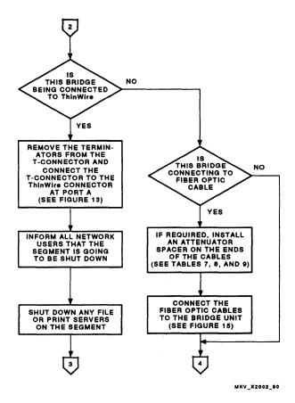
Figure 6 LAN Bridge 200 Installation Flow Diagram (Sheet 3 of 6)
