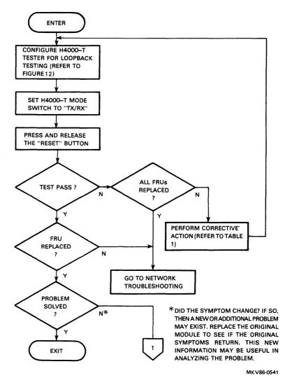
Figure 11 Troubleshooting Flow Diagram (Sheet 1 of 4)
