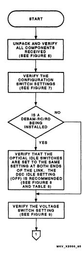
Figure 6 LAN Bridge 200 Installation Flow Diagram (Sheet 1 of 6)
