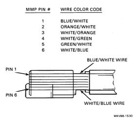
6. Insert the MMP connector into the die-cut mouth of the MMP terminating tool (H8241) until it locks in place.
