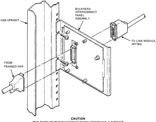
THE BACK OF THE BULKHEAD PANEL CONTAINS A CIRCUIT BOARD THAT CARRIES -15 V. BE SURE THIS CIRCUITRY DOES NOT TOUCH ANYTHING THAT COULD CAUSE A SHORT CIRCUIT ON POWER-UP.
