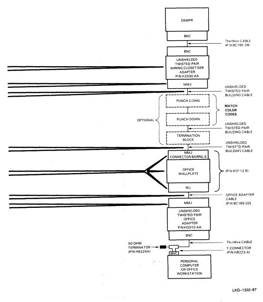
Figure 17 Northern Telecom Unshielded TP Connections (Sheet 2 of 2)
