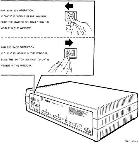
Figure 8 Selecting Operating Voltage
