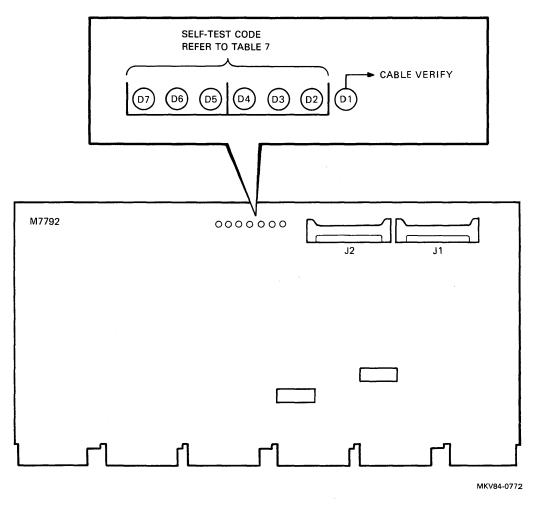
Figure 10 DEUNA Port Module Self-Test LEDs
