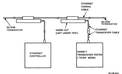
The following figure shows a configuration for a single H4000-T transceiver tester connected to an H4000 UUT (unit under test).
