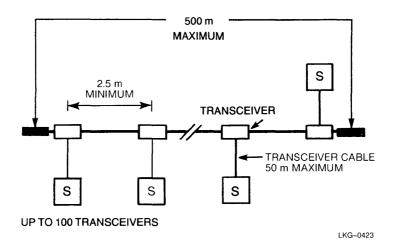
Figure 4 Standard Ethernet Coaxial Cable Segment
