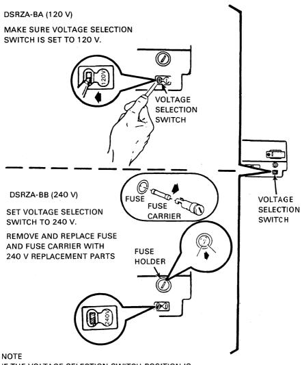
IF THE VOLTAGE SELECTION SWITCH POSITION IS CHANGED, THE FUSE AND FUSE CARRIER MUST ALSO BE CHANGED TO MATCH.
