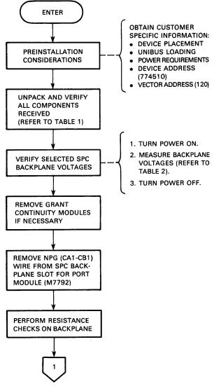
Figure 1 Installation Flow Diagram (Sheet 1 of 5)
