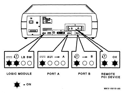
Figure 21 Remote LAN Bridge 200 Loopback Test Status LEDs
