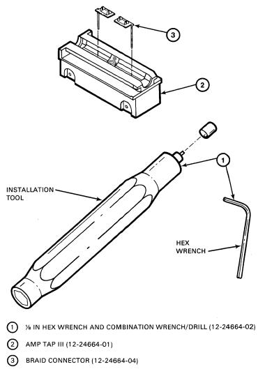
Figure 5 CD Kit for H4000 Transceiver with Removable Tap
