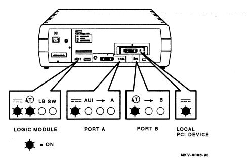
Figure 20 Local LAN Bridge 200 Loopback Test Status LEDs
