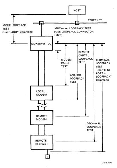
Figure 15 Diagnostic Test Loopback Points
