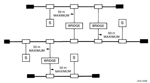
Figure 15 Extended Network with LAN Bridge 100 Local Bridges
