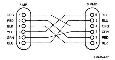
Figure 13 6MP-to-6MMP Pin Diagram (Northern Telecom)
