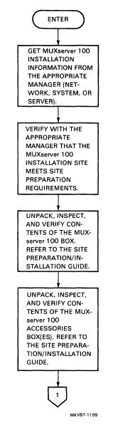
Figure 6 Installation Flow Diagram (Sheet 1 of 3)
