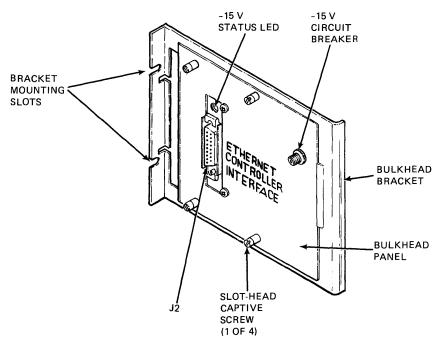
Figure 5 Bulkhead Interconnect I/O Panel Assembly
