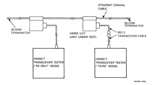
Figure 8 Typical H4000-T Configuration for End-to-End Testing
