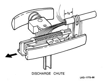
8. Starting at the connector end opposite the cable clamp, slide the index until the contact that is to be terminated aligns with the tool's wire slot.
