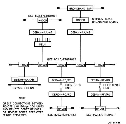
Figure 4 shows transceiver cables connecting bridges to various network interconnect devices.
