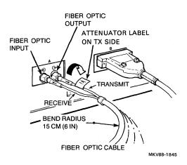
Figure 18 Connecting Fiber Optic Cable to DEBET-RH/RJ
