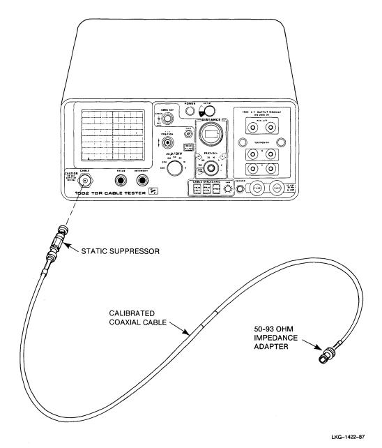
Figure 27 Tektronix TDR 1502 and Accessories.
