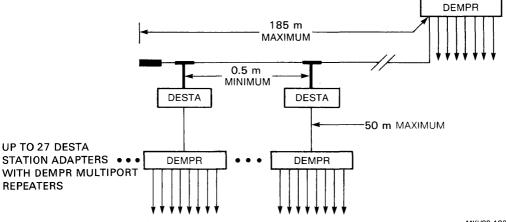
Figure 11 Standalone Cascading DEMPR Configuration
