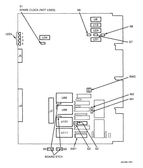
Figure 2 M7130 Controller Module Switch and Jumper Location
