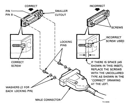
Figure 19 Proper Slide-Latch Configuration
