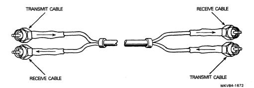
Figure 8 Duplex Fiber-Optic Cable
