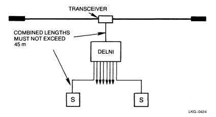
Figure 5 Connecting a DELNI to a Standard Ethernet Coaxial Cable Segment
