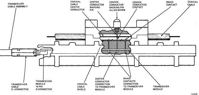
Figure 9 H4000 Ethernet Transceiver: Cutaway View Showing Coaxial Cable Interface
