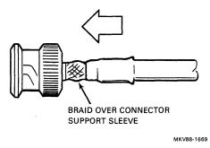
21. Slide the ferrule over the support sleeve to the back of the connector.
