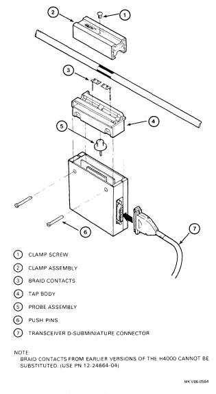
Figure 4 Hardware for Installing the H4005 Transceiver on a Cable
