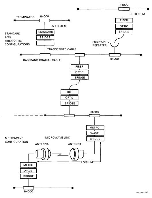
Figure 19 Extended Baseband LAN with METROWAVE Bridge
