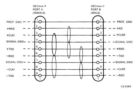
Figure 11 RS-422 Port A to Port B (DECmux II)
