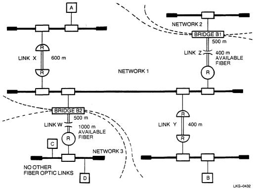
Figure 17 Remote Bridge/Repeater Configuration
