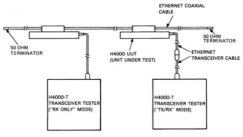
Figure 13 Typical H4000-T Configuration for End-to-End Testing
