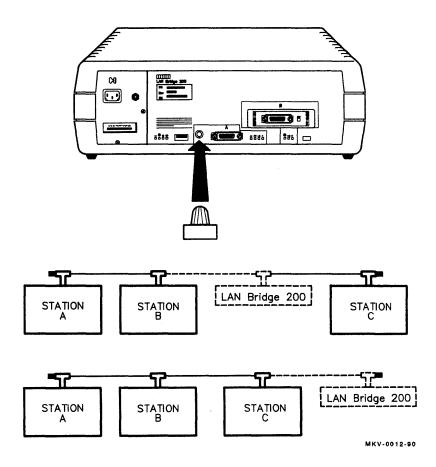
Figure 13 Connecting ThinWire Ethernet Coaxial Cables
