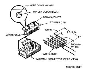
Figure 23 Placement of Wire over the Connector Barrels
