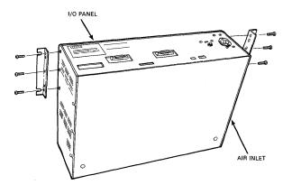
NOTE: BRACKETS ARE SUPPLIED. THE MOUNTING HARDWARE MUST BE OBTAINED SEPARATELY.
