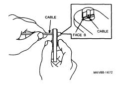
5. Rotate the tool clockwise until cutting stops.
