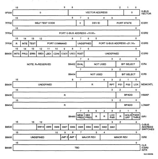
Figure 12 DTQNA Internal Registers
