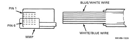
5. Insert the cable into the MMP connector and push it in as far as it will go (about 1/4 inch).
