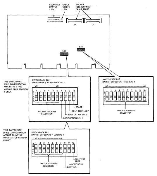
Figure 2 M7792 Switchpacks and Jumpers (Sheet 1 of 2)
