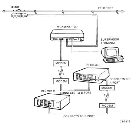
Figure 4 Default Multiplexer Configuration Number 2
