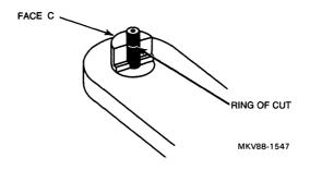
8. Rotate the tool clockwise until cutting stops.
