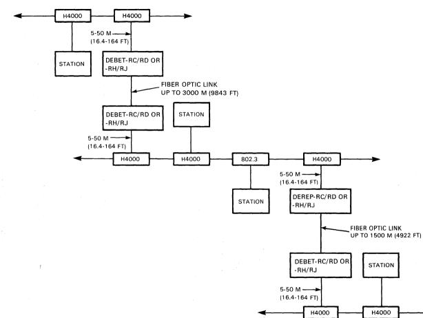
Figure 2 DEBET-RC/RD or -RH/RJ Configuration
