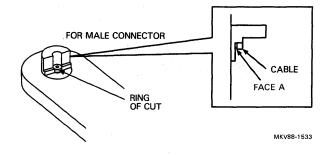
NOTE For steps 8 and 9, hold the tool as shown below for steadier cutting.
