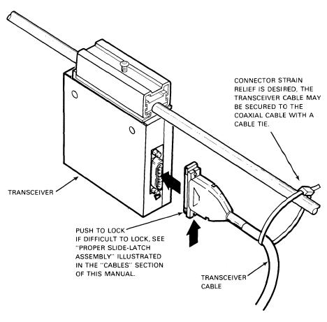
Figure 5 Typical Transceiver Cable Connection
