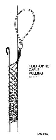
Figure 23 Fiber-Optic Pulling Device
