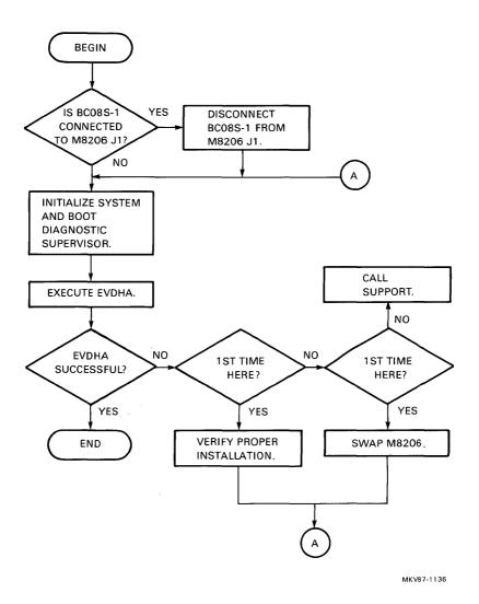
Figure 10 Using EVDHA to Test the M8206 Microprocessor
