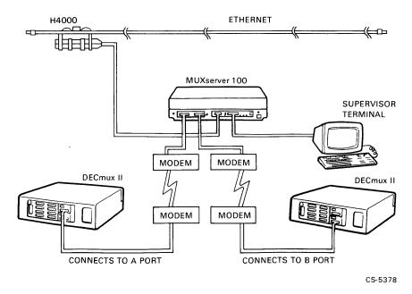
Figure 3 Default Multiplexer Configuration Number 1
