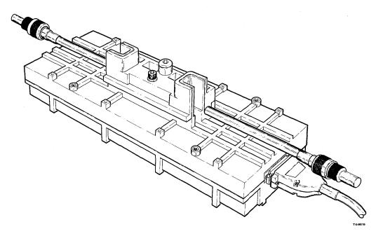
Figure 3 H4080 Loopback Test Connector
