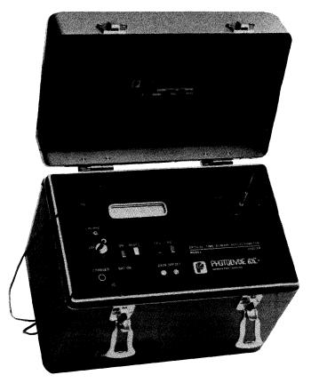
Figure 6 Photodyne Model 5500 FOTDR
