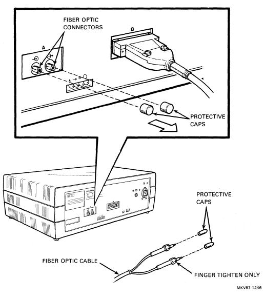
Figure 16 Fiber Optic Cable Attachment
