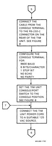
Figure 4 DTUNA Hardware Installation Flowchart (Sheet 6 of 7)
