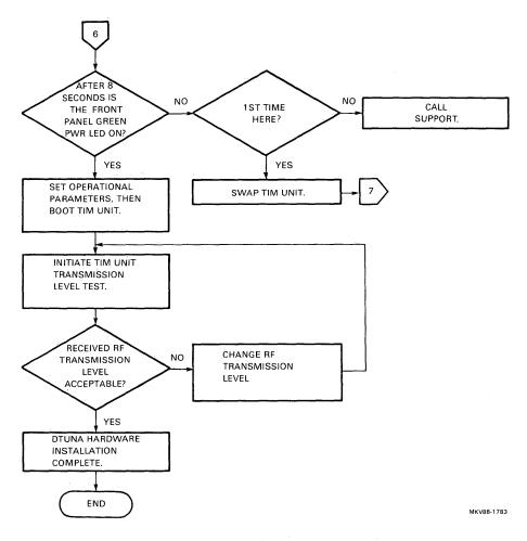
Figure 4 DTUNA Hardware Installation Flowchart (Sheet 7 of 7)
