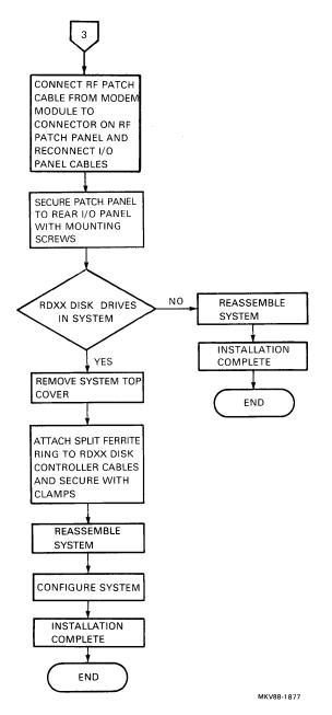
Figure 5 Installation Flowchart for DTQNA in BA23A, BA123, and H9642 Systems (Sheet 3 of 5)
