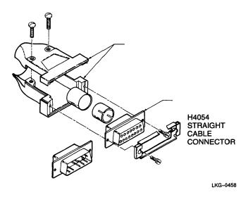
Figure 21 H4054 Transceiver Cable Straight Connector Kit
