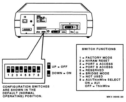
Figure 7 Configuration Switch Settings
