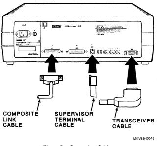
Figure 7 Connecting Cables
