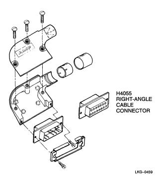
Figure 22 H4055 Transceiver Cable Right-Angle Connector Kit
