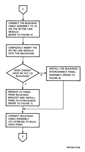
Figure 1 Installation Flow Diagram (Sheet 3 of 5)
