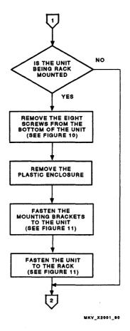
Figure 6 LAN Bridge 200 Installation Flow Diagram (Sheet 2 of 6)
