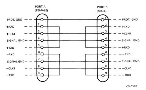
Figure 14 Cable RS-422 Test (DECmux II)
