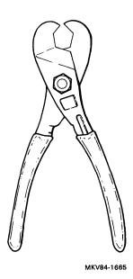
Figure 12 DIGITAL 29-24667 Coaxial Cable Cutter
