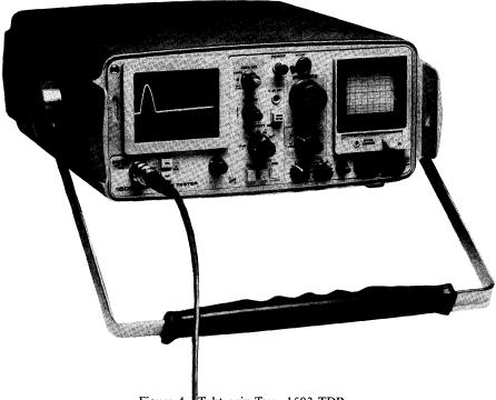
Figure 4 Tektronix Type 1503 TDR
