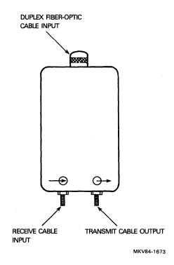
Figure 9 DEXJB Fiber-Optic Junction Box
