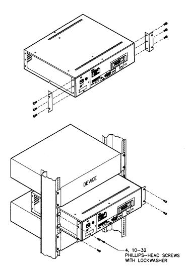
NOTE ALWAYS LEAVE AT LEAST 2.54 cm (1 in) OF SPACE BETWEEN MOUNTED DEVICES FOR PASSING CABLES TO THE BACK OF THE RACK.
