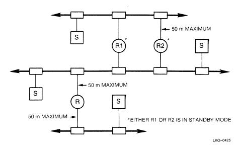
Figure 6 Multiple-Segment Ethernet with Local Repeaters
