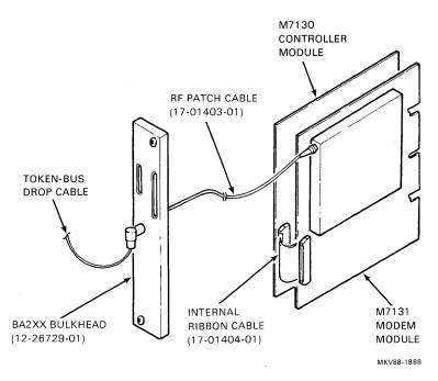
Figure 9 DTQNA Internal Installation in BA2XX Systems (DTQNA-BA)
