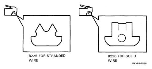
Figure 26 MMP Connectors for Stranded and Solid Wire
