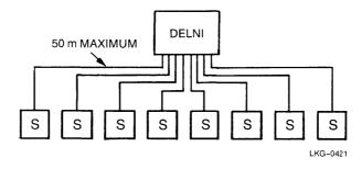
Figure 2 Standalone DELNI Configuration
