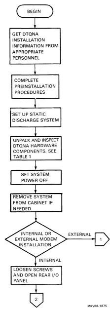
Figure 5 Installation Flowchart for DTQNA in BA23A, BA123, and H9642 Systems (Sheet 1 of 5)
