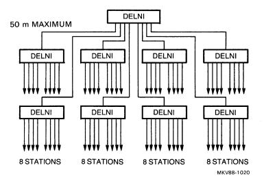
Figure 3 Standalone Cascaded DELNI Configuration
