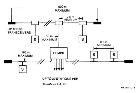
Figure 13 Connecting a DEMPR to a Standard Ethernet Coaxial Cable Segment
