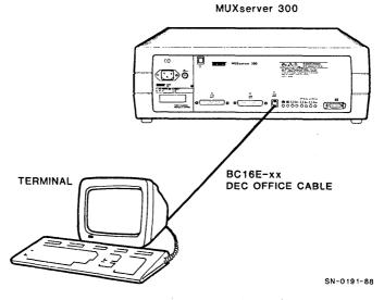
Figure 12 Supervisor Port Connection
