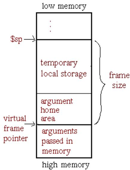
**Figure 5–12: Variable-Size Stack Frame**
