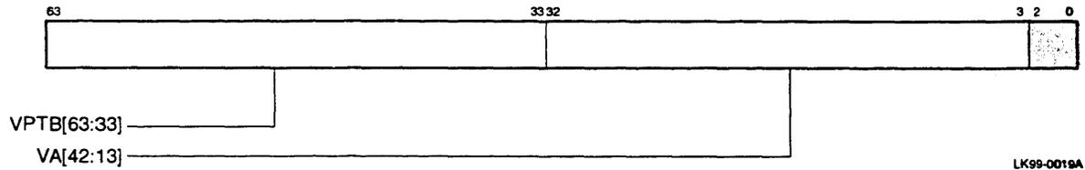
Figure 5–14 shows IVA\_FORM when I\_CTL(VA\_48) equals 1 and I\_CTL(VA\_FORM\_32) equals 0.
