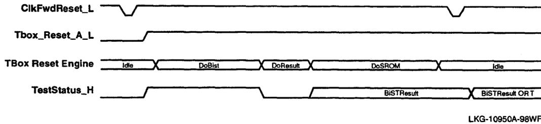
Figure 11–2 TestStat\_H Pin Timing During Built-In Self-Initialization (BiSI)
