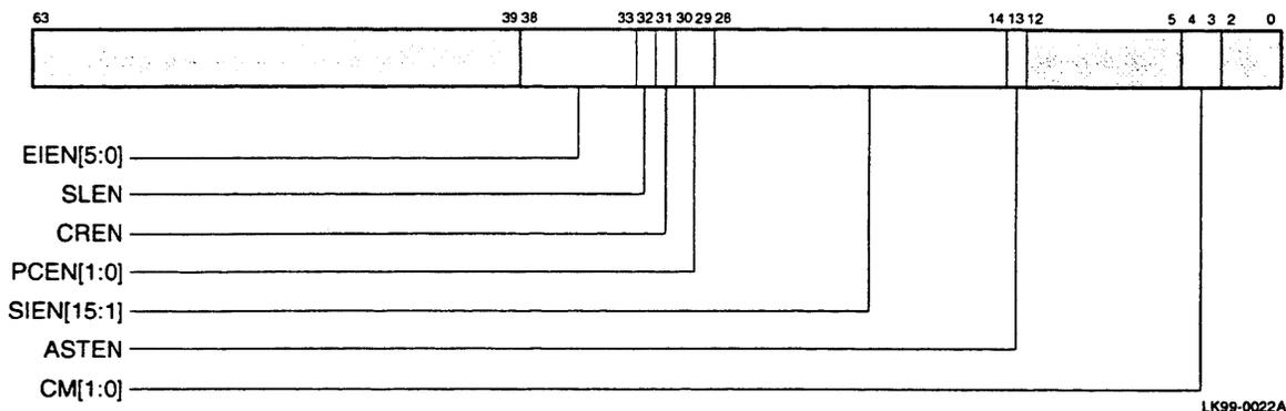
Table 5–5 describes the interrupt enable and current processor mode register fields.
