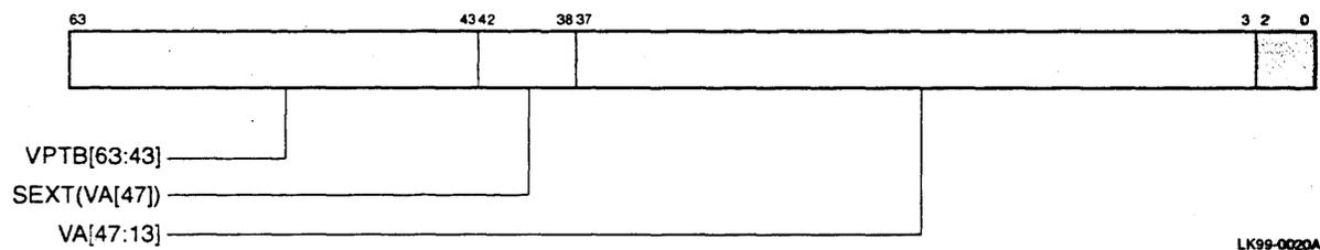
Figure 5–15 shows IVA\_FORM when I\_CTL(VA\_48) equals 0 and I\_CTL(VA\_FORM\_32) equals 1.
