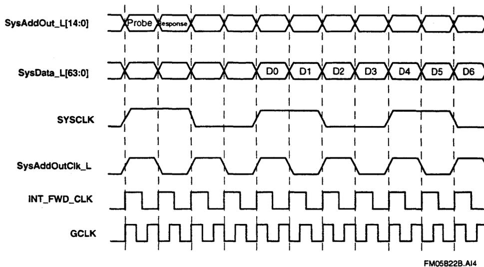
In fast data mode, movement of data into the 21264A requires turning around the SysData bus that is being actively driven by the 21264A. Given a SysDc fill command (ReadDataError, ReadData, ReadDataShared, ReadDataShared/Dirty, ReadDataDirty), the 21264A responds as follows:
