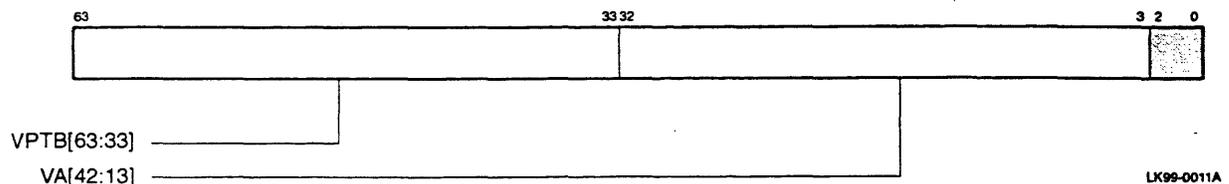
Figure 5–6 shows VA\_FORM when VA\_CTL(VA\_48) equals 1 and VA\_CTL(VA\_FORM\_32) equals 0.
